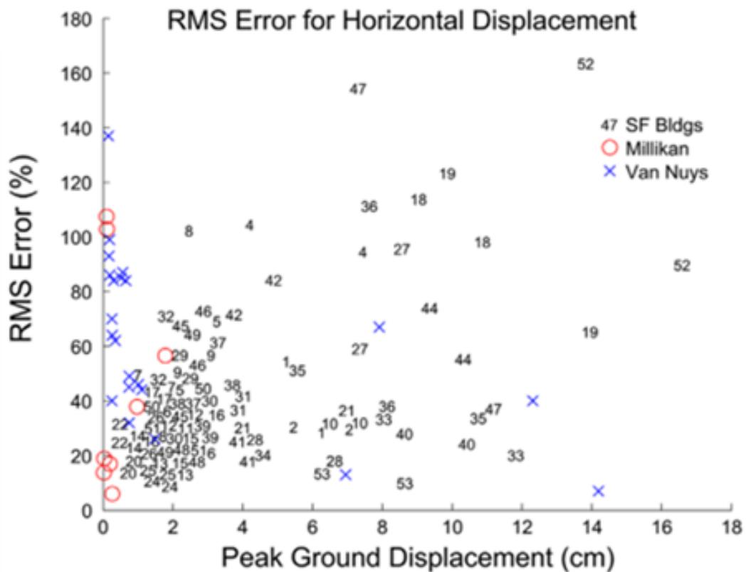
Figure 1.6. PGD and RMS error for the horizontal displacements of 54 buildings [7].
