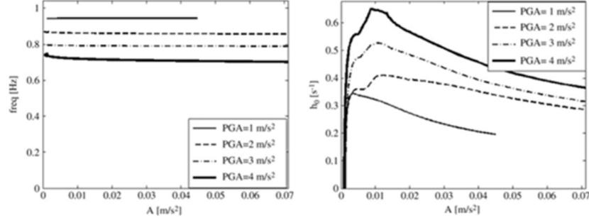
Figure 1.8. The change in the frequency and the instantaneous damping coefficient for the beam experiment [12].
