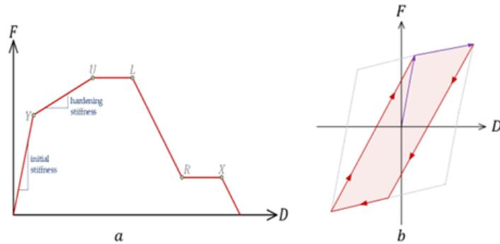
Figure 4.4. The backbone curve and YULRX model (a) and the cyclic energy dissipation.
