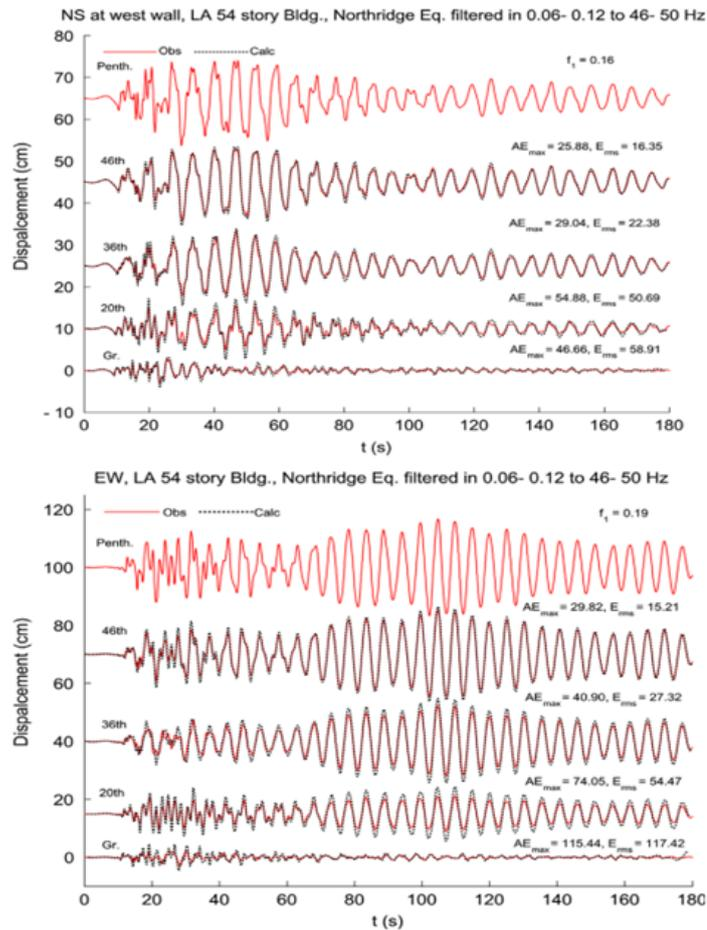
Figure 1.7. The estimated and recorded story displacements at various floor levels of a 54-story office building located in Los Angeles [7].
