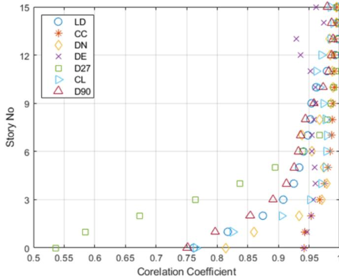
Figure A.13. Story-wise correlation coefficients between the actual and convolved waves with respect to top of the Fr15B.
