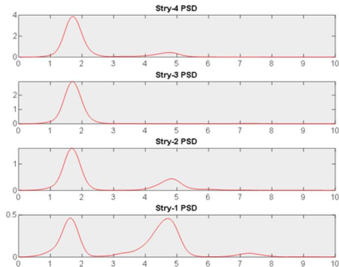
Figure 2.4. The PSD estimate for the Chile earthquake.
