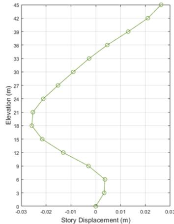
Figure 5.6. The lateral story displacements for the Fr15A subjected to the DN earthquake scaled by a factor of 2.
