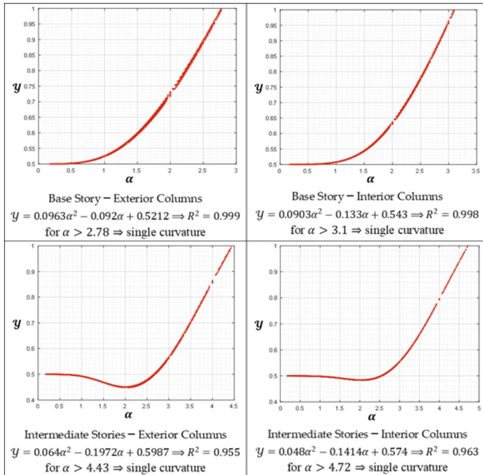
Figure 3.5. The relation between the PI and the  $\alpha$  established from curve fitting of 3136 analyses.
