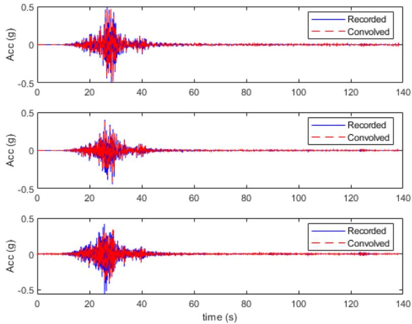
Figure 4.8. Comparison between the convolved and actual responses of the top, seventh, and the first floors for the Fr15A under DE earthquake.
