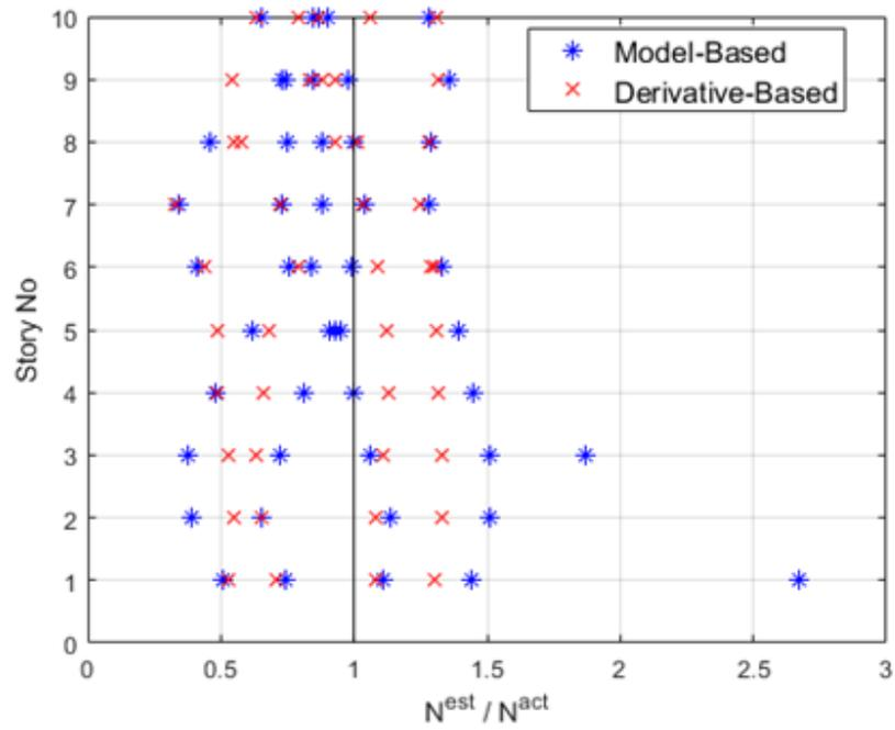
Figure C.1. Ratio of the estimated / actual axial forces for the columns of Fr10A given per story.
