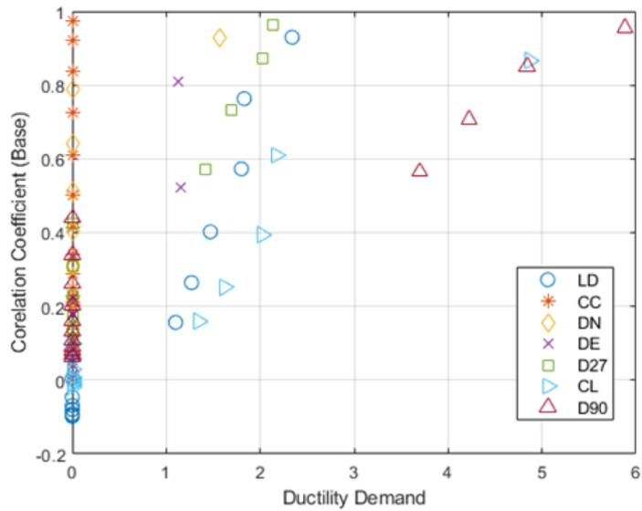
Figure A.33. Correlation coefficients between the actual and convolved waves with respect to base vs the roof ductility demand for W15 (the earthquakes are scaled with 2.5).
