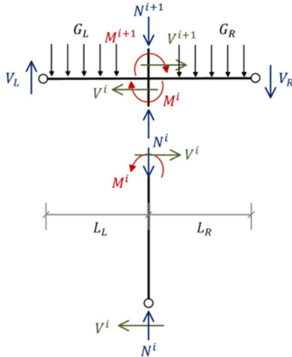
Figure 3.3. Joint equilibrium for a beam-column joint.
