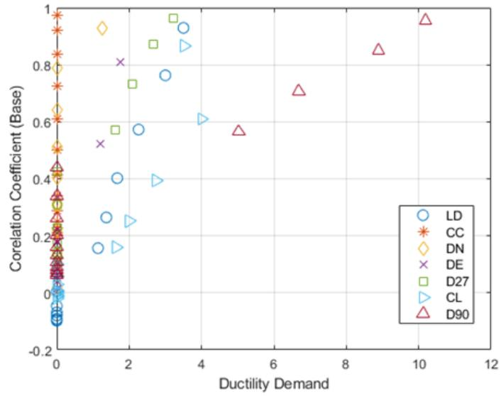
Figure A.32. Correlation coefficients between the actual and convolved waves with respect to base vs the story ductility demand for W15 (the earthquakes are scaled with 2.5).
