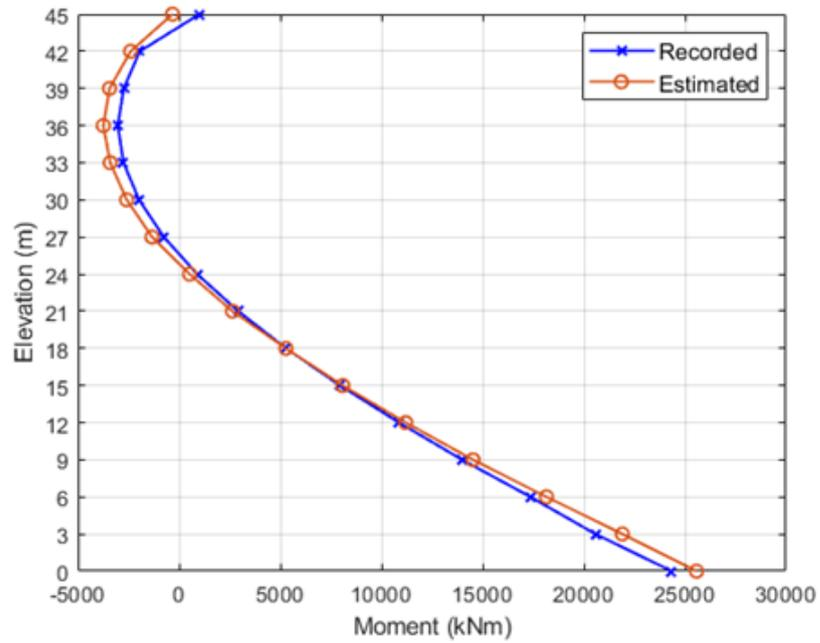
Figure 5.9. Recorded and estimated bending moments for the structural wall in D15.
