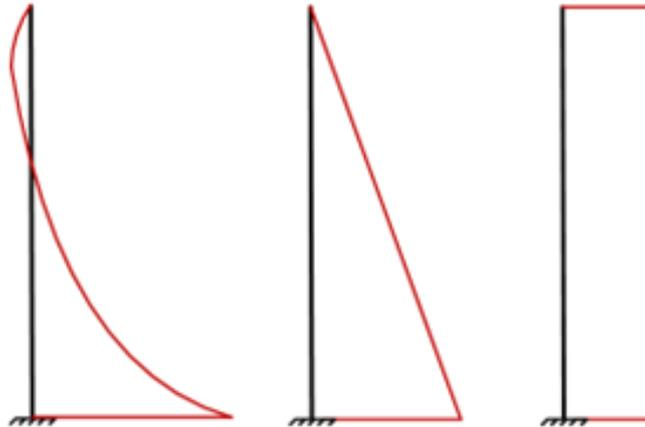
Figure 3.9. Axial load and moment profile options for the program which is coded for the structural walls.
