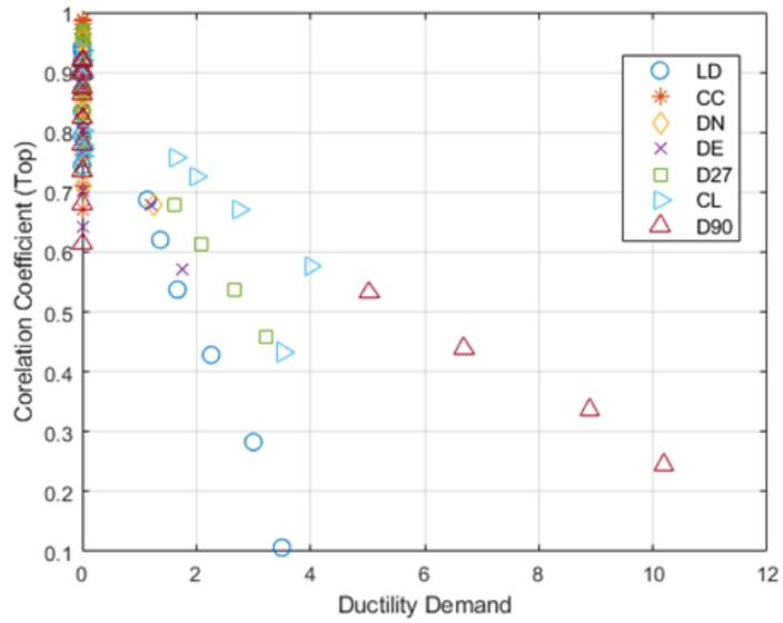
Figure A.26. Correlation coefficients between the actual and convolved waves with respect to top vs the story ductility demand for W15 (the earthquakes are scaled with 2.5).
