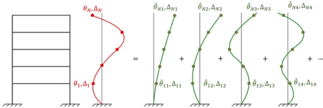
Figure 3.6. The approximation for the joint rotations at any given displacement profile.
