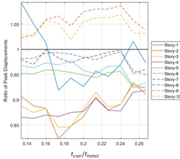
Figure 5.16. Change of the peak story displacements with varying separation point of the data for which a different polynomial is fit.
