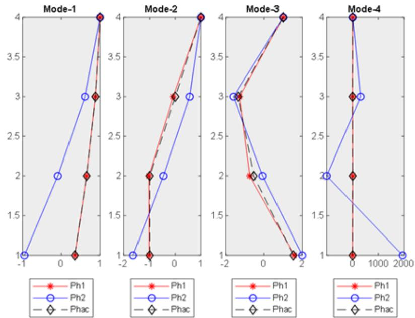
Figure 2.5. The estimated mode shapes under the Chile earthquake obtained via 2 different approaches and the actual mode shape (bandwidth of the bandpass Filter is 0.015 Hz).
