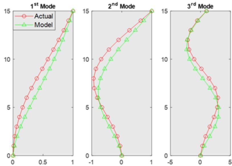
Figure 5.3. The first three x-direction mode shapes of the real-life and model buildings.
