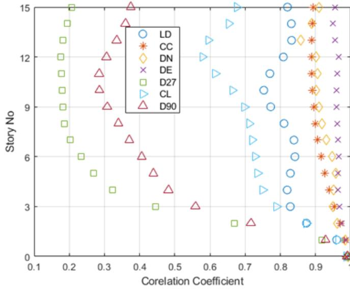
Figure A.17. Story-wise correlation coefficients between the actual and convolved waves with respect to base of the Fr15A.
