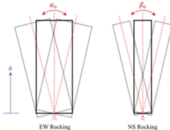
Figure 1.13. The schematic representation of the rocking motion [16].
