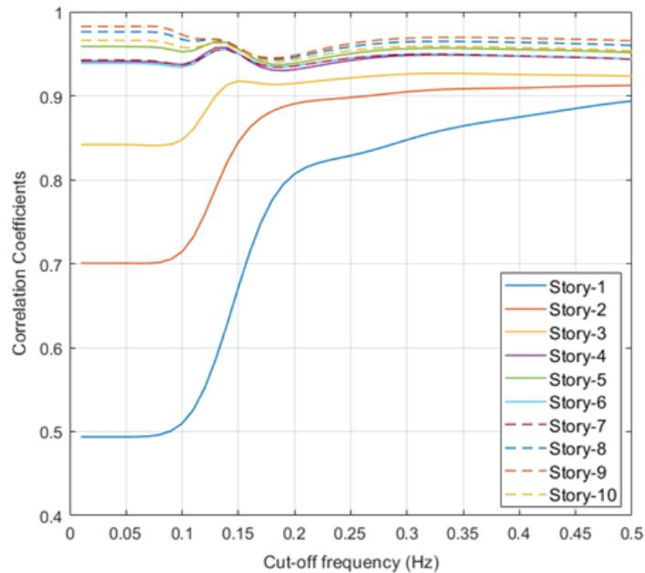
Figure 5.12. Correlation coefficients between the actual and noisy story displacements obtained by double integration vs the cut-off frequencies of the high pass filter applied to the noisy acceleration responses.
