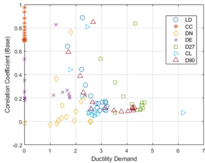
Figure A.31. Correlation coefficients between the actual and convolved waves with respect to base vs ductility demand for D15.
