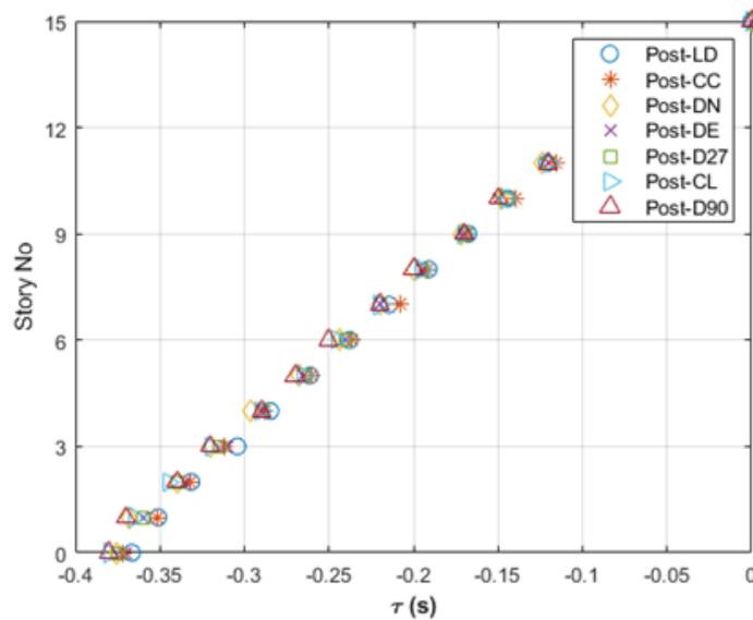
Figure 4.10. The post-earthquake shear wave velocity profiles of the Fr15A.
