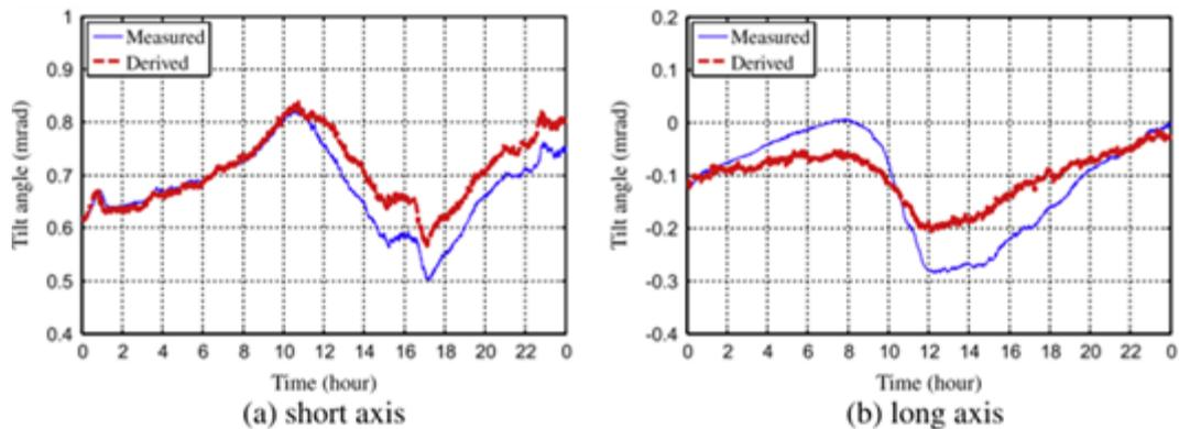
Figure 1.12. The measured and the derived tilts at the height of 443.4 m [14].
