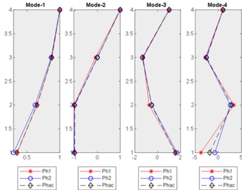
Figure 2.6. The estimated mode shapes under the Chile earthquake obtained via 2 different approaches and the actual mode shape (bandwidth of the bandpass Filter is 0.1 Hz).
