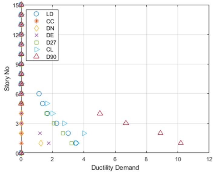
Figure A.10. The story ductility demand values for W15 under all earthquake excitations (the earthquakes are scaled with 2.5)..
