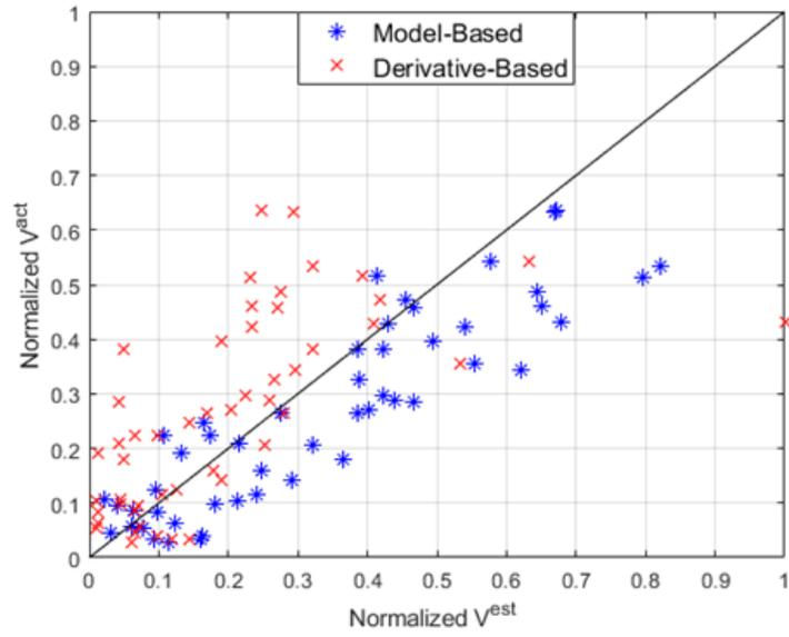
Figure C.6. Ratio of the estimated / actual normalized shear forces for all of the columns of Fr10A.
