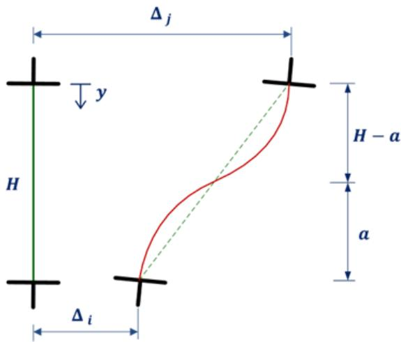
Figure 3.1. The nonlinear flexural fiber model used in both programs in order to find the displacements of members at any given point.
