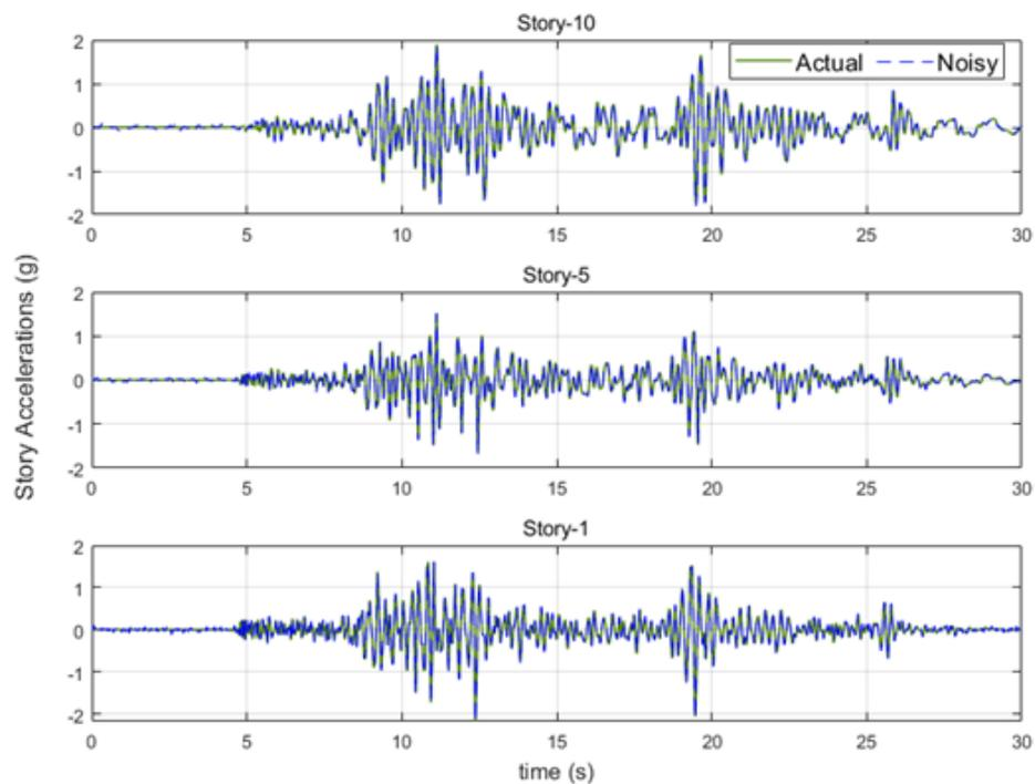
Figure 5.11. The original and the noisy acceleration data for the 1st, 5th, and 10th stories of Fr10A.
