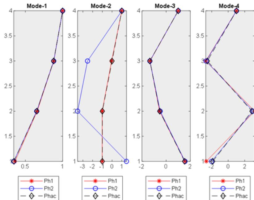
Figure 2.3. The estimated mode shapes obtained via 2 different approaches under the white noise excitation and the actual mode shape (bandwidth of the bandpass filter is 0.015 Hz).
