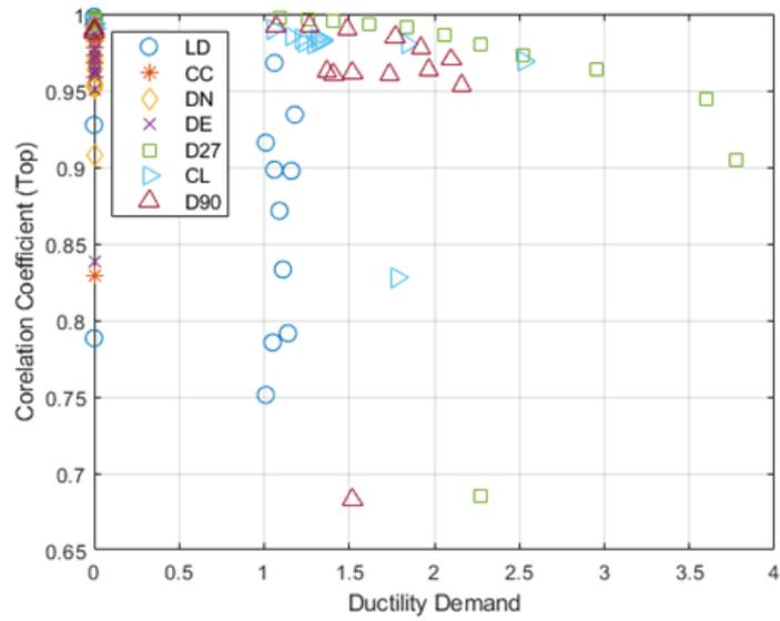
Figure A.24. Correlation coefficients between the actual and convolved waves with respect to top vs the ductility demand for Fr15C.
