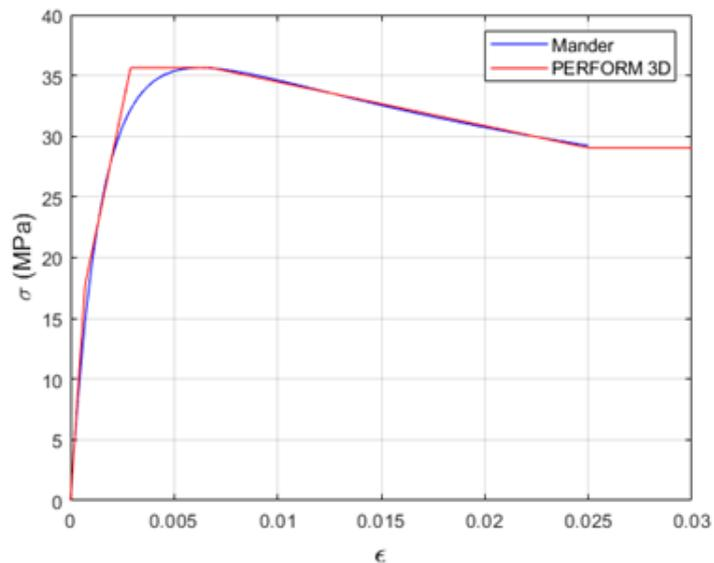
Figure 4.3. Confined concrete stress-strain curve and adjustment to the PERFORM 3D.
