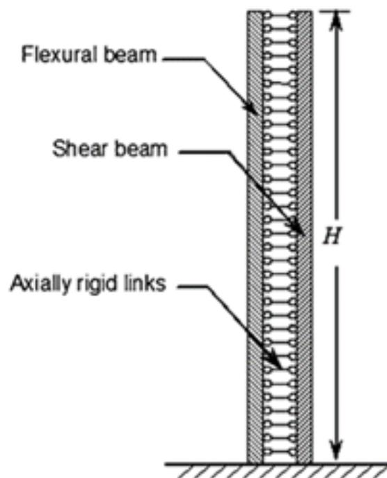
Figure 1.2. The continuum model including both the shear and flexural models [3].
