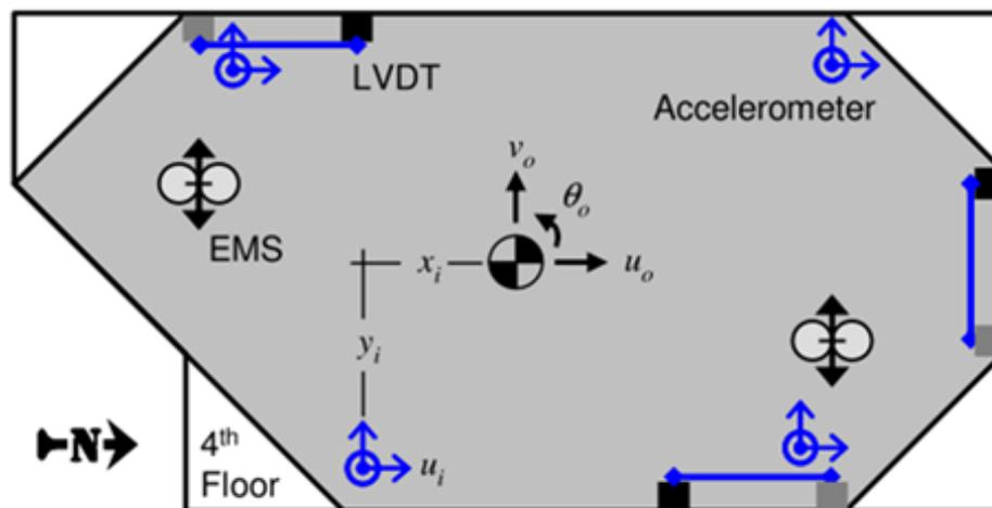
Figure 1.1. The sensor configuration of the 4-story RC building [1].
