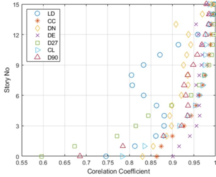
Figure A.12. Story-wise correlation coefficients between the actual and convolved waves with respect to top of the Fr15A.
