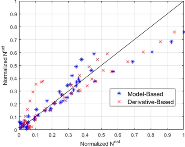
Figure B.4. Ratio of the estimated / actual normalized axial forces for all of the columns of Fr10A.
