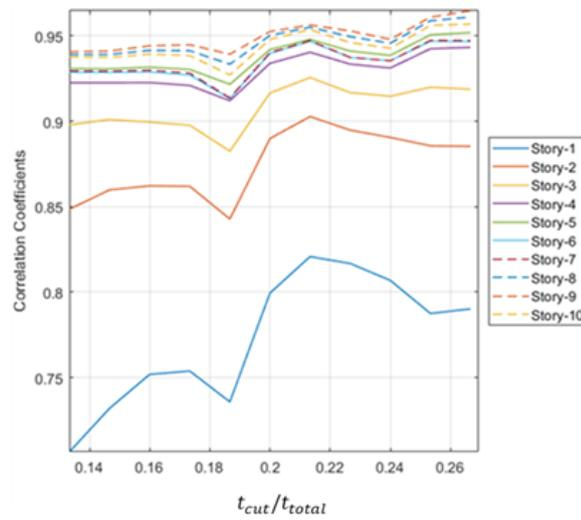
Figure 5.15. Change of the correlation coefficient with varying separation point of the data for which a different polynomial is fit.
