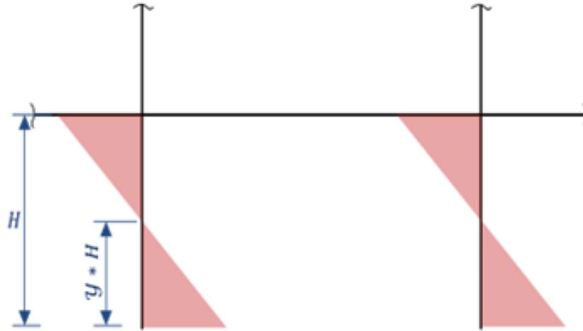
Figure 3.4. Location of the point of inflection of column as a fraction of height.
