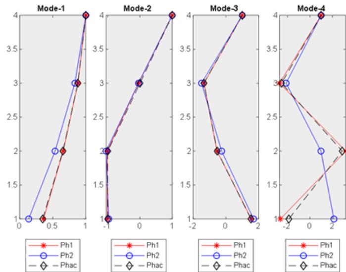
Figure 2.2. The estimated mode shapes obtained via 2 different approaches under the white noise excitation and the actual mode shape (bandwidth of the bandpass Filter is 0.05 Hz).
