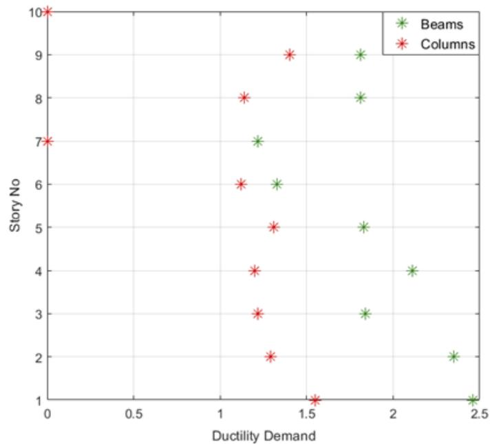
Figure 5.4. Ductility demand for Fr10A subjected to DN scaled by a factor of 2.
