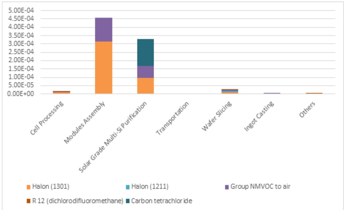
Figure 4.11. Decomposition of substances affecting ozone layer depletion potential.
