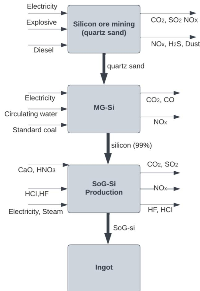
Figure 2.2. Scheme of converting silica ore to solar grade silicon.
