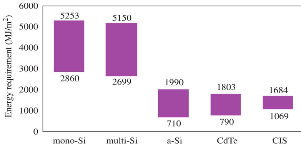
Figure 2.5. Energy requirements for the manufacturing of photovoltaic solar panels (Peng et.al., 2013).
