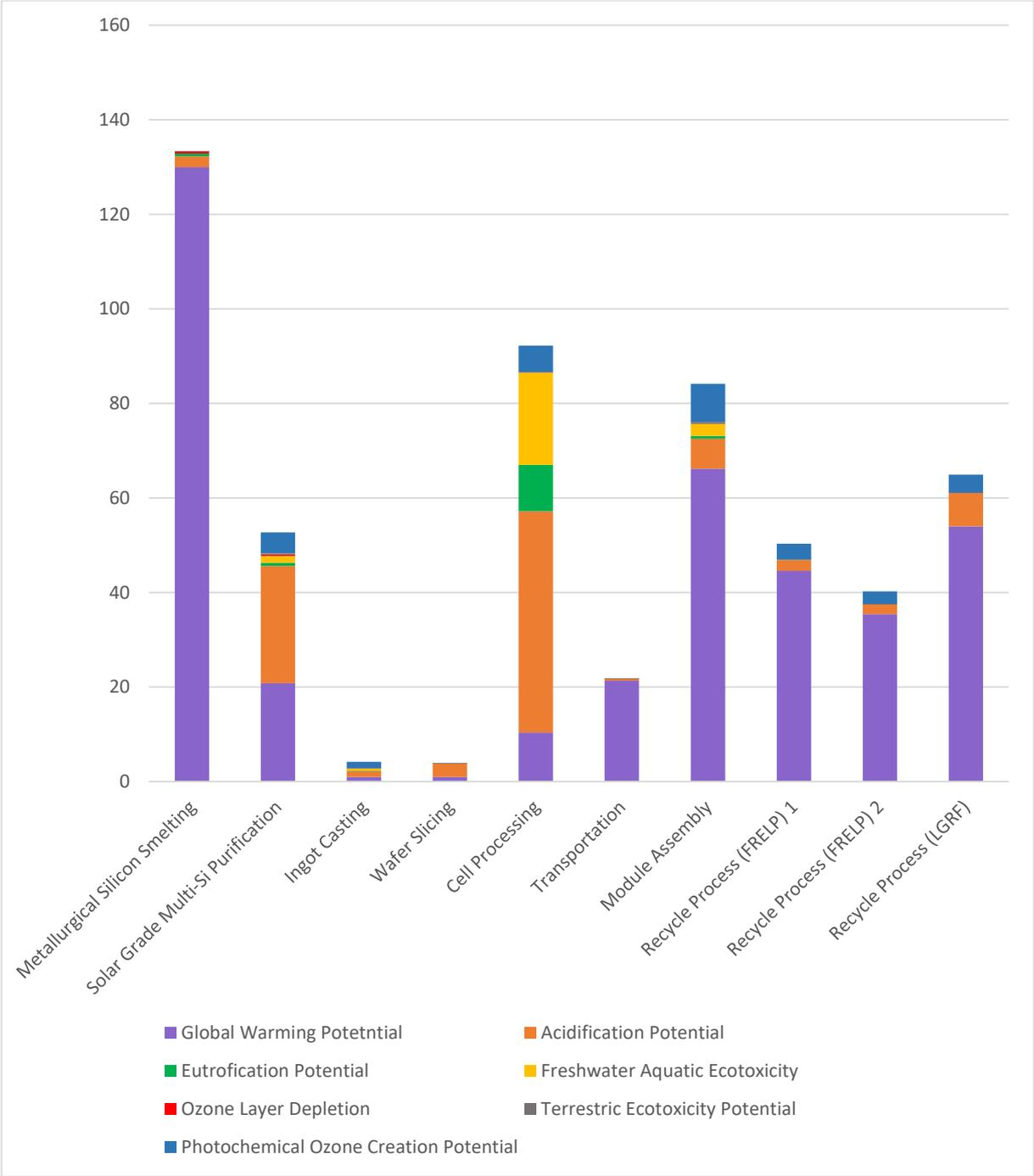
Figure 4.3. Normalization of environmental impact categories in multi-Si solar panel life cycle [kg].
