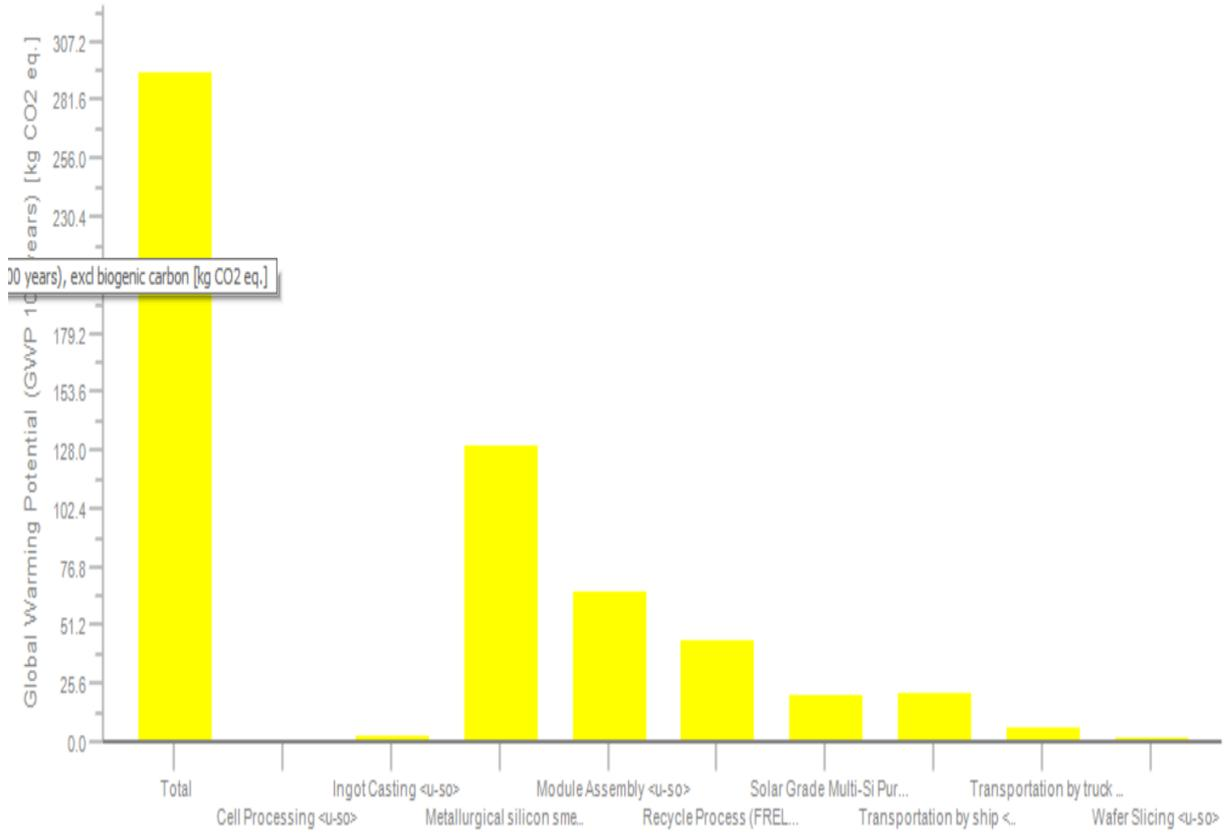
Diagram:Life Cycle of multi-Si Solar Panel - Outputs
