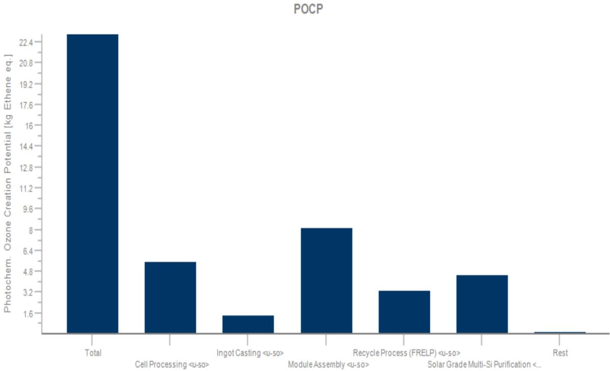
Diagram:Life Cycle of multi-Si Solar Panel - Outputs
