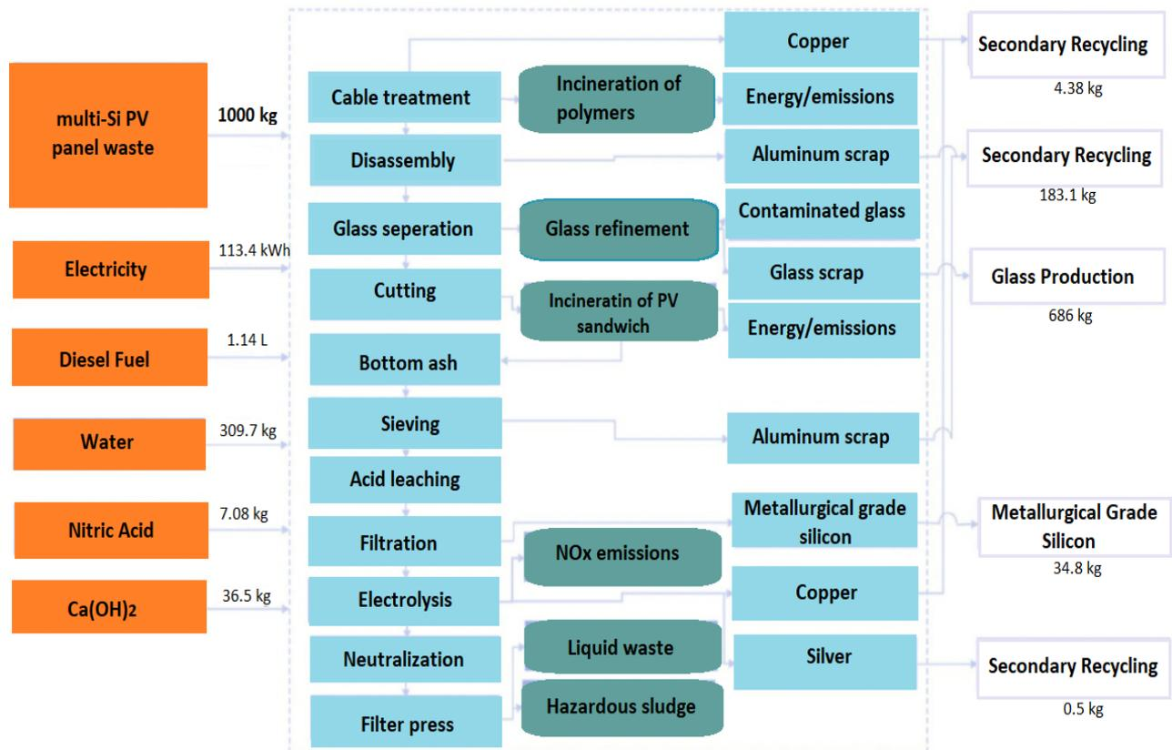
Figure 2.13. Process diagram for the FREL P process of multi-Si PV waste (mechanical and chemical combined version).
