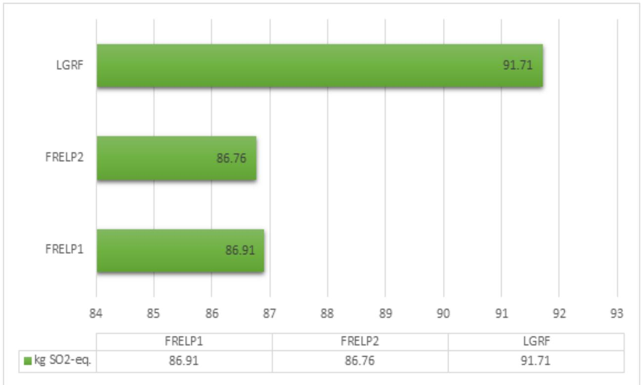
Figure 5.2. Comparison of three different recycling scenarios in terms of AP over the entire life cycle of a multi-Si PV panel.
