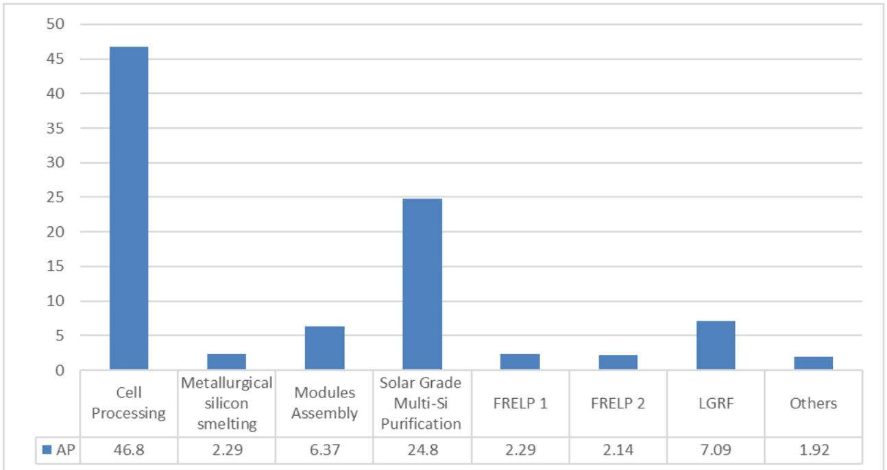
Figure 4.6. Acidification potential [kg SO<sub>2</sub>-equivalent].
