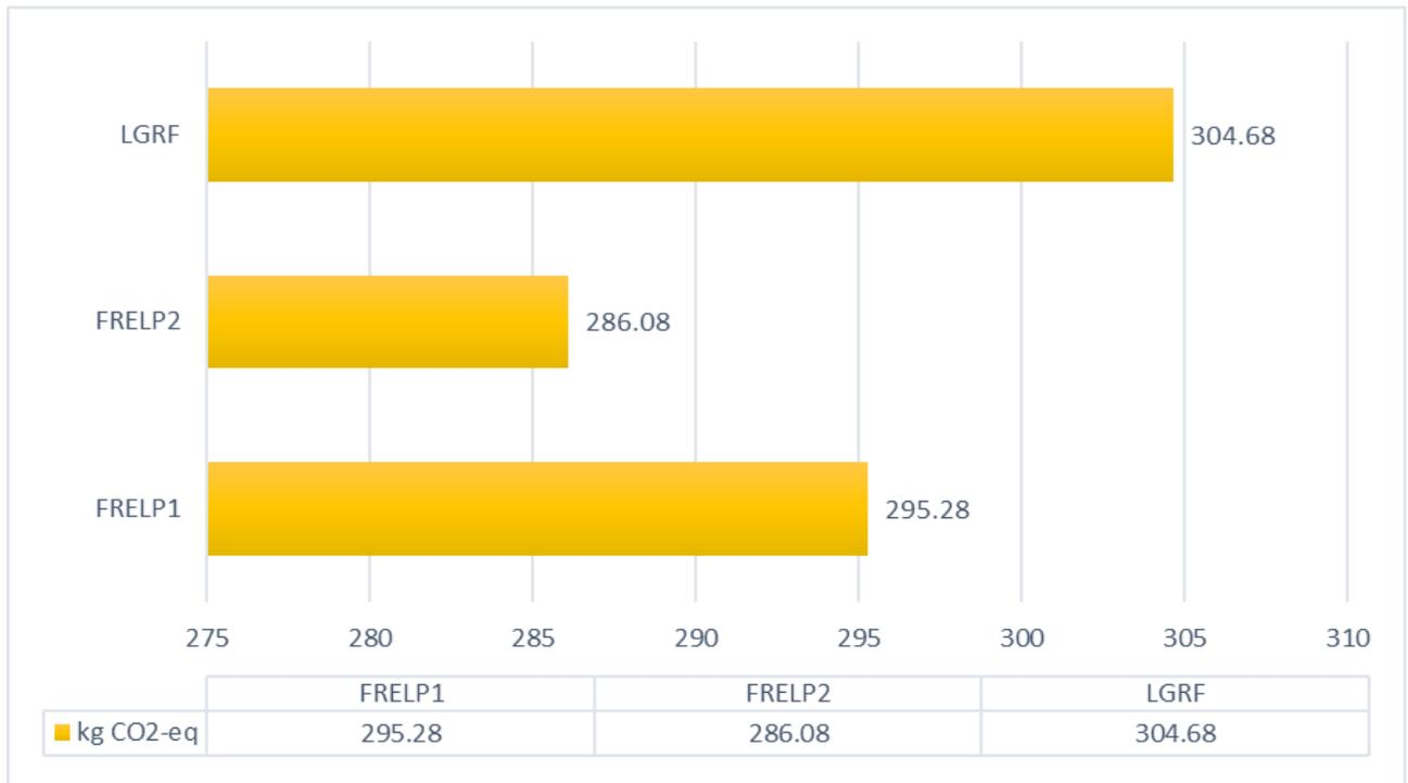
Figure 5.1. Comparison of three different recycling scenarios in terms of GWP over the entire life cycle of a multi-Si PV panel.
