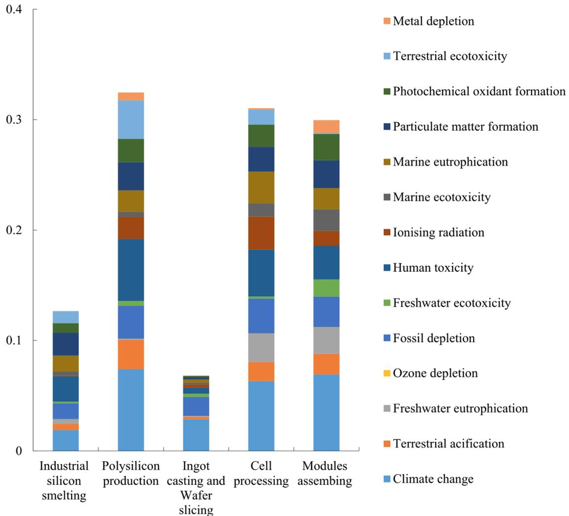
Figure 2.9. Environmental effects of multicrystalline solar panels (Huang et al., 2017).
