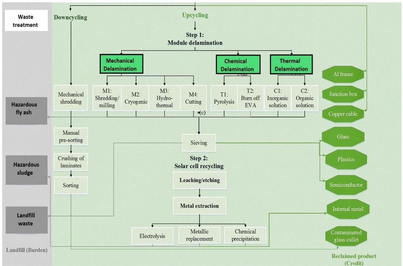
Figure 2.12. Delamination pathways to recycle multi-Si PV panels (Deng et. al., 2019).
