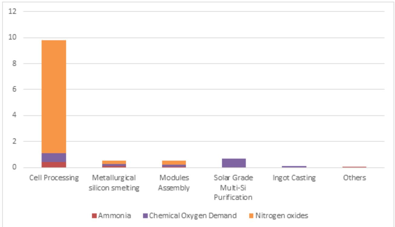
Figure 4.9. Decomposition of substances affecting eutrophication [kg PO<sub>4</sub>- equivalent].
