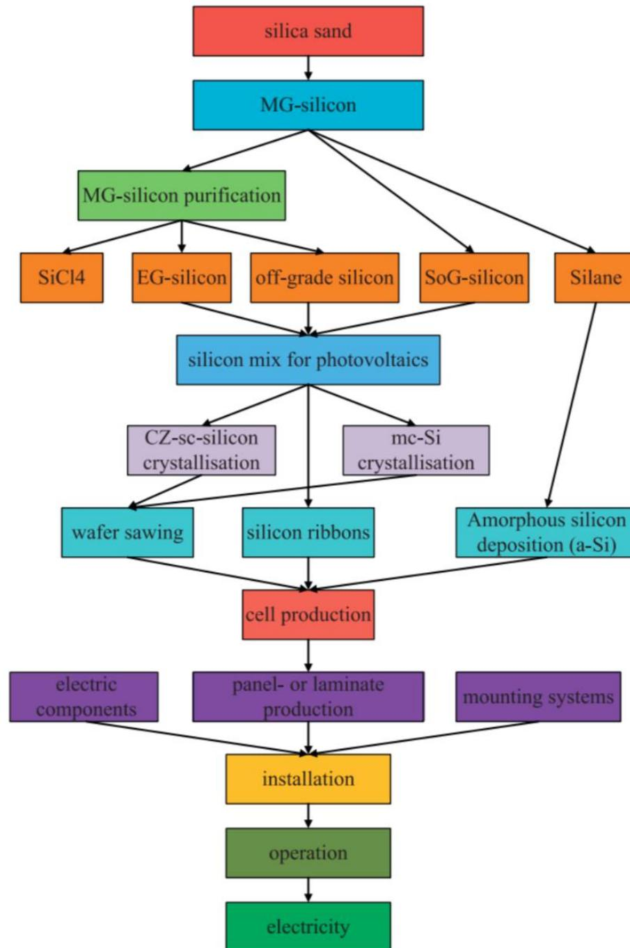
Figure 2.7. The LCA diagram of multi-Si PV panels (Peng et al., 2013).
