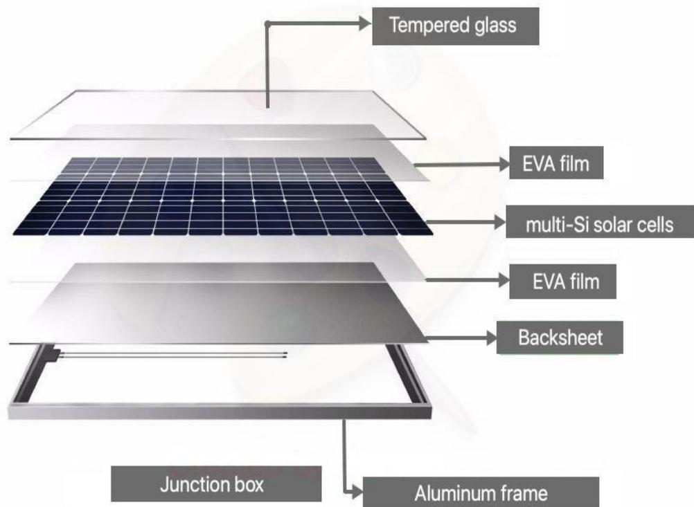
Figure 2.16. Structure of multicrystalline solar panel.
