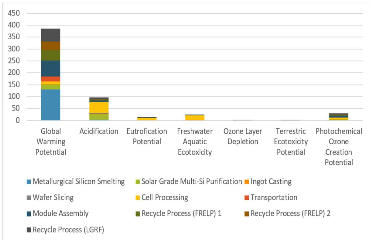
Figure 4.2. Characterization of environmental impact categories in multi-Si solar panel life cycle [kg].
