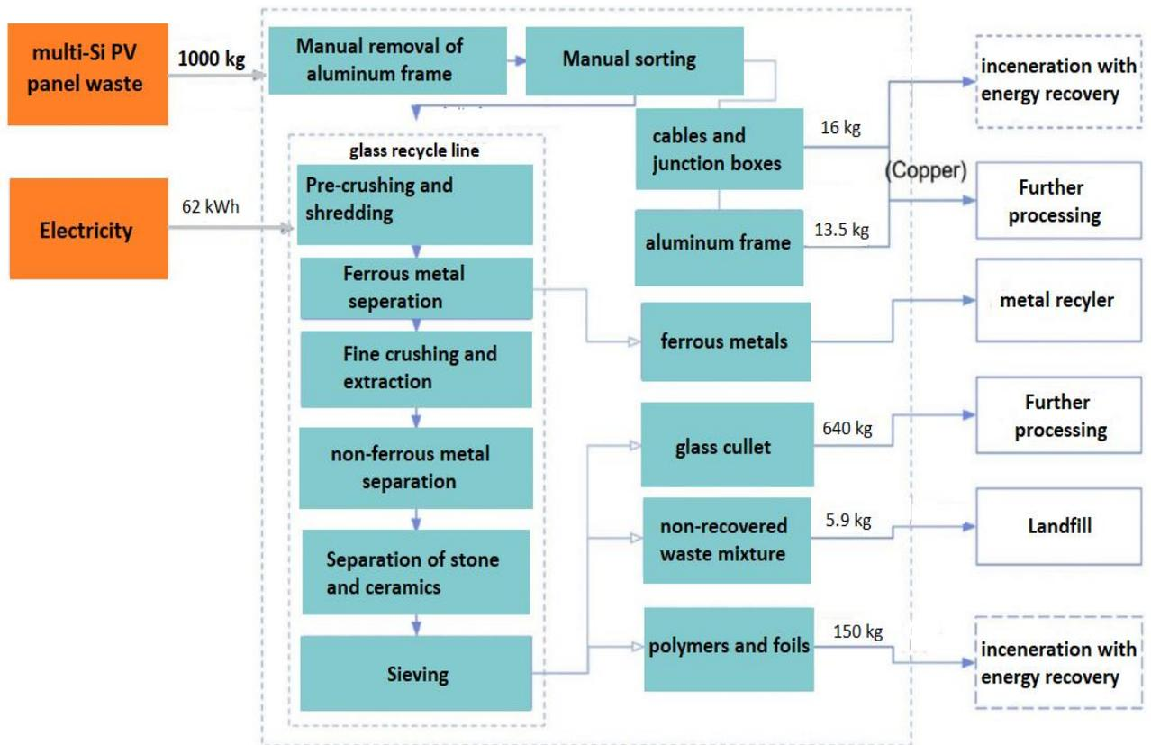
Figure 2.14. Process diagram for the LGRF process of multi-Si PV waste.
