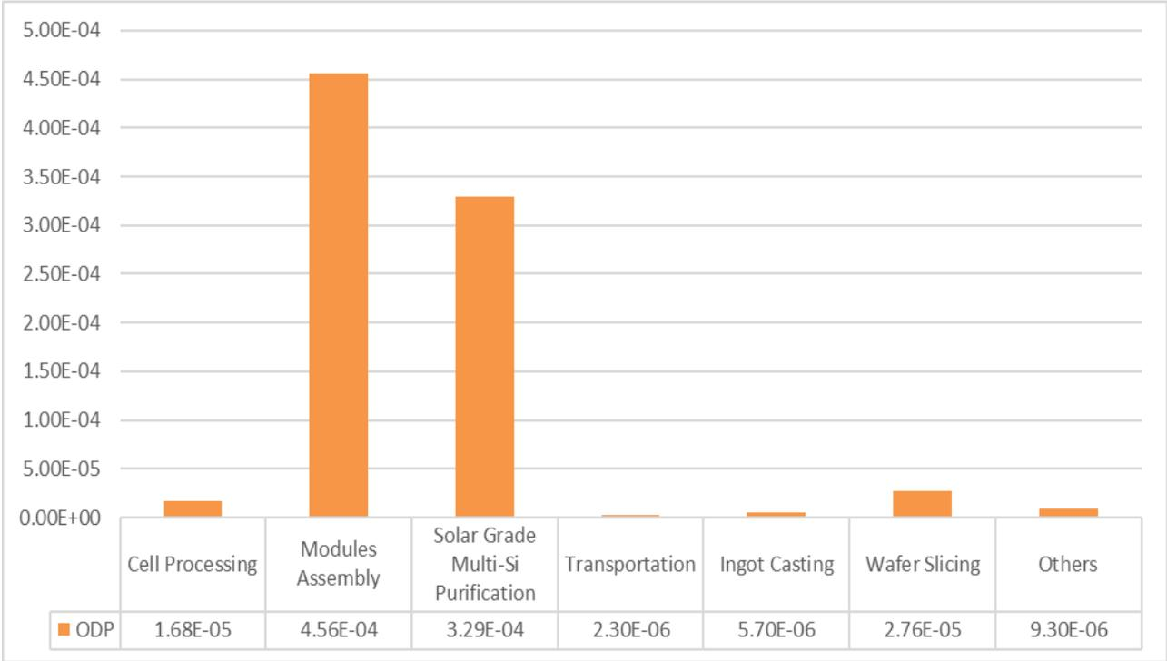
Figure 4.10. Ozone layer depletion potential [kg R11-equivalent].
