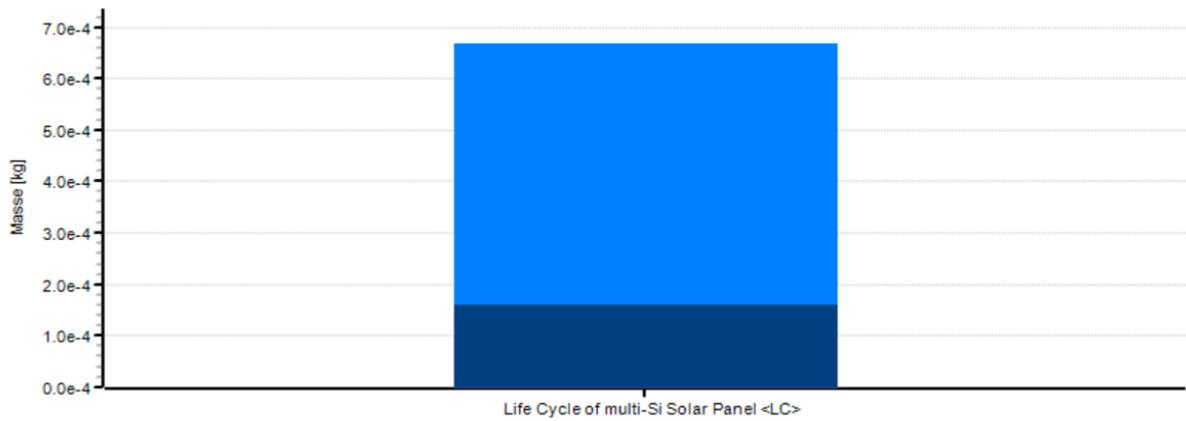
GaBi diagram:Photochemical ozone\_LCA of multi-Si Solar Panel - Inputs
