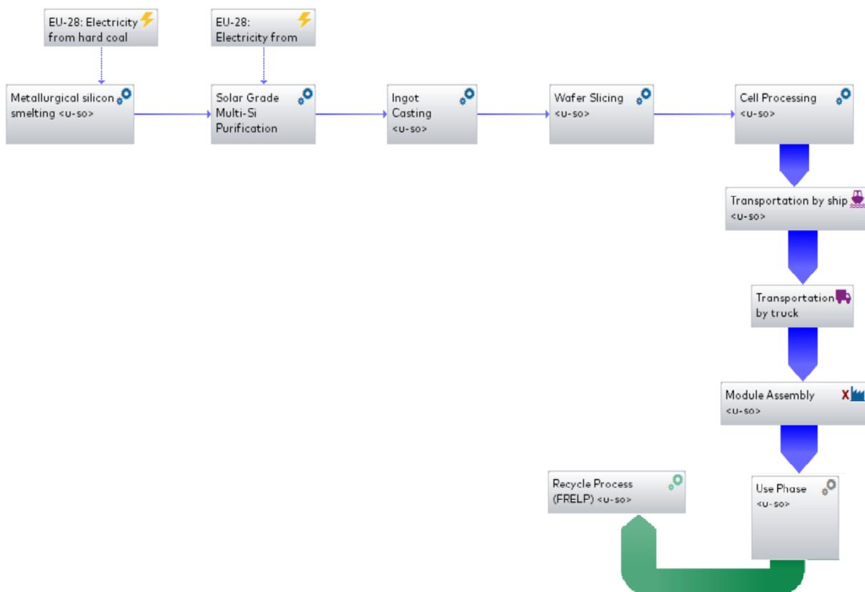
Figure 4.1. Gabi 9.5 Software screenshot for LCA of multi-Si solar panel
