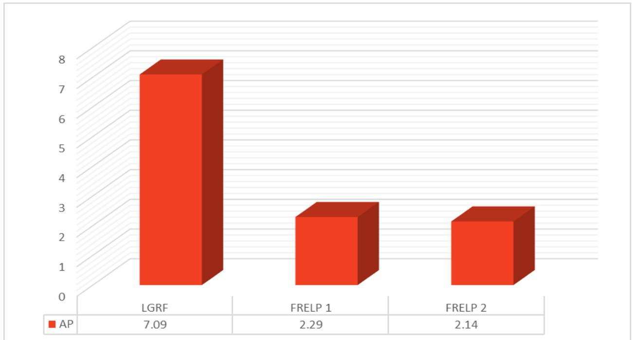
Figure 4.18. Acidification potential of recycling scenarios [kg SO<sub>2</sub>-equivalent].
