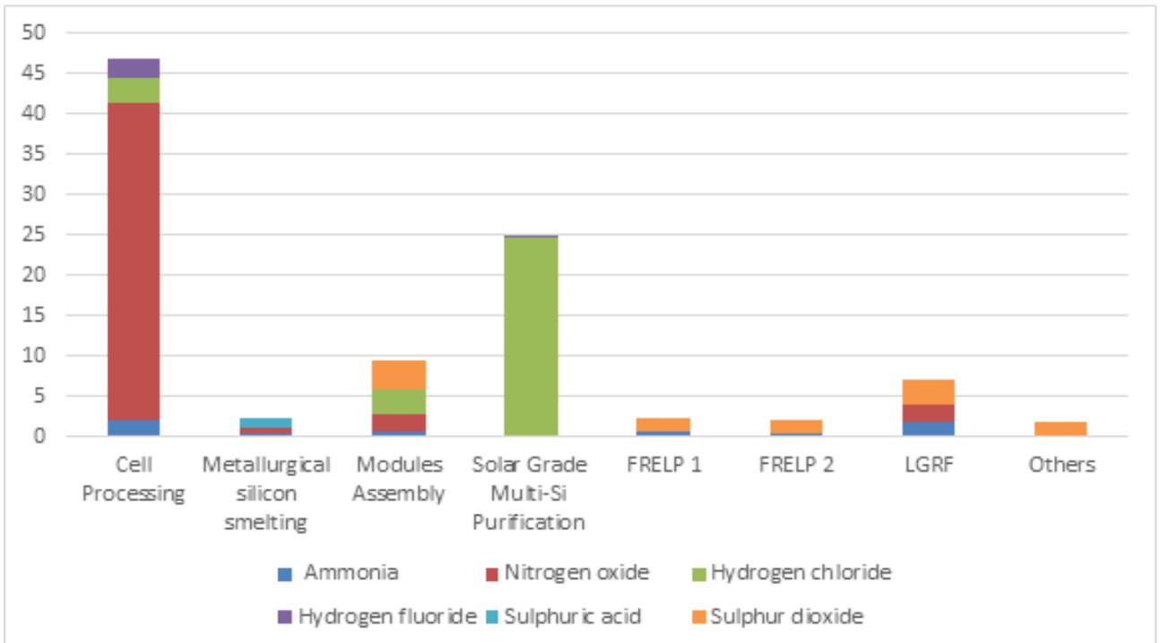
Figure 4.7. Decomposition of substances affecting acidification potential [kg SO<sub>2</sub>-equivalent].
