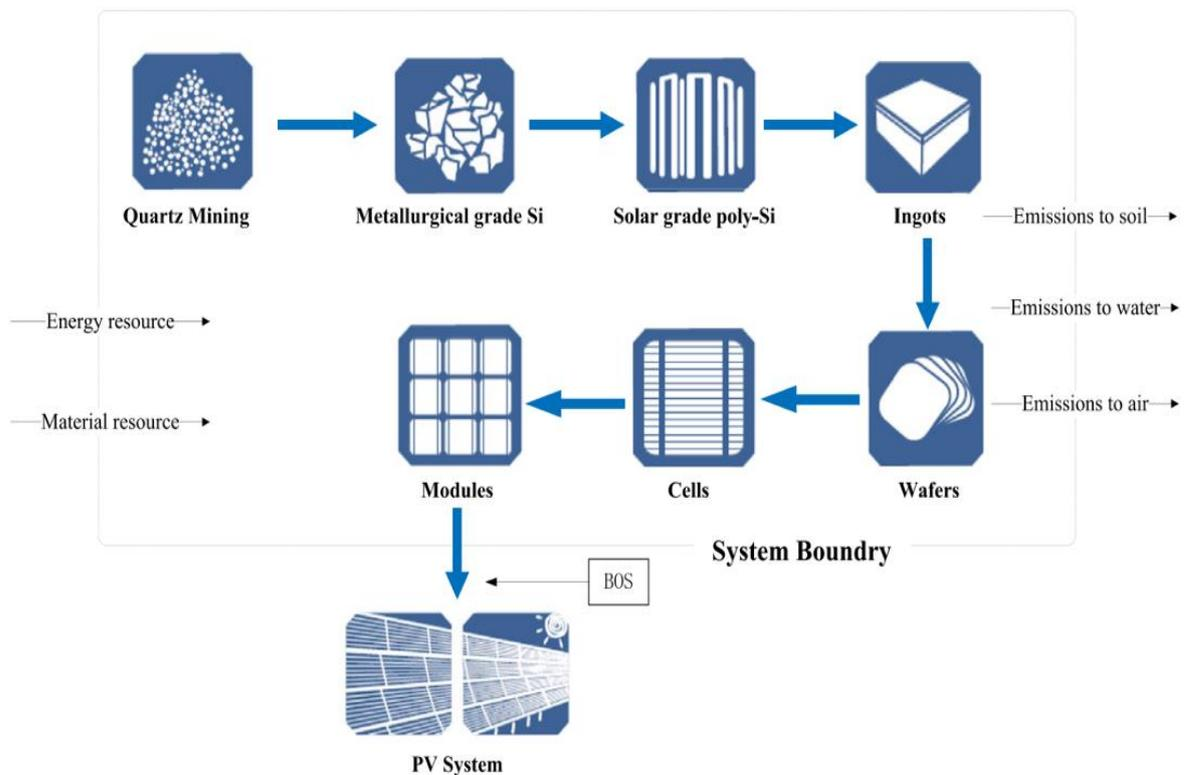
Figure 2.8. Life cycle of a multi-Si PV panel production stage (Fu et al., 2015).
