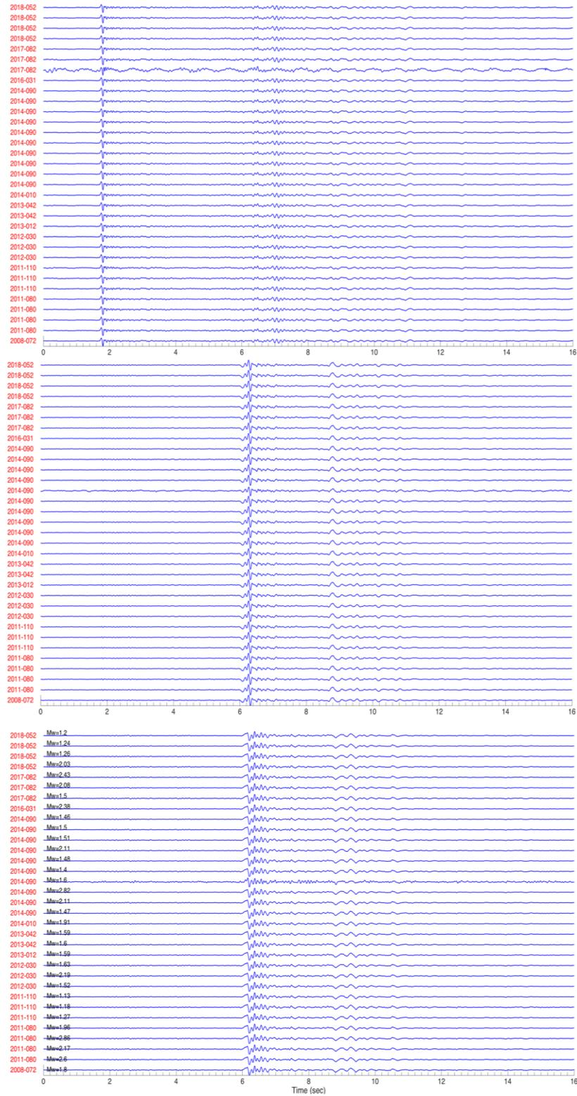
Figure 5.24. The repeating waveforms detected in Cluster 3 from the SLVM station between 2008-2018: vertical (top), N-S (middle) and E-W (bottom) components. Traces are normalized by the maximum value of each trace. The numbers on the left of the traces (red labels) shows the recording date of the event. The numbers on the traces of the E-W components shows the moment magnitudes of each event.
