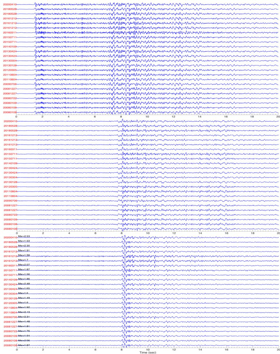
Figure 5.26. The repeating waveforms detected in Cluster 3 from the SLVT station between 2008-2020: vertical (top), N-S (middle) and E-W (bottom) components. Traces are normalized by the maximum value of each trace. The numbers on the left of the traces (red labels) shows the recording date of the event. The numbers on the traces of the E-W components shows the moment magnitudes of each event.
