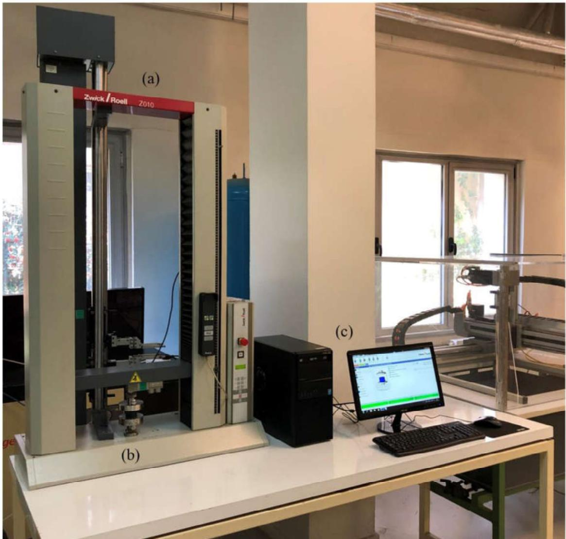
Figure 3.7. Test setup components (a) Zwick / Roell Z010, (b) compression tools and sample and (c) computer.
