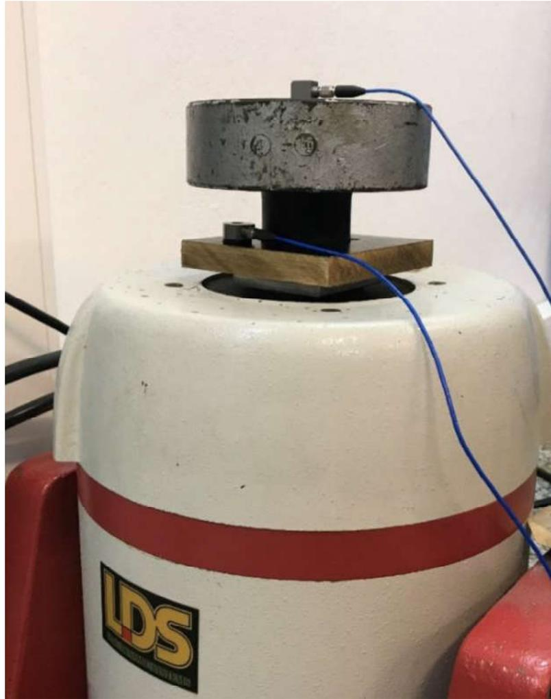
Figure 3.9. Dynamic stiffness test set-up with electromagnetic shaker, the proof mass and the accelerometers.
