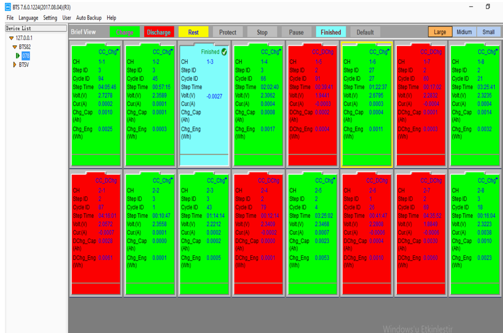
Figure 3.3. Screenshot of the BTS software used to control Neware battery cycler.
