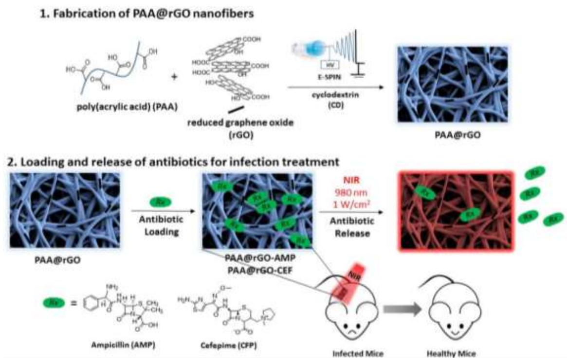
Figure 1.20. General scheme for fabrication and applications of photo-thermally triggered nanofibers [8]
