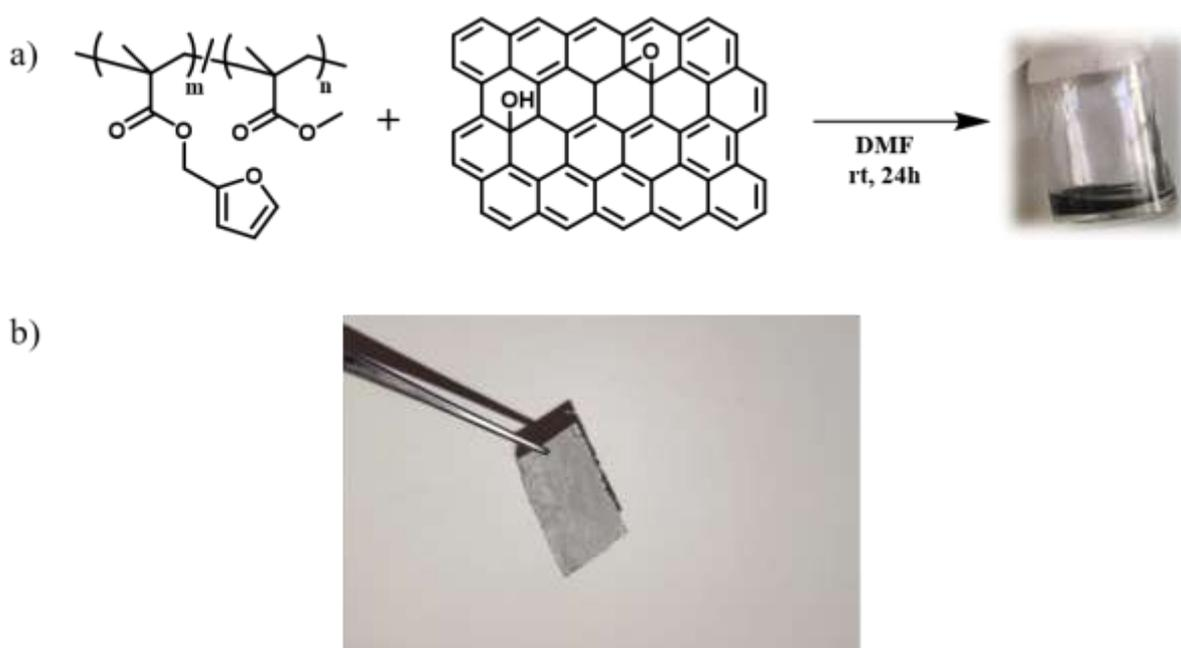
Figure 4.7. a) Schematic presentation of the preparation of r-GO-PFMA-PMMA polymer solution before applying electrospinning, b) Digital image of r-GO-PFMA-PMMA-NFs.
