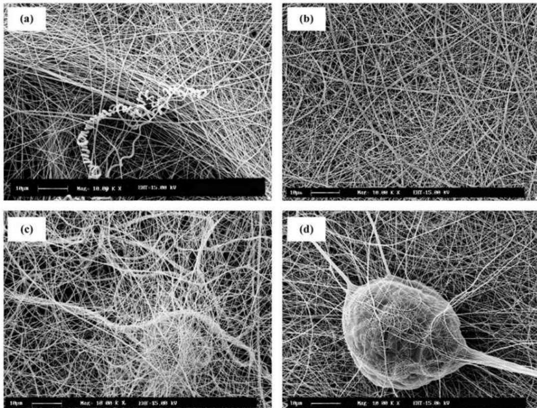
Figure 1.9. SEM images of Nylon 6 nanofibers upon increase in flow rate where (a) 0.1mL/hr, (b) 0.5 mL/hr, (c) 1 mL/hr, (d) 1.5 mL/hr [20].
