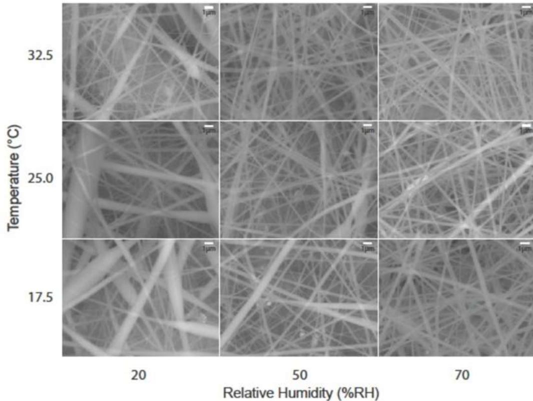
Figure 1.11. SEM images of cellulose acetate-based polymeric nanofibers under different atmospheric conditions; temperatures and humidity [26]
