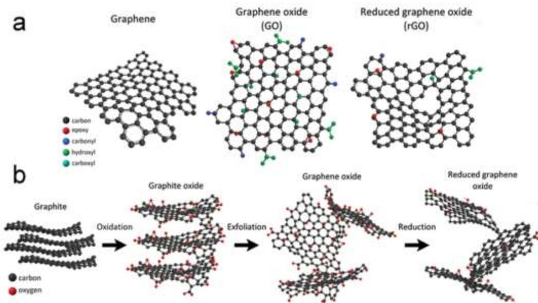
Figure 1.21. a) Scheme for the chemical structure of graphene, graphene oxide, and reduced graphene oxide; b) Schematic route for reduction of graphite to reduced graphene oxide [69].
