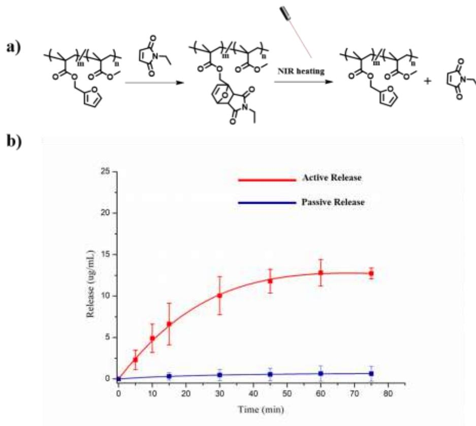
Figure 4.11. a) Reaction scheme for loading and photothermal release of E-Mal, b) Release profile of photothermally stimulated E-Mal from r-GO-PFMA-PMMA-NFs vs. non-triggered r-GO-PFMA-PMMA-NFs.
