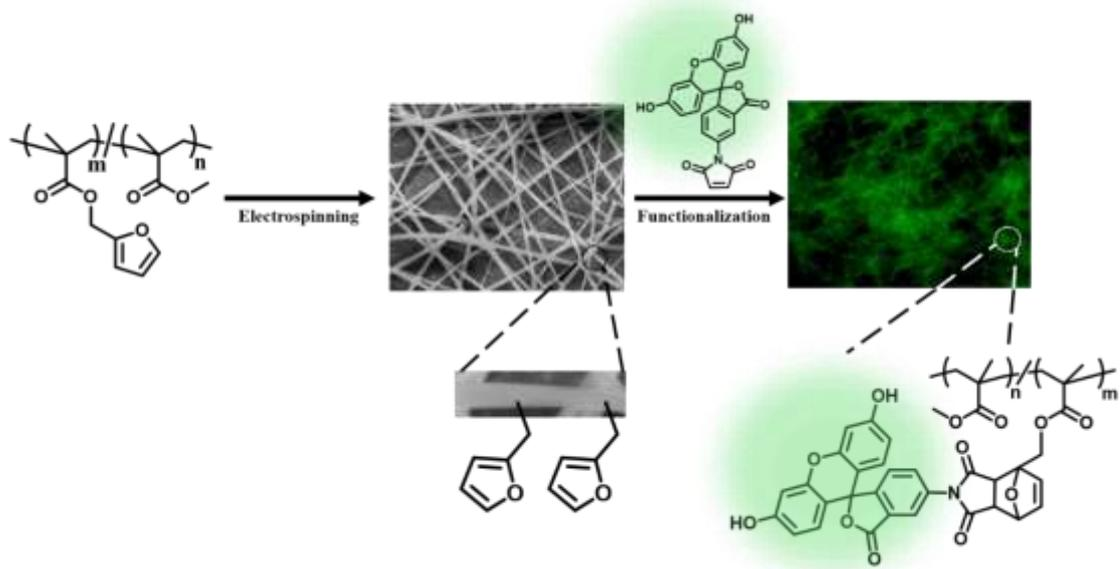
Figure 4.9. Schematic scheme for conjugation of F-Mal to r-GO-PFMA-PMMA-NFs.
