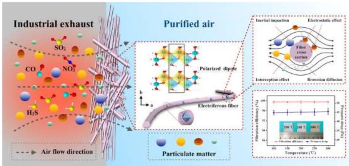
Figure 1.14. Representative filtration process through electreted PSA/PAN-B-based electrospun mats [37].
