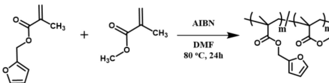
Figure 4.1. Schematic representation of the free radical polymerization to synthesize furan functionalized copolymer.
