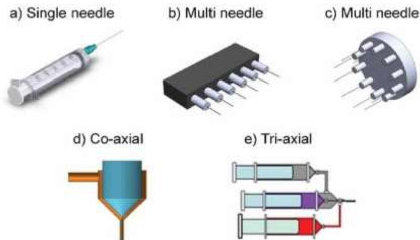
Figure 1.4. Schematic illustration of different types of electrospinning spinnerets [15].
