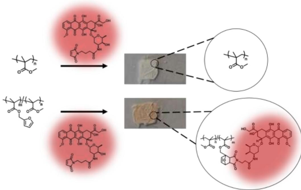
Figure 4.19. Schematic illustration of DOX-Mal loading to r-GO-PMMA-NFs and r-GO-PFMA-PMMA-NFs, respectively.
