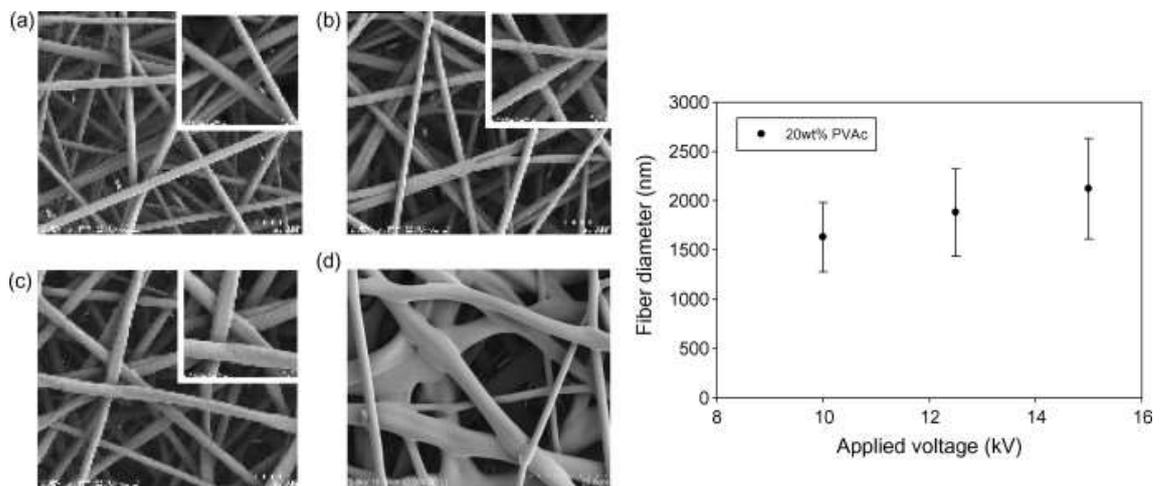
Figure 1.7. SEM images of 20 weight percent of PVAc nanofibers at different voltages on the left and on the right, the average diameter of electrospun nanofiber [19].
