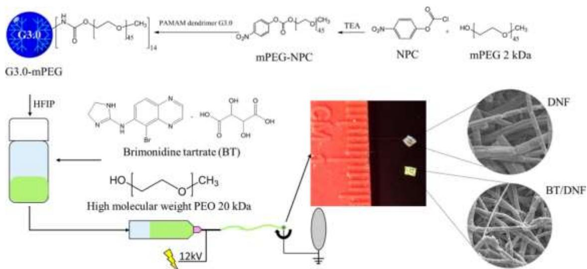
Figure 1.16. Schematic synthesis and manufacturing of dendrimer-based, brimonidine tartrate (BT) polymeric electrospun nanofibers for administering antiglaucoma [48].
