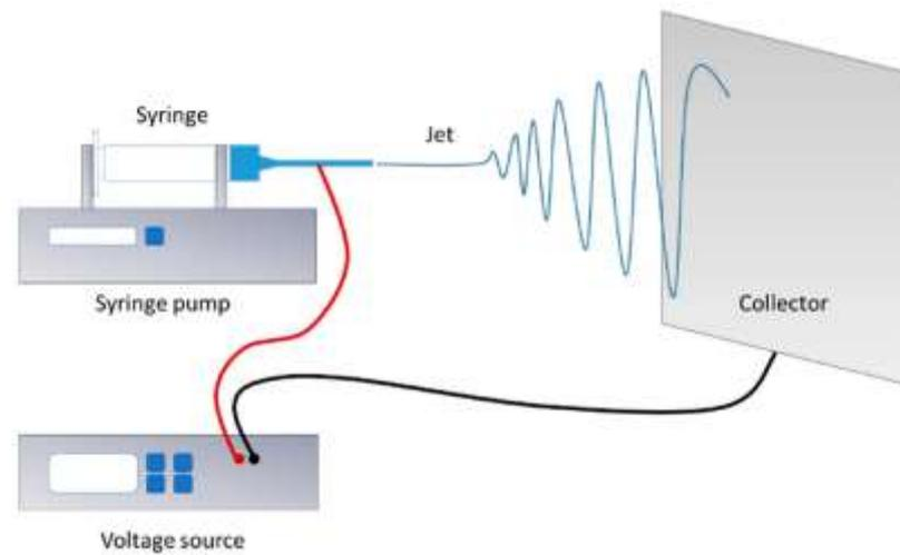
Figure 1.3. Schematic illustration of a traditional electrospinning setup [14]
