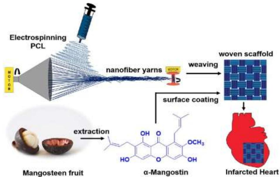
Figure 1.17. Depicted scheme for fabrication of a woven electrospun scaffold and extraction of  $\alpha$ -mangostin for cardiac patch applications [50].
