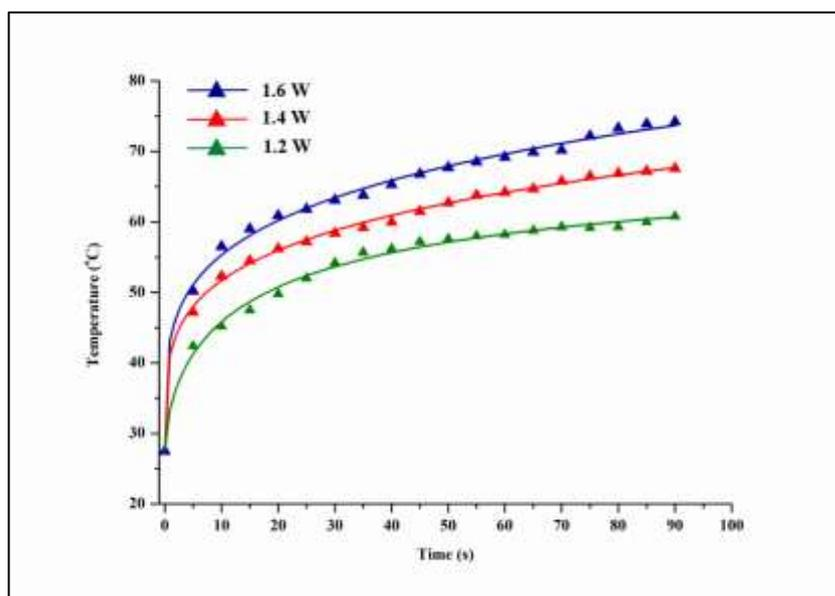
Figure 4.8. Temperature vs. time graph of the r-GO (1% w/w) containing functional nanofibrous mat under different beam powers.
