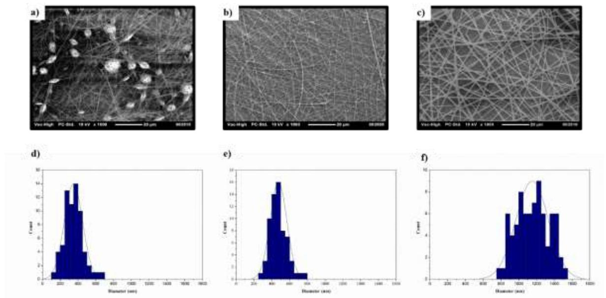
Figure 4.6. SEM images of the fabricated nanofibers at different concentrations; a) 275, b) 250, and c) 225  $\mu\text{L}$  DMF, histogram results belonging to d) 275 e) 250 f) 225  $\mu\text{L}$  DMF.
