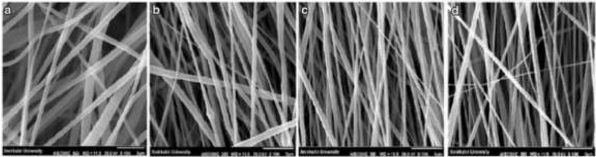
Figure 1.8. SEM images of PVDF nanofibers with the increase in distance between collector and the tip of spinneret: a) 18cm, b) 20 cm, c) 22 cm, and d) 24 cm [21].
