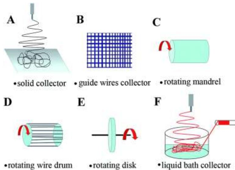
Figure 1.10. Different types of collectors used in electrospinning which are a) solid collector, b) guide wires collector, c) rotating mandrel, d) rotating wire drum, e) rotating disk f) liquid bath collector [24].
