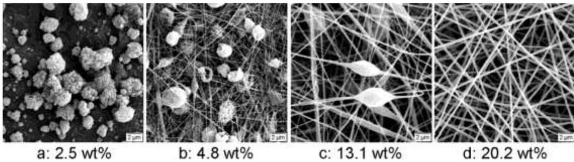
Figure 1.5. SEM images of polystyrene polymer-based nanofibers upon increasing concentration since other parameters are constant [17].
