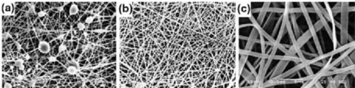
Figure 1.6. Photography of polymeric nanofibers produced from different molecular weights where a) 9000–10,000 g/mol, b) 13,000–23,000 g/mol and c) 31,000–50,000 g/mol (solution concentration: 25 wt. %) [18].
