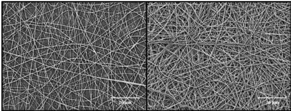
Figure 4.18. SEM images of r-GO-PFMA-PMMA-NFs after and before DOX-Mal loading, respectively.
