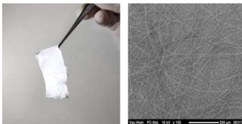
Figure 4.5. On the left; a piece of PFMA-PMMA nanofibrous mat, on the right; SEM image of the manufactured nanofiber.
