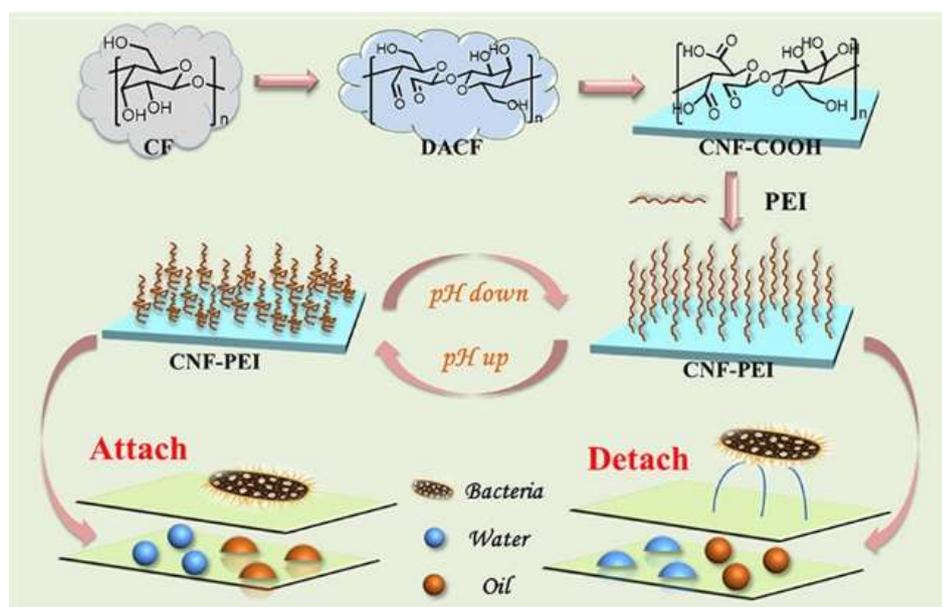
Figure 1.18. Scheme for how cellulose-based nanofibers (CNF-PEI) upon a change in a narrow pH range for antibacterial response [57].
