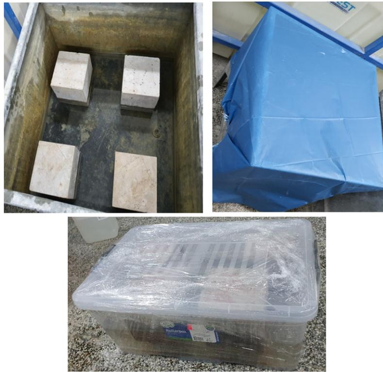
Figure 3.5. a) Re-curing container, b) Sealed re-curing container, c) HCl re-curing container.
