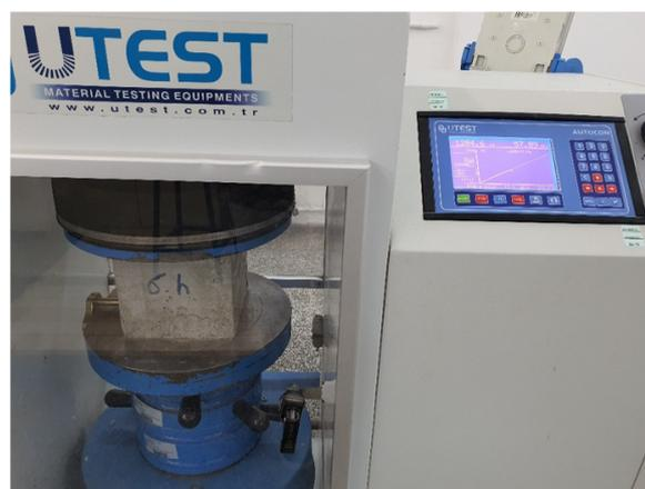
Figure 3.8. UTEST Automatic Compression Testing Machine.
