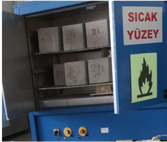
Figure 3.1. Drying Oven.
