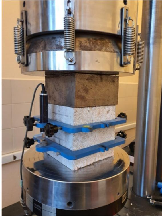
Figure 3.9. Compressometer frame.
