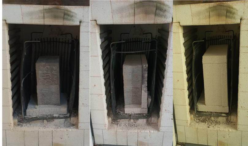
Figure 3.3. Position of the specimens and heat insulations inside the furnace.
