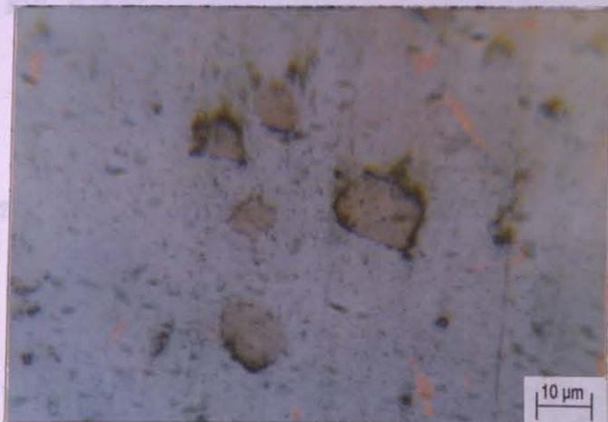
Fig. 4.13. Microstructure at the same region of the Zn-Bi specimen squeeze cast under 85 MPa (x800, oil lens).
