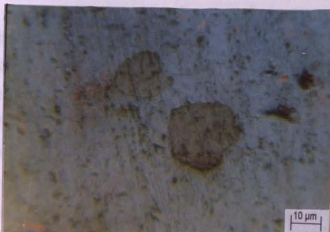
Fig. 4.11. Microstructure at 1.5 cm from bottom end of the specimen squeeze cast at 85 MPa (x800, oil lens).
