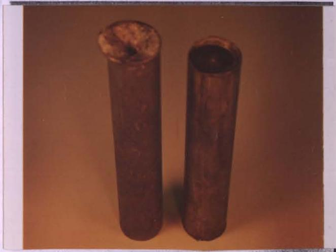
Fig. 3.4. Castings produced by gravity casting (at left hand side) and, by squeeze casting (at right hand side) methods.
