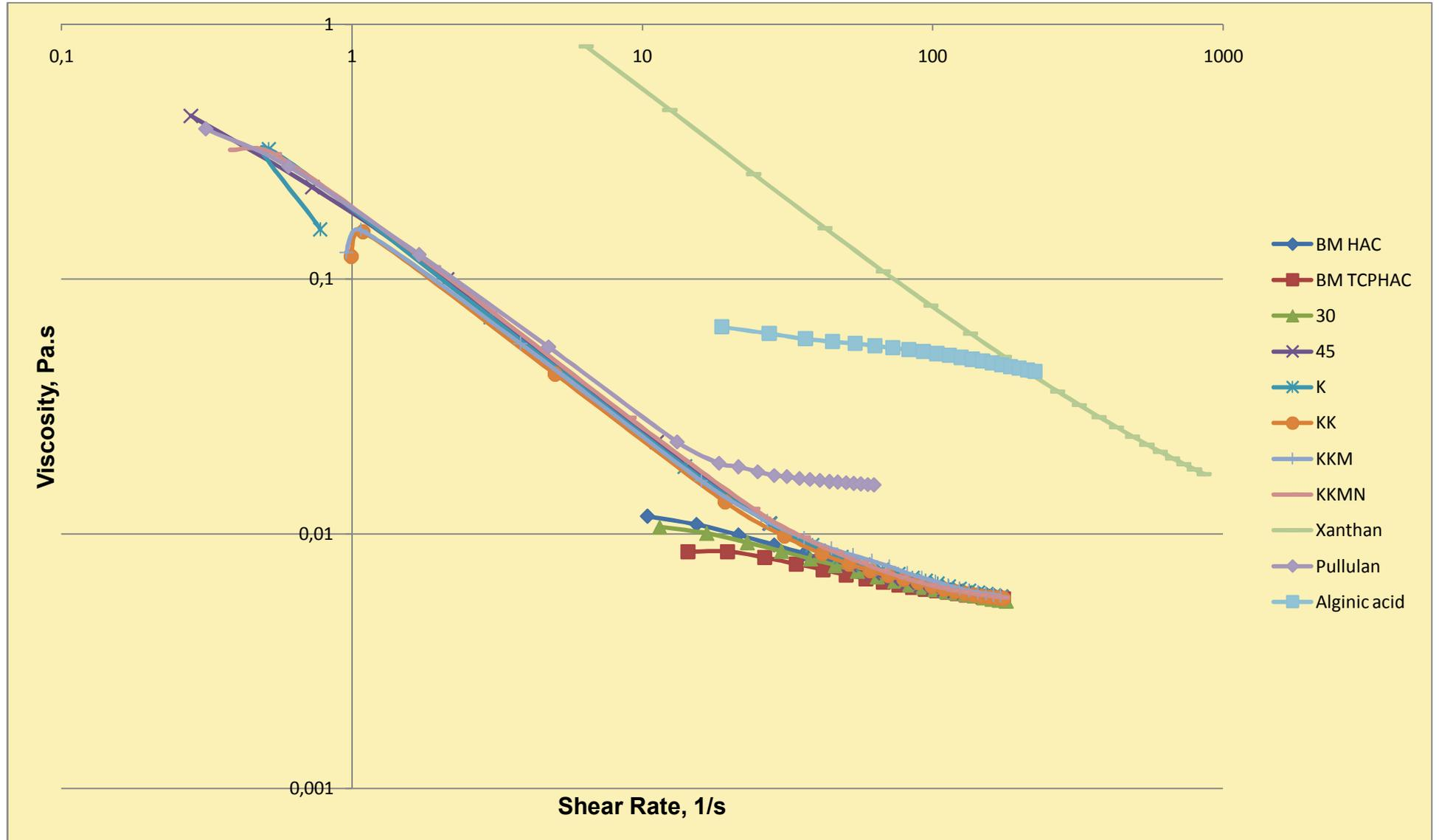
Figure 4.12. Viscosity versus shear rate curves of the %1 (w/v) exopolysaccharide solutions at 20 °C
