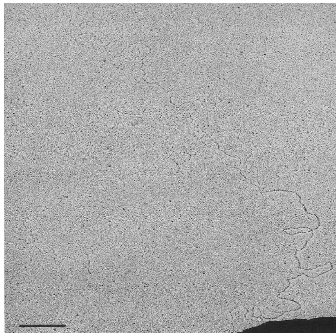
Figure 2.5. Electron micrograph of a xanthan preparation showing the apparently double stranded chain separating into two thinner strands (Sutherland, 1990).
