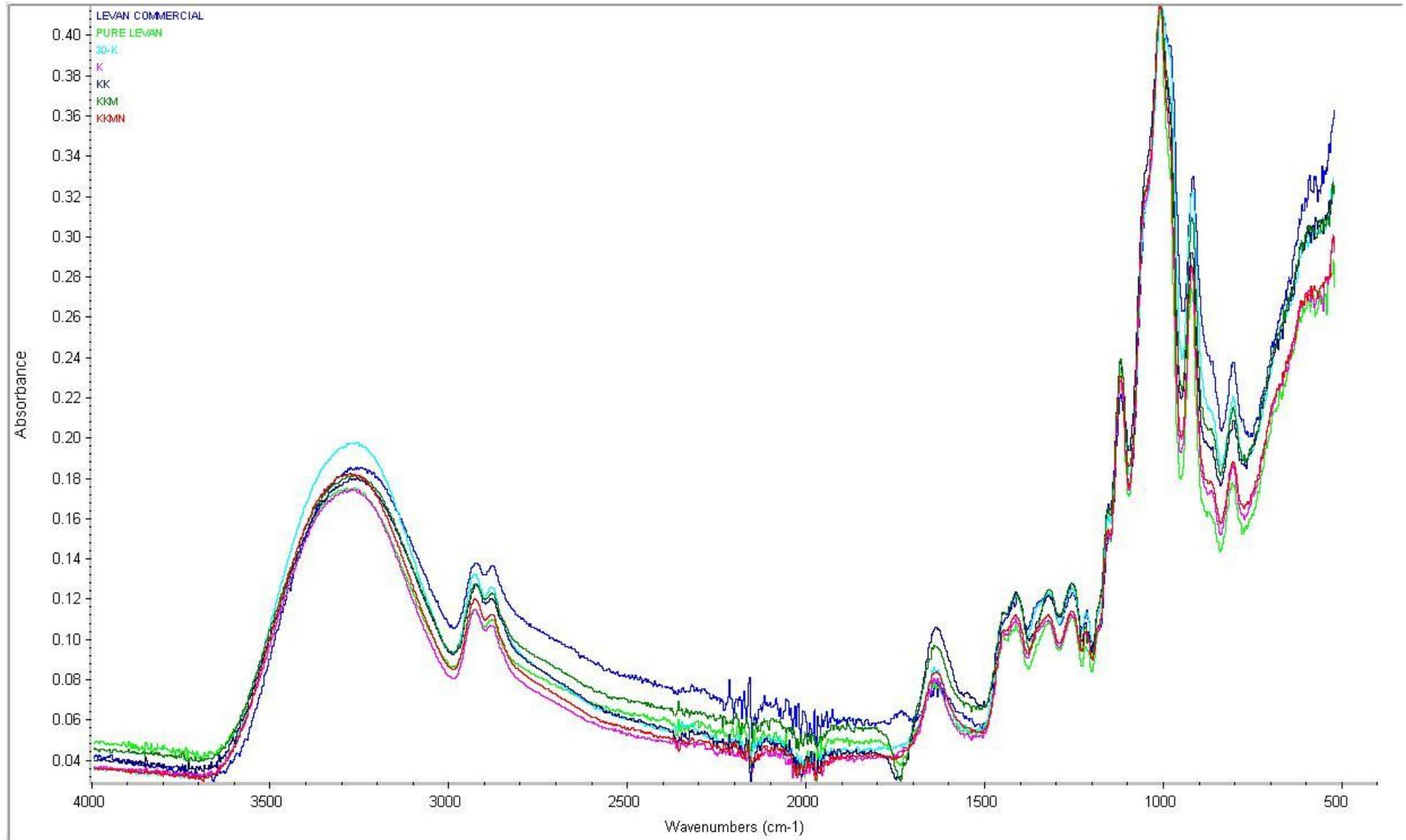
Figure 4.10. FT-IR spectra of commercial levan, pure levan, and EPSs produced from pretreated BM with salt drop out
