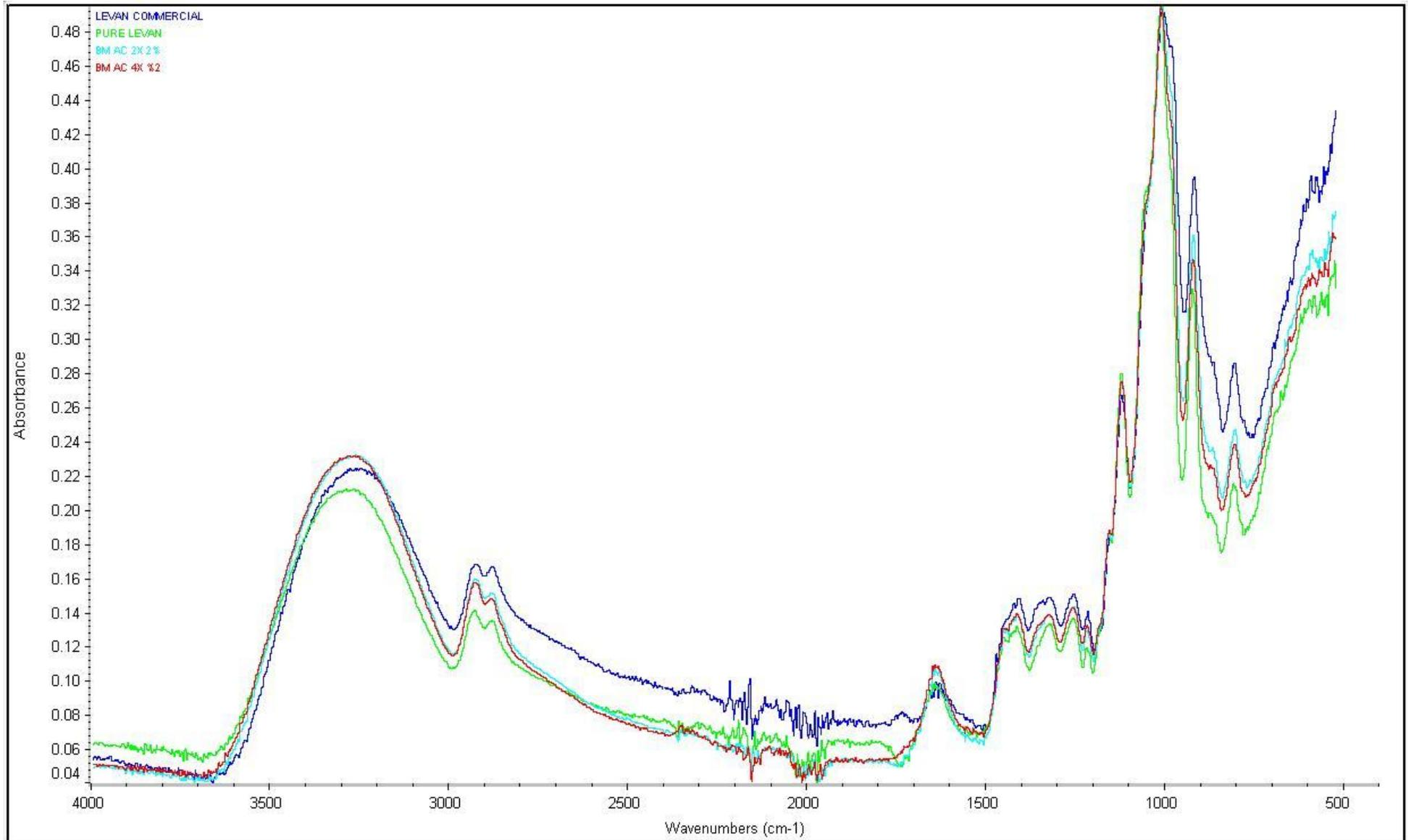
Figure 4.11. FT-IR spectra of commercial levan, pure levan, and EPSs produced from BM subjected to different runs of AC pretreatment
