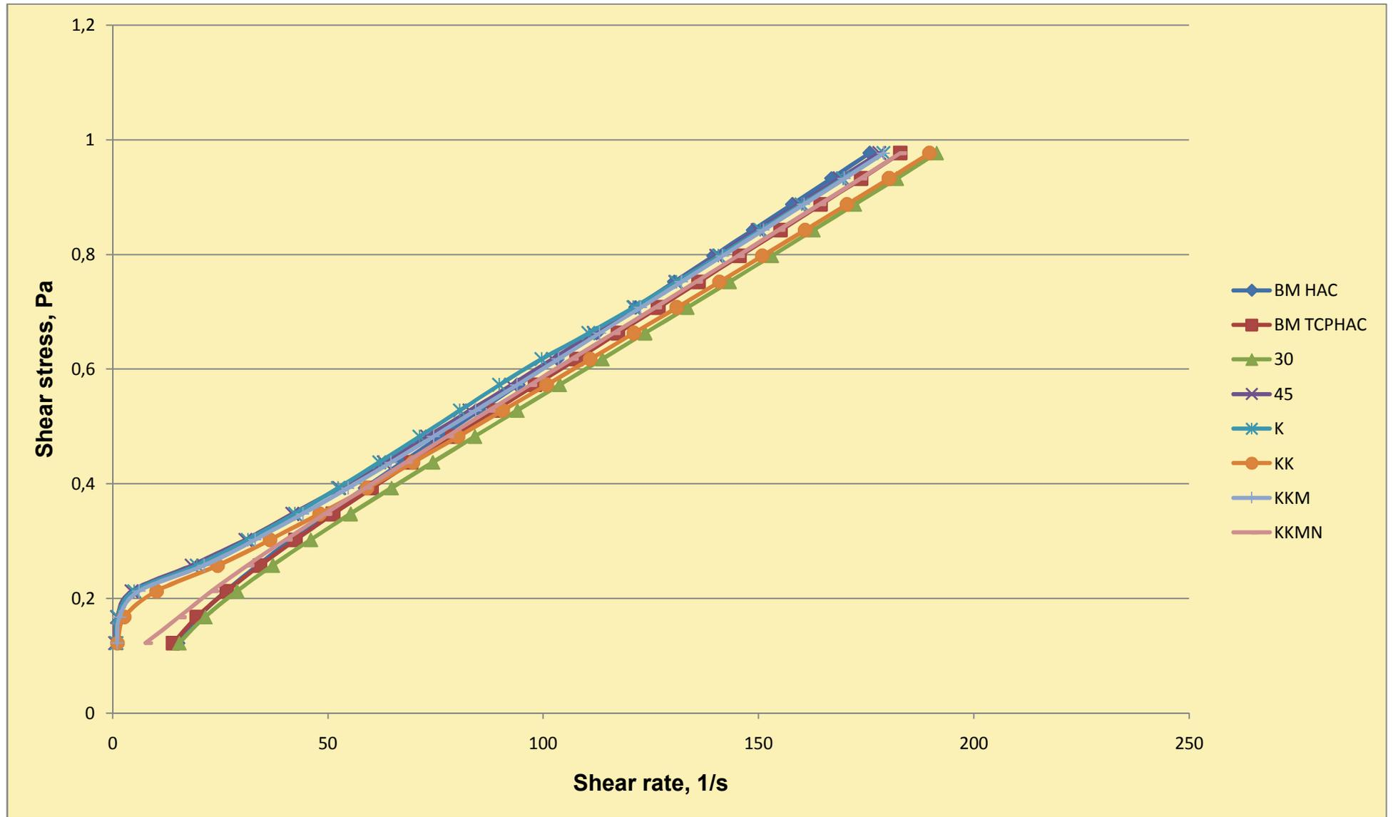
Figure 4.19. Rheograms of the %1 (w/v) exopolysaccharide solutions at 37 °C and in %10 NaCl solution
