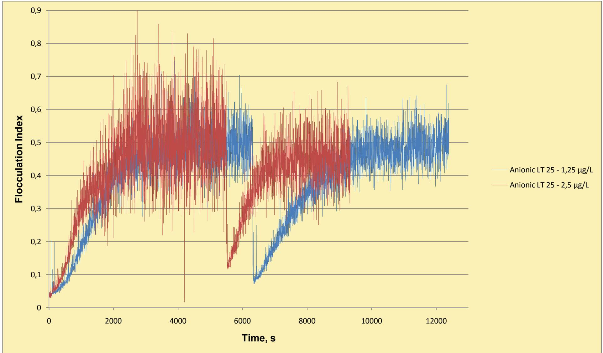
Figure 4.26. Relative floc sizes of the flocculation experiments done with different concentrations of anionic polyelectrolyte Magnafloc LT 25 in real sea water
