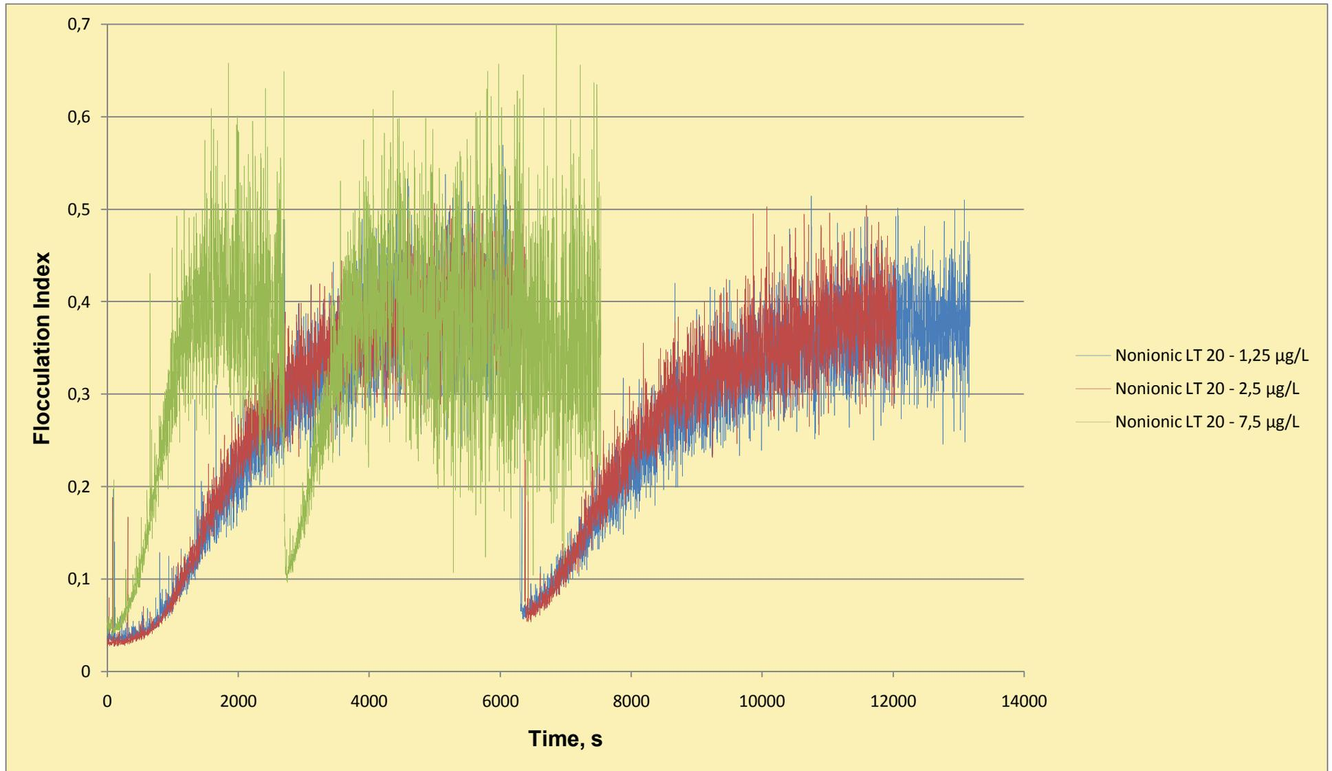
Figure 4.28. Relative floc sizes of the flocculation experiments done with different concentrations of nonionic polyelectrolyte Magnafloc LT 20 in real sea water
