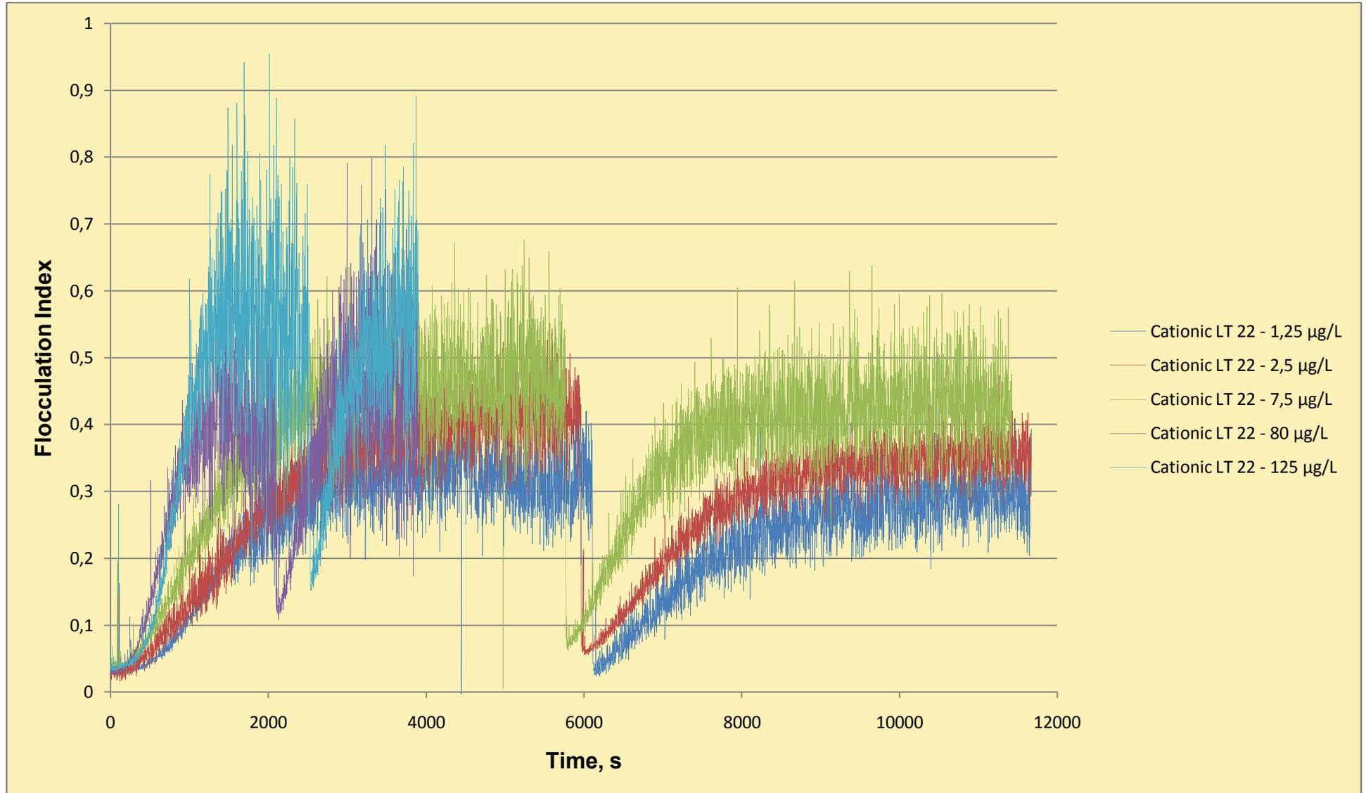
Figure 4.24. Relative floc sizes of the flocculation experiments done with different concentrations of cationic polyelectrolyte Magnafloc LT 22 in real sea water
