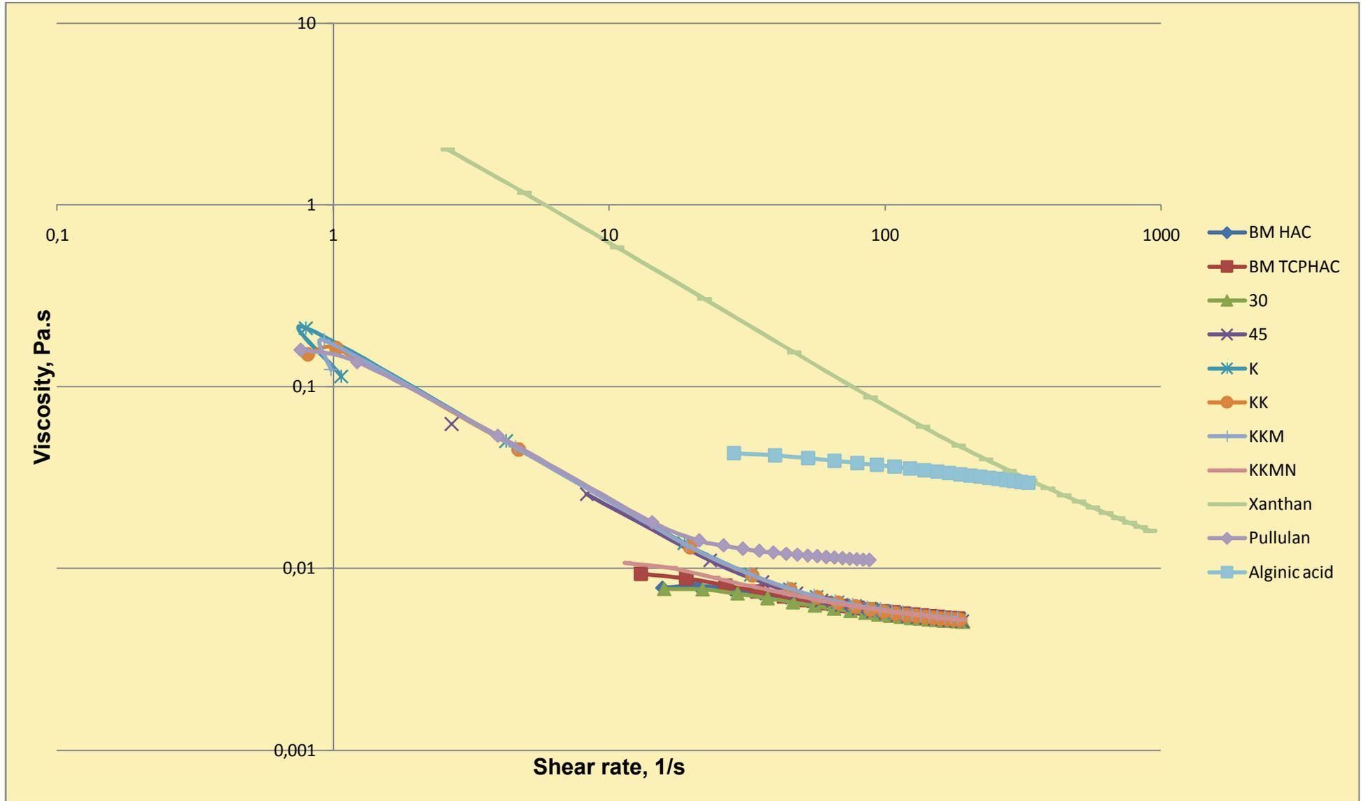
Figure 4.13. Viscosity versus shear rate curves of the %1 (w/v) exopolysaccharide solutions at 37 °C
