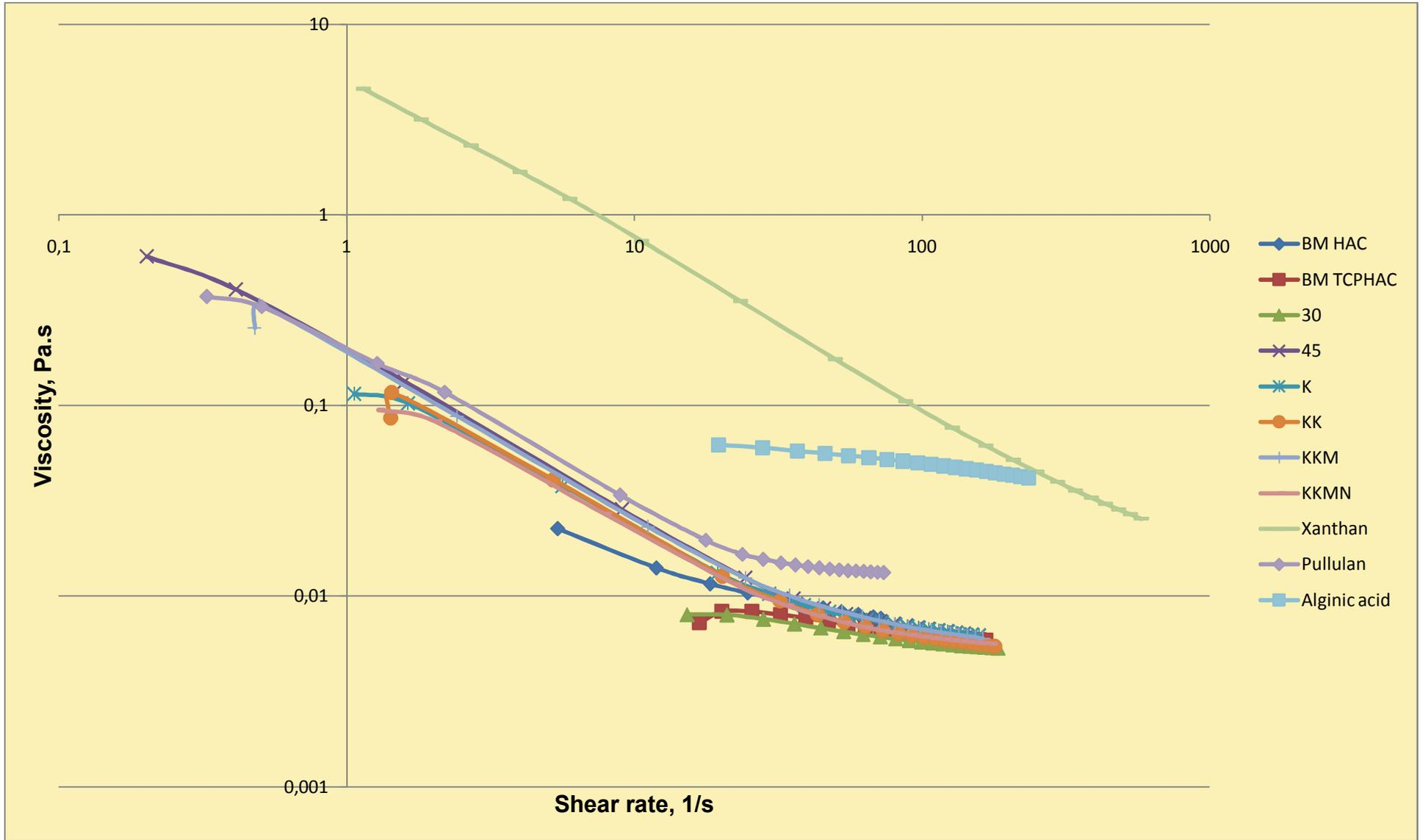
Figure 4.14. Viscosity versus shear rate curves of the %1 (w/v) exopolysaccharide solutions at 20 °C and in %10 NaCl solution
