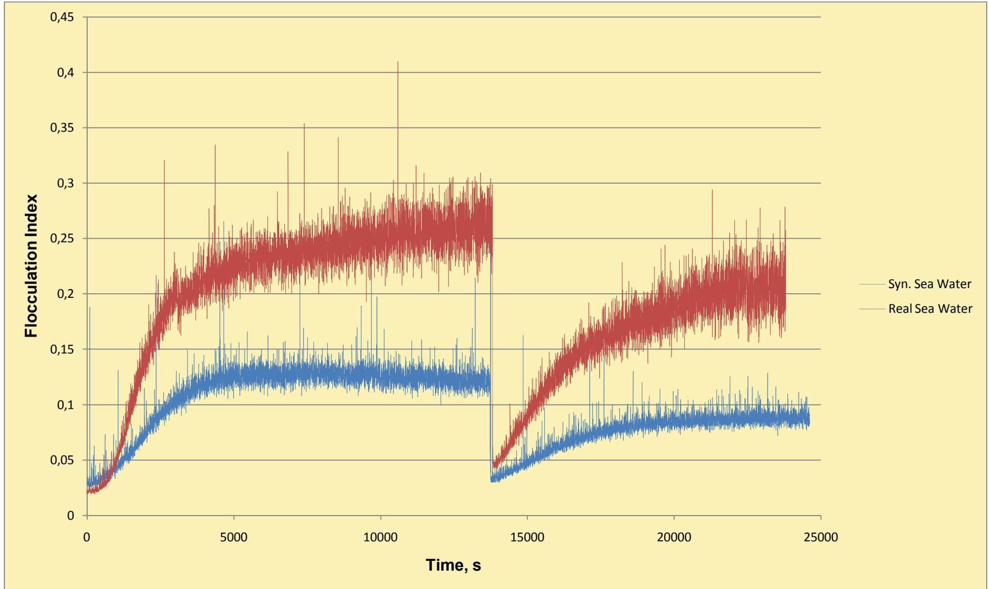
Figure 4.21. Relative floc sizes of the flocculation experiments done with SM HAC (10mg/L) in synthetic sea water and real sea water
