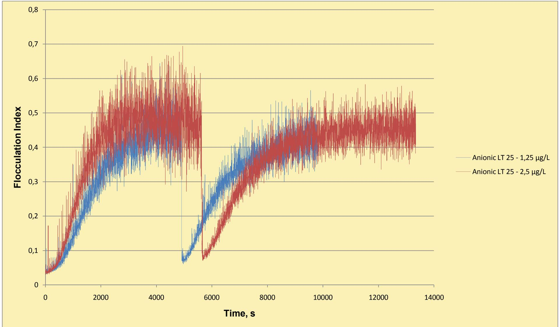
Figure 4.25. Relative floc sizes of the flocculation experiments done with different concentrations of anionic polyelectrolyte Magnafloc LT 25 in synthetic sea water
