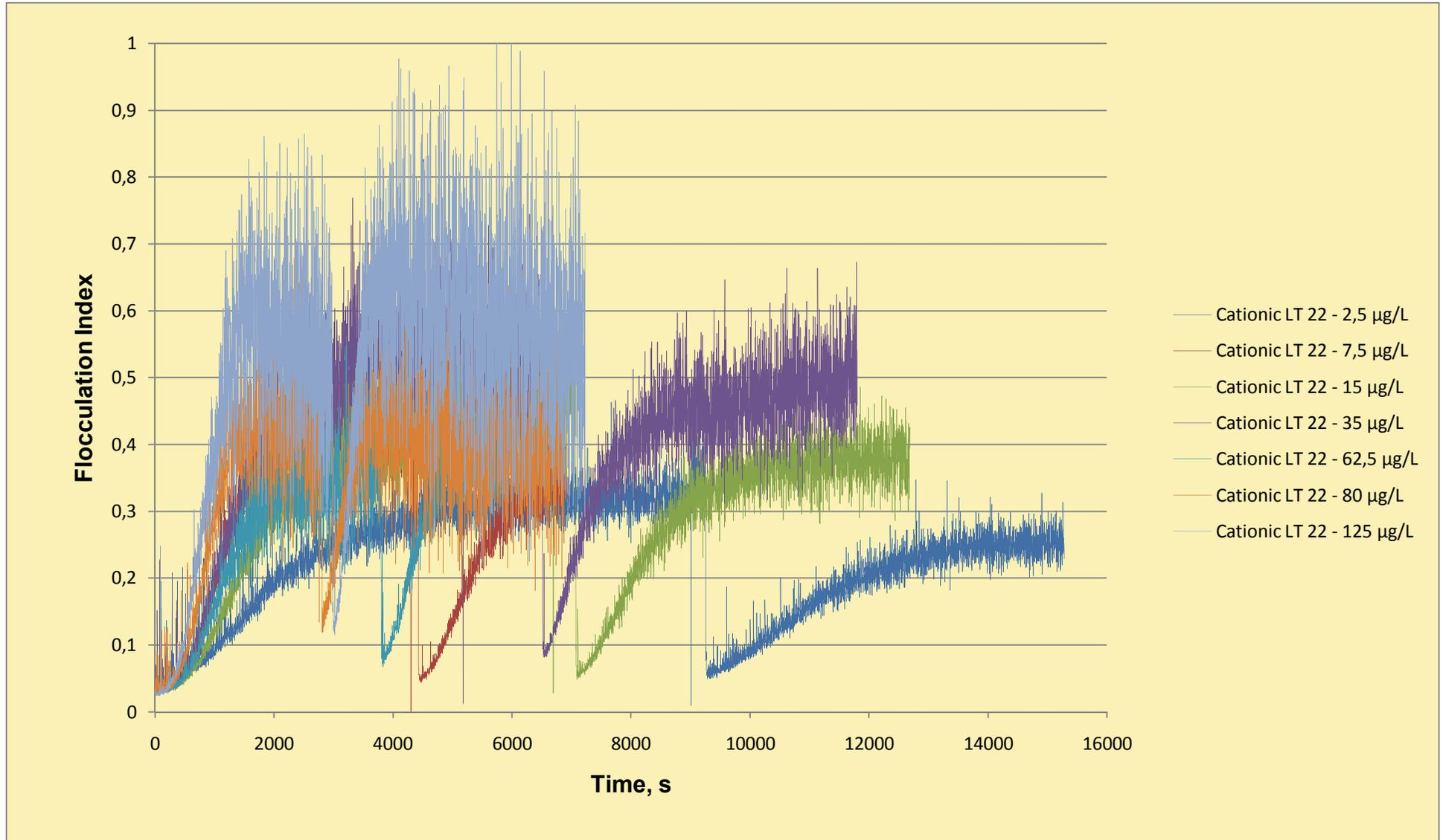
Figure 4.23. Relative floc sizes of the flocculation experiments done with different concentrations of cationic polyelectrolyte Magnafloc LT 22 in synthetic sea water
