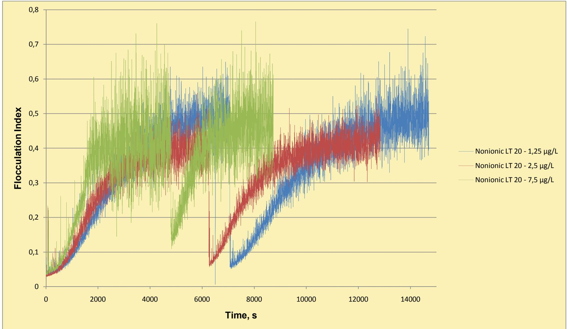
Figure 4.27. Relative floc sizes of the flocculation experiments done with different concentrations of nonionic polyelectrolyte Magnafloc LT 20 in synthetic sea water
