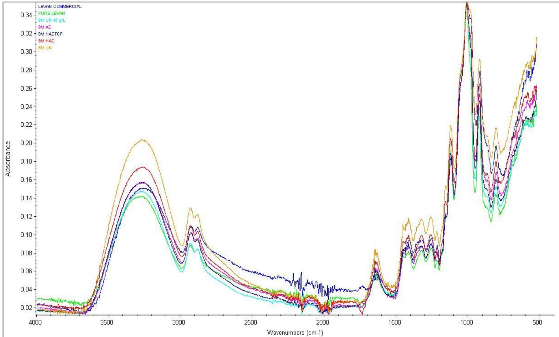
Figure 4.9. FT-IR spectra of commercial levan, pure levan, and EPSs produced from pretreated BM
