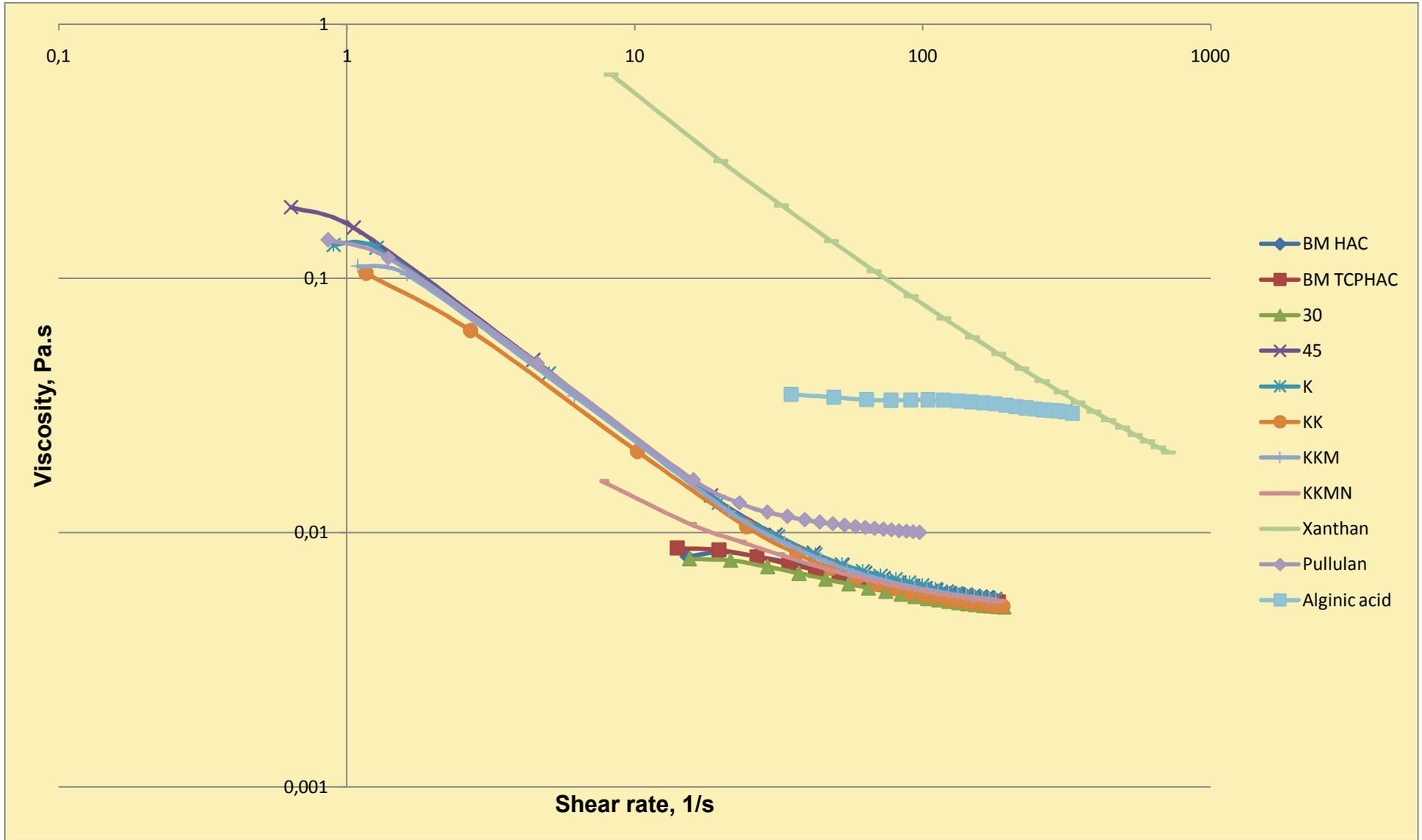
Figure 4.15. Viscosity versus shear rate curves of the %1 (w/v) exopolysaccharide solutions at 37 °C and in %10 NaCl solution
