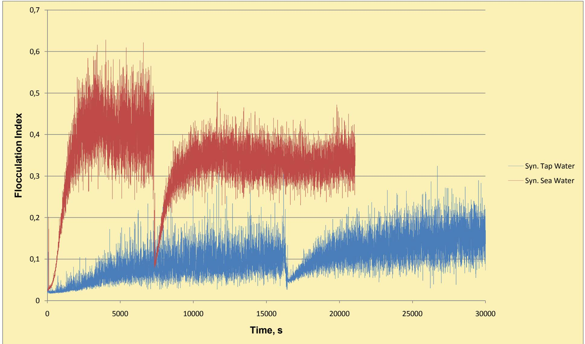
Figure 4.20. Relative floc sizes of the flocculation experiments done with SM HAC (100mg/L) in synthetic tap and sea water
