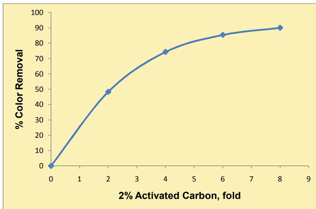
Figure 4.7. The effect of activated carbon treatment on the color removal of the beet molasses solution
