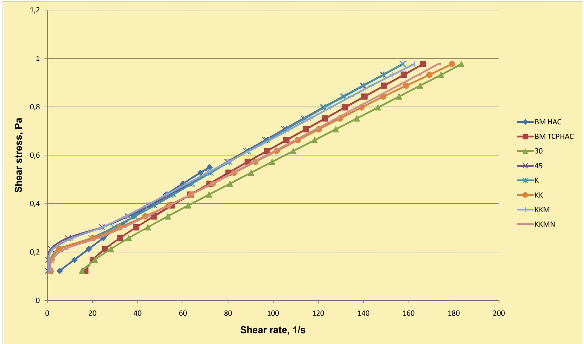
Figure 4.18. Rheograms of the 1% (w/v) exopolysaccharide solutions at 20 °C and in 10% NaCl solution
