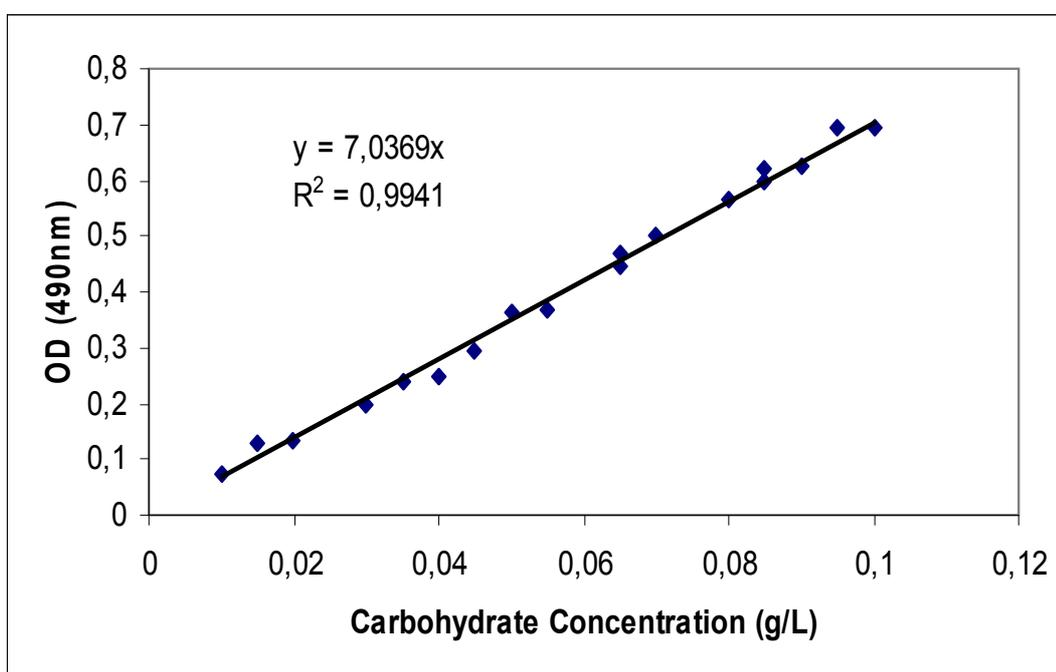
Figure A.1. Total carbohydrate concentration calibration chart
