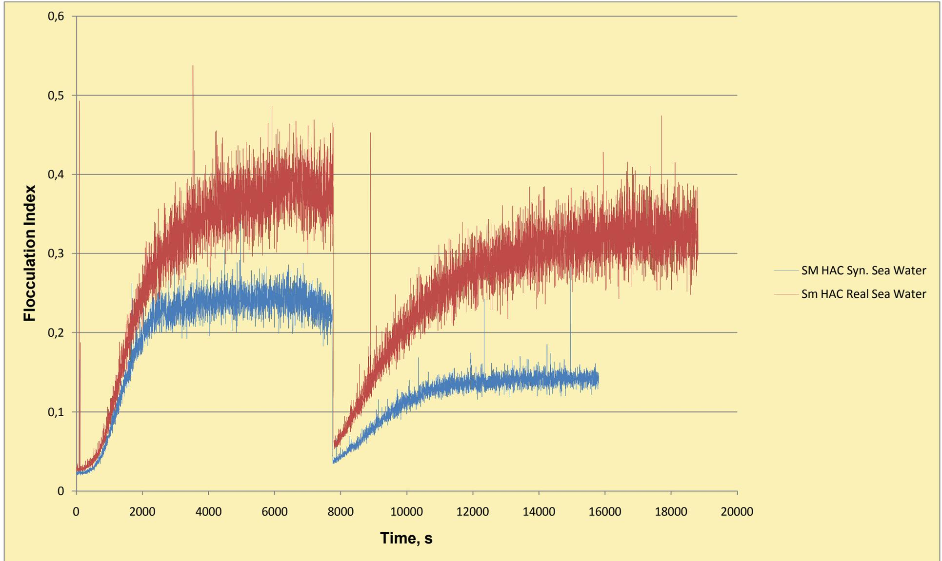
Figure 4.22. Relative floc sizes of the flocculation experiments done with SM HAC (20mg/L) in synthetic sea water and real sea water
