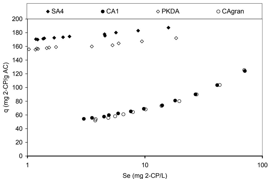
Figure 4.21. 2-Chlorophenol desorption isotherms for activated carbon types SA4, CA1, PKDA and CAgran.
