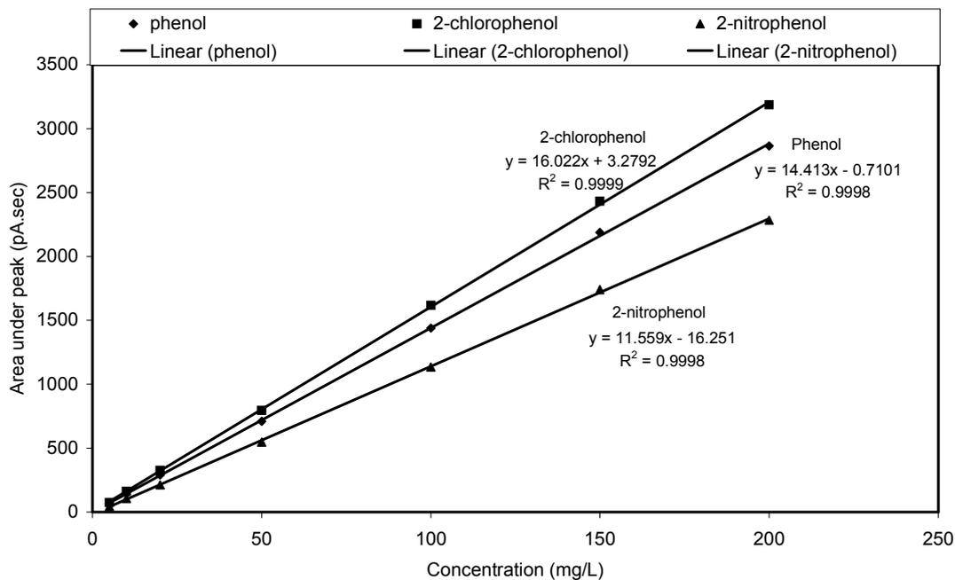
Figure A.5. Calibration curves for gas chromatographic analysis.
