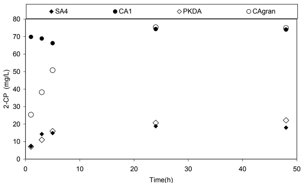
Figure 4.20. 2-Chlorophenol profiles during desorption at a dose of 2 g/L of activated carbons SA4, CA1, PKDA and CAgran.
