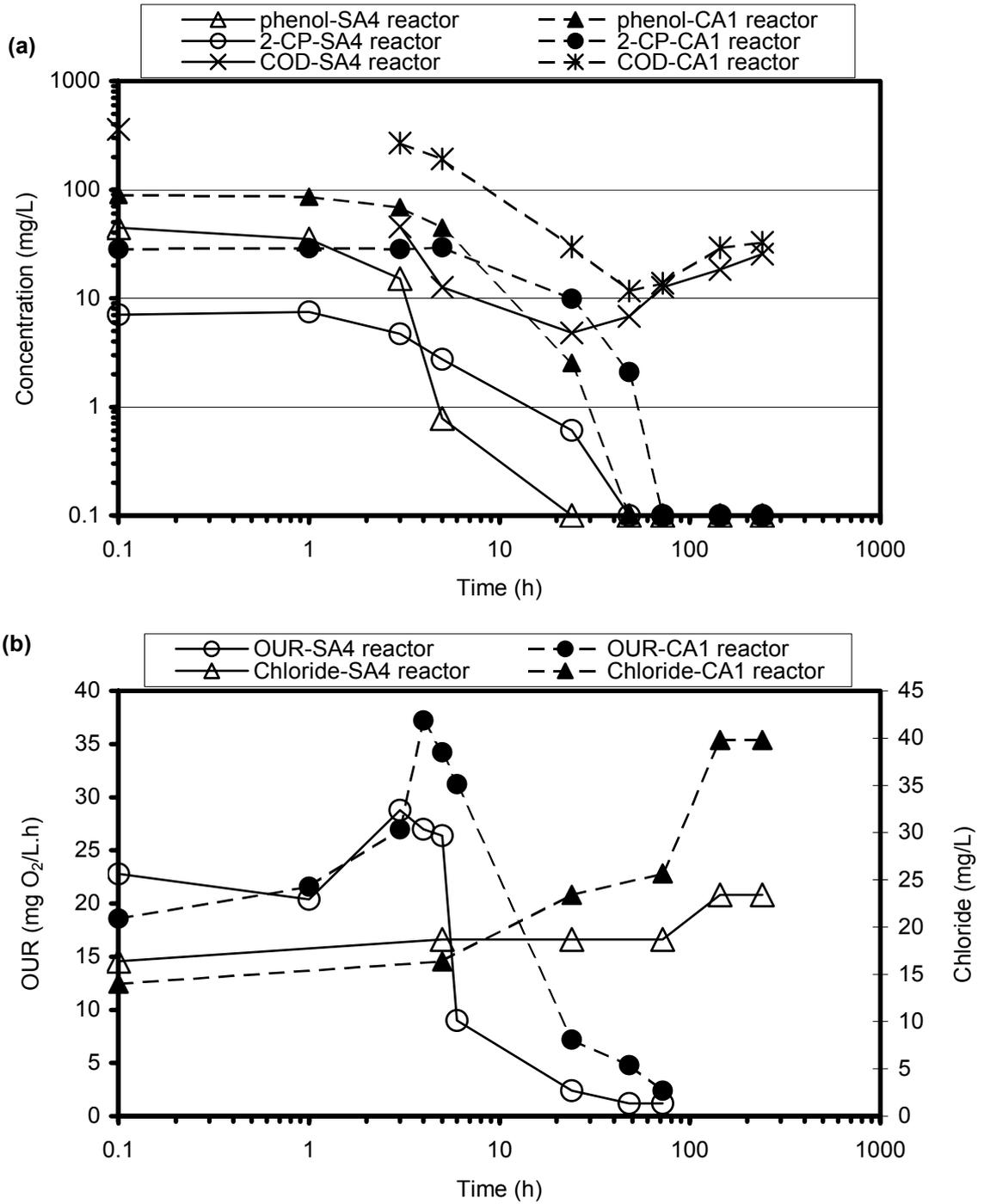
Figure 4.34. a) Phenol, 2-CP and COD profiles b) OUR and chloride profiles in bioregeneration reactors with SA4 (powdered, thermally activated) and CA1 (powdered, chemically activated) in RUN 14.
