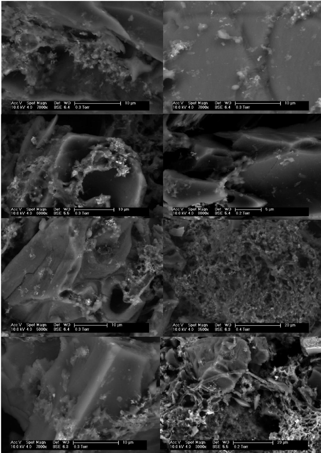
Figure B.5. Environmental scanning electron micrographs of microorganisms on CA1 carbon at t=3 days in RUN 14.
