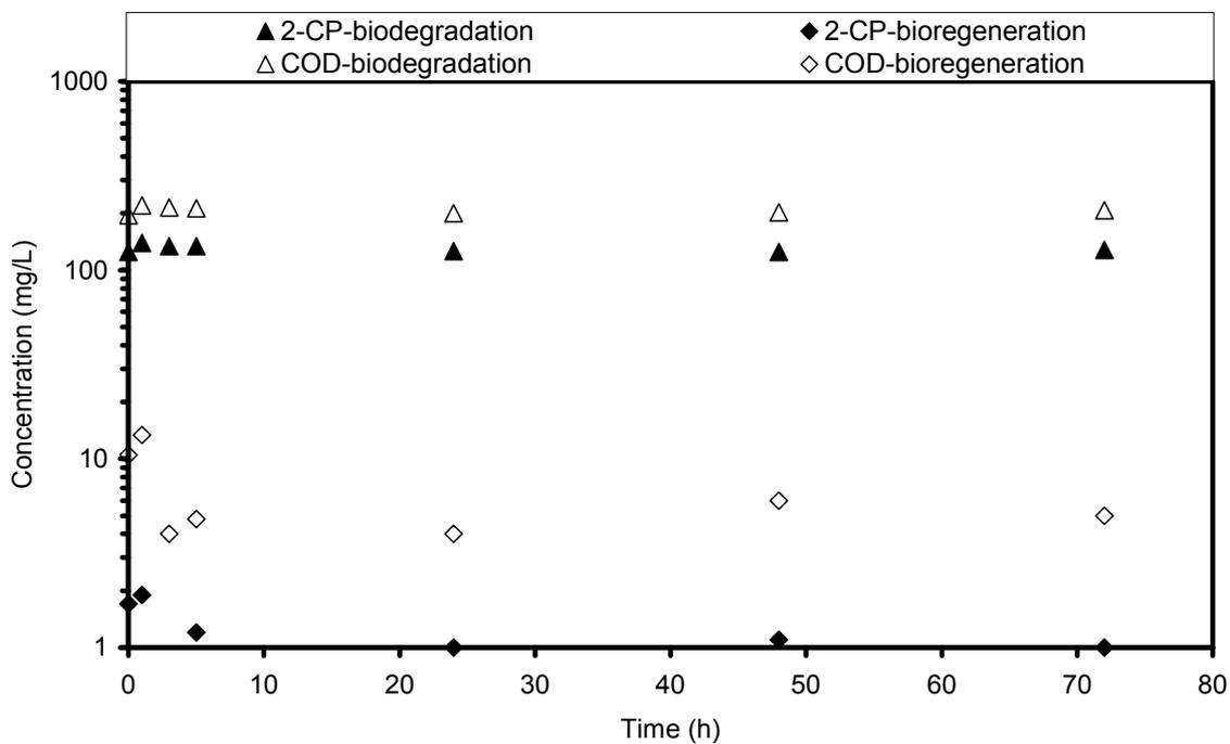
Figure 4.24. 2-chlorophenol and COD profiles in biodegradation and bioregeneration reactors in RUN 9 with 2-chlorophenol when acclimated biomass and SA4 carbon were used.
