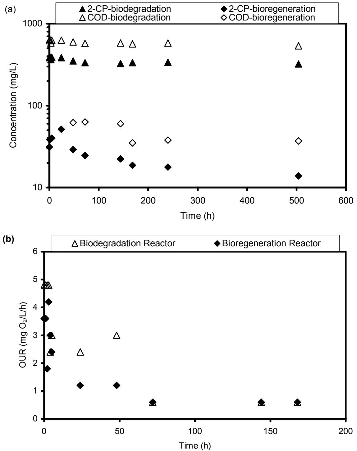
Figure 4.23. a) 2-chlorophenol and COD profiles and b) OUR profiles in biodegradation and bioregeneration reactors in RUN 8 with 2-chlorophenol when non-acclimated biomass and SA4 carbon were used.
