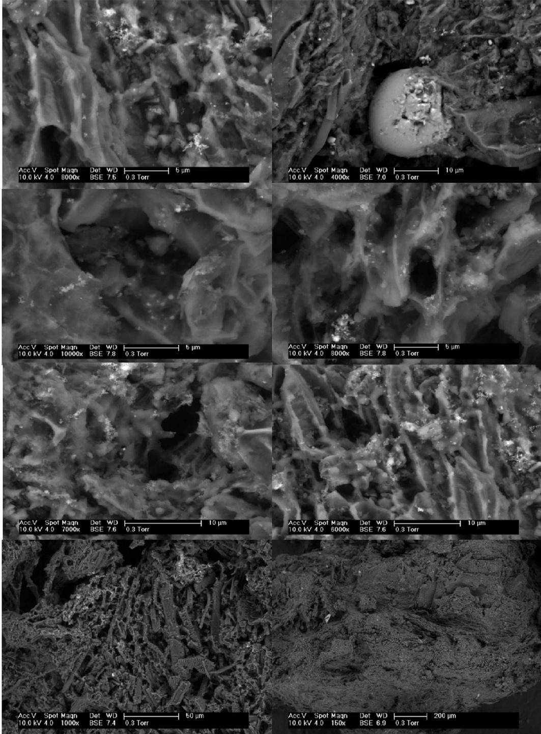
Figure B.6. Environmental scanning electron micrographs of microorganisms on PKDA carbon at t=3 days in RUN 15.
