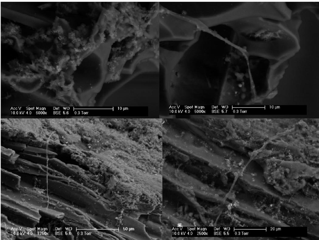
Figure B.8. Environmental scanning electron micrographs of microorganisms on CAgan at t=8 days in RUN 15.
