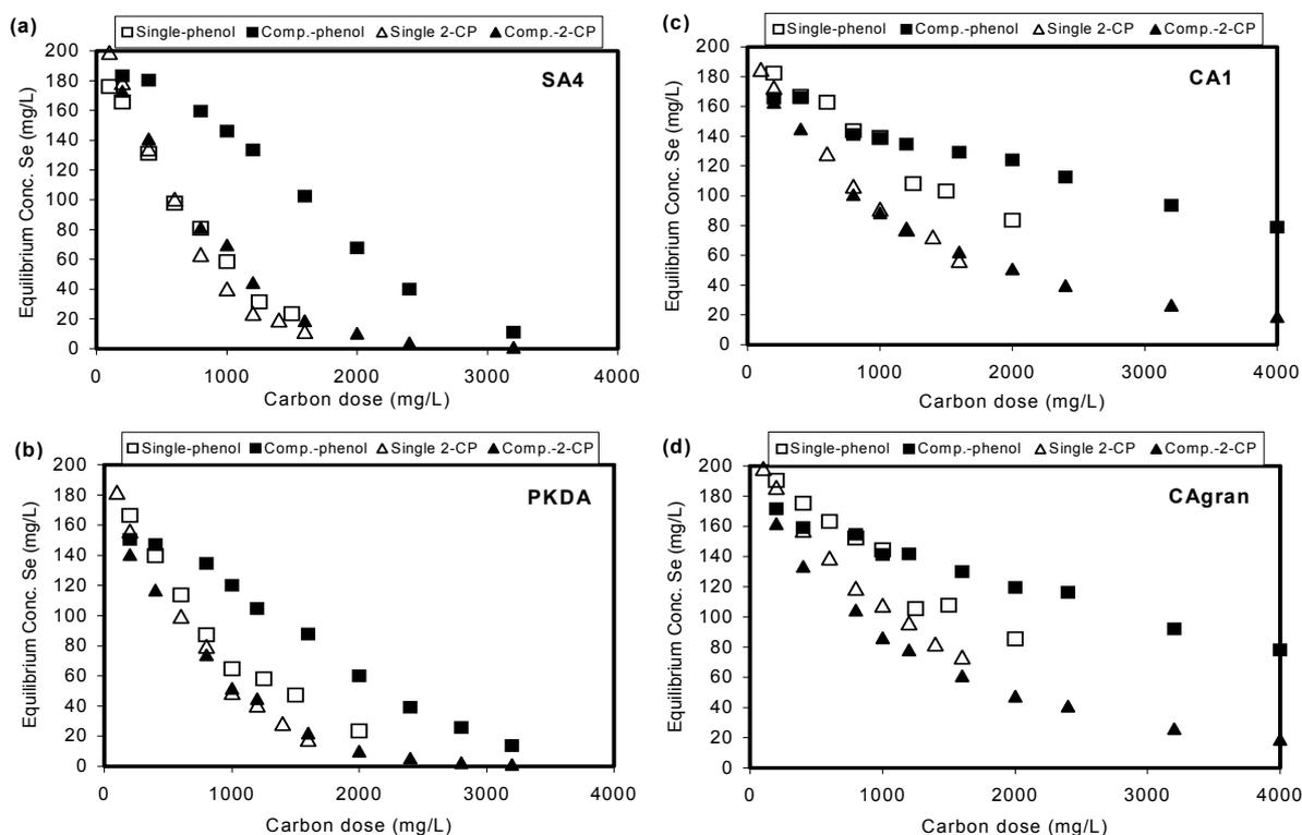
Figure 4.26. Effect of activated carbon dose on equilibrium phenol and 2-CP concentrations in competitive bi-solute and single-solute adsorption studies with initial concentrations of 200 mg/L for a) SA4, b) PKDA, c) CA1, d) CAgan. (open data points refer to single-solute adsorption, closed data points refer to bi-solute adsorption).
