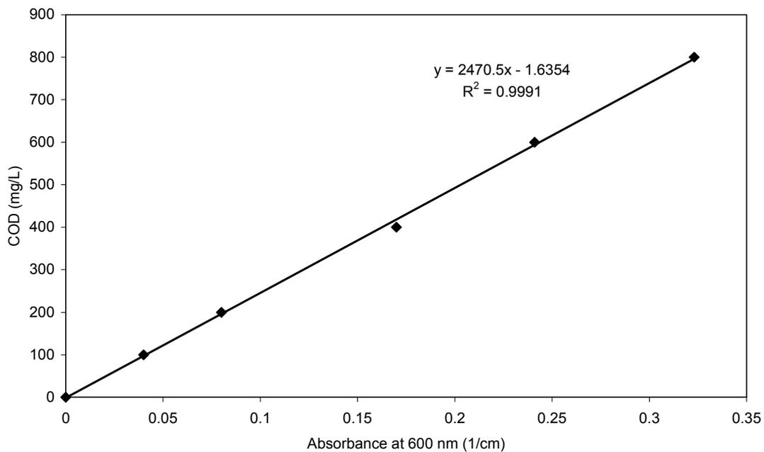
Figure A.1. Calibration curve for high range chemical oxygen demand (COD) analysis.
