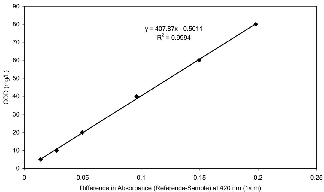
Figure A.2. Calibration curve for low range chemical oxygen demand (COD) analysis.
