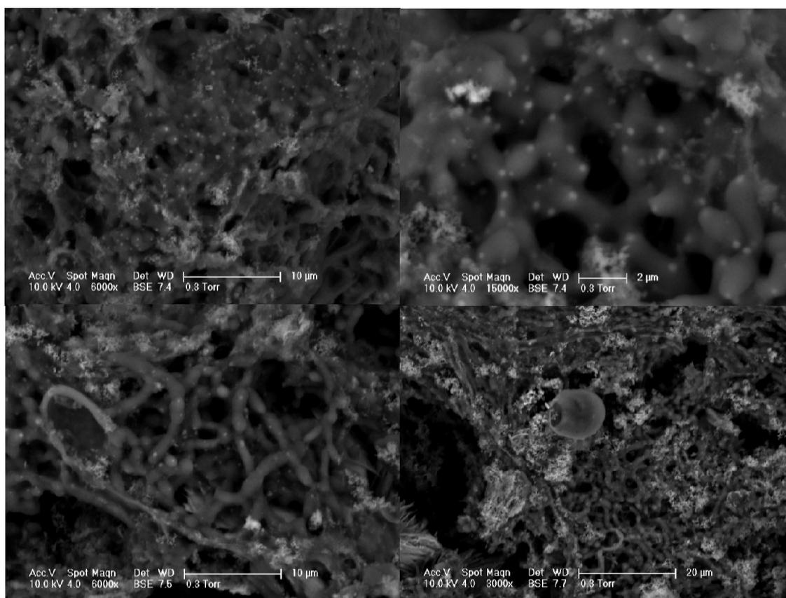
Figure 3.4. Environmental scanning electron microscopy of microorganisms in activated sludge acclimated with phenol and 2-CP.
