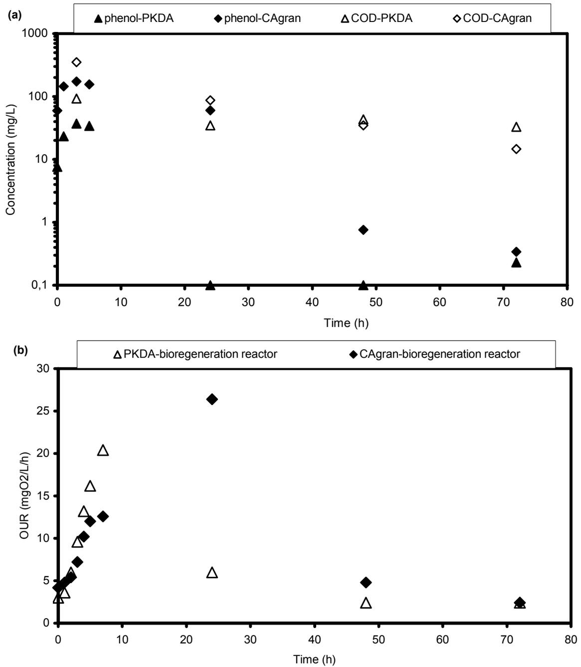
Figure 4.13. a) Phenol and COD profiles b) OUR profiles in bioregeneration reactors with 2000 mg/L PKDA (granular, thermally activated) and CAgran (granular, chemically activated) in RUN 7.
