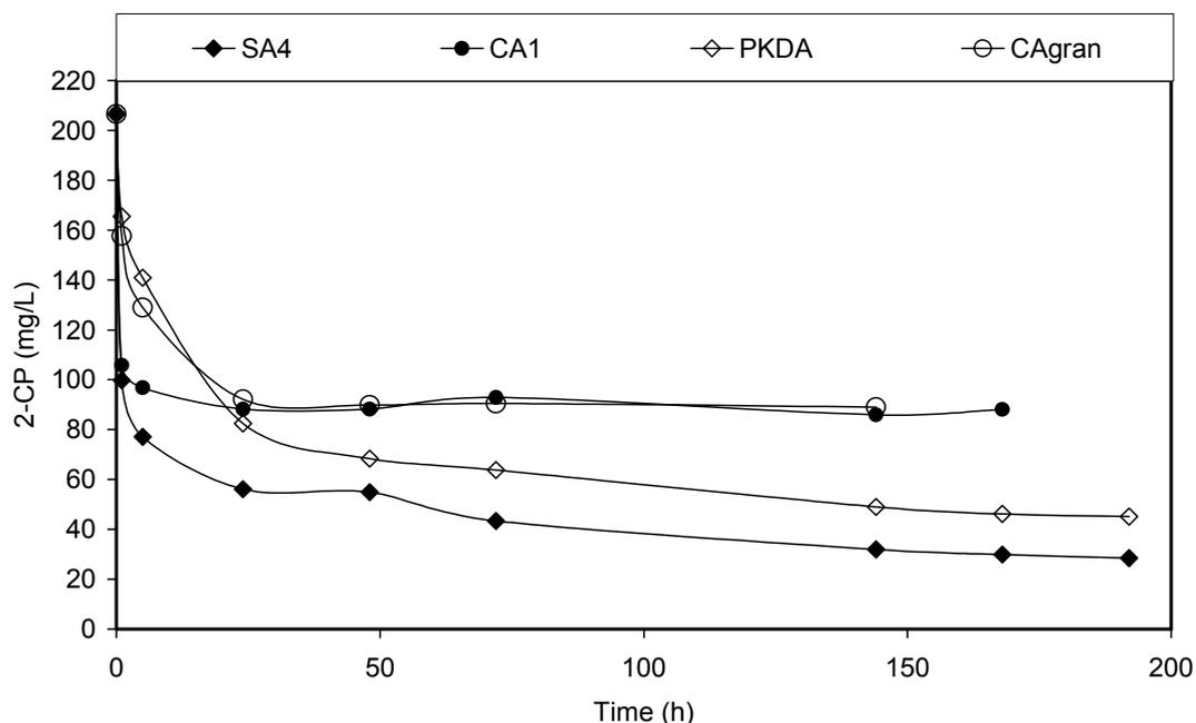
Figure 4.17. 2-Chlorophenol profiles during adsorption at an initial 2-CP concentration of 200 mg/L and 1 g/L of activated carbons SA4, CA1, PKDA and CAgran.
