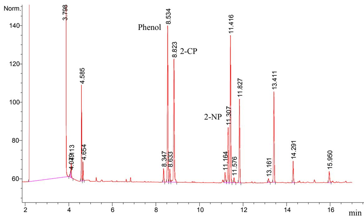
Figure A.7. Gas chromatogram of mixed phenols standard (each 20 mg/L in methanol).
