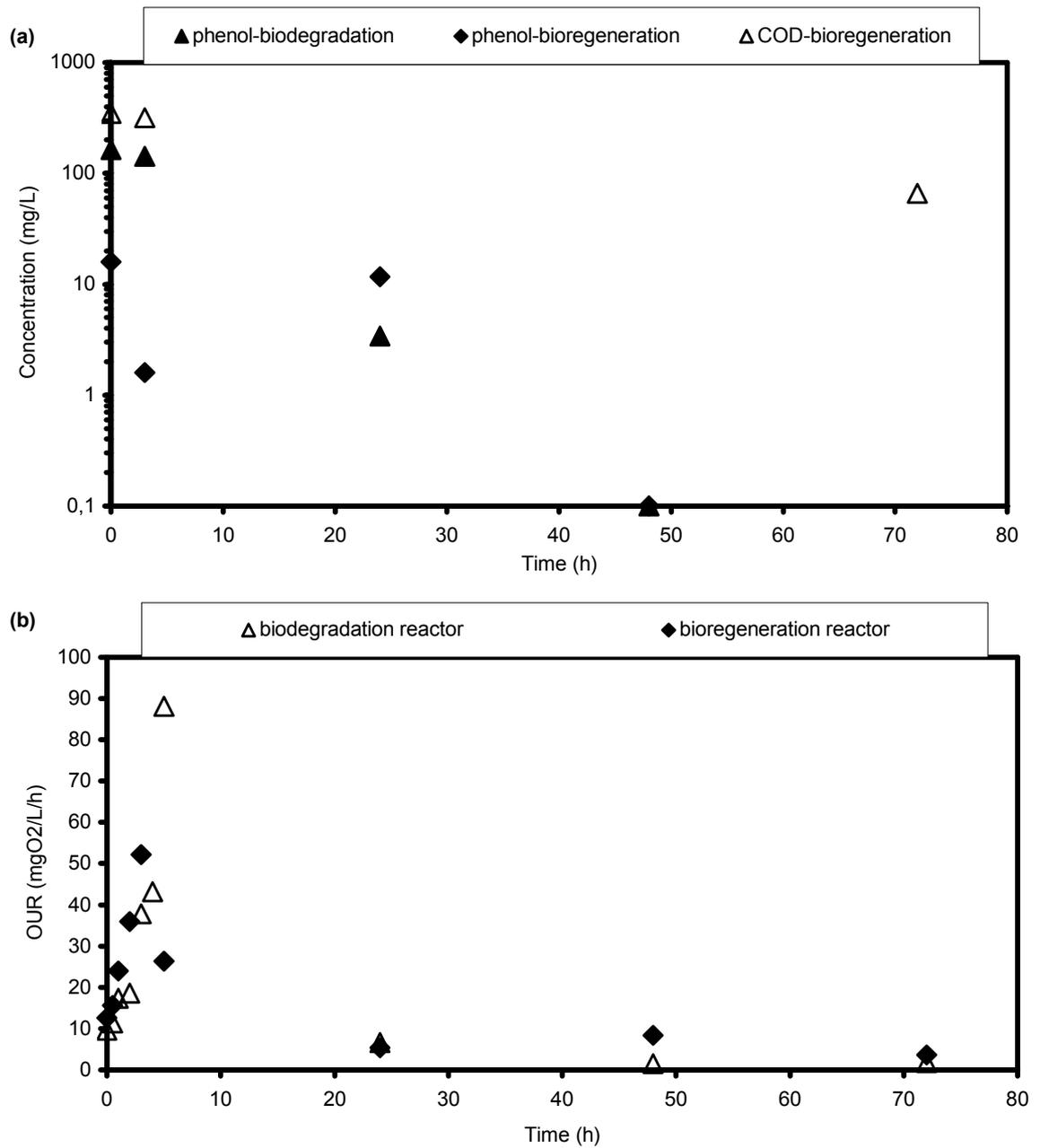
Figure 4.7. a) Phenol and COD profiles b) OUR profiles in biodegradation reactor and bioregeneration reactor with 1000 mg/L SA4 (powdered, thermally activated) in RUN 1.
