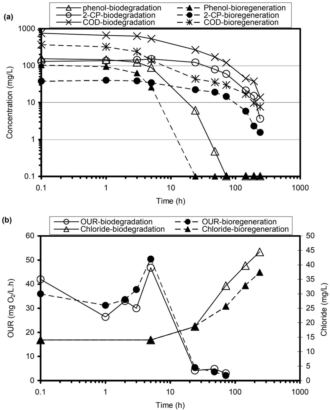
Figure 4.31. a) Phenol, 2-CP and COD profiles b) OUR and chloride profiles in biodegradation reactor and bioregeneration reactor with 2000 mg/L CA1 (powdered, chemically activated) in RUN 11.
