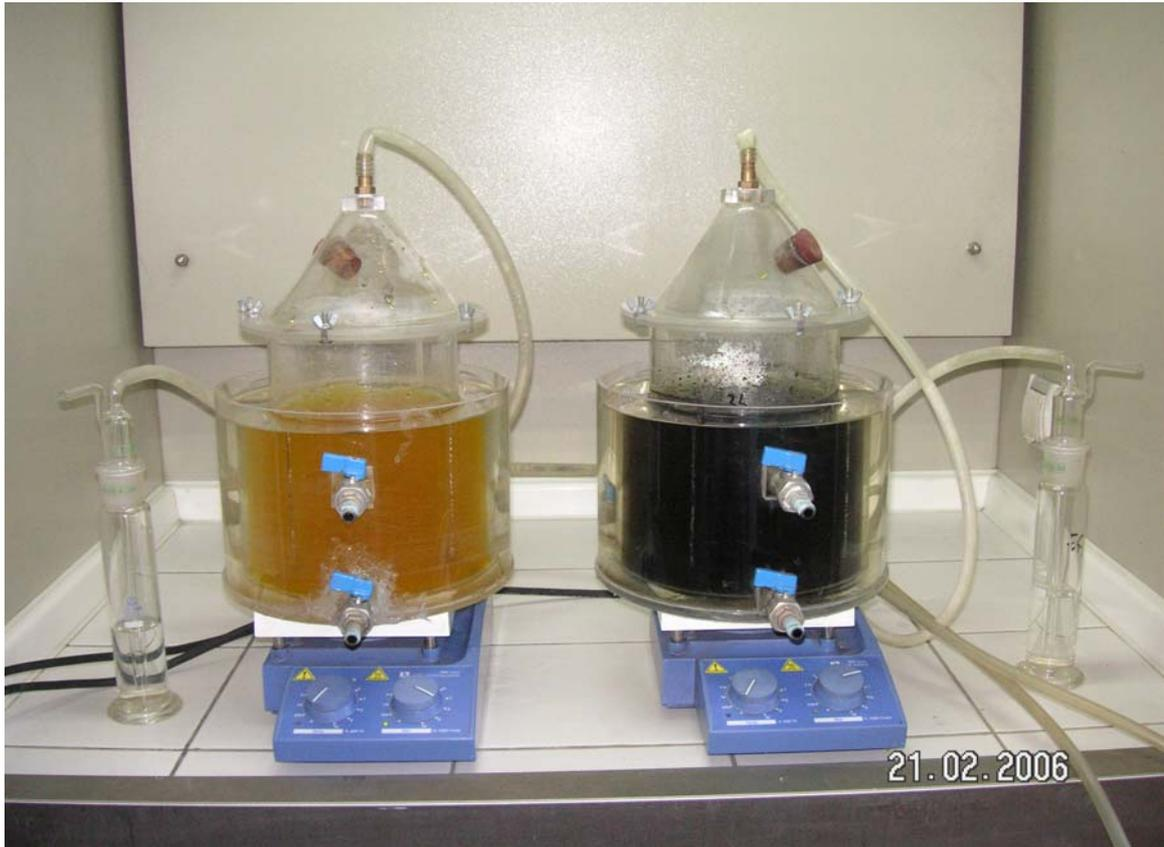
Figure 3.2. Simultaneously operated batch activated sludge reactors; left: biodegradation reactor without activated carbon and right: bioregeneration reactor with loaded activated carbon.
