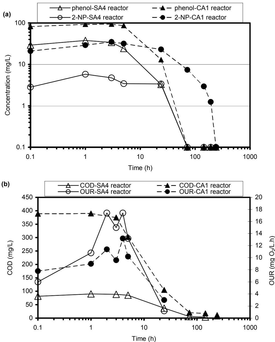
Figure 4.46. a) Phenol and 2-NP profiles b) COD and OUR profiles in bioregeneration reactors with SA4 (powdered, thermally activated) and CA1 (powdered, chemically activated) in RUN 19.
