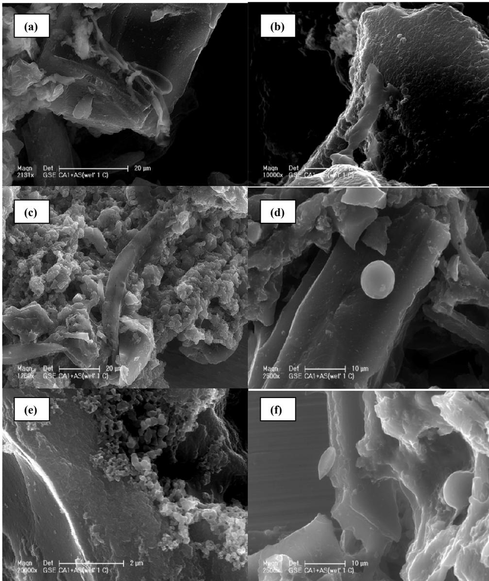
Figure 4.15. Scanning Electron Micrographs of microorganisms on activated carbon a) filamentous bacteria b) spiral-shaped bacteria c) a protozoan d) a spherical protozoan attached to the carbon surface e) group of cocci-shaped bacteria clustered in the carbon cavities f) a stalked protozoan attached to carbon cavities.
