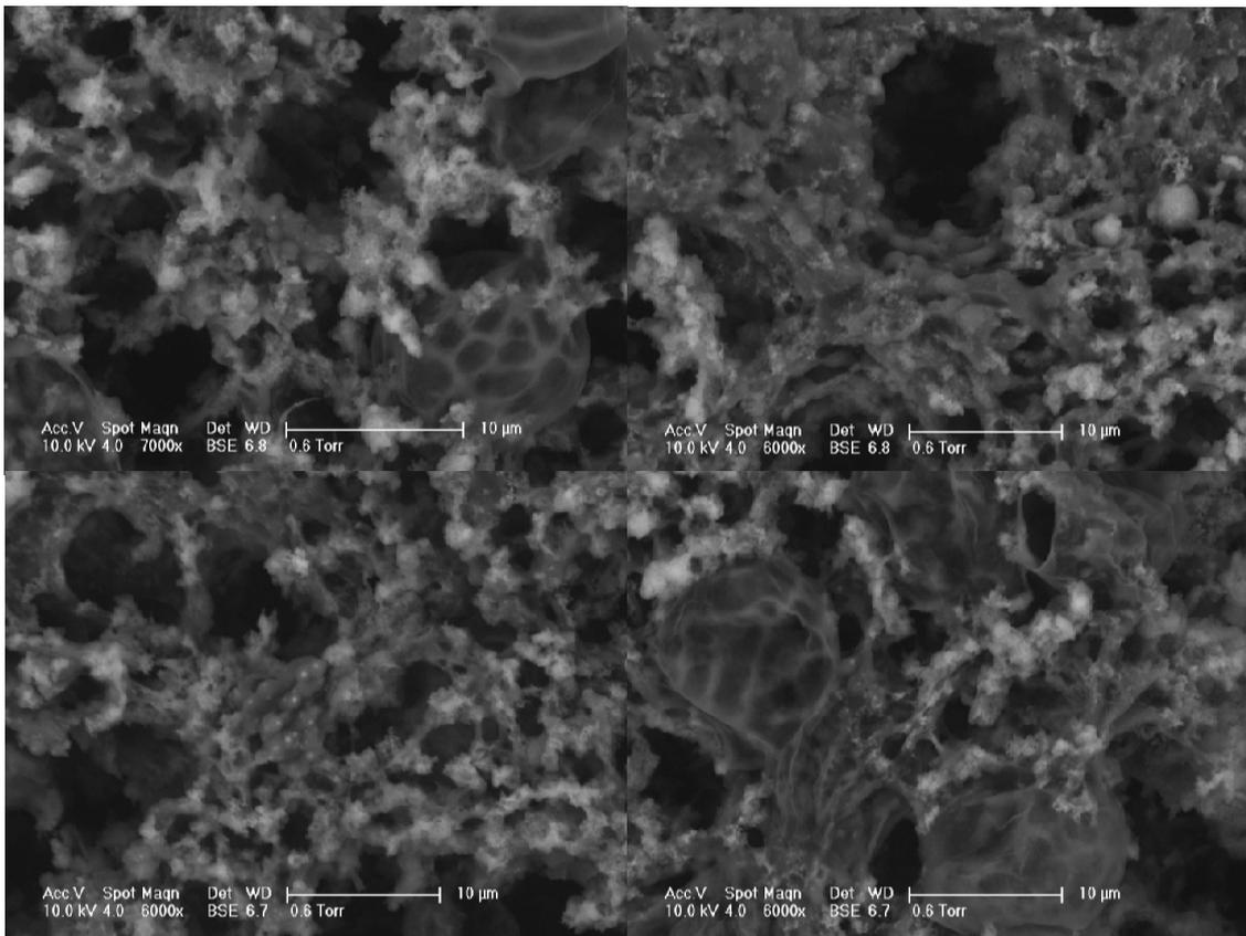
Figure 3.5. Environmental scanning electron microscopy of microorganisms in activated sludge acclimated with phenol and 2-NP.
