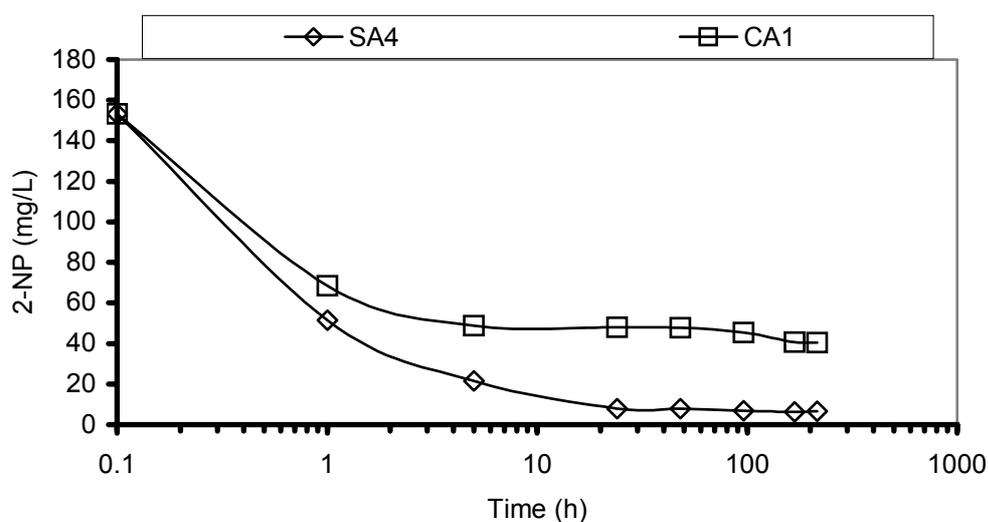
Figure 4.40. 2-Nitrophenol profiles during adsorption onto 1 g/L of activated carbons SA4 and CA1.
