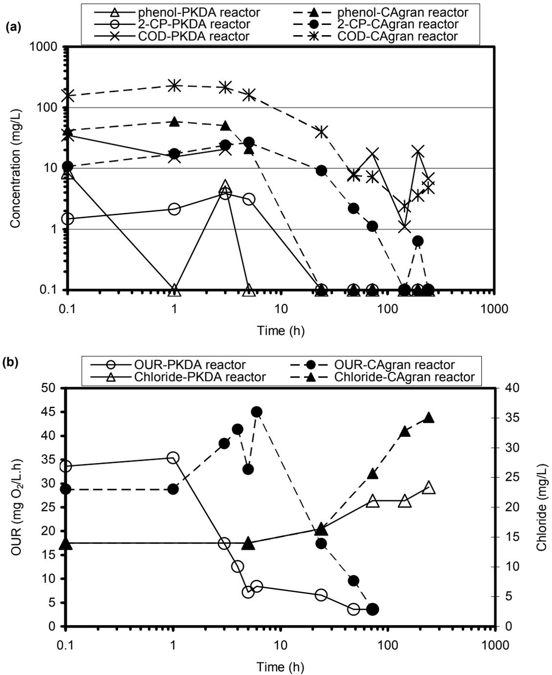
Figure 4.35. a) Phenol, 2-CP and COD profiles b) OUR and chloride profiles in bioregeneration reactors with PKDA (granular, thermally activated) and CAgran (granular, chemically activated) in RUN 15.
