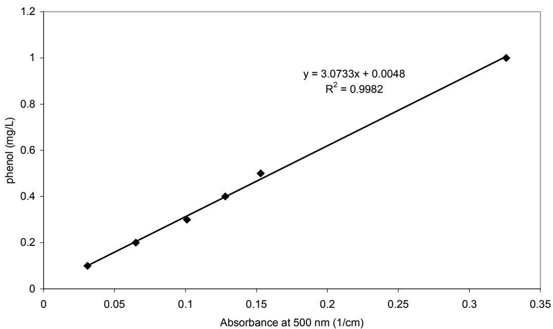
Figure A.3. Calibration curve for phenol analysis with the 4-aminoantipyrine method within the concentration range of 0.1-1 mg/L.
