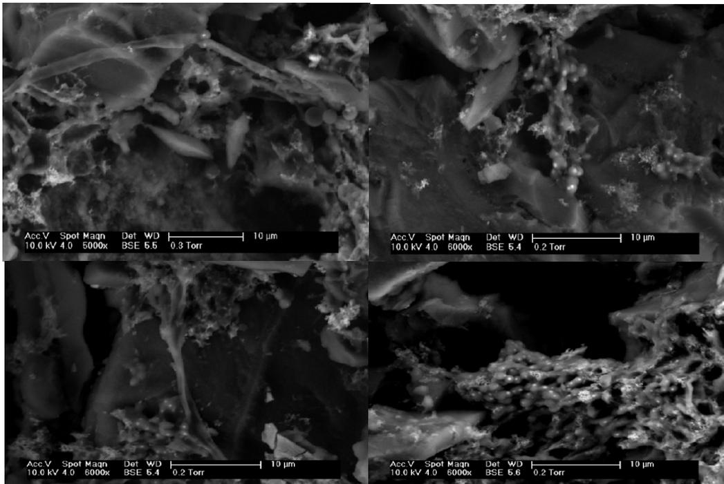
Figure 4.37 Scanning Electron Micrographs of microorganisms on CA1 in RUN 14.
