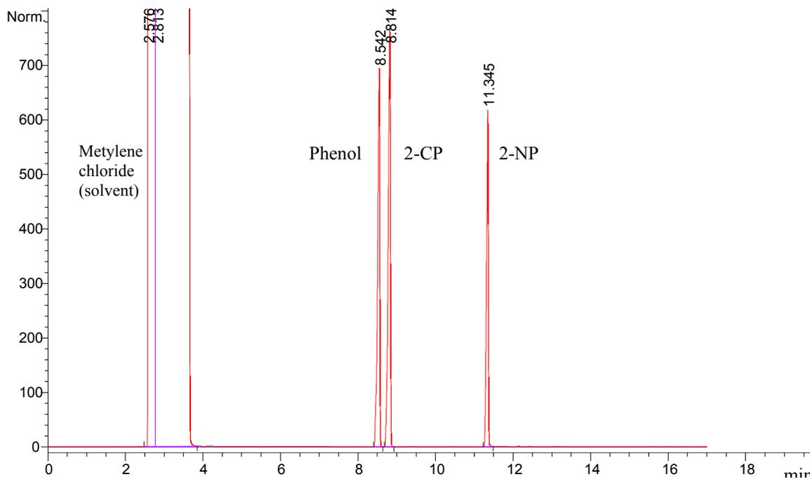
Figure A.6. Example of a gas chromatogram for a sample containing 200 mg/L of each compound; phenol, 2-chlorophenol (2-CP) and 2-nitrophenol (2-NP).
