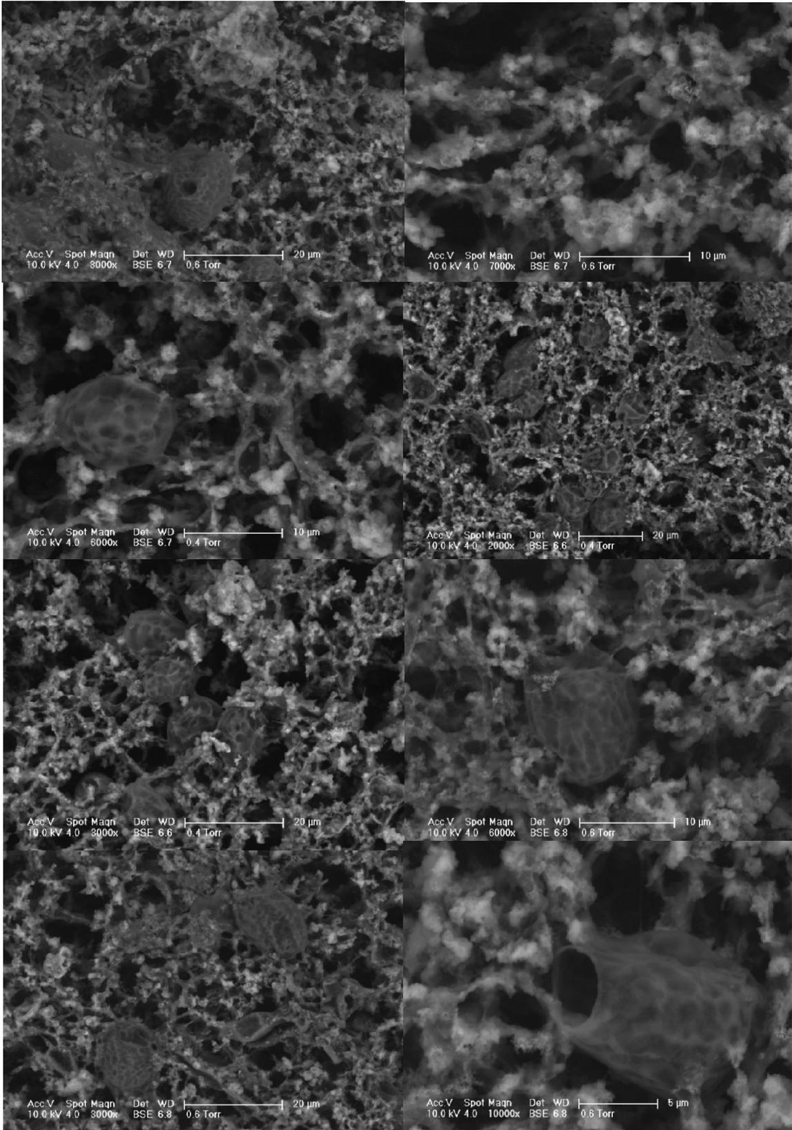
Figure B.3. Environmental scanning electron microscopy of activated sludge acclimated to phenol and 2-nitrophenol.
