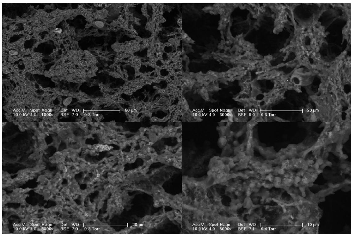
Figure 3.3. Environmental scanning electron microscopy of microorganisms and flocs in non-acclimated activated sludge taken from the mother reactor.
