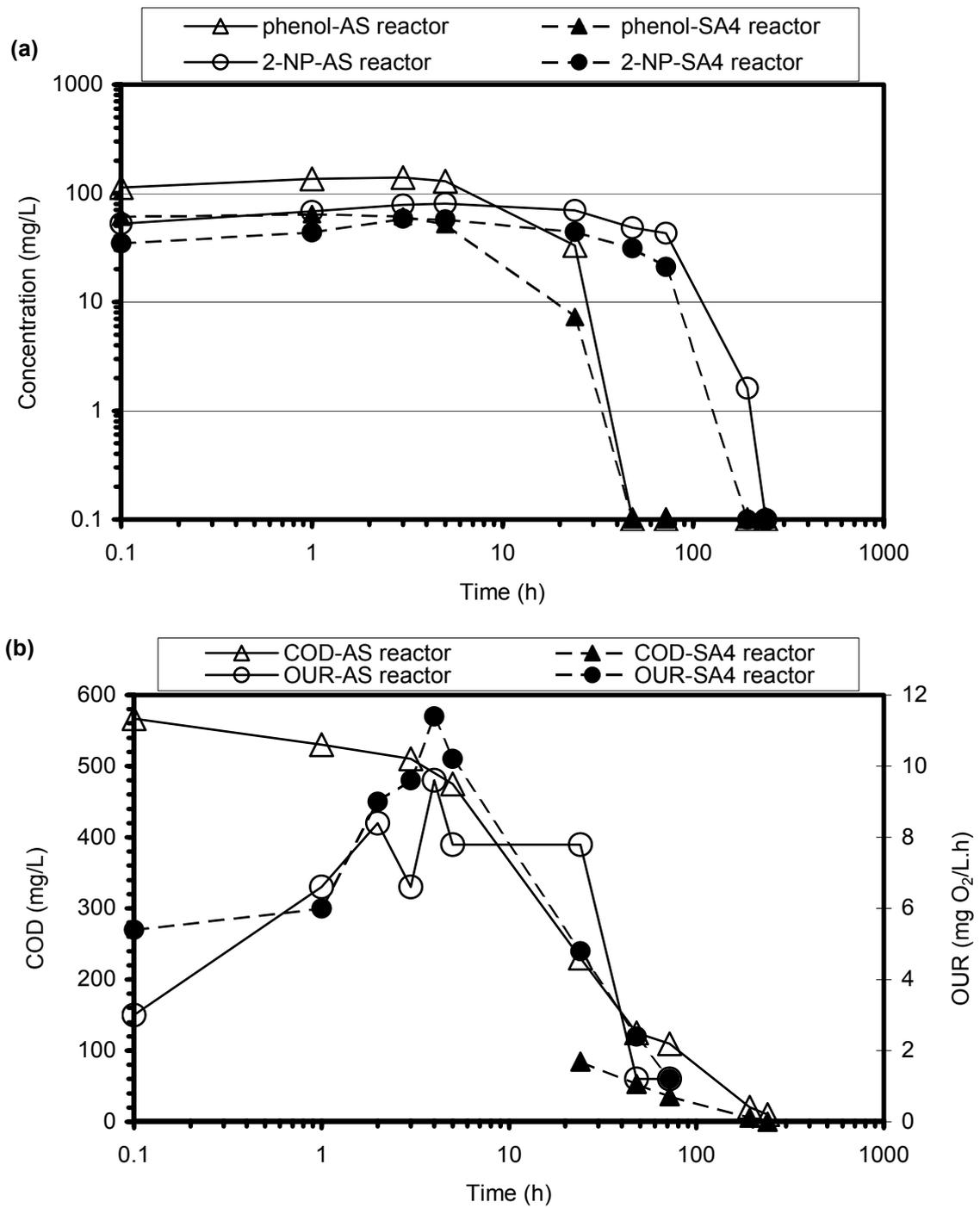
Figure 4.44. a) Phenol and 2-NP profiles b) COD and OUR profiles in biodegradation reactor and bioregeneration reactor with 2000 mg/L SA4 (powdered, thermally activated) in RUN 17.
