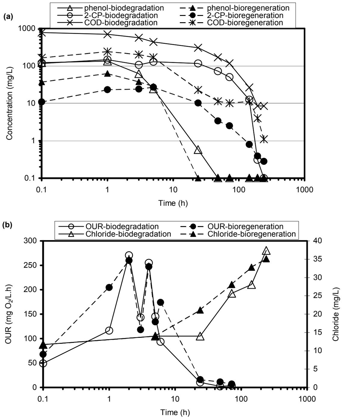
Figure 4.33. a) Phenol, 2-CP and COD profiles b) OUR and chloride profiles in biodegradation reactor and bioregeneration reactor with 2000 mg/L CAgran (granular, chemically activated) in RUN 13.
