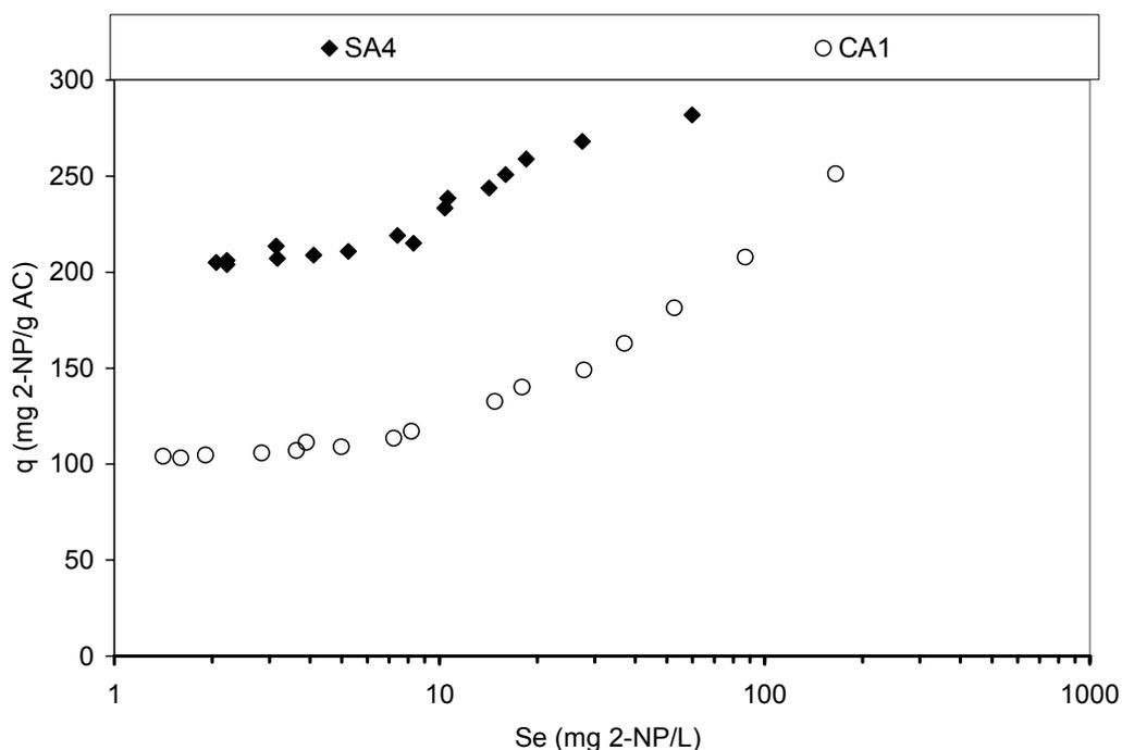
Figure 4.42. 2-Nitrophenol desorption isotherms for activated carbon types SA4 and CA1.
