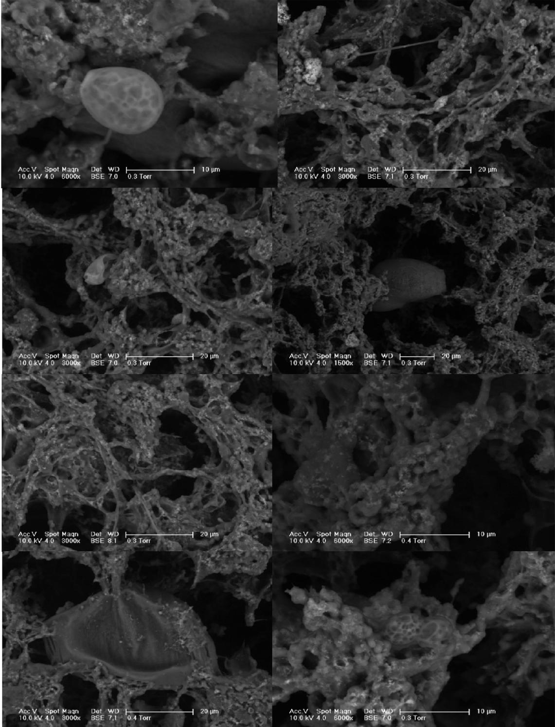
Figure B.1. Environmental scanning electron microscopy of non-acclimated activated sludge taken from the mother reactor
