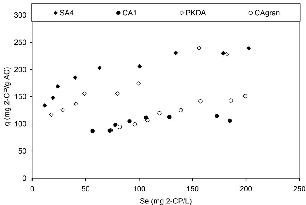
Figure 4.18. 2-Chlorophenol adsorption isotherms for each activated carbon type SA4 (powdered, thermally activated), CA1 (powdered, chemically activated), PKDA (granular, thermally activated) and CAgran (granular, chemically activated).
