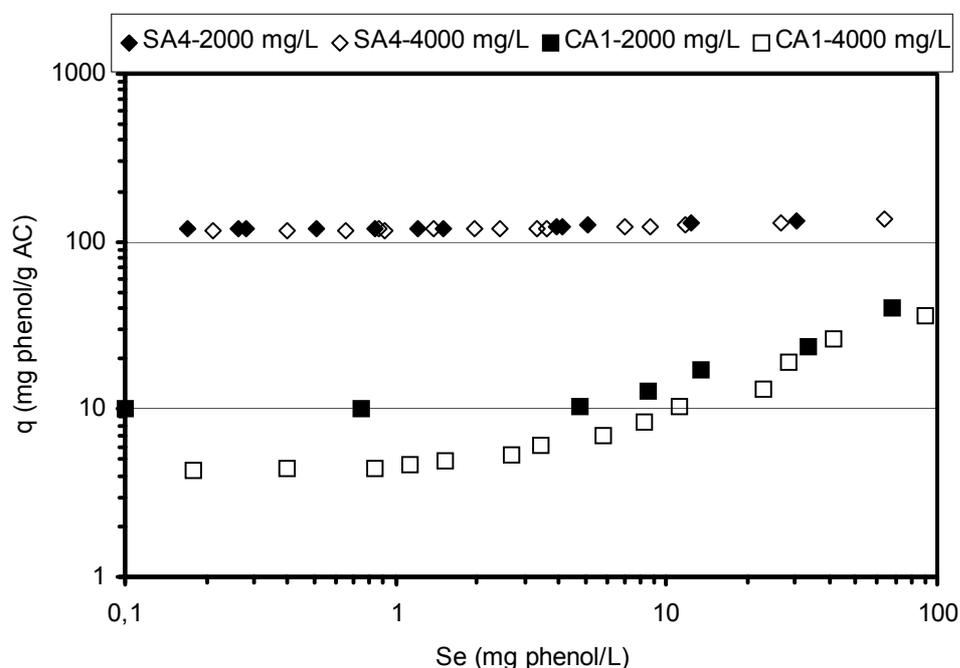
Figure 4.3. Phenol desorption isotherms for the powdered carbons SA4 (thermally activated) and CA1 (chemically activated) at doses of 2000 mg/L and 4000 mg/L .
