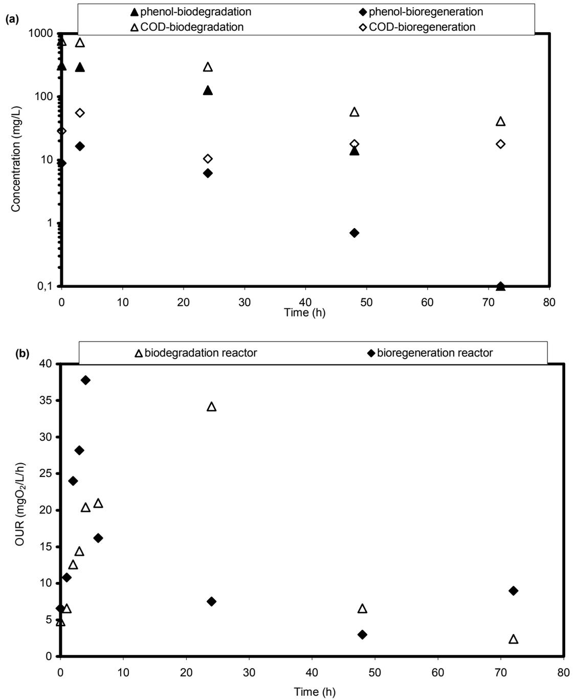
Figure 4.10. a) Phenol and COD profiles b) OUR profiles in biodegradation reactor and bioregeneration reactor with 2000 mg/L PKDA (granular, thermally activated) in RUN 4.
