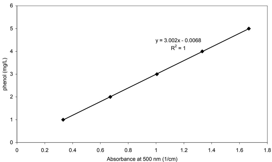
Figure A.4. Calibration curve for phenol analysis with the 4-aminoantipyrine method within the concentration range of 1-5 mg/L.
