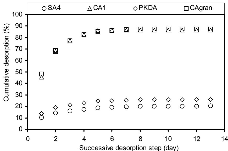
Figure 4.6. Cumulative desorption of phenol from loaded activated carbons at the end of each successive desorption step.
