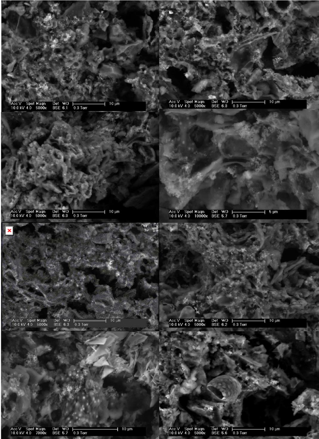
Figure B.4. Environmental scanning electron micrographs of microorganisms on SA4 carbon at t=3 days in RUN 14.
