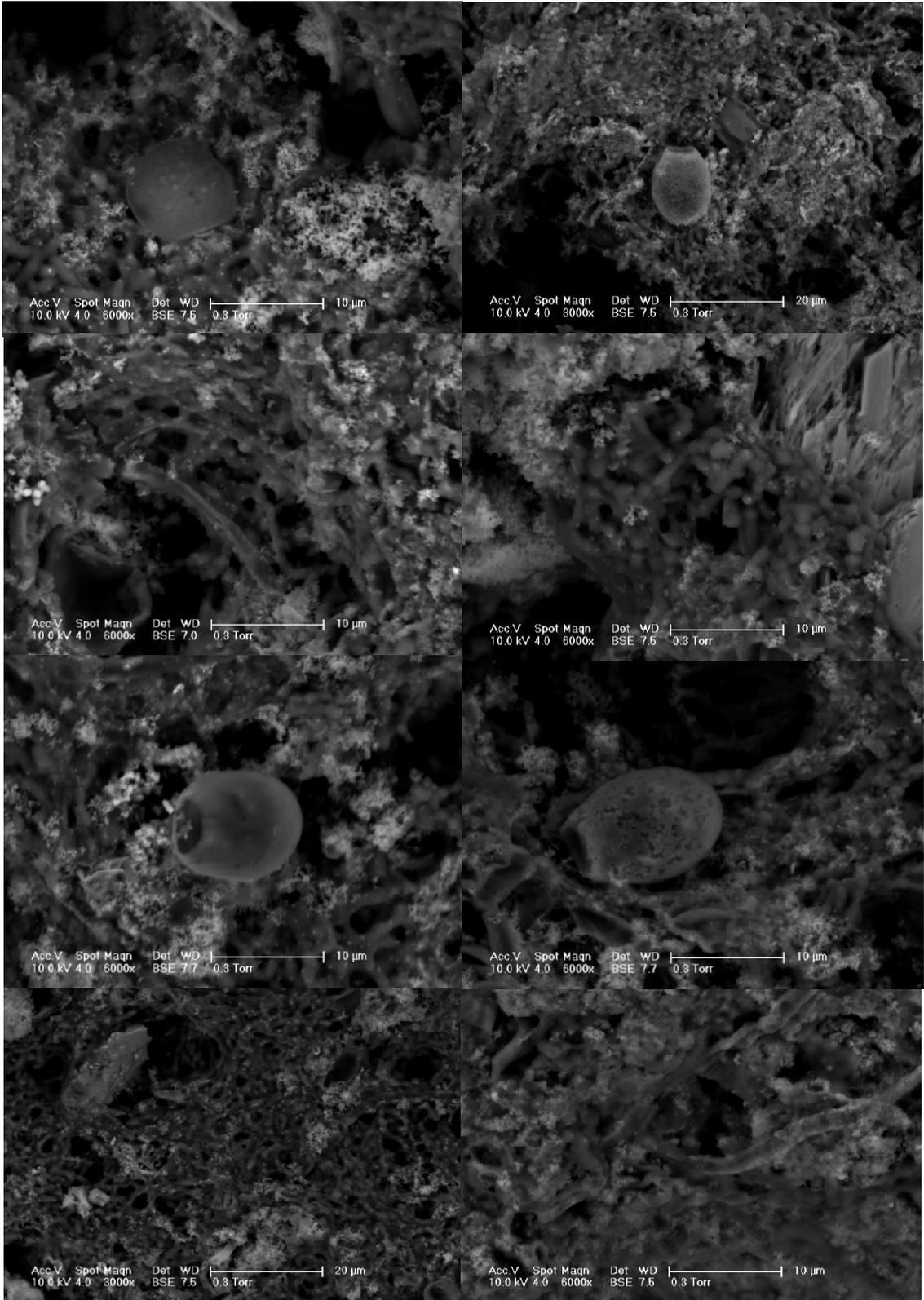
Figure B.2. Environmental scanning electron microscopy of activated sludge acclimated to phenol and 2-chlorophenol.
