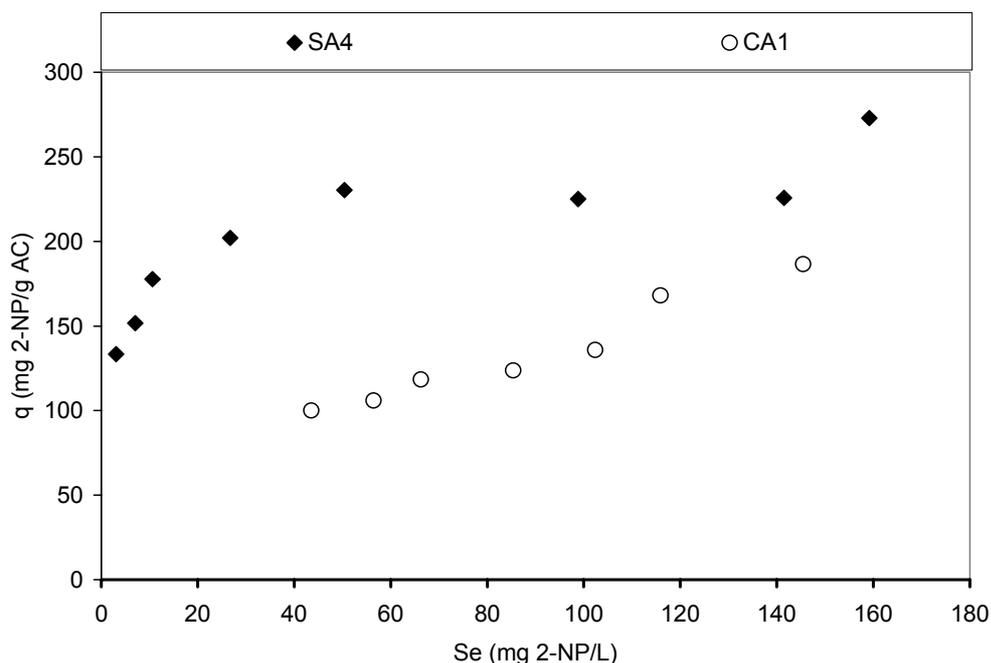
Figure 4.41. 2-Nitrophenol adsorption isotherms for activated carbon types SA4 and CA1.
