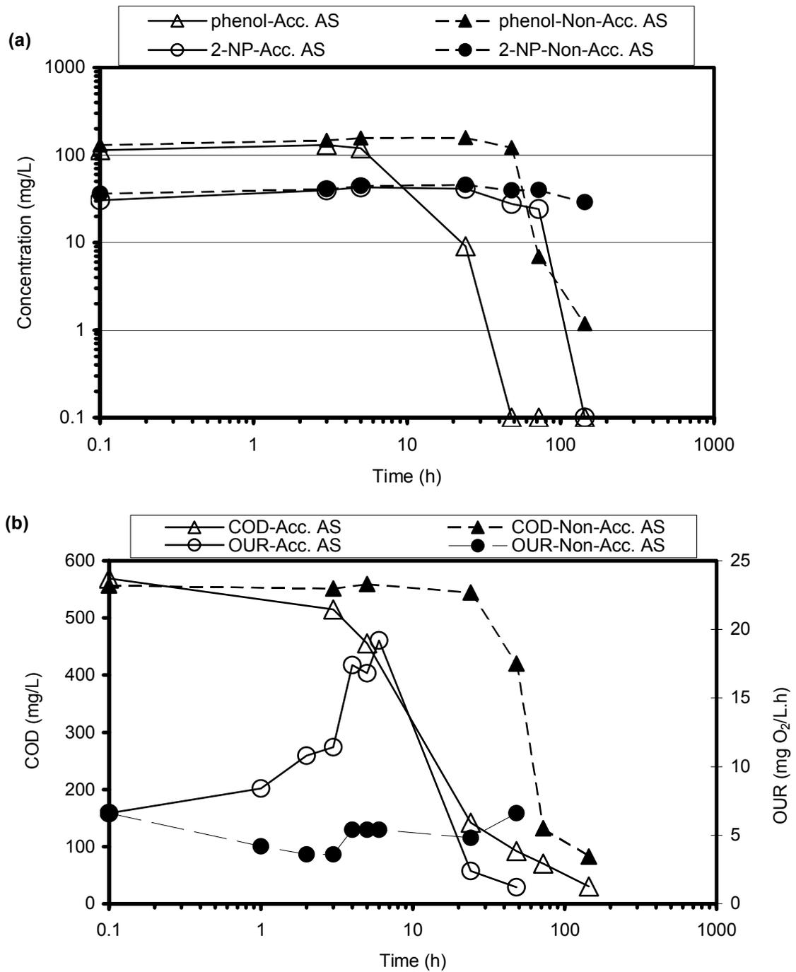
Figure 4.43. a) Phenol and 2-NP profiles b) COD and OUR profiles in biodegradation reactors receiving acclimated (Acc. AS) and non-acclimated (Non-Acc. AS) activated sludges in RUN 16.
