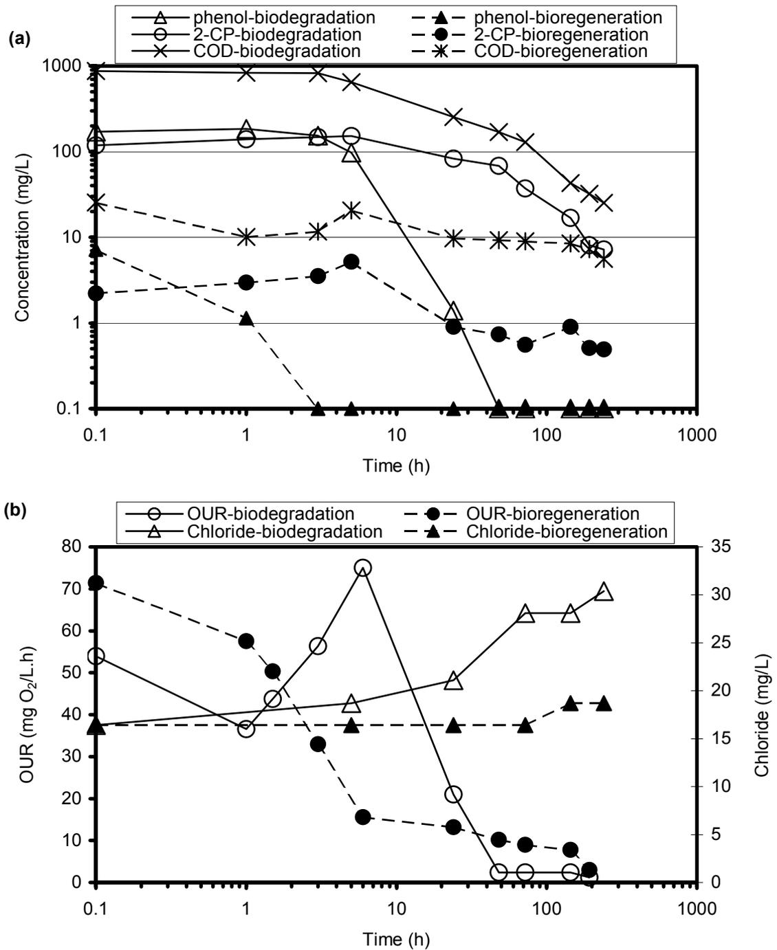
Figure 4.32. a) Phenol, 2-CP and COD profiles b) OUR and chloride profiles in biodegradation reactor and bioregeneration reactor with 2000 mg/L PKDA (granular, thermally activated) in RUN 12.
