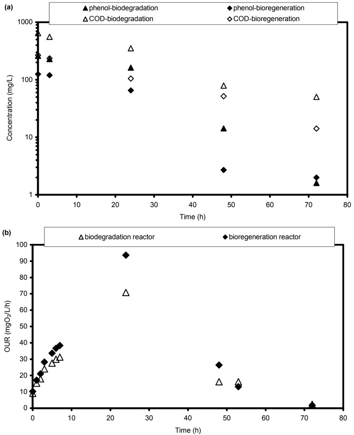
Figure 4.9. a) phenol and COD profiles b) OUR profiles in biodegradation reactor and bioregeneration reactor with 2000 mg/L CA1 (powdered, chemically activated) in RUN 3.
