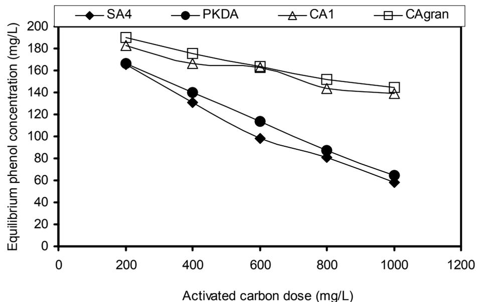
Figure 4.2. Effect of activated carbon dose on equilibrium phenol concentrations with an initial phenol concentration of 200 mg/L.
