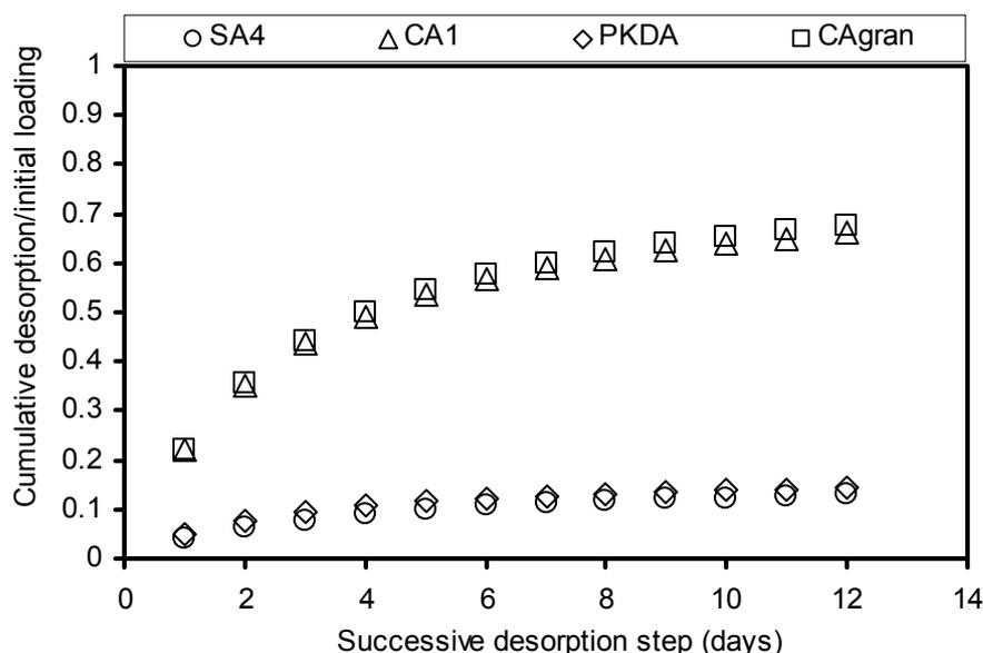
Figure 4.22. Cumulative desorption of 2-chlorophenol from loaded activated carbons at the end of each successive desorption step (SA4: powdered, thermally activated, CA1: powdered, chemically activated, PKDA: granular, thermally activated and CAgran: granular, chemically activated).
