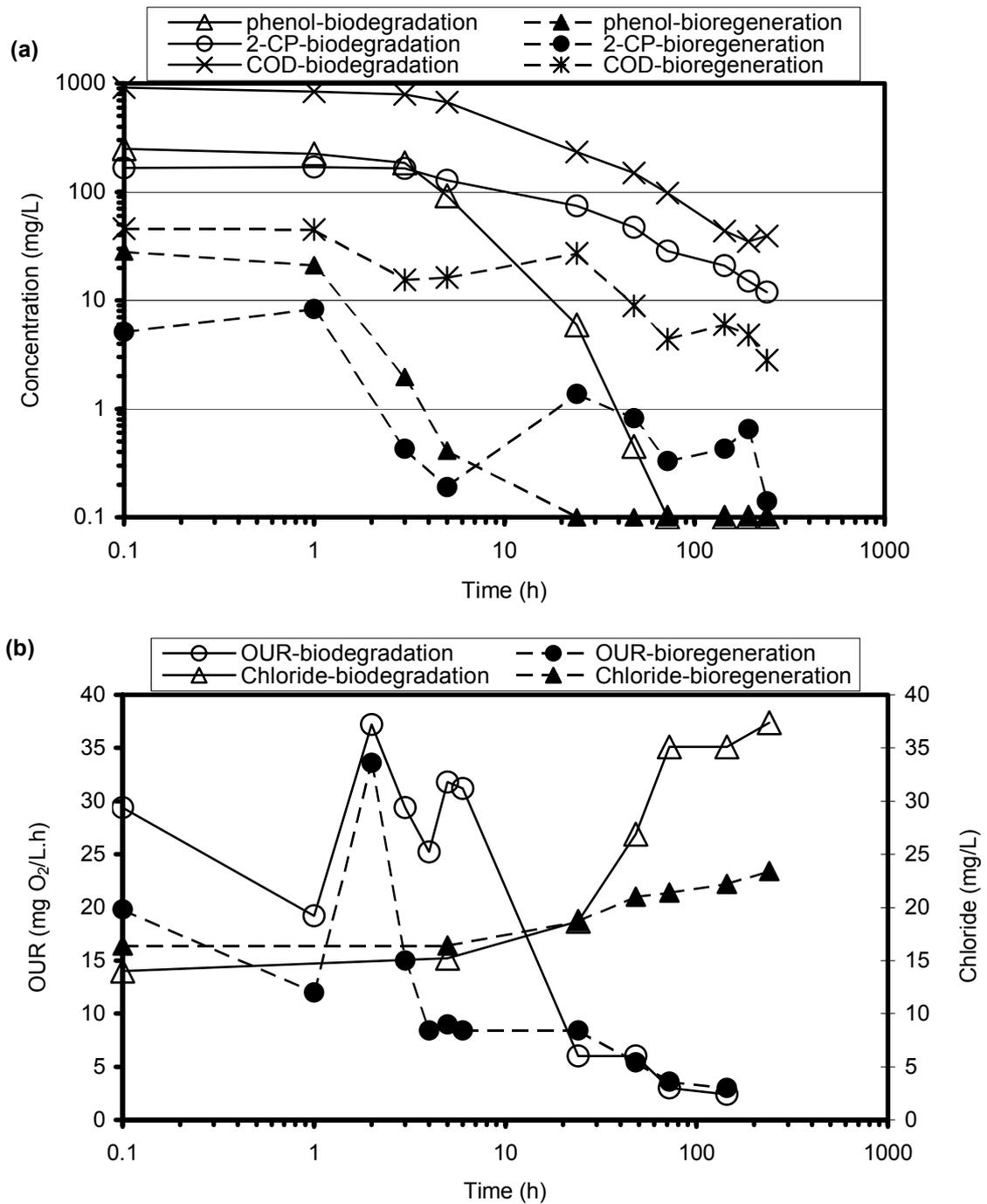
Figure 4.30. a) Phenol, 2-CP and COD profiles b) OUR and chloride profiles in biodegradation reactor and bioregeneration reactor with 2000 mg/L SA4 (powdered, thermally activated) in RUN 10.
