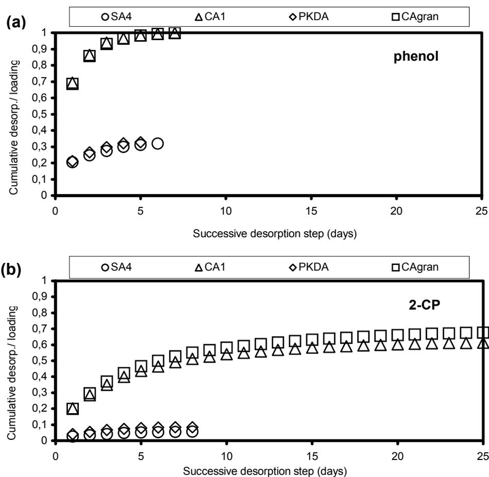
Figure 4.29. Cumulative desorption of a) phenol and b) 2-CP from competitively loaded activated carbons at the end of each successive desorption step
