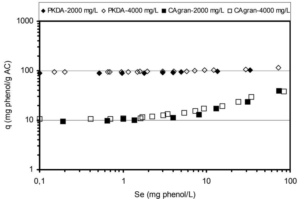
Figure 4.4. Phenol desorption isotherms for the granular carbons PKDA (thermally activated) and CAgran (chemically activated) at doses of 2000 mg/L and 4000 mg/L.
