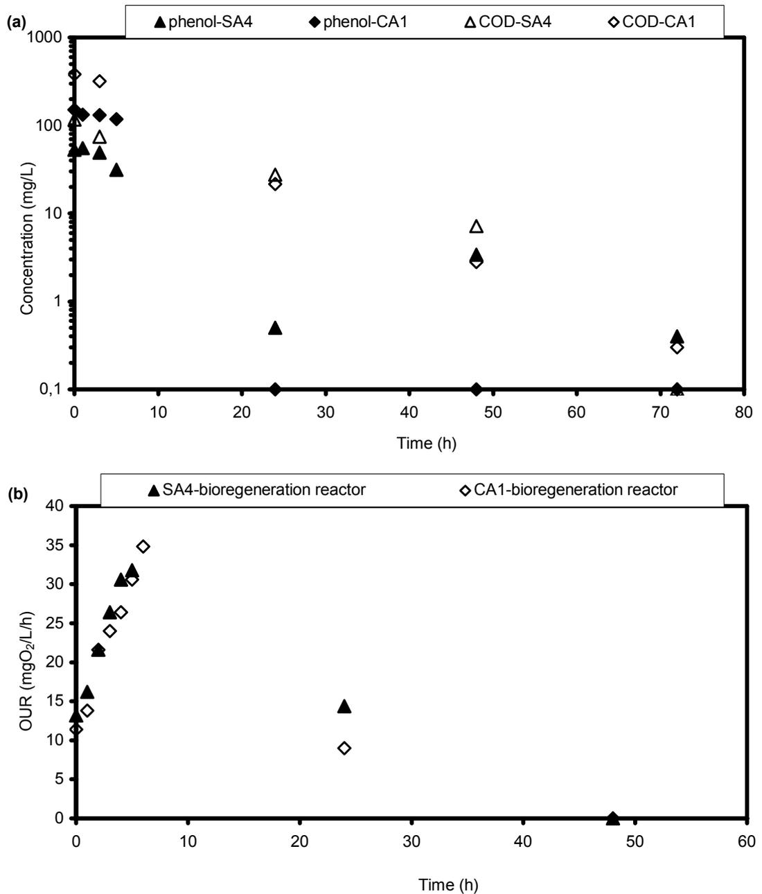
Figure 4.12. a) Phenol and COD profiles b) OUR profiles in bioregeneration reactors with 2000 mg/L SA4 (powdered, thermally activated) and CA1 (powdered, chemically activated) in RUN 6.
