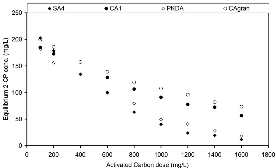
Figure 4.19. Effect of activated carbon dose on equilibrium 2-chlorophenol concentrations with an initial 2-chlorophenol concentration of 200 mg/L for each activated carbon type.
