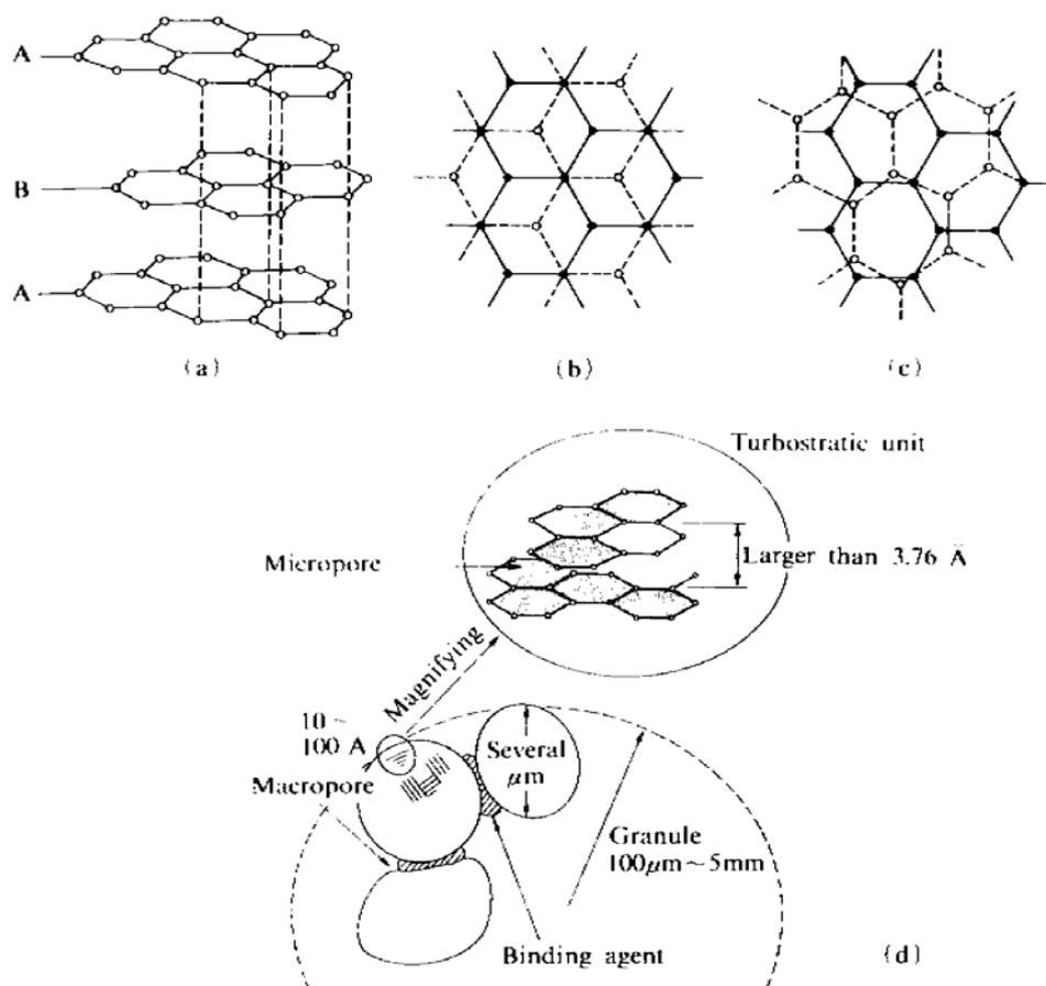
Figure 2.1. Graphite structure (a,b) and turbostratic structure (c) of activated carbon. Conceptual illustration of granular activated carbon (d) (Suzuki, 1990).
