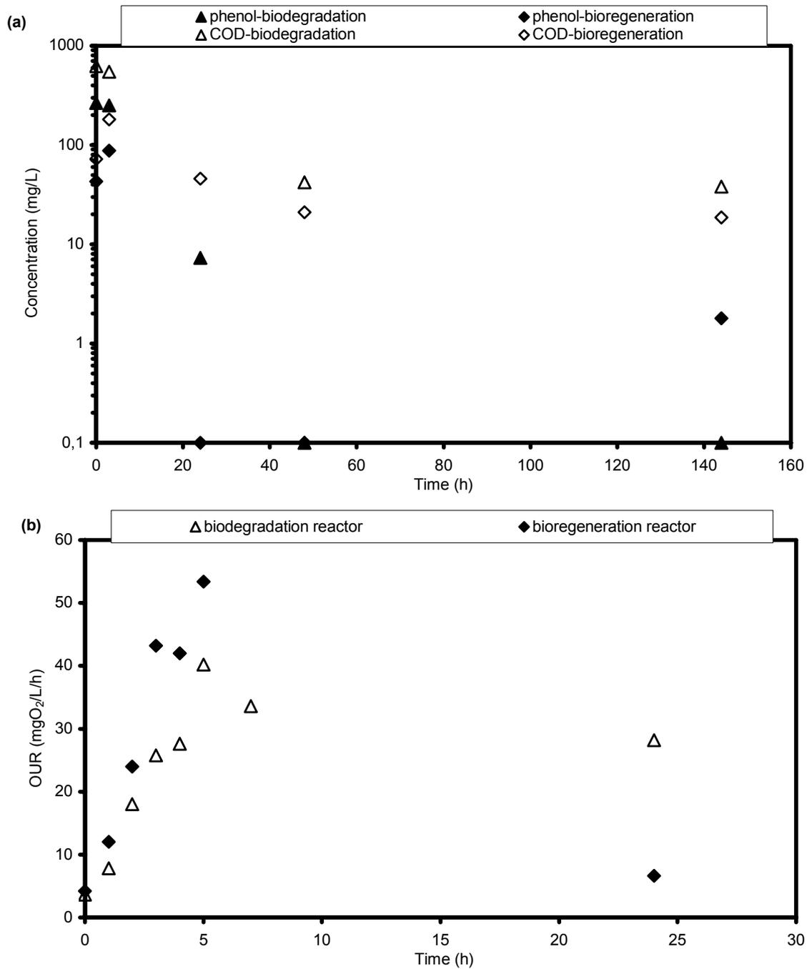
Figure 4.11. a) Phenol and COD profiles b) OUR profiles in biodegradation reactor and bioregeneration reactor with 2000 mg/L CAgan (granular, chemically activated) in RUN 5.
