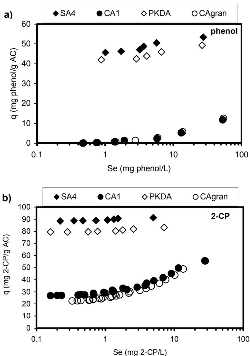
Figure 4.28. Competitive desorption isotherms of each activated carbon type for a) phenol and b) 2-CP.
