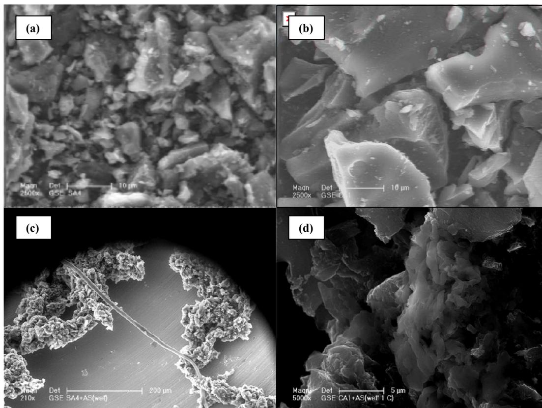
Figure 4.16. Scanning Electron Micrographs of a) virgin dry SA4 b) virgin dry CA1 c) slime matrix covering parts of carbon surface forming a bright white gelatinous structure. d) Slime matrix covering microorganisms on activated carbon
