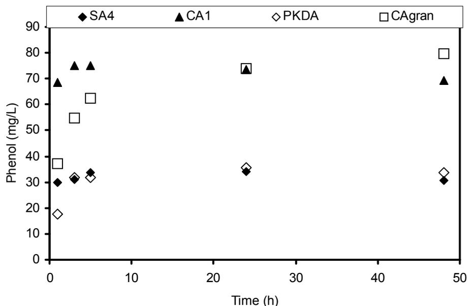
Figure 4.5. Desorption of phenol from the four loaded activated carbons with respect to time.
