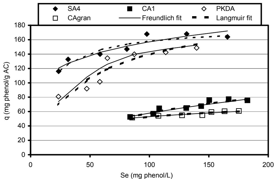
Figure 4.1. Phenol adsorption isotherms for the powdered carbons SA4 (thermally activated) and CA1 (chemically activated) and granular carbons PKDA (thermally activated) and CAgran (chemically activated) with their Freundlich and Langmuir fits.
