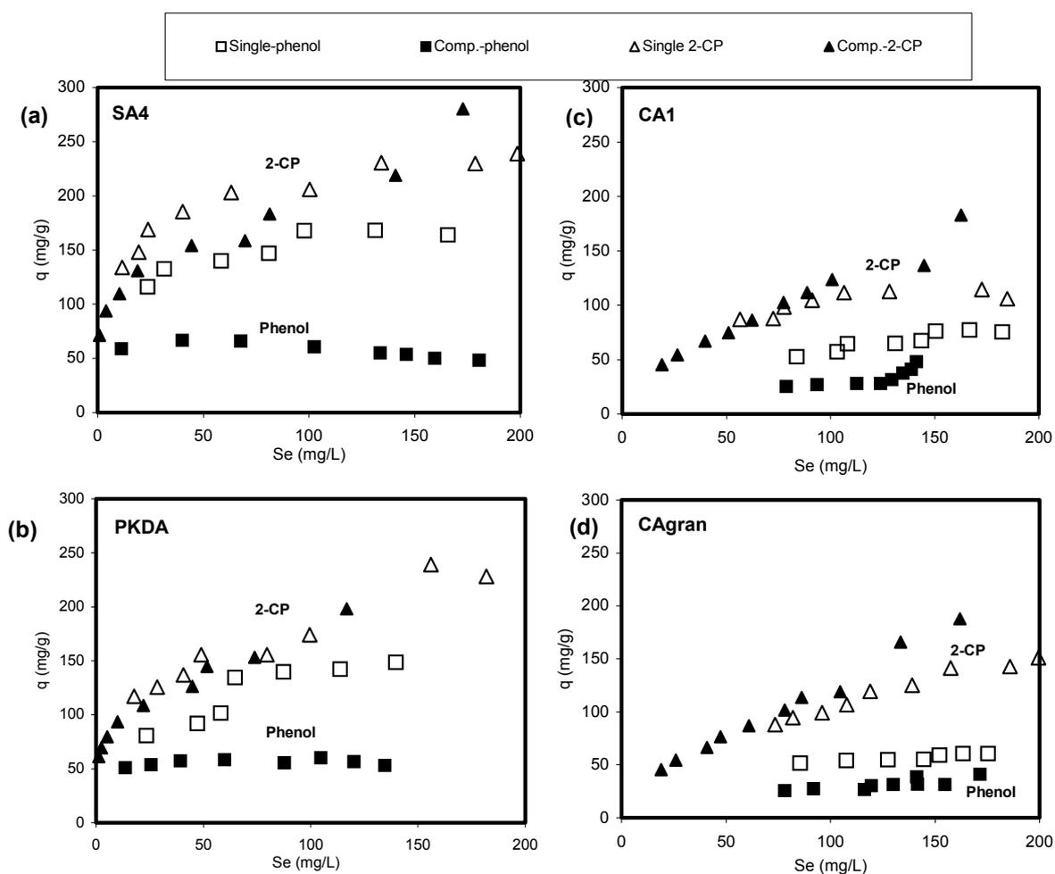
Figure 4.25. Competitive bi-solute and single-solute adsorption isotherms for phenol and 2-CP for a) SA4, b) PKDA, c) CA1, d) CAgran. (open data points refer to single-solute adsorption, closed data points refer to bi-solute adsorption).
