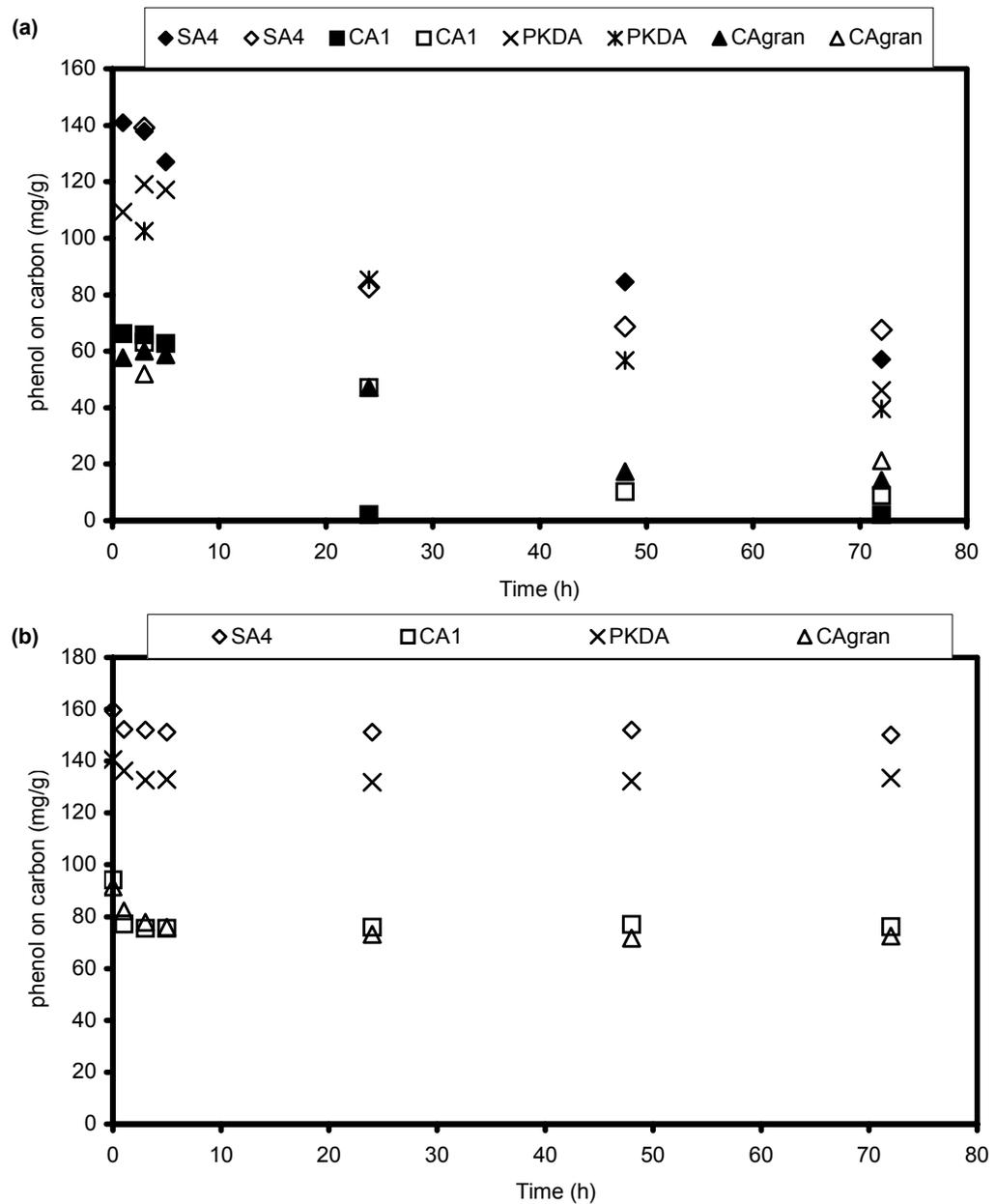
Figure 4.14. Profiles of phenol loadings on activated carbons SA4 (powdered, thermally activated), CA1 (powdered, chemically activated), PKDA (granular, thermally activated) and CAgran (granular, chemically activated) a) in bioregeneration reactors in RUNS 2-7 and b) during desorption equilibrium.
