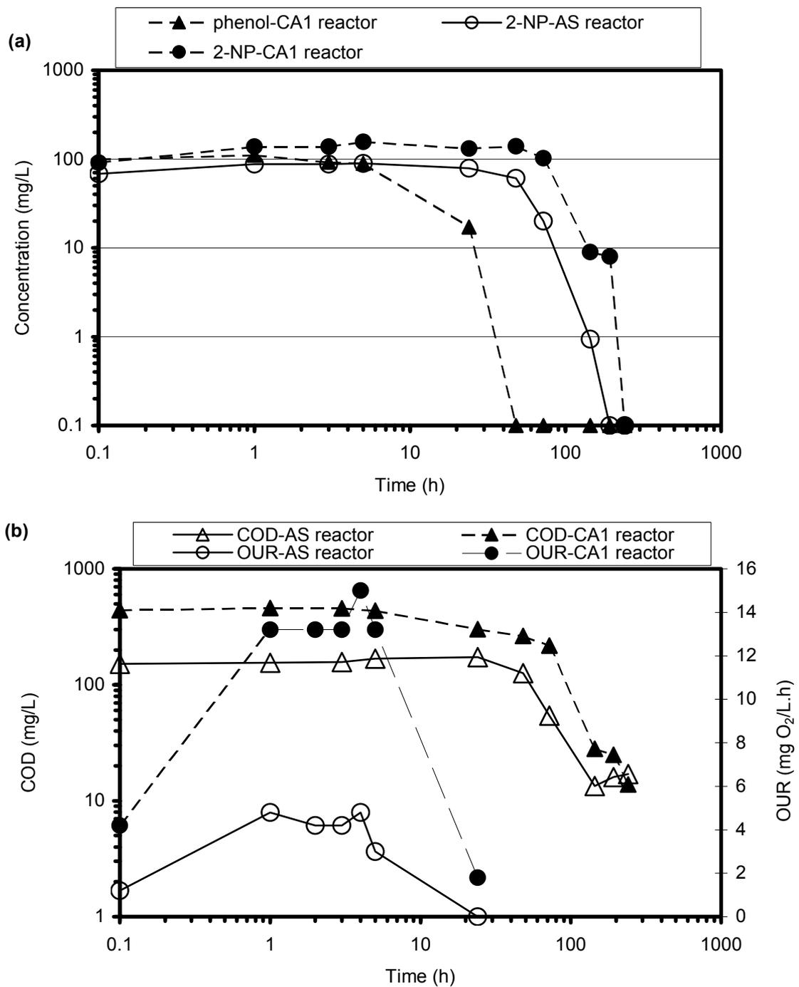
Figure 4.45. a) Phenol and 2-NP profiles b) COD and OUR profiles in biodegradation reactor (receives 2-NP as the only carbon source) and bioregeneration reactor with 2000 mg/L CA1 (powdered, chemically activated) in RUN 18
