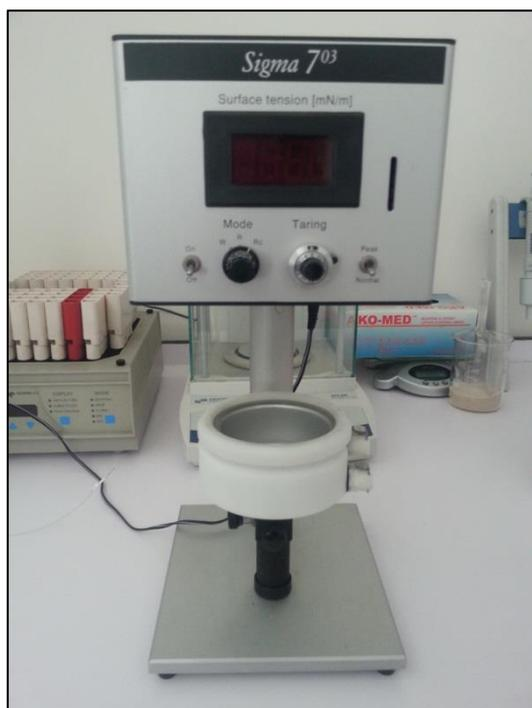
Figure 4.1. Interfacial tension meter (KSV 703 Digital Tensiometer).
