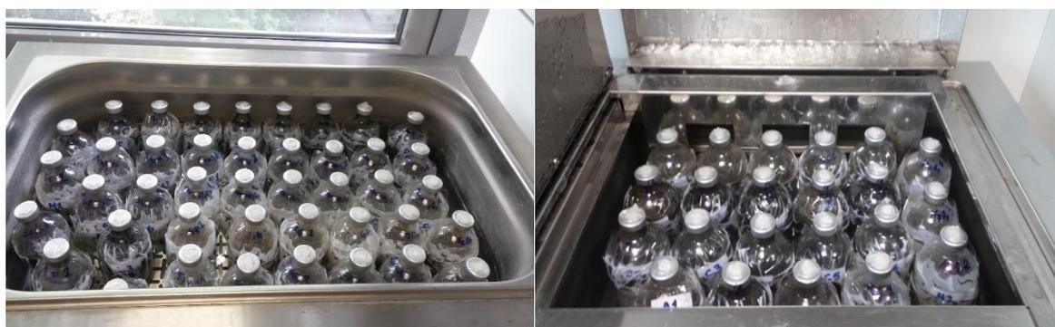
Figure 4.4. The anaerobic batch reactors at  $37^\circ\text{C}$  in water bathes.
