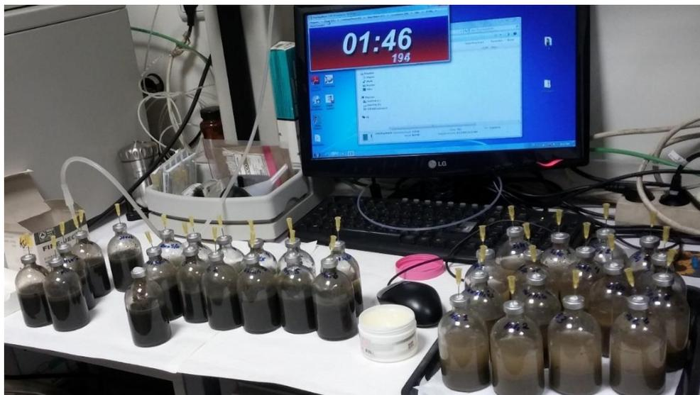
Figure 4.3. Reactors during flushing with nitrogen gas.
