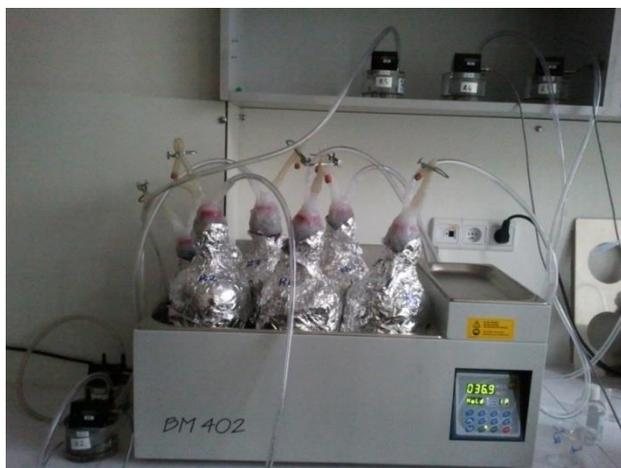
Figure 3.4. Anaerobic reactors used in this study.
