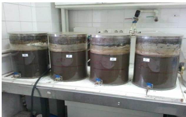
Figure 3.5. Aerobic reactors used in this study.
