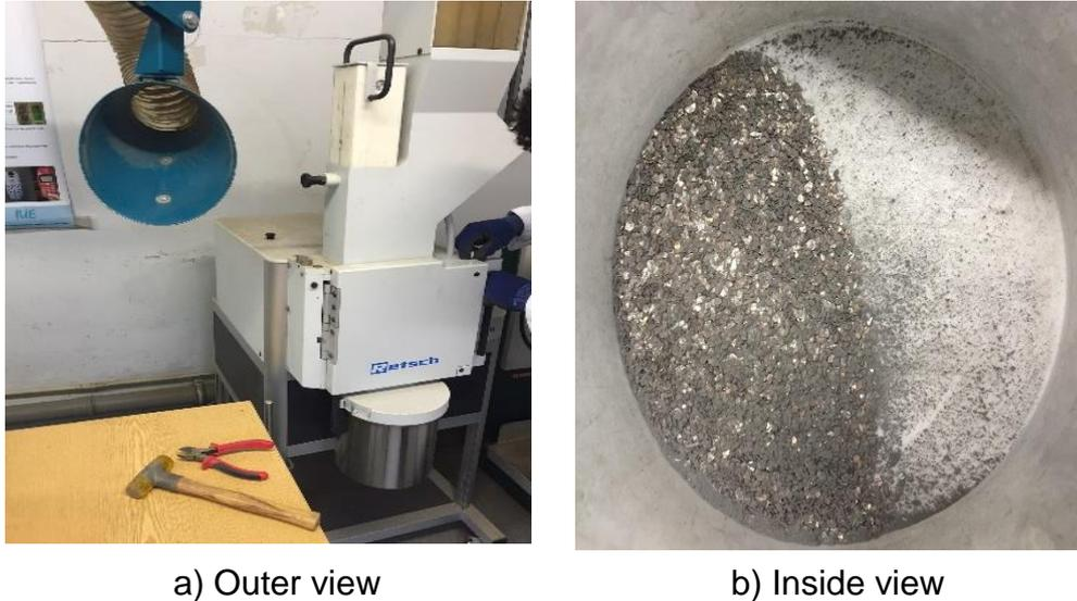
Figure 4.1. Mechanical miller (Retsch SM 300, Germany) used in the size reduction at TUHH.
