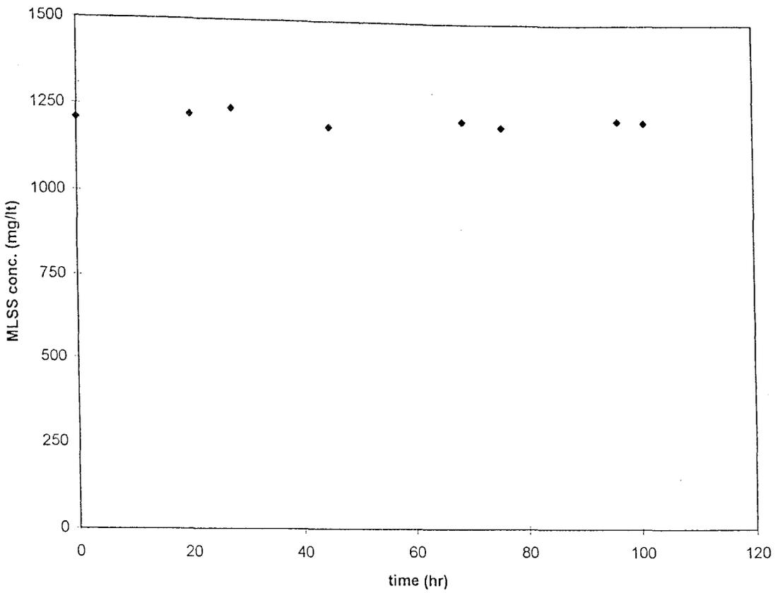
Figure 6.46: Change in MLSS Concentration of Run 7a
