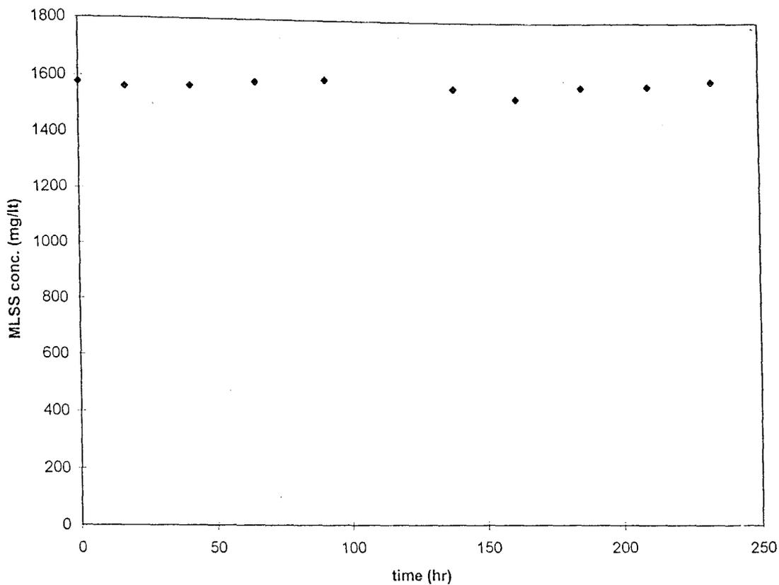
Figure 6.3: Change in MLSS Concentration of Acclimation Run 1
