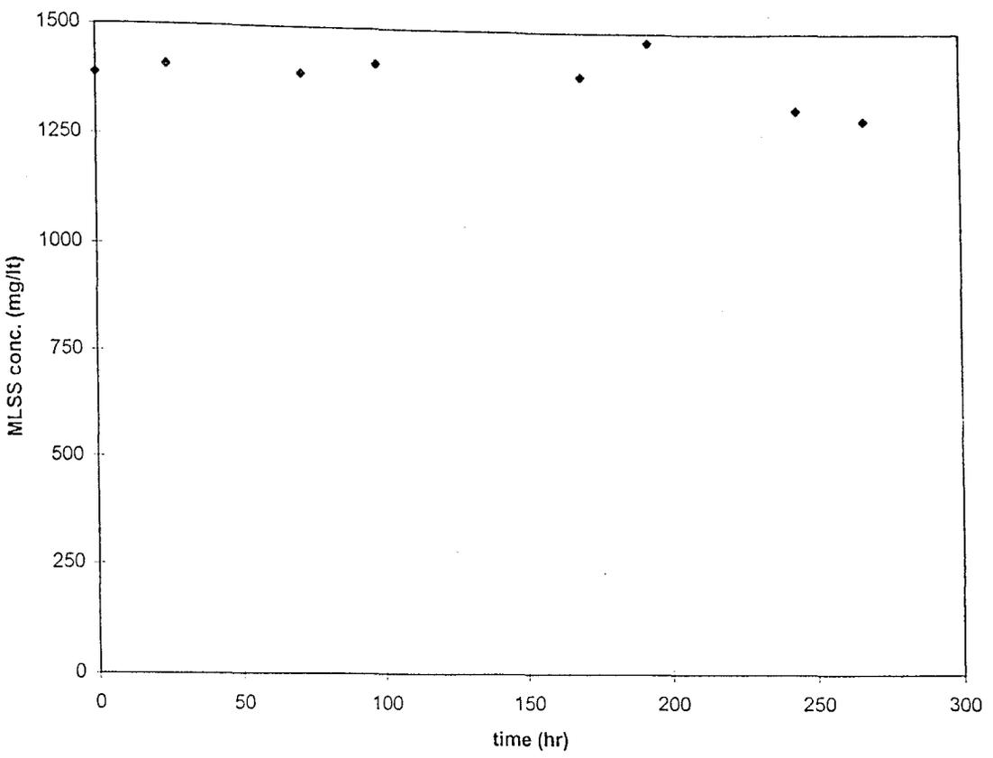
Figure 6.36: Change in MLSS Concentration of Run 6a
