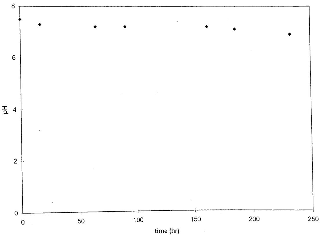
Figure 6.12: Change in pH of Acclimation Run 3
