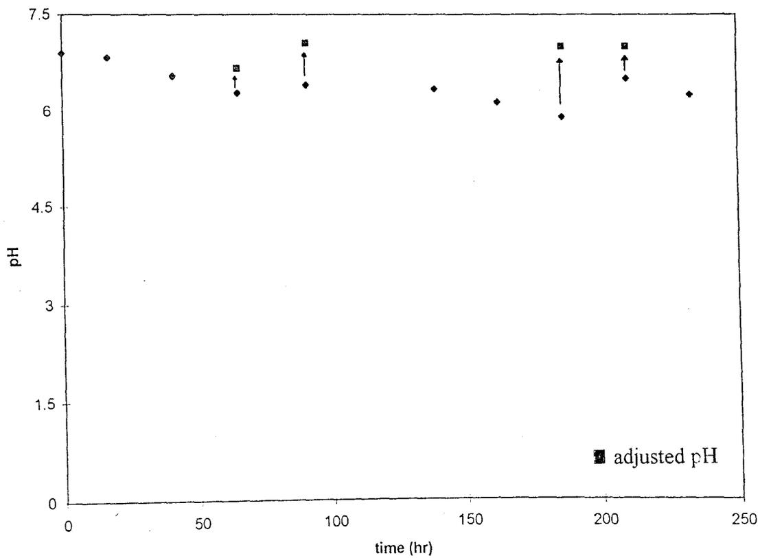
Figure 6.4: Change in pH of Acclimation Run 1
