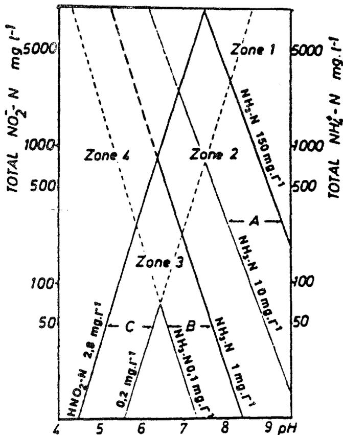
FIGURE 3.1: Nitrification Tolerance Graph, (Anthonisen, et al., 1976)
