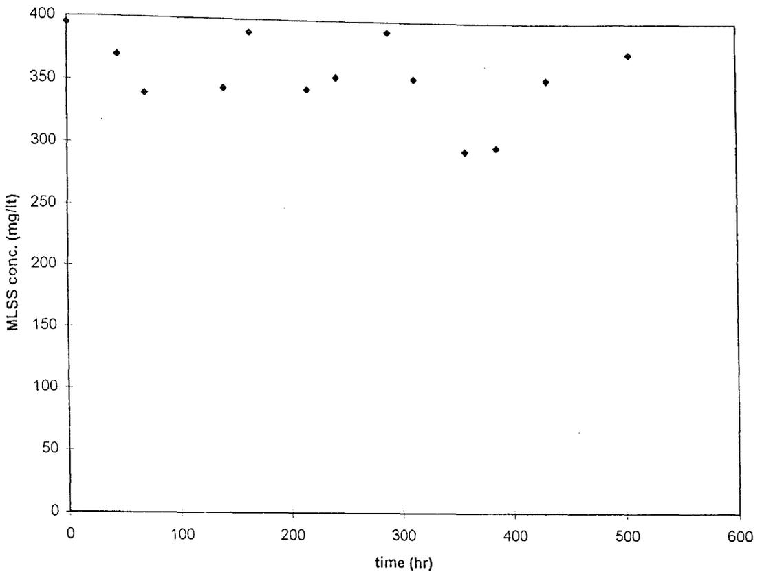
Figure 6.26: Change in MLSS Concentration of Run 5b
