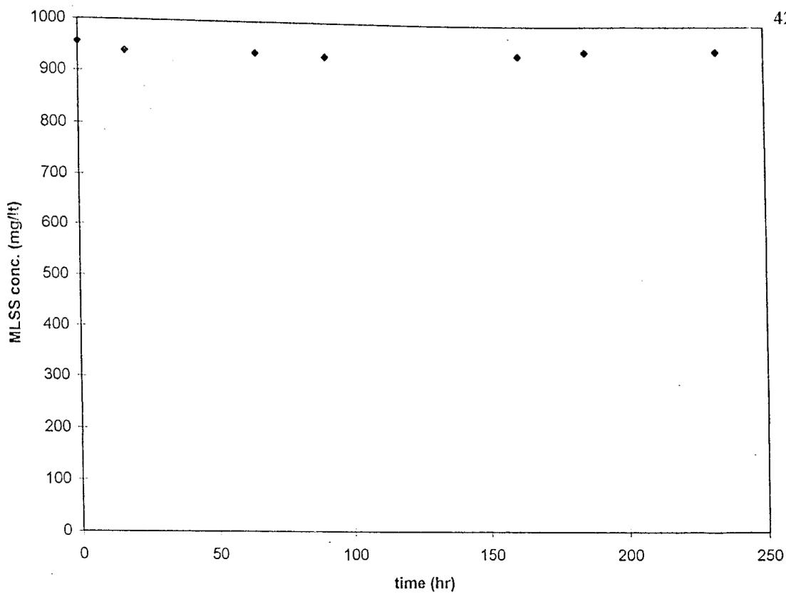
Figure 6.11: Change in MLSS Concentration of Acclimation Run 3
