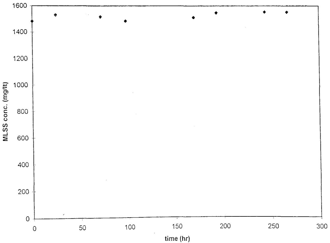
Figure 6.41: Change in MLSS Concentration of Run 6b
