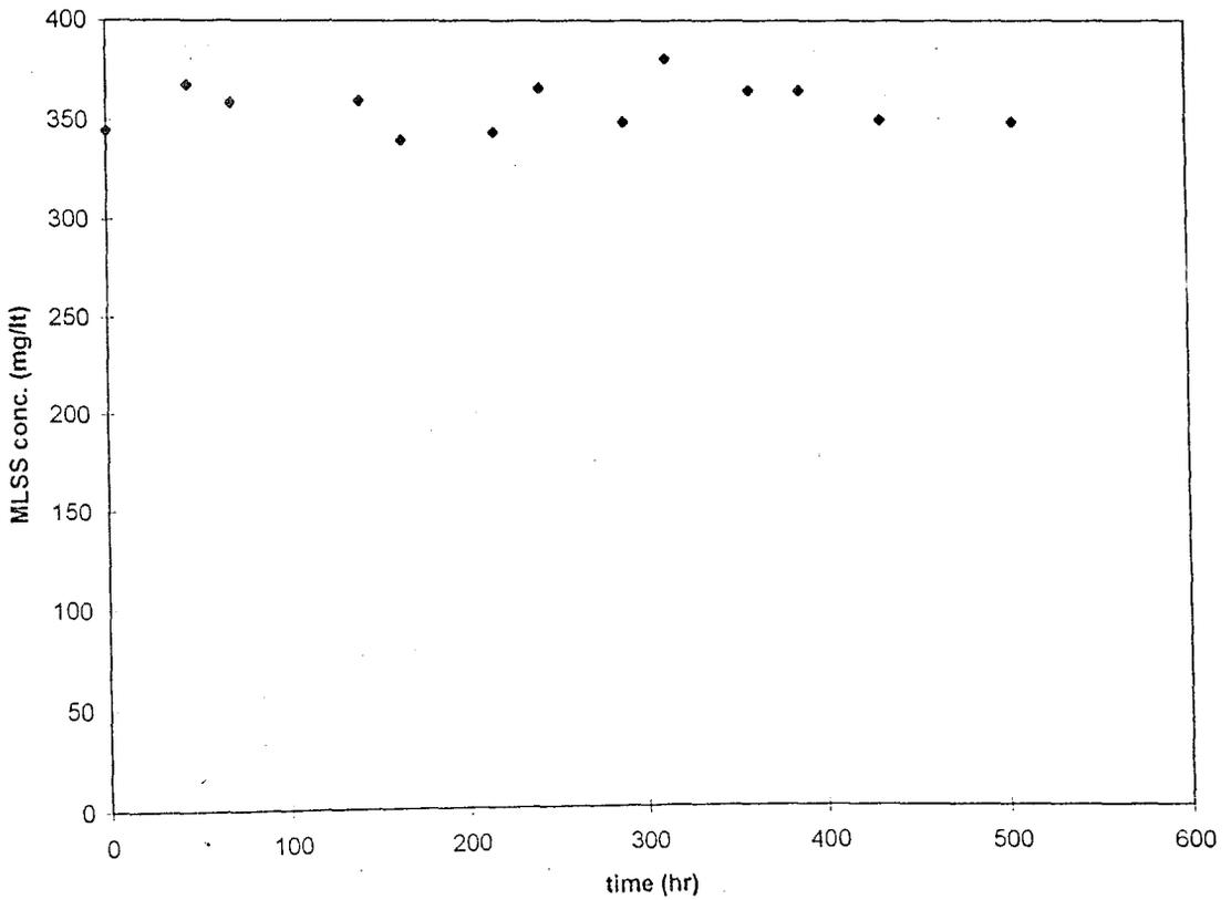
Figure 6.31: Change in MLSS Concentration of Run 5c
