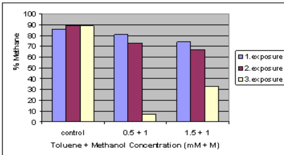
Figure 5.7. Effect of toluene + methanol on methane composition.
