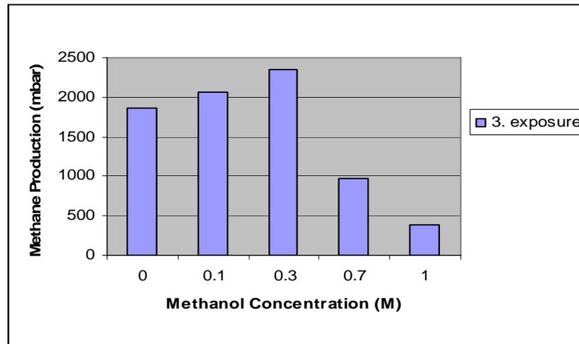
Figure 5.2. The effect of methanol on methane production.
