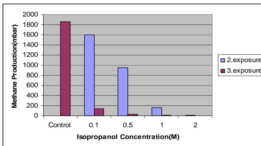
Figure 5.6. Effect of iso-propanol on methane production.
