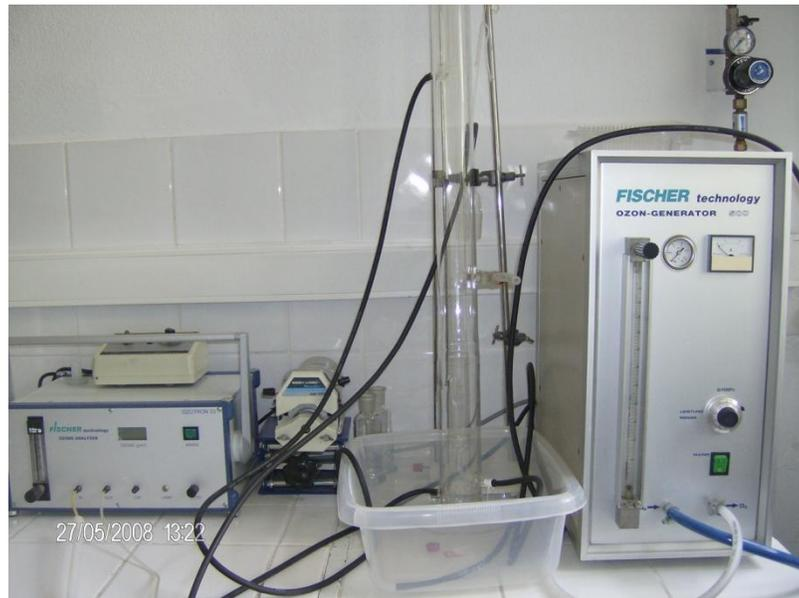
Figure 3.2. Schematic presentation (a) and image of ozone reactor (b).
