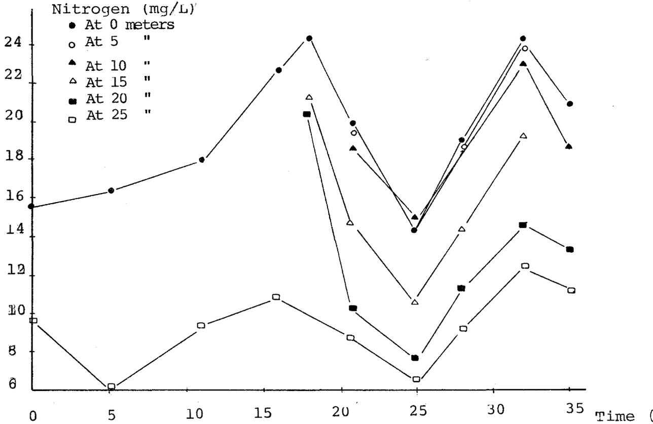
Figure 32 : Graphical Presentation Showing the Variation of Nitrogen with Time in the Channel Full with Gravel
