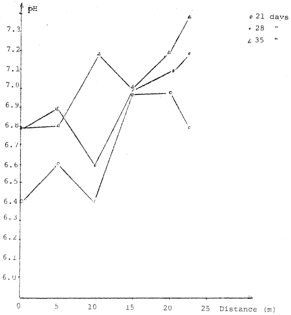
Figure 55 : Variation of pH with Distance in the Channel Full with Sand
