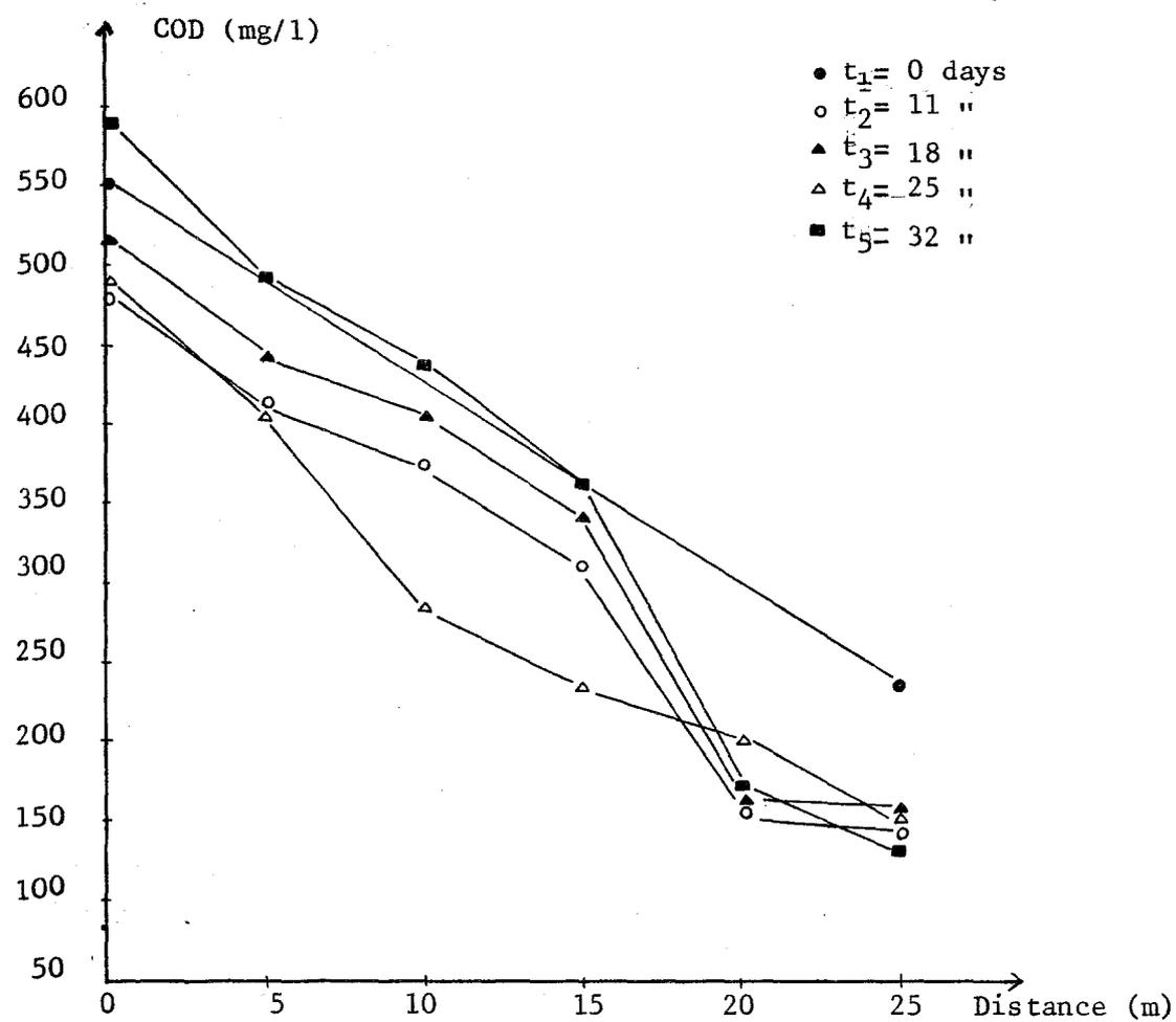
Figure 21 : Graphical Presentation Showing the Variation of COD with Distance in the Channel Full with Sand
