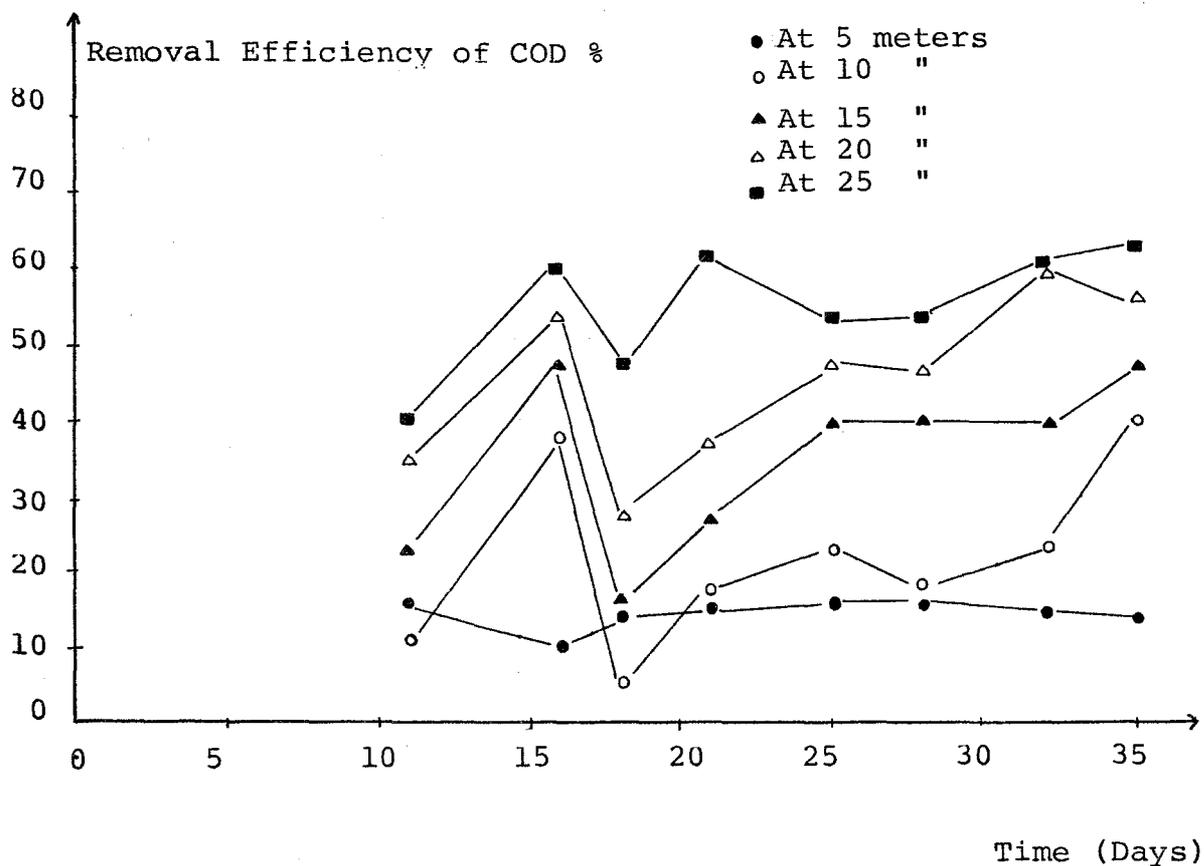
Figure 23 : Graphical Presentation Showing the Removal Efficiency of COD with Time in the Channel Full with Gravel
