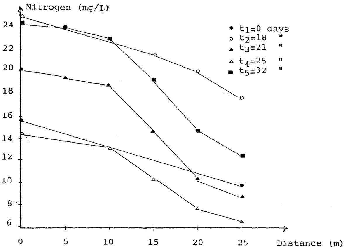
Figure 34 : Graphical Presentation Showing the Variation of Nitrogen with Distance in the Channel Full with Gravel
