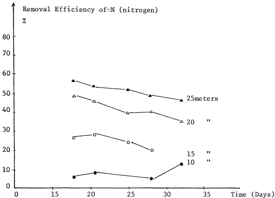
Figure 31 : Graphical Presentation of the Removal Efficiency of Nitrogen with Time in the Channel Full with Gravel
