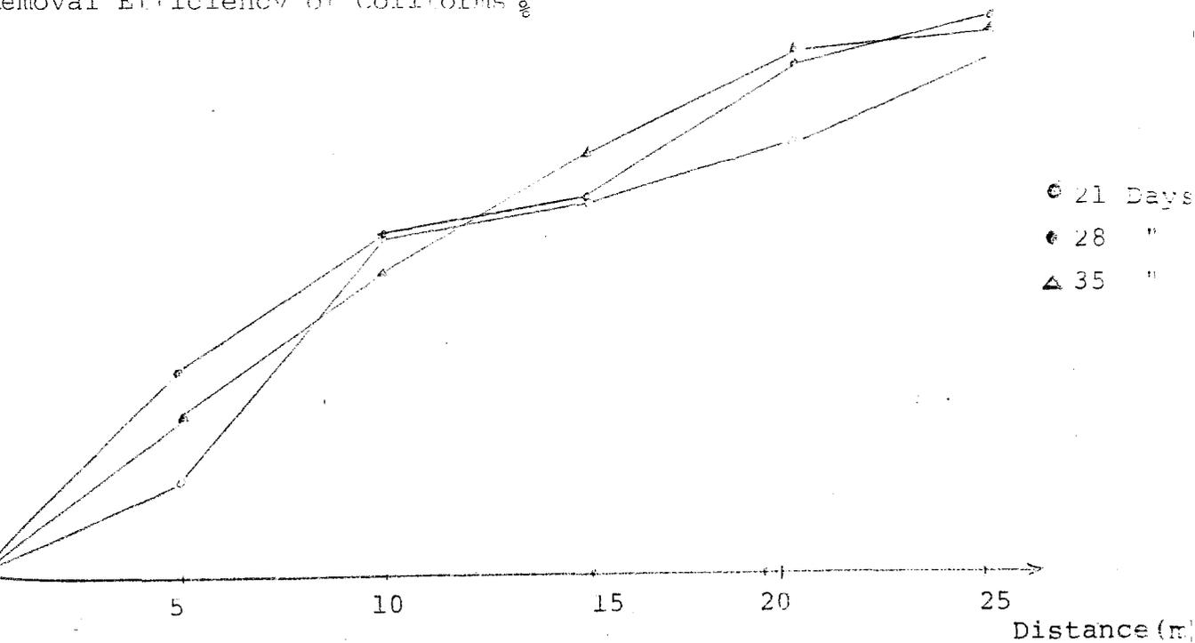
Figure 58 : Removal Efficiency of Coliform with Distance in Sand Bed
