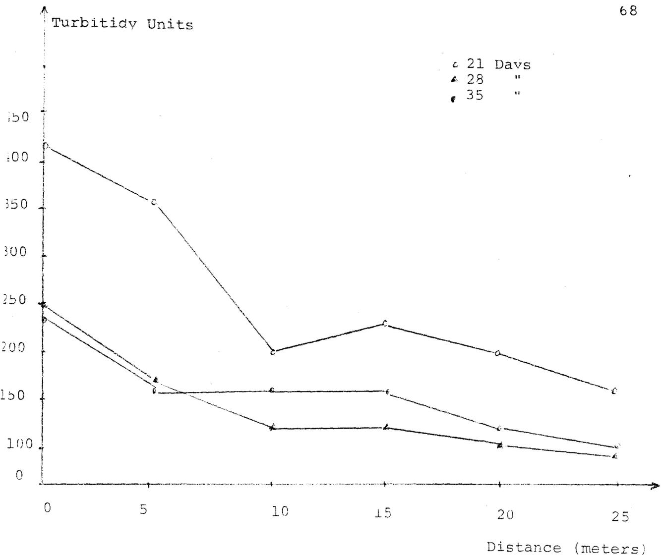
Figure 52 : Variation of Turbidity with Distance in the Channel Full with Gravel
