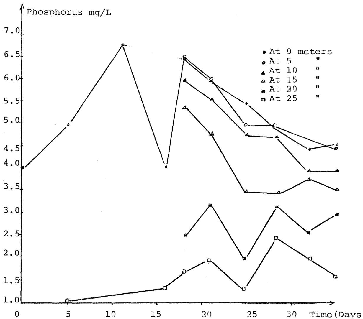
Figure 38 : Variation of Phosphorus with Time in the Channel Full with Sand
