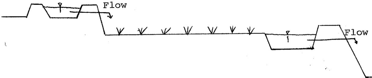
Figure 1 : Surface Irrigation
