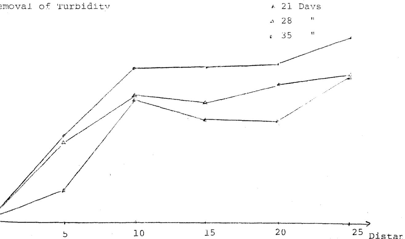
Figure 49 : Removal Efficiency of Turbidity with Distance in the Channel Full with Sand
