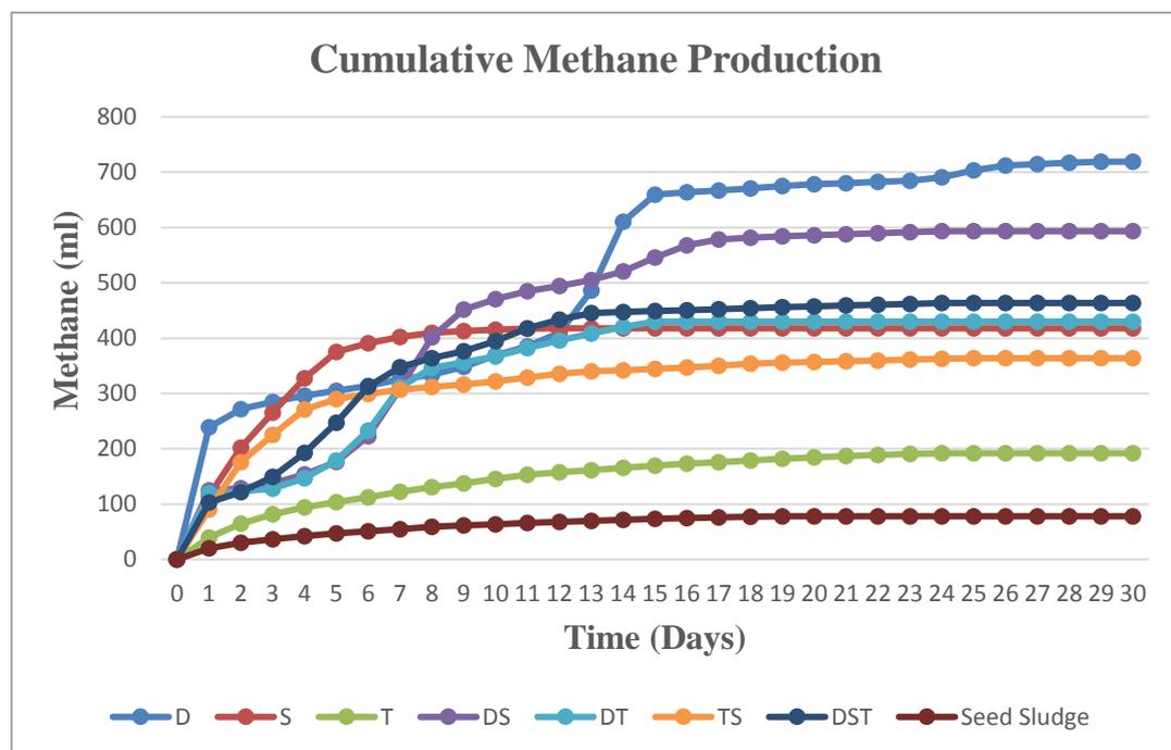
Figure 4.3. The cumulative methane productions during anaerobic digestion and co-digestion.
