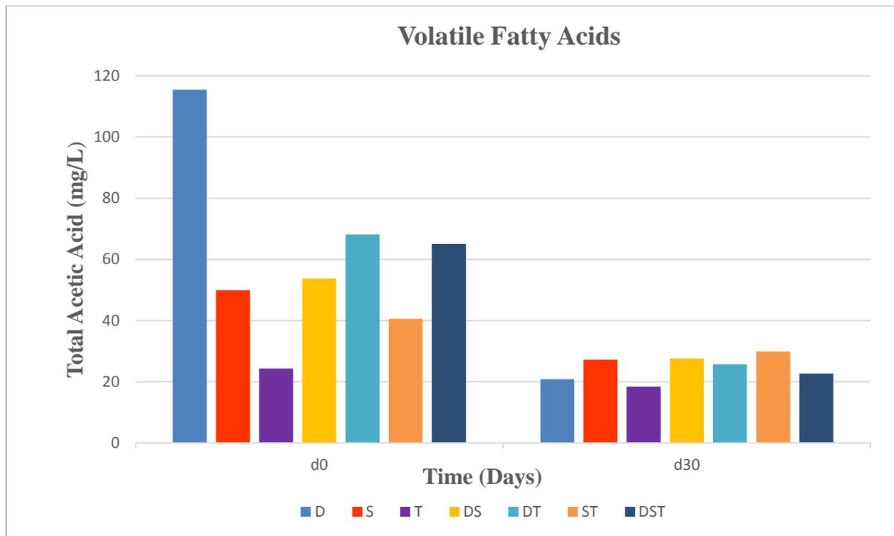
Figure 4.2. Results of VFA concentrations of the anaerobic digesters during digestion and co-digestion.
