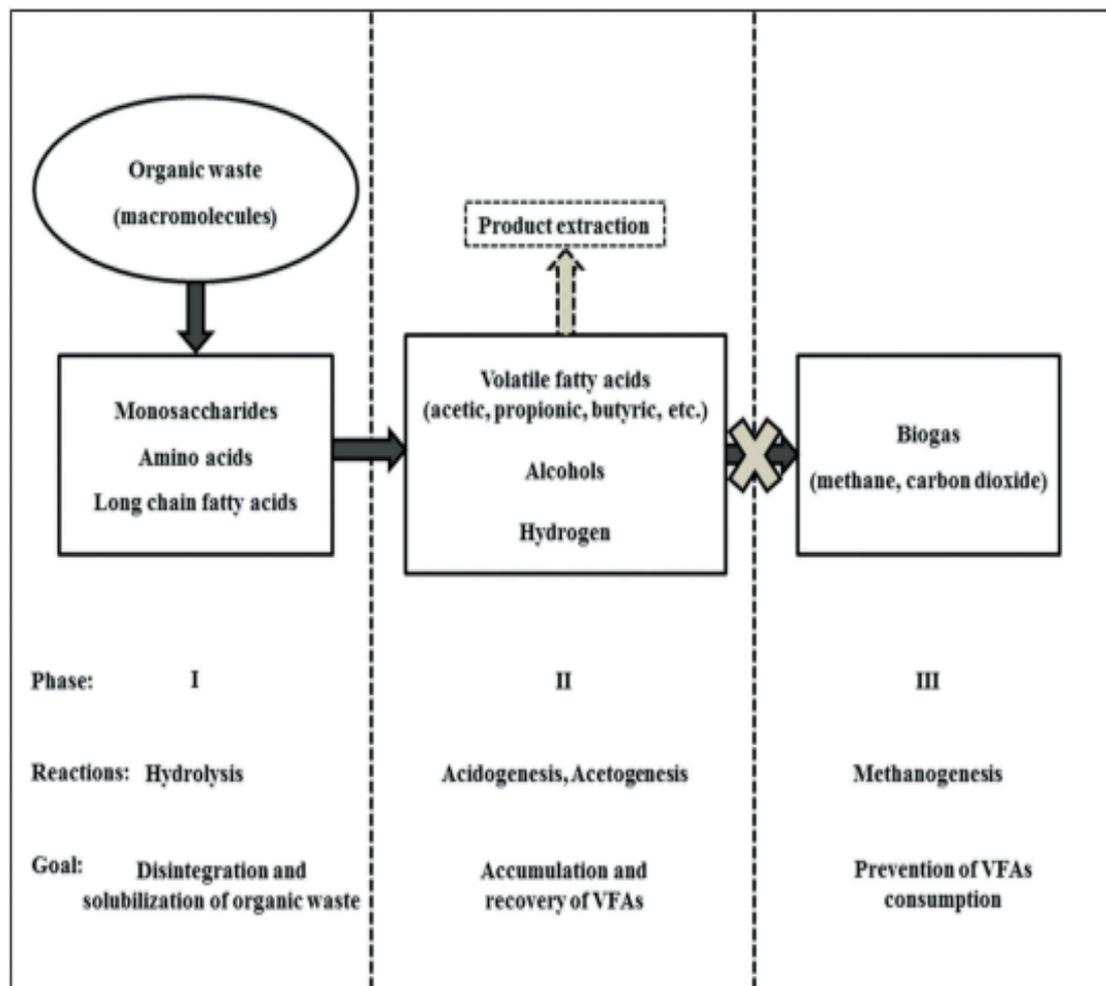
Figure 2.5. Formation of volatile fatty acids during anaerobic digestion (Wainaina et al., 2019).
