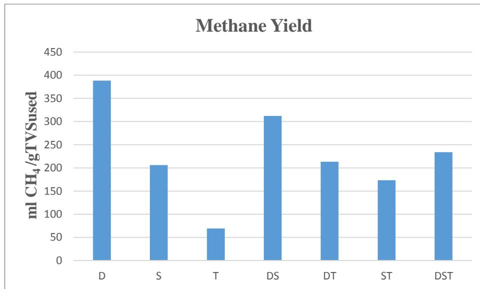
Figure 4.4. The calculated methane yields of the BMP digesters as per gram volatile solids added (CH<sub>4</sub>/g TVS<sub>used</sub>).
