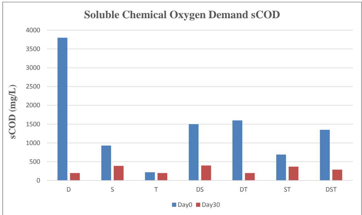
Figure 4.1. sCOD concentrations in all digesters with the digestion time.
