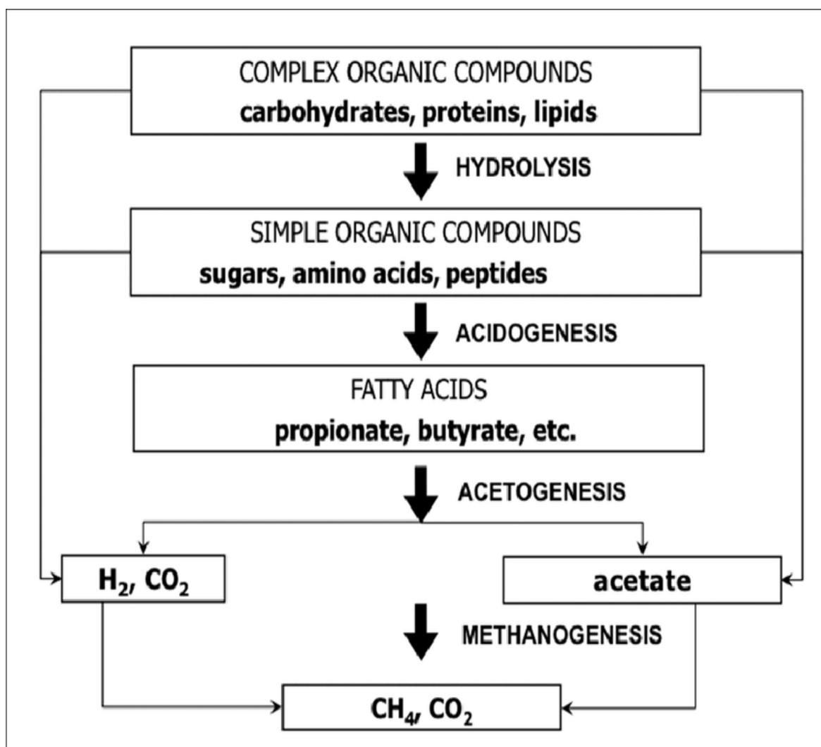
Figure 2.2. Four steps involved in the anaerobic digestion process (Drosg, 2013).
