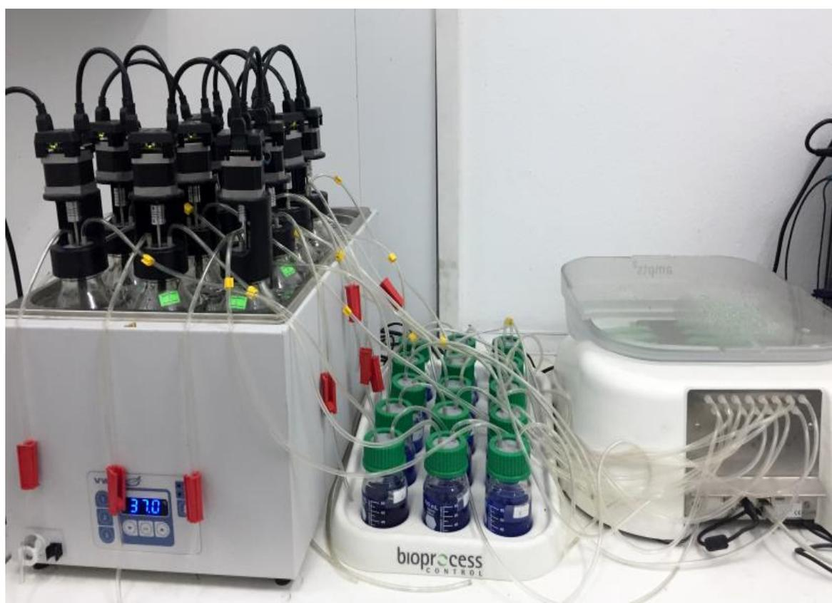
Figure 3.2. The Automated Methane Potential Test System II (AMPTS II).
