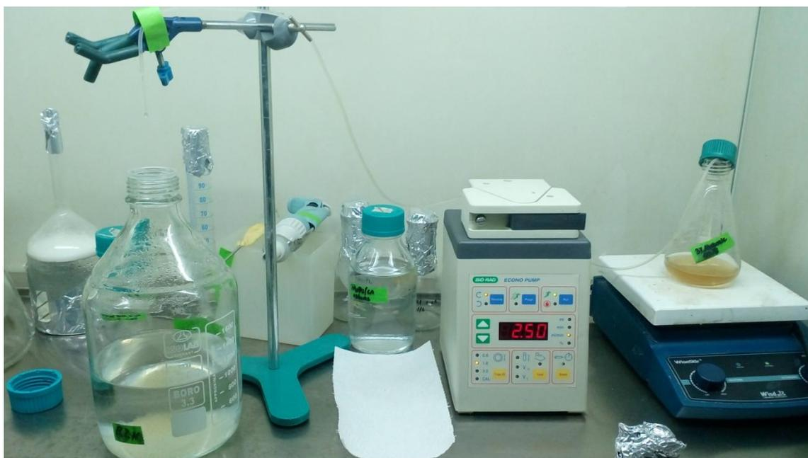
Figure 3.3. Ca-alginate bead preparation setup
