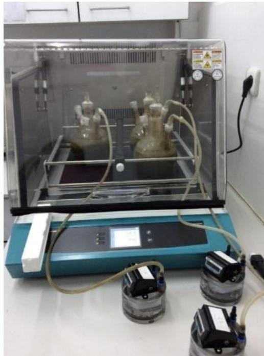
Figure 4.1. The anaerobic batch digesters in the incubator and Milli Gas Counters used in this study.
