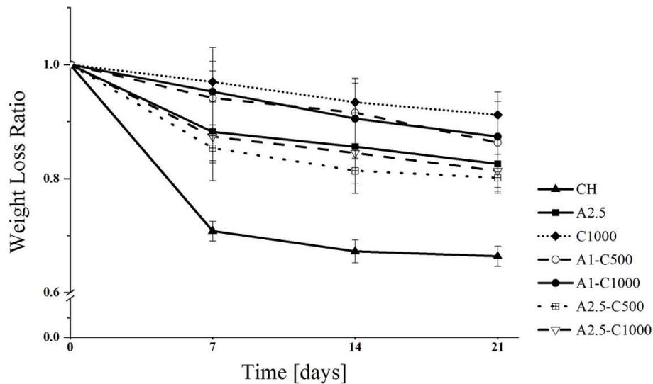
**Figure 4.17** Lysozyme-induced enzymatic degradation (CH: Chitosan, A2.5: 2.5 mg/mL Amp, C1000:  $1000\mu\text{M}$  CAPE, A1-C500: 1 mg/mL Amp +  $500\mu\text{M}$  CAPE, A1-C1000: 1 mg/mL Amp +  $1000\mu\text{M}$  CAPE, A2.5-C500: 2.5 mg/mL Amp +  $500\mu\text{M}$  CAPE, A2.5-C1000: 2.5 mg/mL Amp +  $1000\mu\text{M}$  CAPE).
