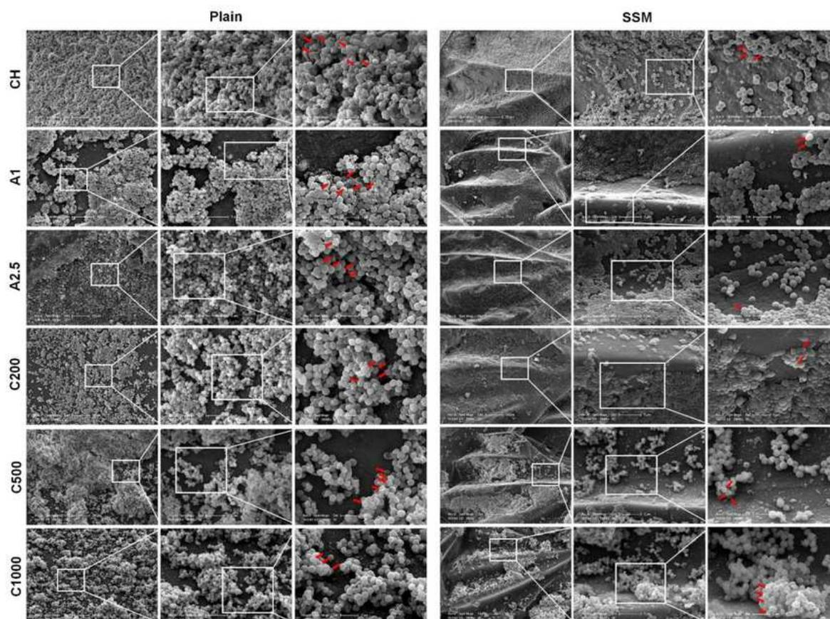
**Figure 4.11** SEM images of *S. aureus* growth on plain and SSM CH membranes after 24 h incubation at 37°C. Red arrows indicate layers of bacteria on the surface of the membranes. Scale bars: 20  $\mu\text{m}$ , 5  $\mu\text{m}$ , and 2  $\mu\text{m}$  (SSM: sharkskin mimicked, Amp: Ampicillin sodium salt, CAPE: Caffeic acid phenethyl ester, CH: Chitosan, A1: 1 mg/mL Amp, A2.5: 2.5 mg/mL Amp, C200: 200  $\mu\text{M}$  CAPE, C500: 500  $\mu\text{M}$  CAPE, C1000: 1000  $\mu\text{M}$  CAPE).
