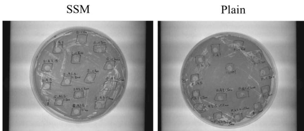
**Figure 4.9** Zone of inhibition of plain and SSM samples against *S. aureus* bacteria on TSA plate after 24 h incubation at 37°C.
