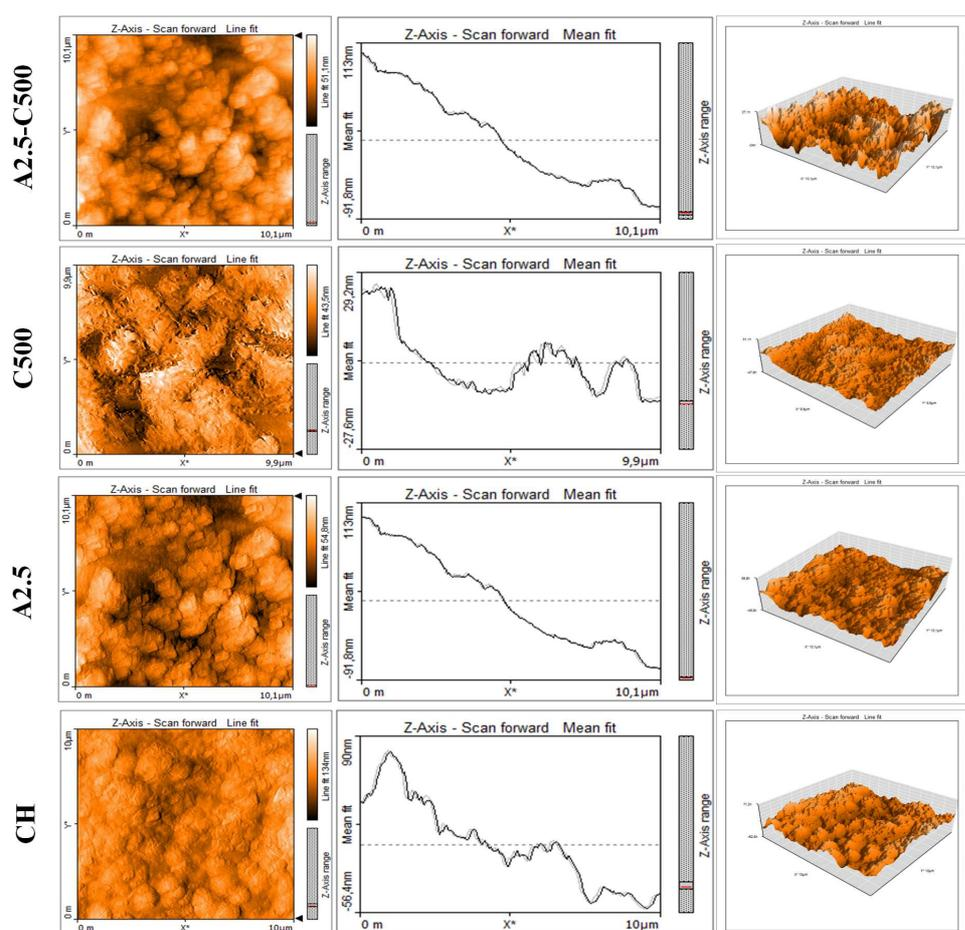
**Figure 4.6** AFM results ( $10\ \mu\text{m} \times 10\ \mu\text{m}$  scan area) of plain membranes (CH: chitosan, Amp: Ampicillin sodium salt, CAPE: Caffeic acid phenethyl ester, A2.5: 2.5 mg/mL Amp, C500: 500  $\mu\text{M}$  CAPE, A2.5-C500: 2.5 mg/mL Amp + 500  $\mu\text{M}$  CAPE).
