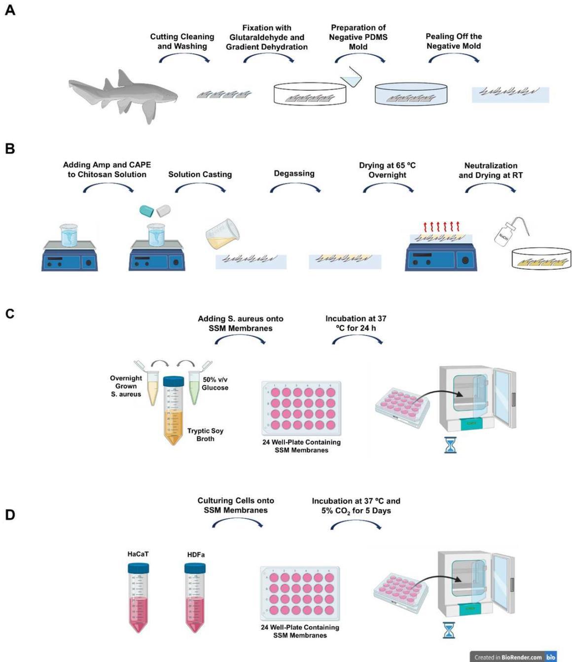
**Figure 4.1** Schematic representation of experimental procedures for SSM CH/Amp/CAPE membrane preparation. **A)** Sharkskin mimicked negative mold preparation, **B)** Amp-CAPE loaded CH membrane fabrication, **C)** Bacterial biofilm growth test, and **D)** HaCaT and HDFa cell culture experiments.
