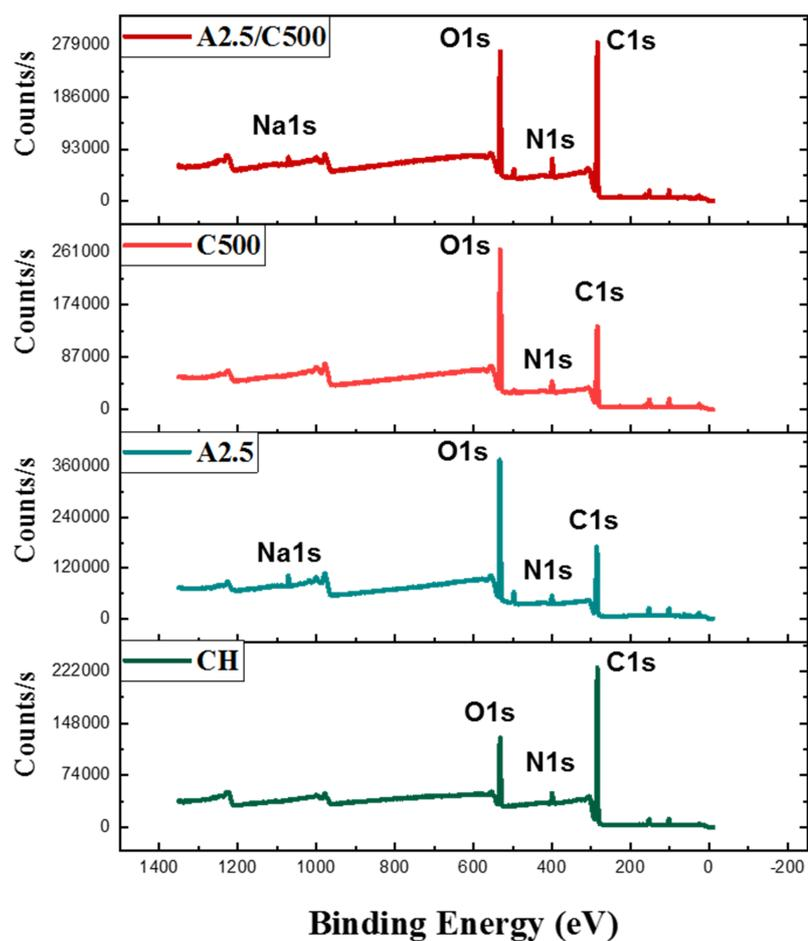
**Figure 4.4** XPS survey spectra (SSM: sharkskin mimicked, CH: chitosan, Amp: Ampicillin sodium salt, CAPE: Caffeic acid phenethyl ester, A2.5: 2.5 mg/mL Amp, C500: 500  $\mu$ M CAPE, A2.5-C500: 2.5 mg/mL Amp + 500  $\mu$ M CAPE).
