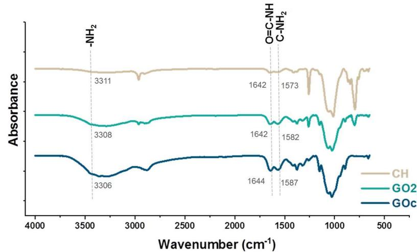
**Figure 3.2** FTIR spectra of CH, GO and GOc membranes (CH: chitosan, GO2: 0.2%wt graphene oxide/chitosan nanocomposite, GOc: graphene oxide coated chitosan).
