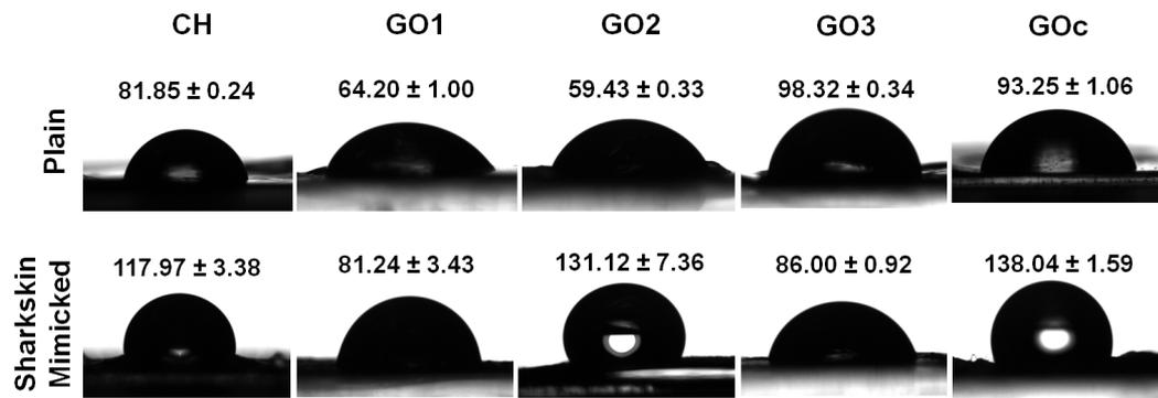
**Figure 3.3** Water contact angle results for plain and sharkskin mimicked membranes (Mean ± SD, n=5) (CH: chitosan, GO: graphene oxide, GO1, GO2, GO3: 0.1, 0.2, 0.3 %wt graphene oxide/chitosan nanocomposites, GOc: graphene oxide coated)
