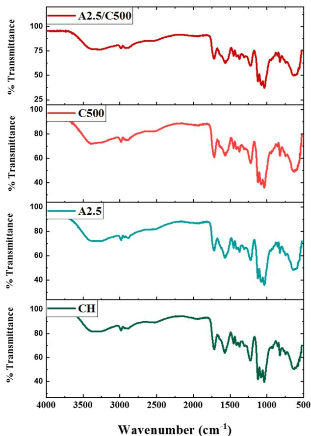
**Figure 4.5** FTIR spectra of CH, A 2.5, C500, and A2.5-C500 membranes (CH: chitosan, Amp: Ampicillin sodium salt, CAPE: Caffeic acid phenethyl ester, A2.5: 2.5 mg/mL Amp, C500: 500  $\mu$ M CAPE, A2.5-C500: 2.5 mg/mL Amp + 500  $\mu$ M CAPE)
