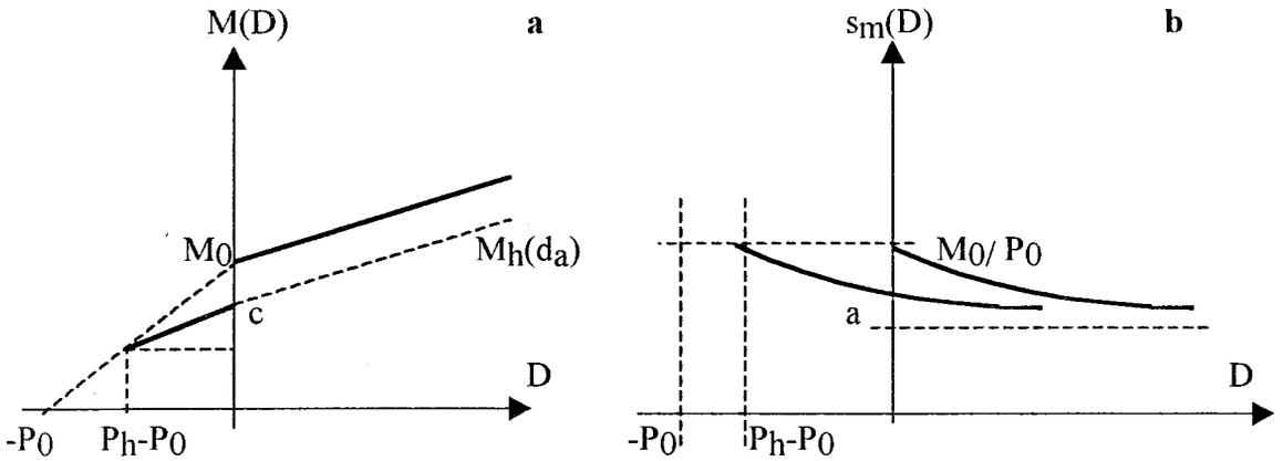
Figure 2.3. CRT algorithm. (a) CRT of  $M$  values. After intercepting  $Y$  axis at  $c$ ,  $M_h(d_a)$  line gives contradictory results (dashed).  $M_0$  corresponds to sea level permissible tension;  $c$  is the  $M$  value of for a depth of  $(P_0 - P_h)$  in altitude dives at  $P_h$ ; (b) critical ratios corresponding to CRT.
