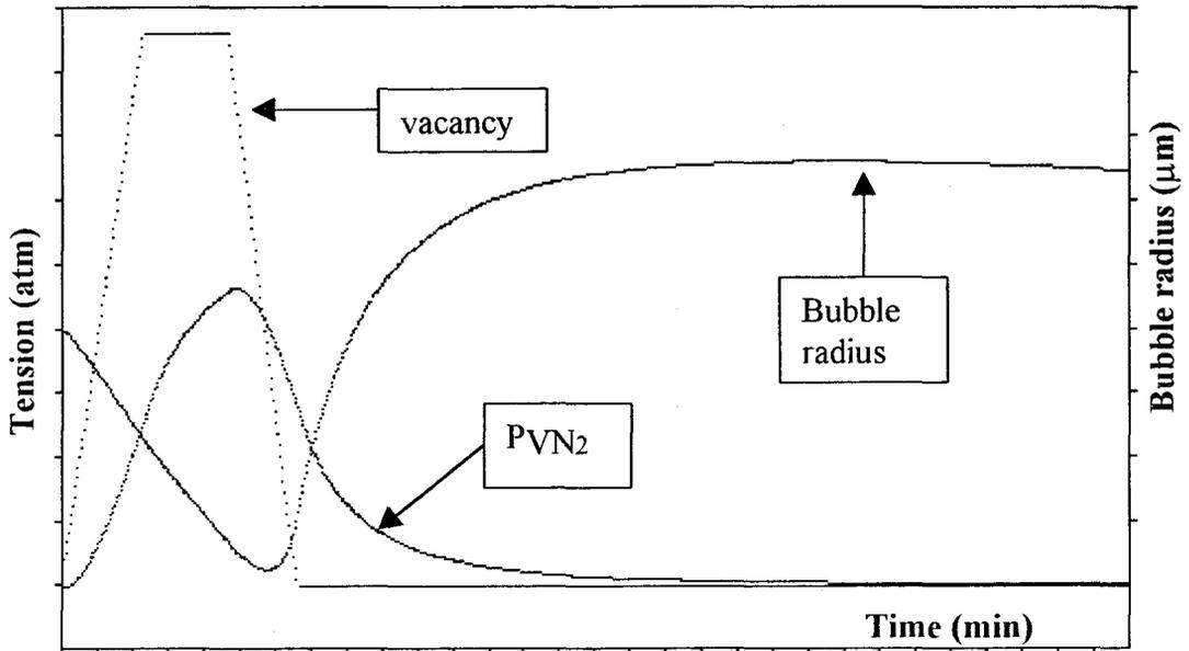
Figure 5.3. Simulation of a 42m/6 min dive at 3500 m. altitude. The ascent time = 2.5 min. Vertical axis scale = 0.484 atm/division for the vacancy and tissue tension, 5 μm/div for the bubble radius. Time axis scale = 1.283 min/div. At 30<sup>th</sup> min following surfacing the bubble radius is almost stable (38 μm).
