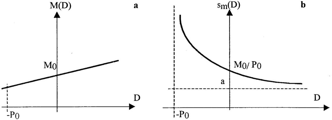
Figure 2.2. LEM algorithm. When linearly extrapolated (a),  $M$  values still give a positive tolerable tension at ideal vacuum ( $-P_0$ ). This corresponds to an infinite tolerable supersaturation ratio at vacuum (b).
