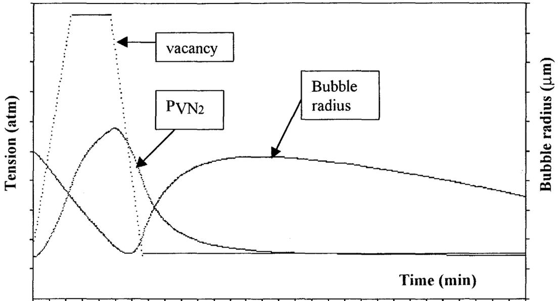
Figure 5.1. Simulation of a 42m/6 min dive at sea level. The ascent time = 2.5 min. Vertical axis scale = 0.5 atm/division for the vacancy and tissue tension, 5  $\mu\text{m}/\text{div}$  for the bubble radius. Horizontal axis represents the time (1.283 min/div). At 30<sup>th</sup> min following surfacing the bubble radius drops to 17  $\mu\text{m}$ .
