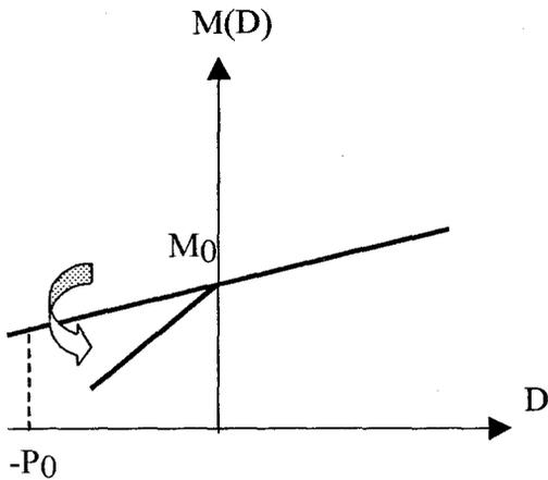
Figure 2.8. Change in the slope of  $M(D)$  function as bottom time is increased. The safety factor of assuming that all tissues are sea level equilibrated for an altitude-equilibrated diver is equivalent to introducing a new set of  $M$  values.
