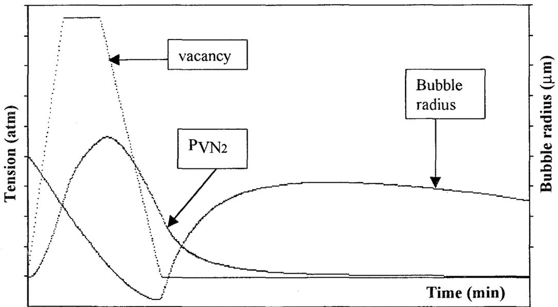
Figure 5.4. Simulation of a 42m/6 min dive at 3500 m. altitude. The ascent time = 5 min. The vertical axis scales are the same as in Figure 5.3. Time axis scale = 1.366 min/div. At 30<sup>th</sup> min following surfacing the bubble radius drops to 17 μm.
