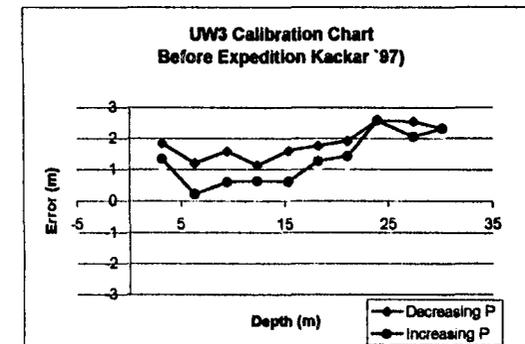
Figure 10.2. Validation of depth gauges before Kaçkar '97
