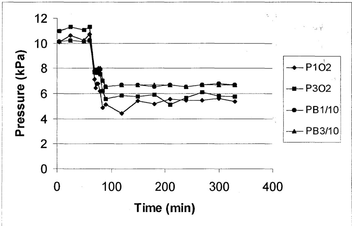
Figure 7.4. The chamber ambient pressure and partial pressure of end expiratory  $O_2$ . The  $P_{O_2}$  level of pig1 decreases significantly down to 4.44 kPa 30 min following the ascent but gradually recovers.
