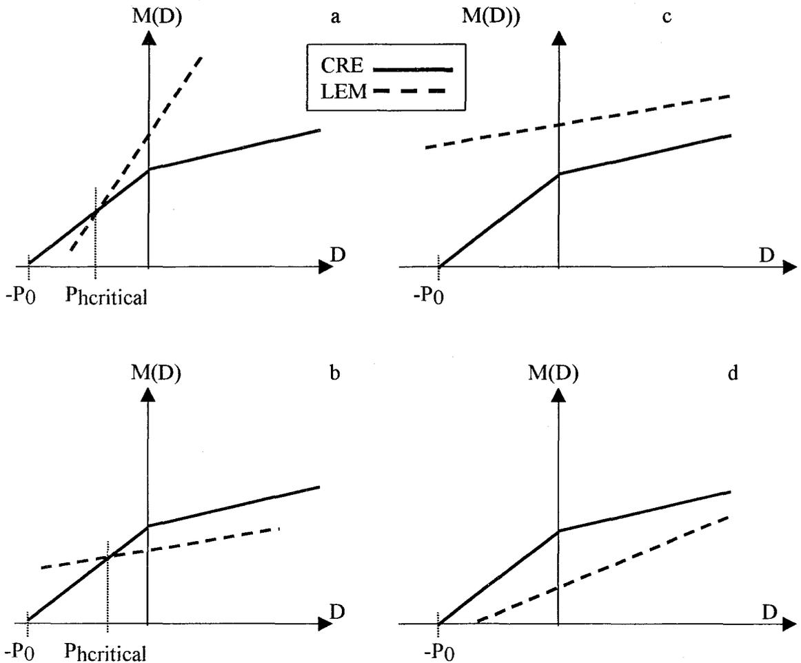
Figure 2.7. Possible combinations of CRE and LEM algorithms applied to M values of two different models. LEM is more conservative for all ambient pressures lower than  $P_{critical}$  (a), higher than  $P_{critical}$  (b), for all altitudes (d); in c CRE is always more conservative.
