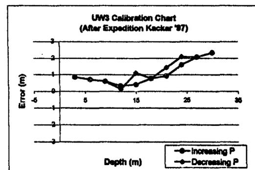
Figure 10.3. Validation of depth gauges after Kaçkar '97
