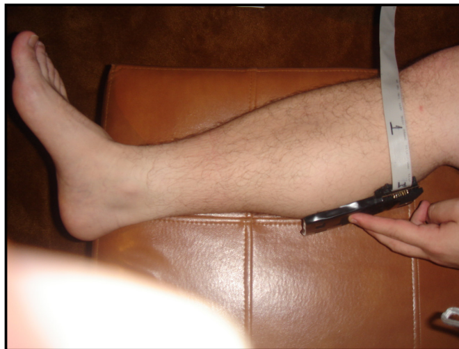
Figure 4.2 – The placement of the Niroxcope 301 probe on the gastrocnemius.
