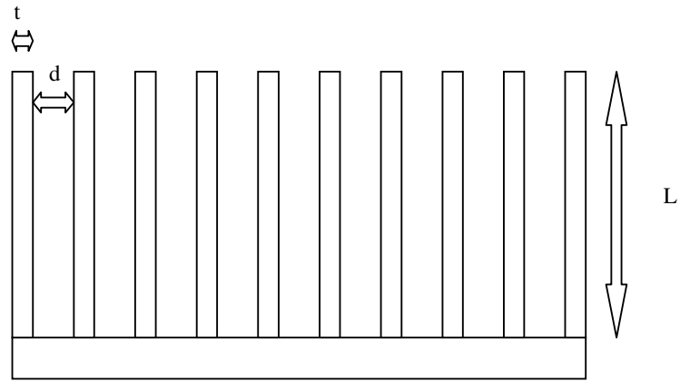
Figure 2.5 Parallel Hole Collimator where t is the septal thickness, d is the hole size, and L is the hole length
