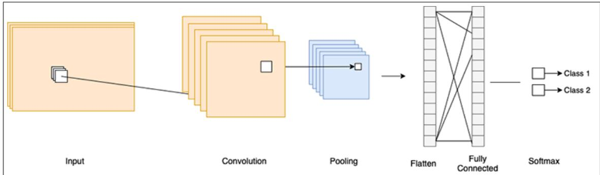
**Figure 2.5** CNN Architecture.
