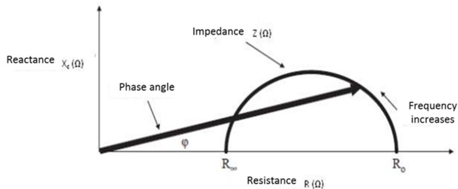
**Figure 2.7** Relationship Between Phase Angle, Resistance, Reactance, Impedance, and Applied Current Frequency [45].
