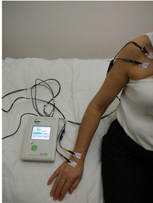
**Figure 3.2** Placement of Electrodes and The BIS Device.
