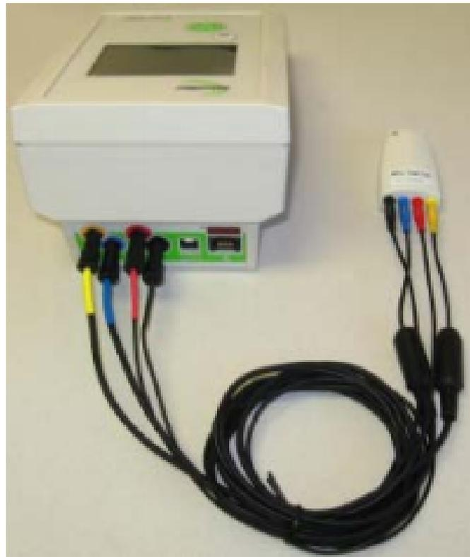
**Figure 3.1** Impedimed Multifrequency Analyzer (IMA) (Model SFB7) with Test Cell. [52]
