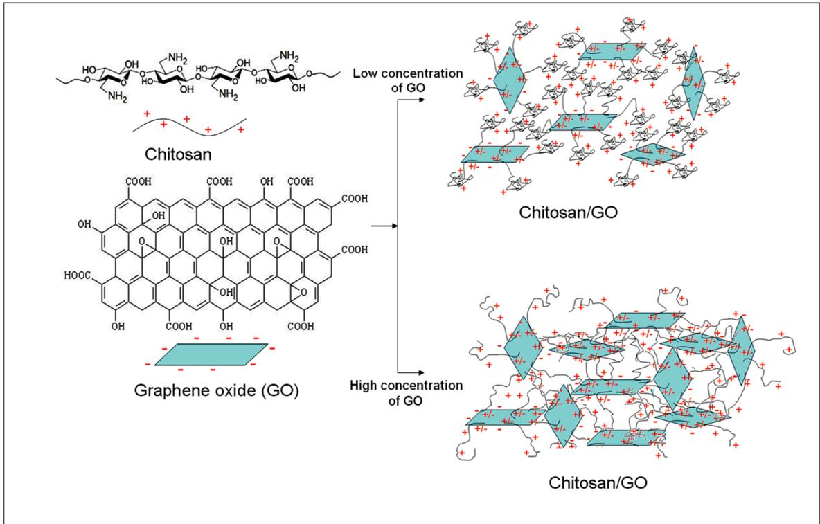
**Figure 3.4** Schematic illustration of dispersion of GO sheets in chitosan solution [19].
