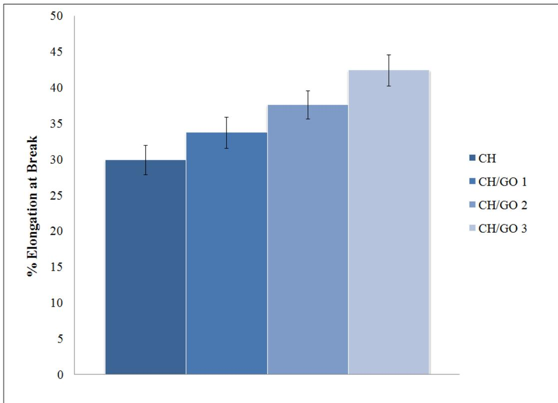
**Figure 4.13** Elongation at Break (%) of Plain Membranes. Data are expressed in means  $\pm$  SE.
