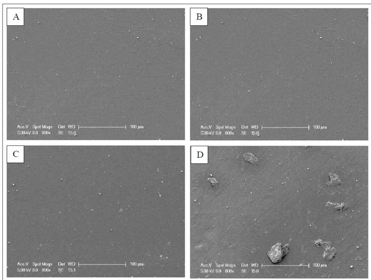
**Figure 4.8** Surface Images of CH Based Membranes at 800x Magnification: A) Plain Pristine CH, B) Plain CH/GO1, C) Plain CH/GO2 and D) Plain CH/GO3.
