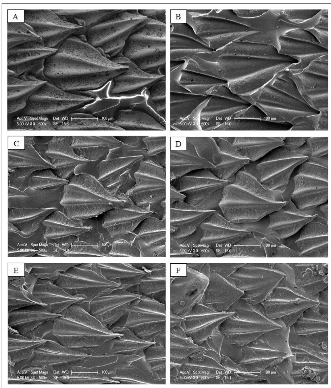
**Figure 4.3** Sharkskin, PDMS Negative Mould and Sharkskin Mimicked CH Based Membranes at 500x Magnification: A) Sharkskin, B) Negative, PDMS mold, C) Sharkskin Mimicked CH, D) Sharkskin Mimicked CH/GO1, E) Sharkskin Mimicked CH/GO2, F) Sharkskin Mimicked CH/GO3.
