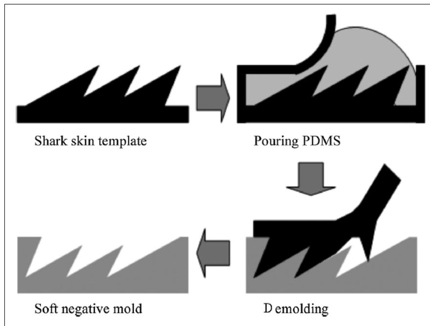
**Figure 2.2** Schematic Illustration of Sharkskin Replication Using Micro-Molding Method [2].
