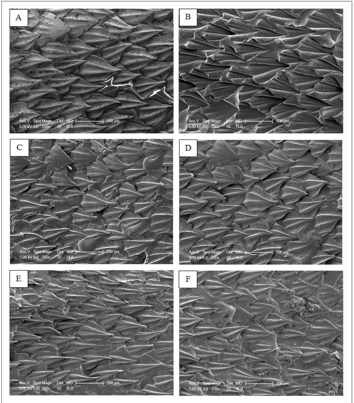
**Figure 4.2** Sharkskin, PDMS Negative Mould and Sharkskin Mimicked CH Based Membranes at 250x Magnification: A) Sharkskin, B) Negative PDMS mold, C) Sharkskin Mimicked CH, D) Sharkskin Mimicked CH/GO1, E) Sharkskin Mimicked CH/GO2, F) Sharkskin Mimicked CH/GO3.
