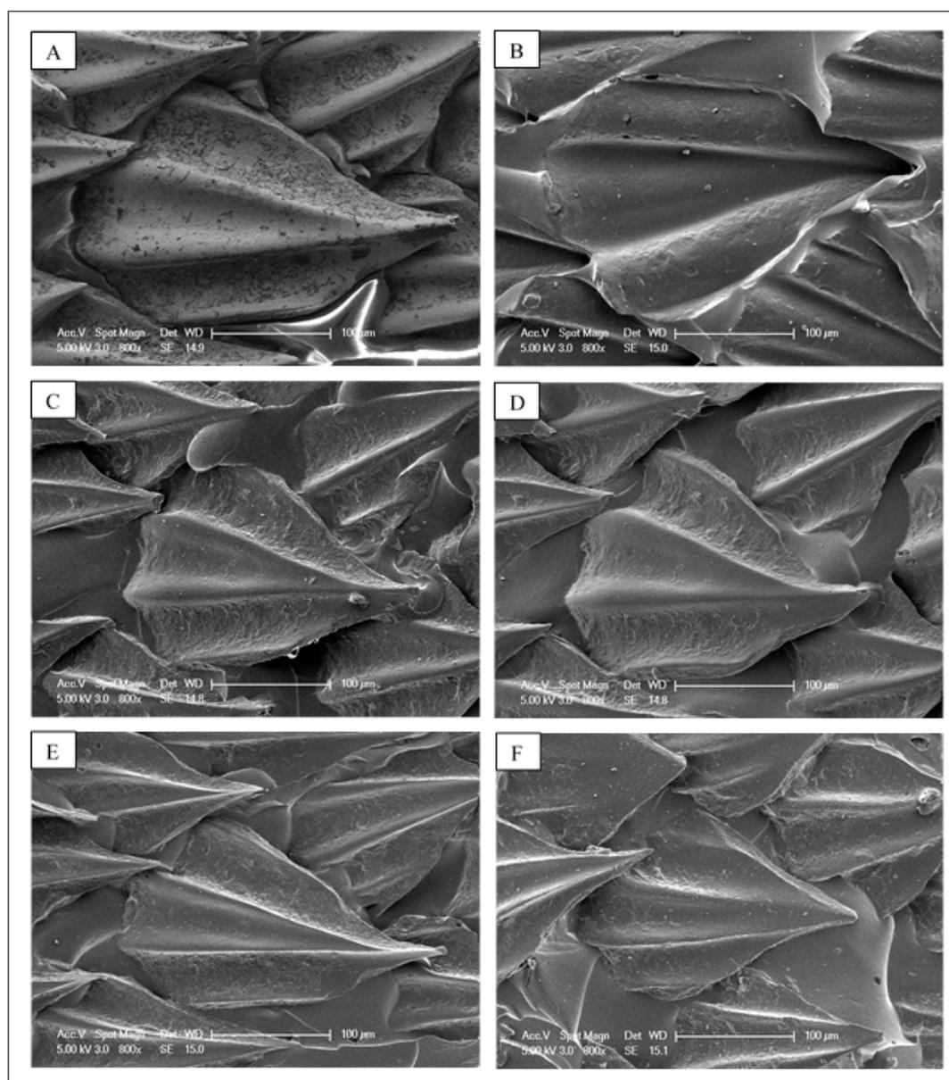
**Figure 4.4** Sharkskin, PDMS Negative Mould and Sharkskin Mimicked CH Based Membranes at 800x Magnification: A) Sharkskin, B) Negative PDMS mold, C) Sharkskin Mimicked CH, D) Sharkskin Mimicked CH/GO1, E) Sharkskin Mimicked CH/GO2, F) Sharkskin Mimicked CH/GO3.
