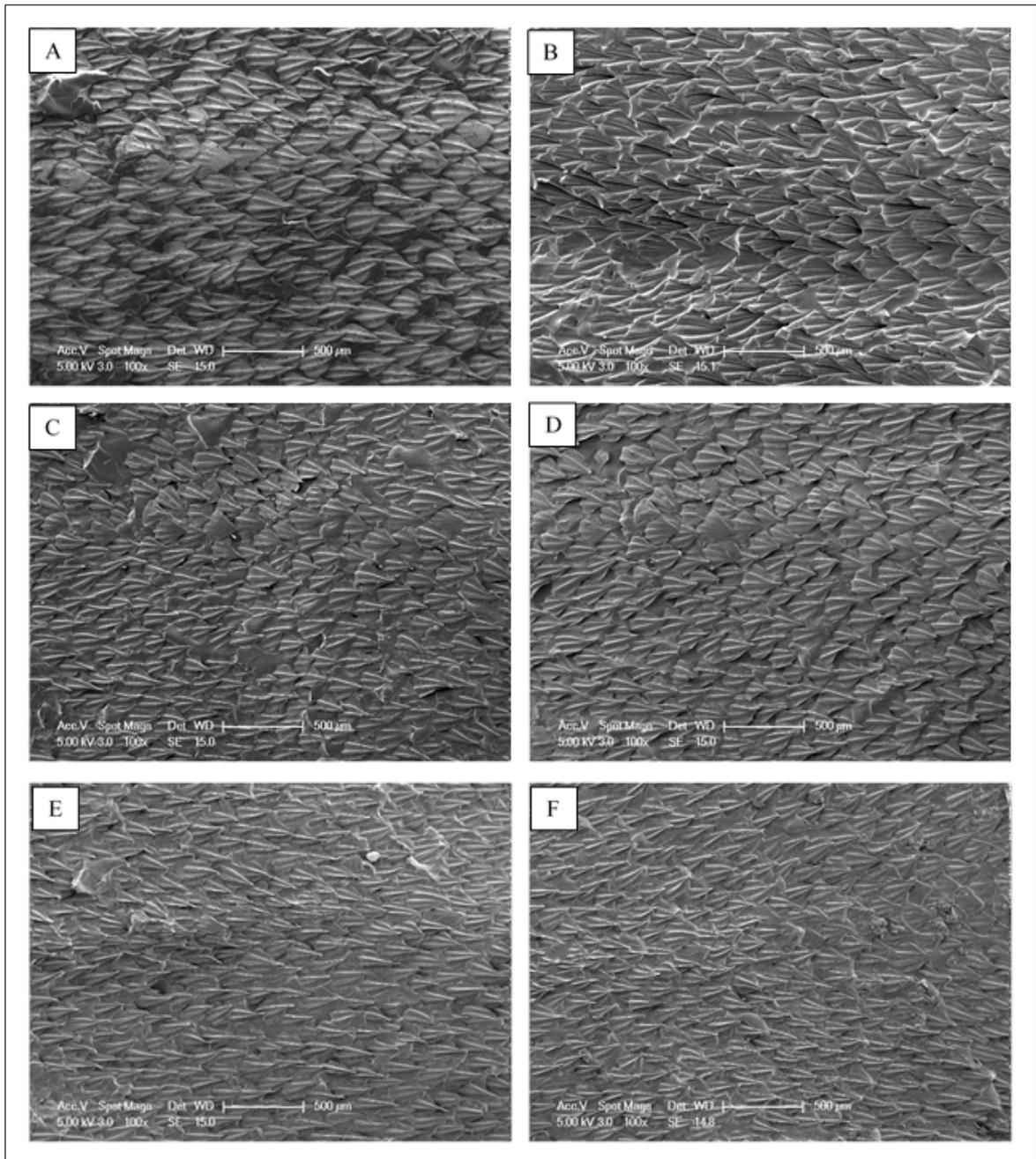
**Figure 4.1** Sharkskin, PDMS Negative Mould and Sharkskin Mimicked CH Based Membranes at 100x Magnification: A) Sharkskin, B) Negative PDMS mold, C) Sharkskin Mimicked CH, D) Sharkskin Mimicked CH/GO1, E) Sharkskin Mimicked CH/GO2, F) Sharkskin Mimicked CH/GO3.
