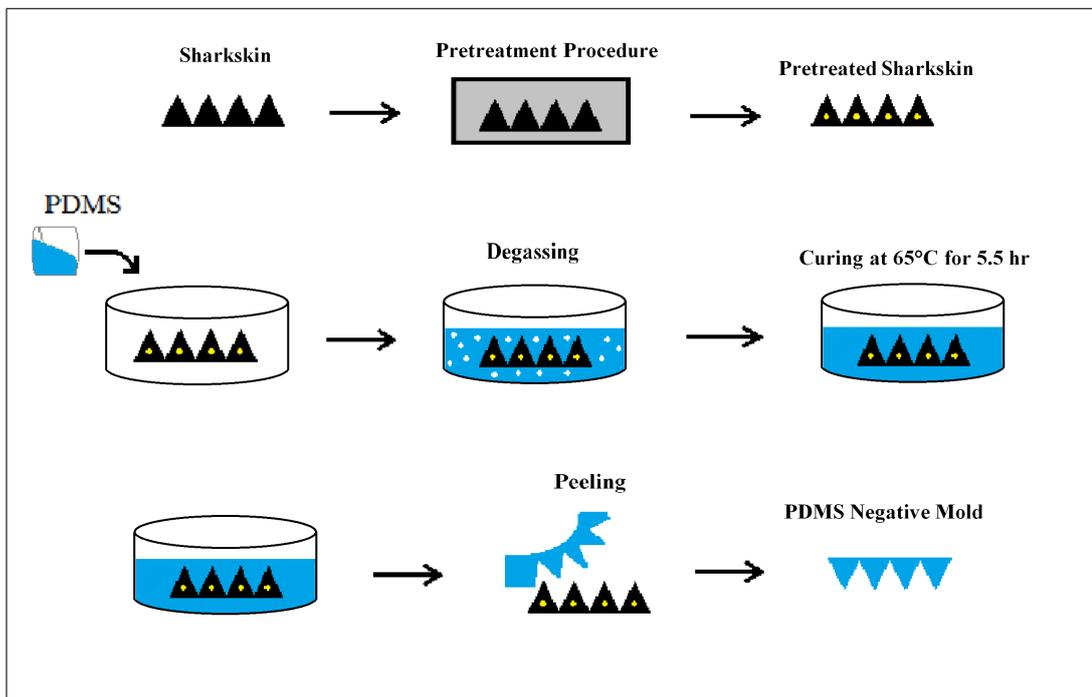
**Figure 3.2** Schematic Illustration of PDMS Mold Preparation Steps.
