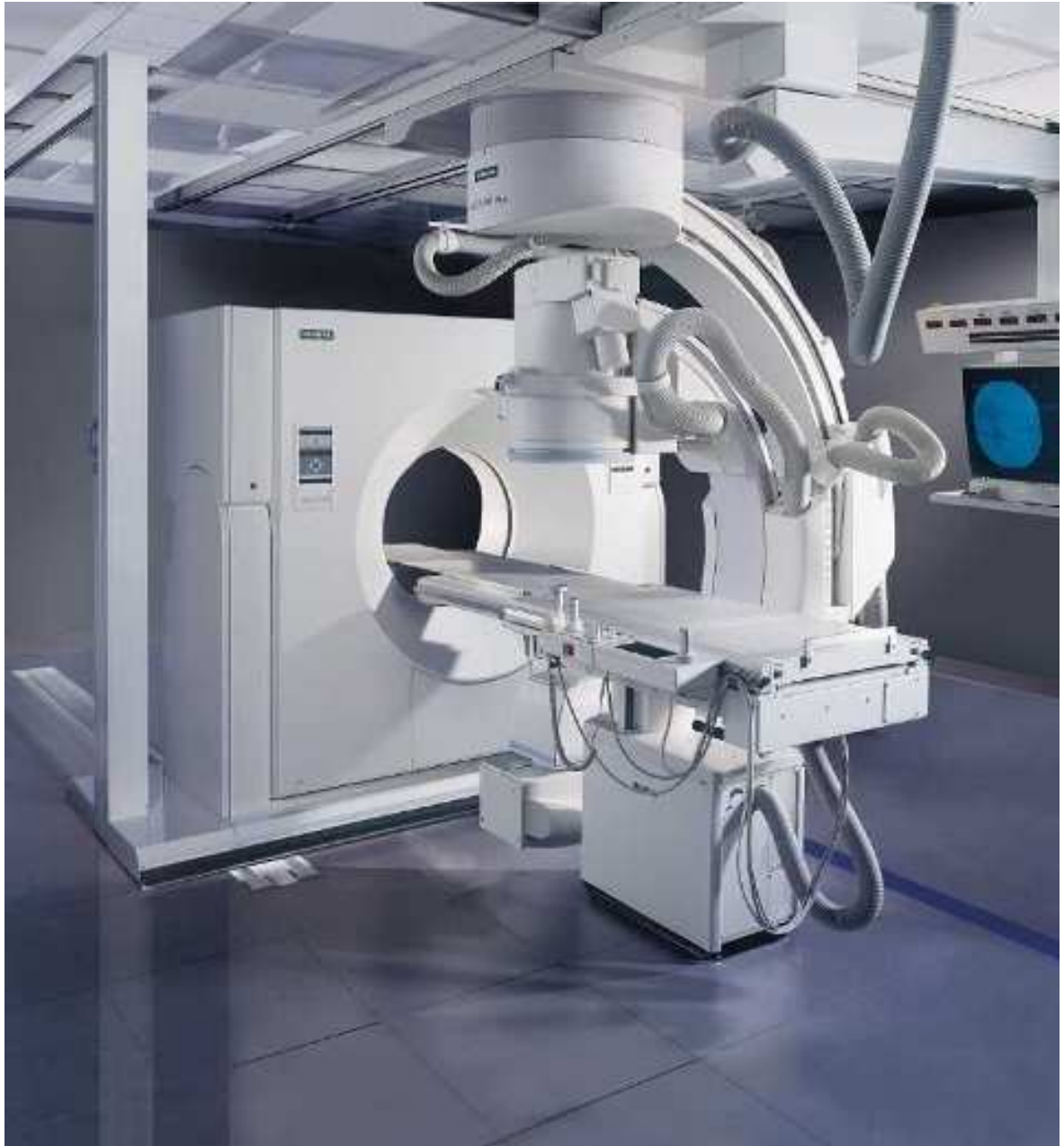
Figure 1.1 Combination of a 16 slice CT, and X-ray Fluoroscopy. Advantage of CT on acquisition of cross-sectional images of the body which could be combined to give the 3D volume, and practical use of XF combined together. [10]
