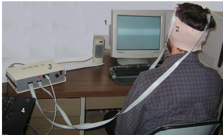
Figure 6.1 A photograph of the experimental setup. In the figure, the computer numbered as 1 was used as a patient computer for Stroop task, number 2 is 16-channel Niroxcope Probe, number 3 is Control Box and number 4 is the computer for real-time monitoring and storing the data.
