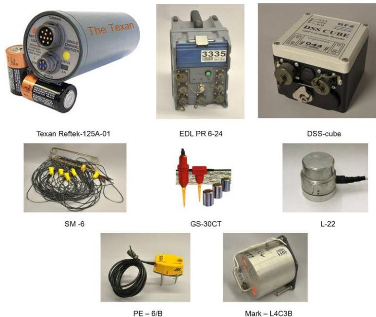
Figure 4.2. Seismic recorders (top), vertical component sensors (middle) and three component sensors (bottom).
