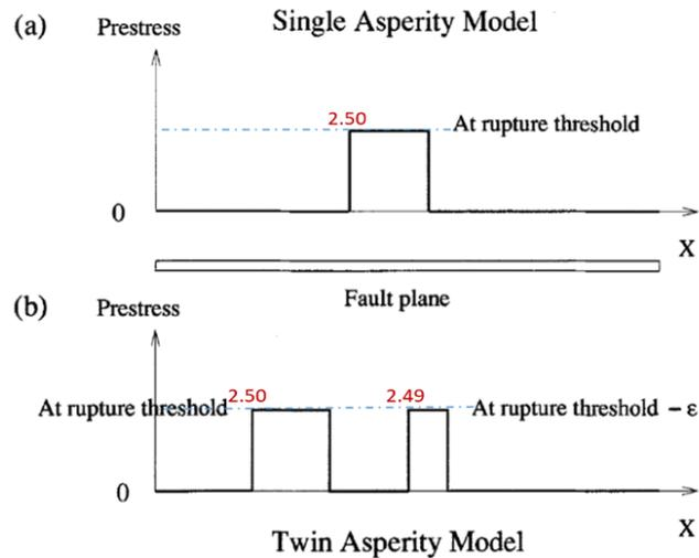
Figure 4.4. Initial stress states for the numerical simulations which are given in the paper. (a) One asperity model. (b) Two asperity model. The stress is zero outside of the asperities (Cochard and Madariaga, 1994).
