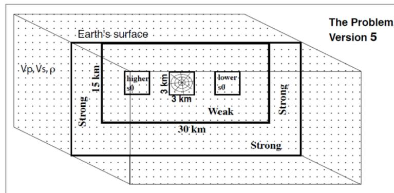
Figure 6.1. Definition of SCEC TPV5 and TPV205 geometry.
