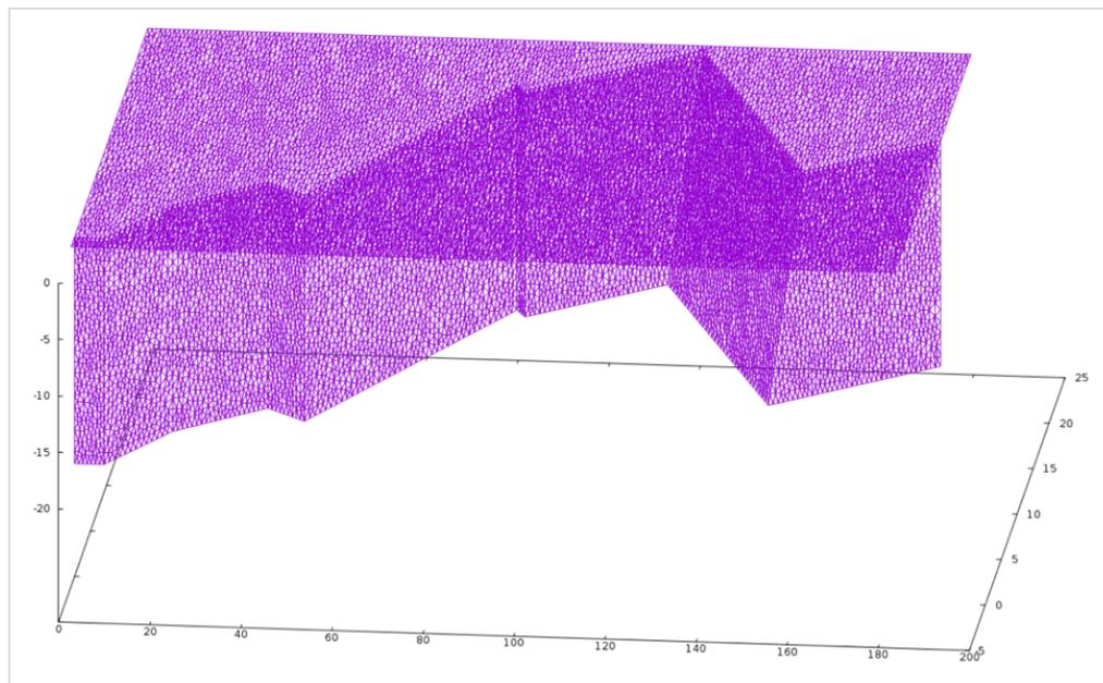
Figure 4.17. The fault geometry based on the model of Oglesby and Mai (2012), grid size is 1 km, the number of triangular elements is 21608, and required memory for the solution of the stress kernels is 4TB.
