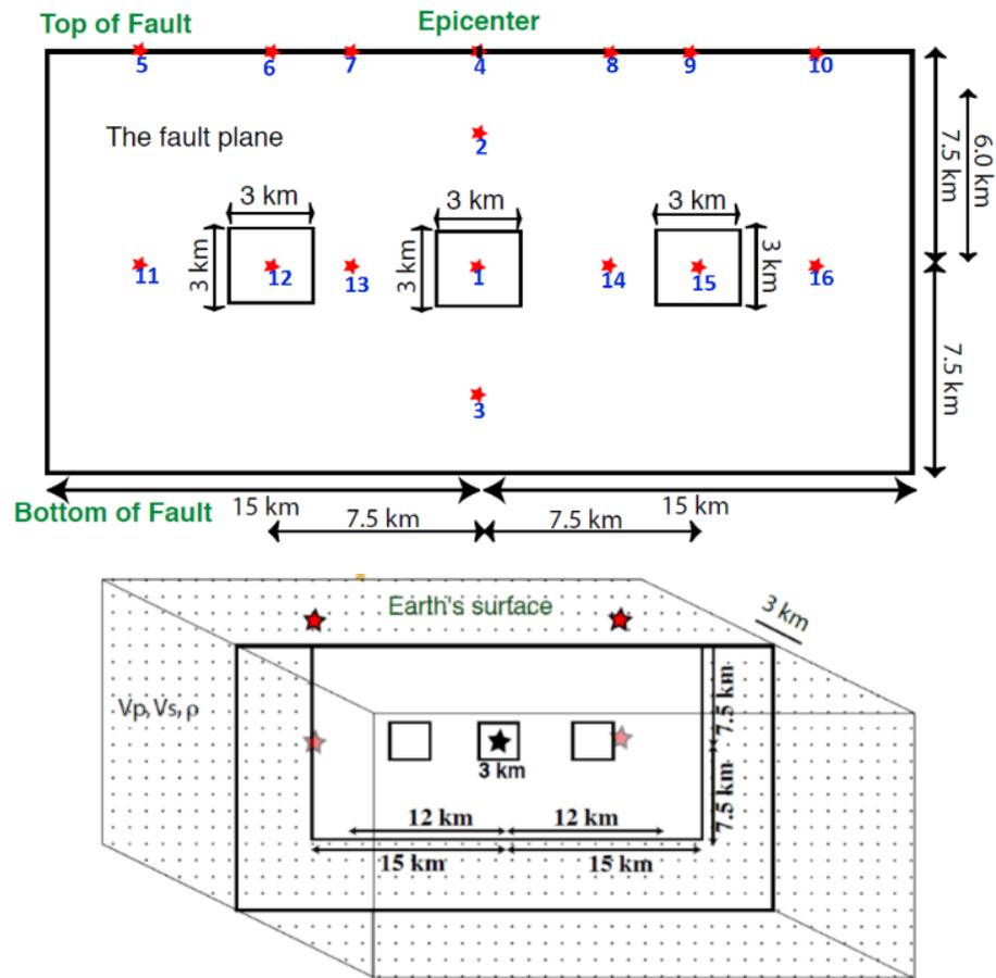
Figure 6.2. Positions of on-fault (top) and off-fault (bottom) observation points.
