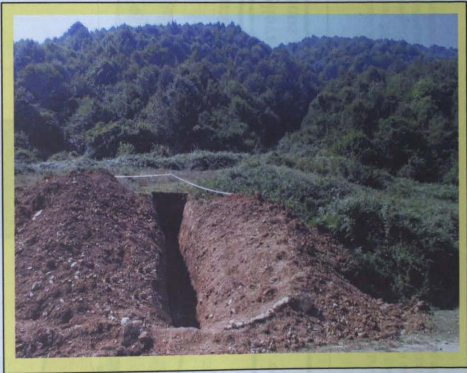
**Figure 55.** The picture of the Töngelli-1 trench (looking from north). Alluvial cone of the Töngelli stream was excavated perpendicular to the surface rupture of the 1999 Düzce earthquake. See figure 46 for the location of the trench.
