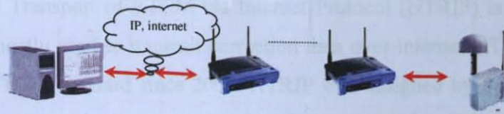
Figure 3.9. Setup schema of a wireless connection
