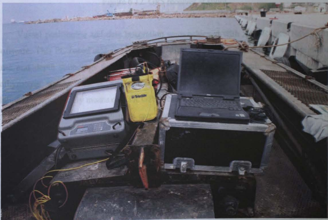
Figure 6.11. Survey system in survey boat
