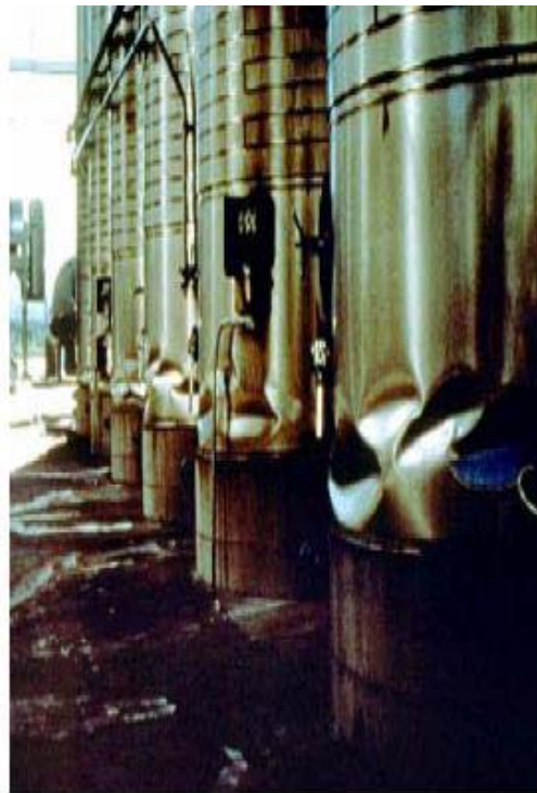
Figure 2.1. Diamond shape buckling developed at the wall of wine tanks
