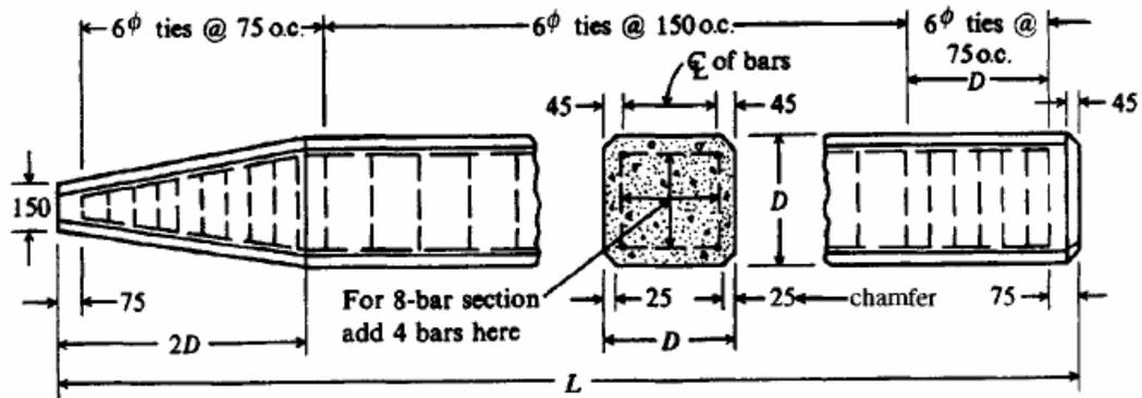
Figure 4.2. Precast concrete piles (Foundation analysis and design, 1997)
