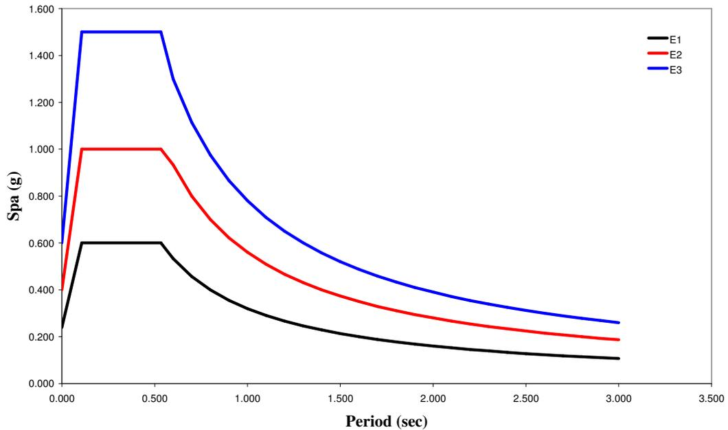
Figure 7.2. Design spectra used in this study
