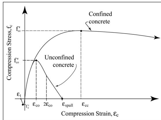
Figure 5.5. Stress-strain curves for confined and unconfined concrete
