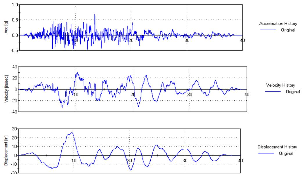
Figure A6 Acceleration-Velocity and Displacement History of Earthquake Record P0778
