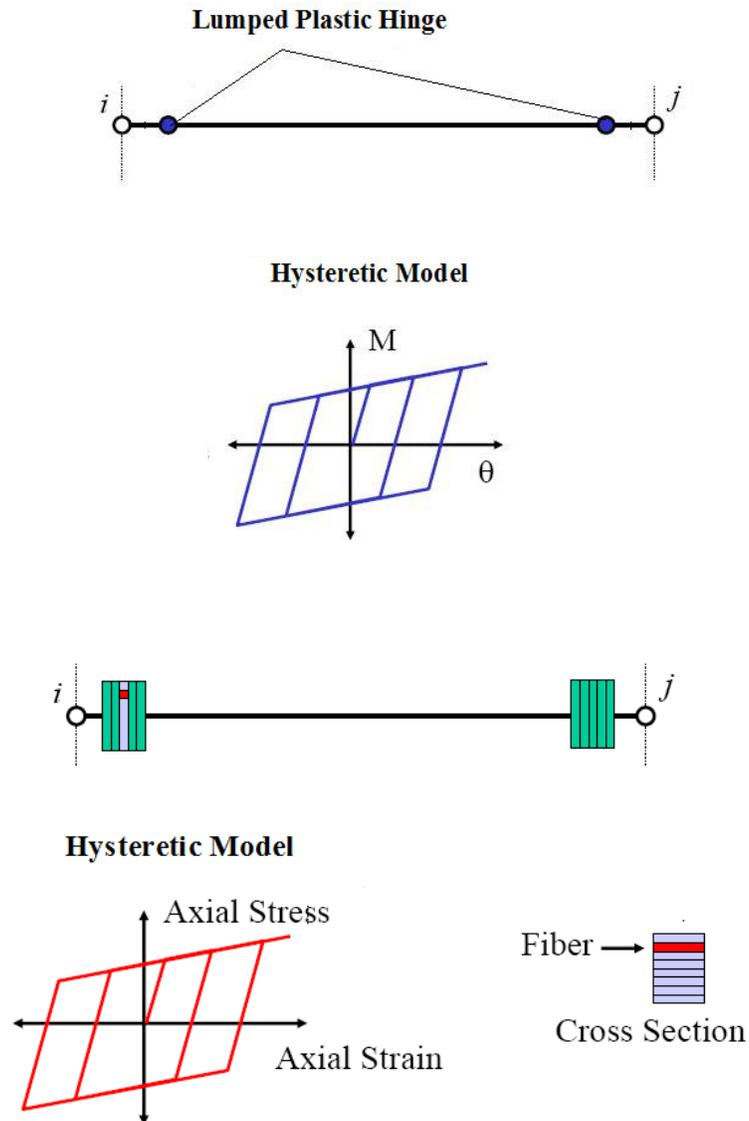
Figure 5.4. Lumped plastic hinge and fiber element model
