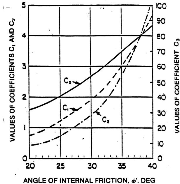
Figure 5.10. API coefficients for sand (API, 1994)
