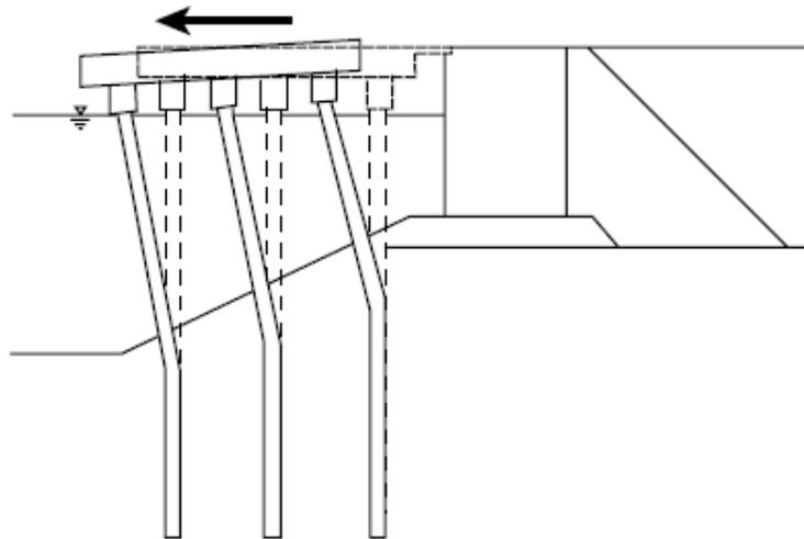
Figure 3.9. Damage due to inertia forces (Balkema, 2001)
