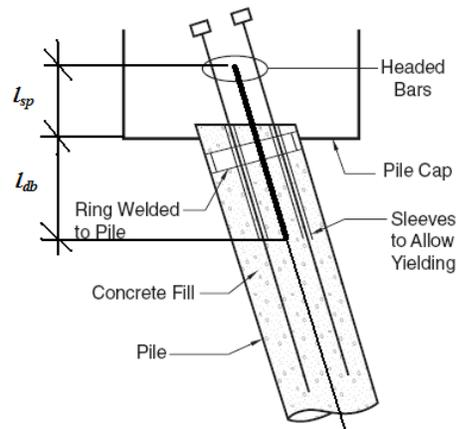
Figure 8.39. Tension fuse
