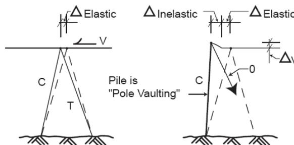
Figure 4.11. The pole vaulting phenomenon (Harn, 2004)
