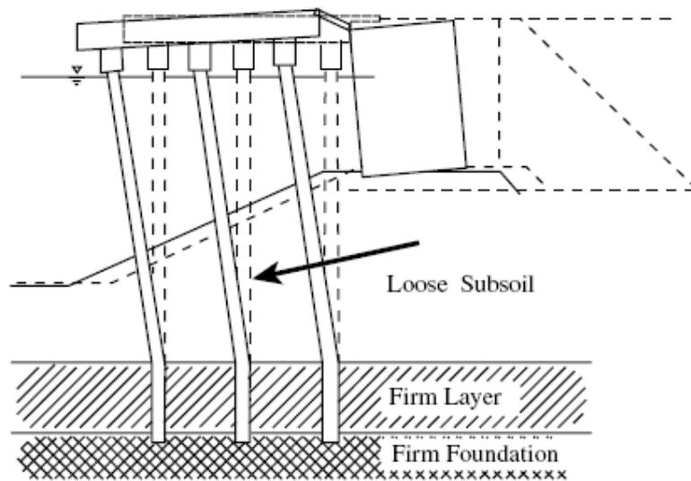
Figure 3.8. Damage due to localized ground movement (Balkema, 2001)
