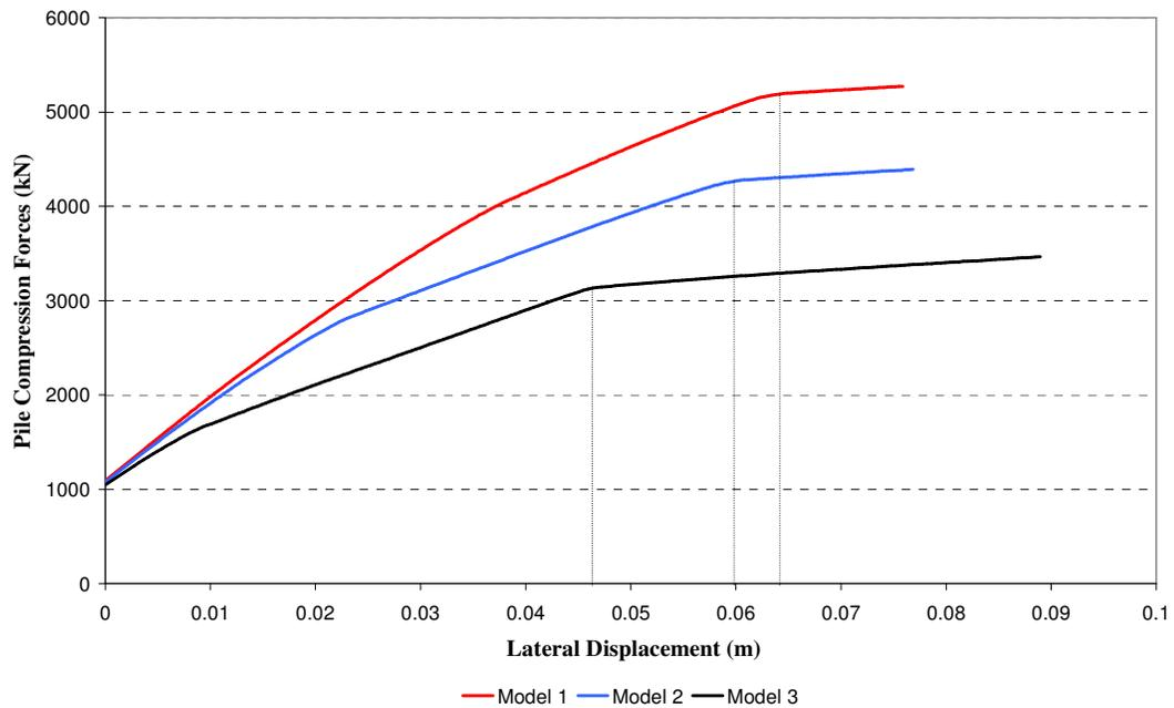
Figure 8.17. Variation of compression forces of the pile for %10 /50 earthquake event at a pier having batter piles with an inclination of  $1/4$ , with respect to lateral deformation and strength levels
