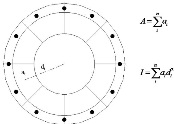
Figure 8.6. Fiber model of a reinforced concrete section
