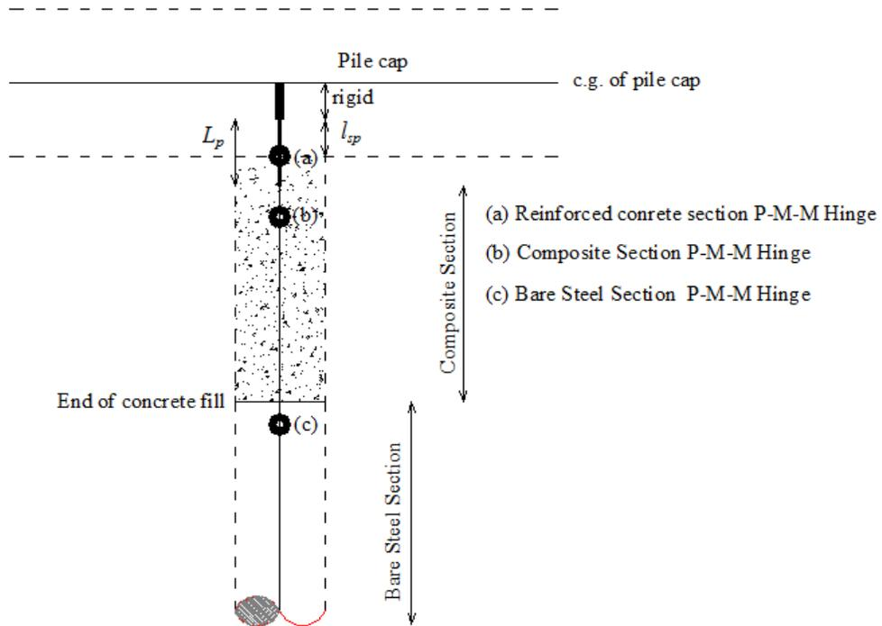
Figure 5.1. Structural model at the pile top
