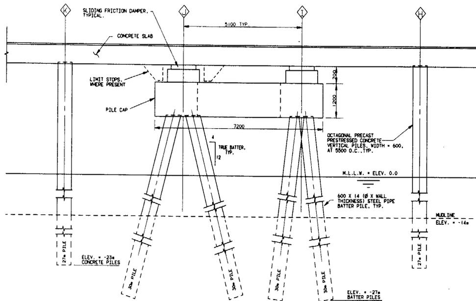
Figure 6.1. Partial wharf cross section (Zmuda *et al*, 1995)
