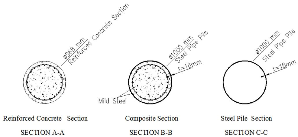
Figure 8.4. Plan view of pile sections
