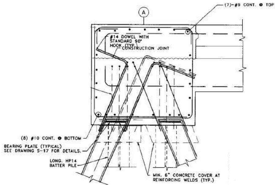
Figure 4.18. Alternative steel pile connections of a H-section pile (Roder, 2002)
