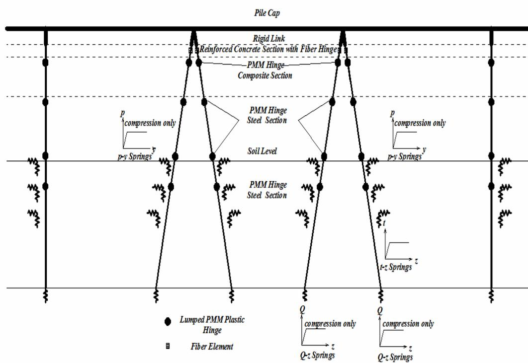
Figure 8.5. 2-Dimensional analysis model of generic pier
