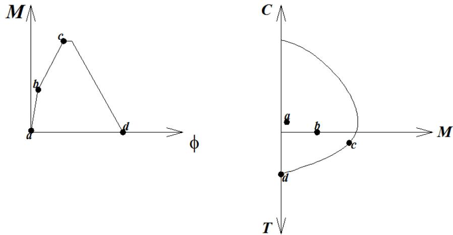
Figure 8.18. Yielding mechanism of pile-to-cap-beam connection in tension
