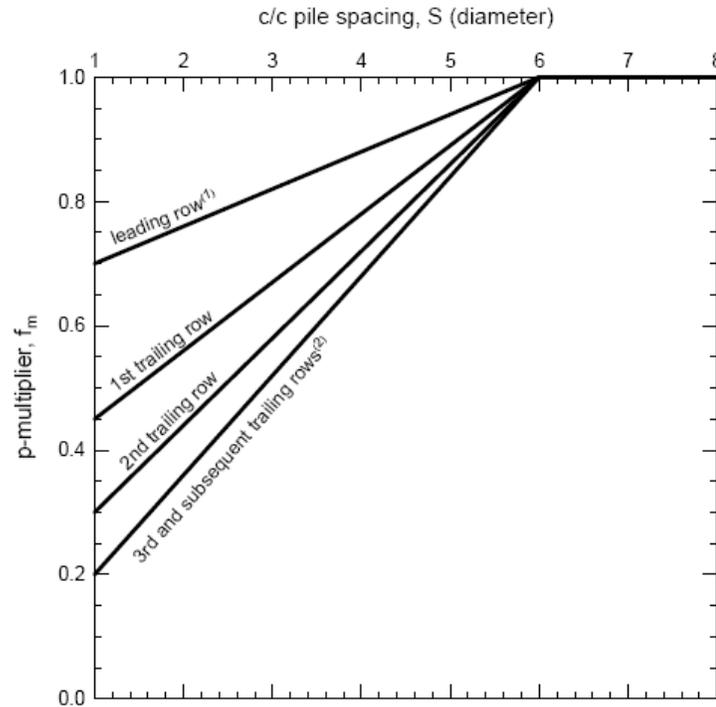
Figure 5.15. p-multiplier design curves (Mokwa et al, 2001)
