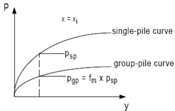
Figure 5.14. P-multiplier concept for lateral group analysis
