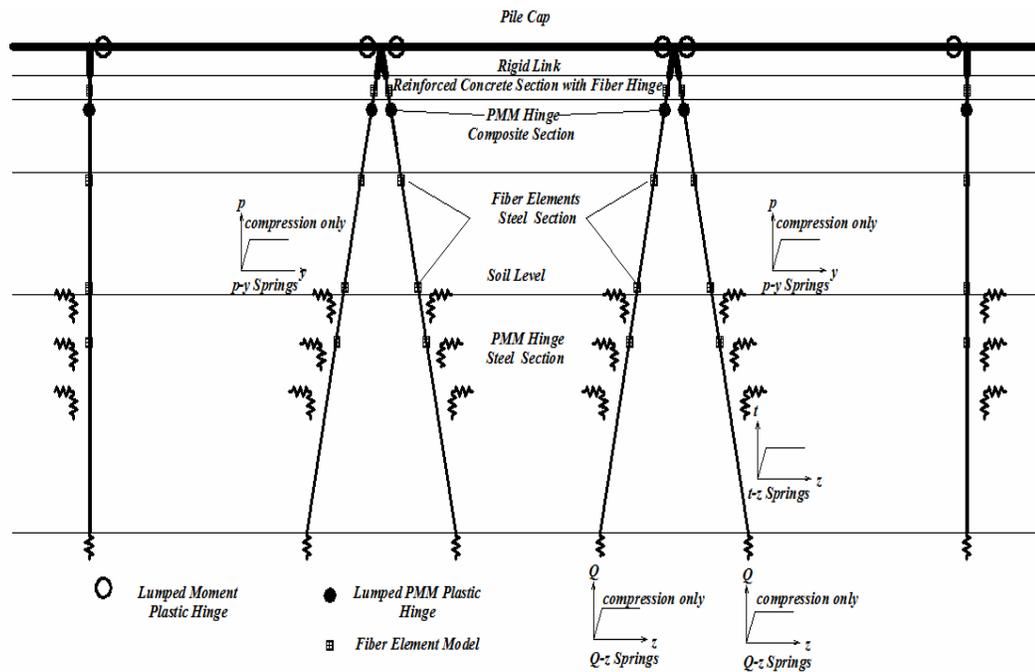
Figure 8.34. 2-Dimensional analysis model of generic pier
