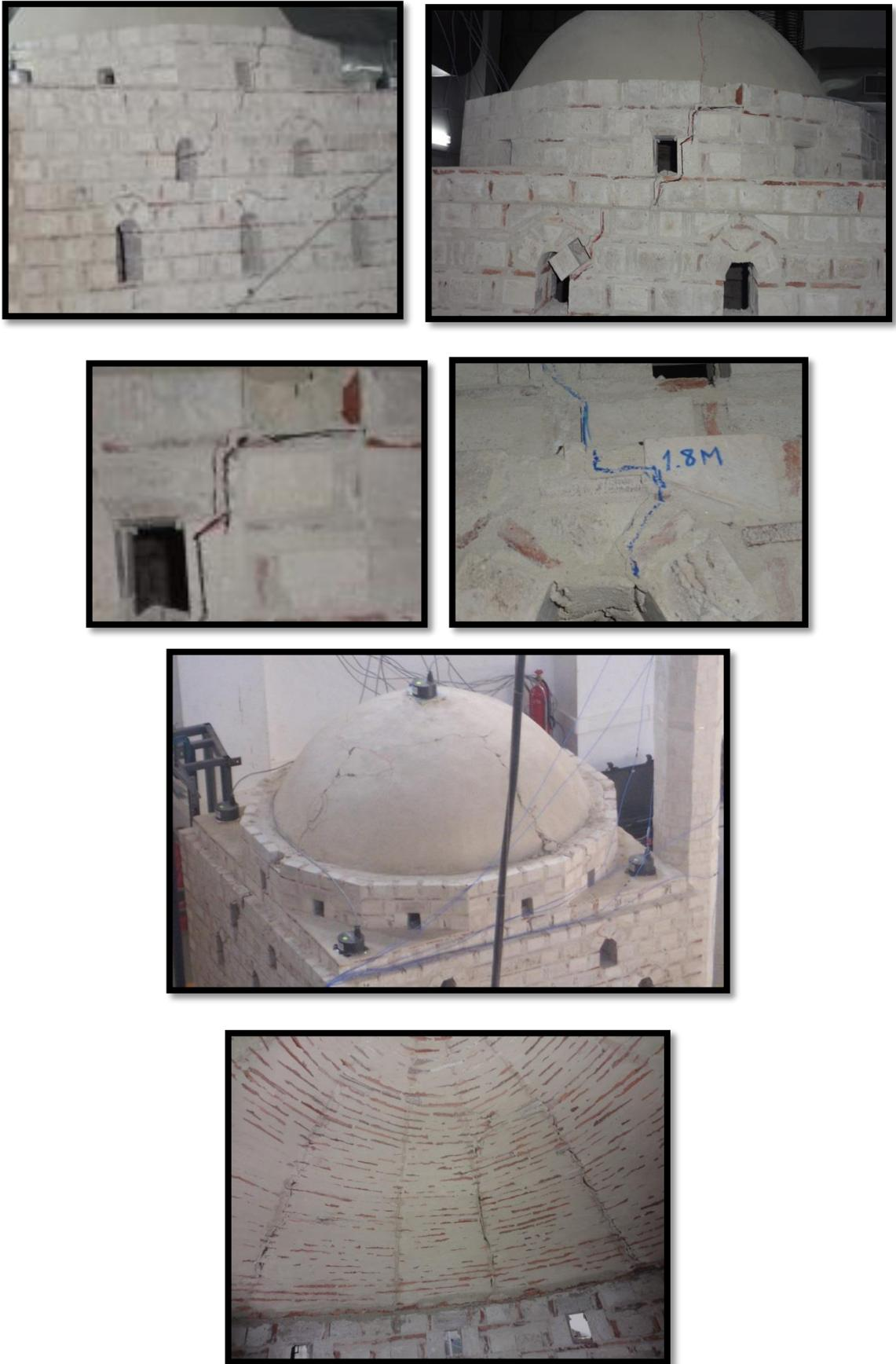
Figure 3.15. Damage to the drum, walls and dome.
