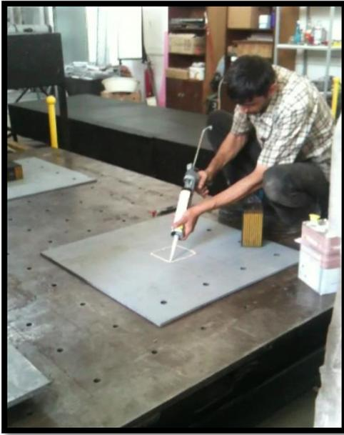
(a) Fixing steel plates to the table top
