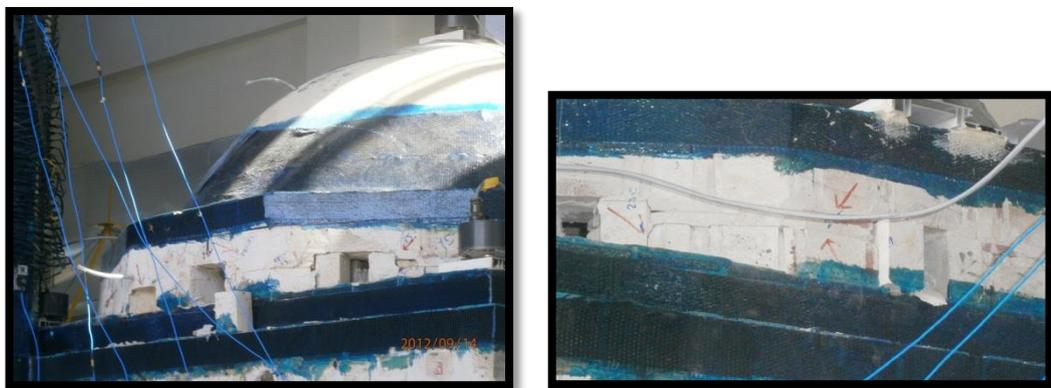
Figure 3.19. Damage to the strengthened model, details from the windows and the dome base.
