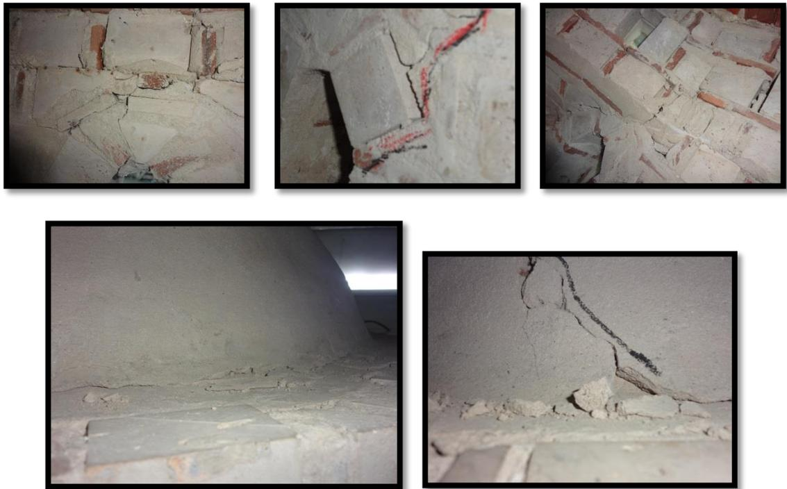
Figure 3.16. Damage to the experimental model, details from the windows and the dome base.
