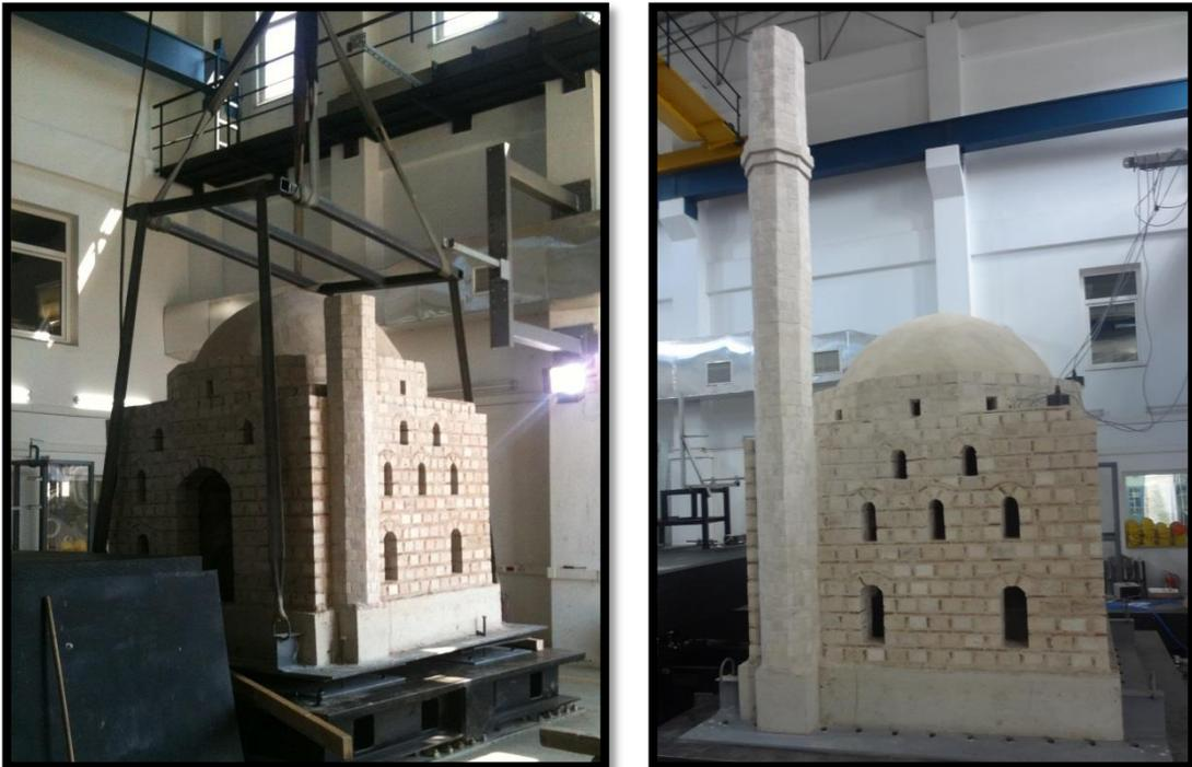
Figure 3.3. Images of 1:10 scale model of the Mustafa Paşa Mosque during its transfer on to the shake table.
