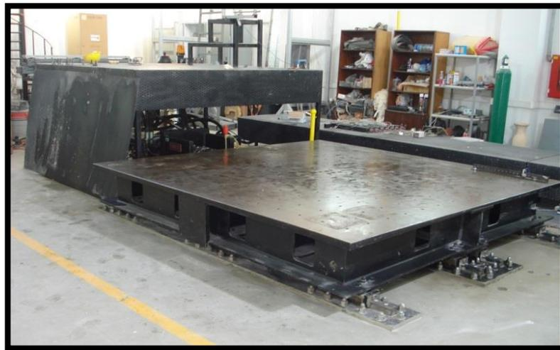
Figure 3.6. Image of shake table at the Department of Earthquake Engineering of Kandilli Observatory and Earthquake Research Institute of Boğaziçi University.
