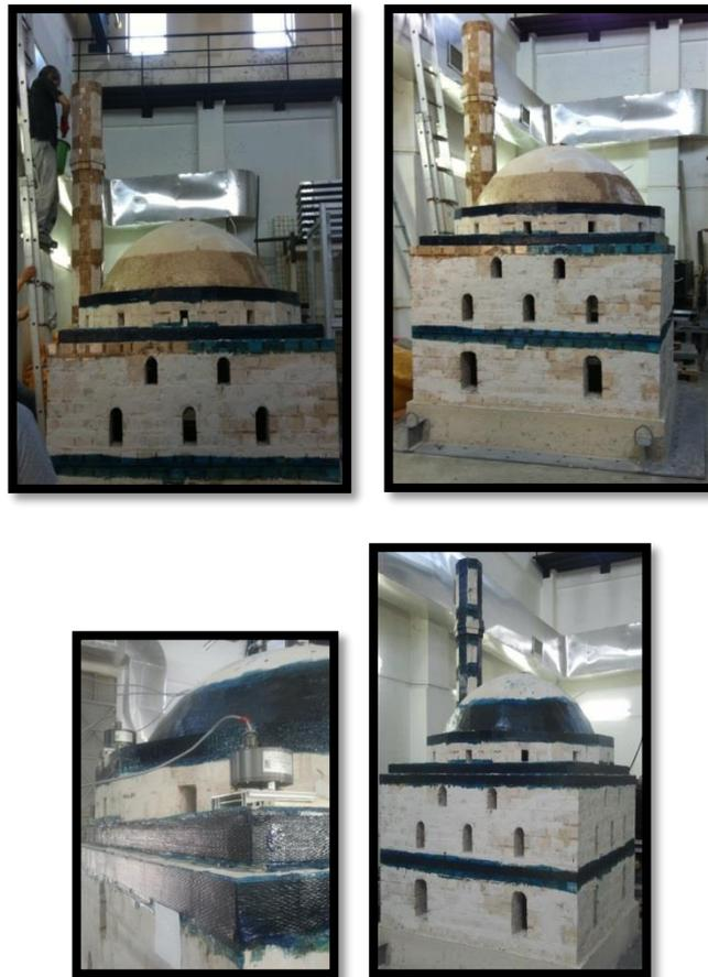
Figure 3.17. Images from FRP application (upper two images) and the strengthened model.
