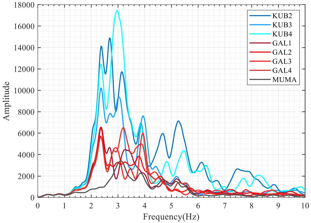
Figure 4.48. Horizontal-Y: FAS of the Mw5.7 Silivri offshore earthquake.
