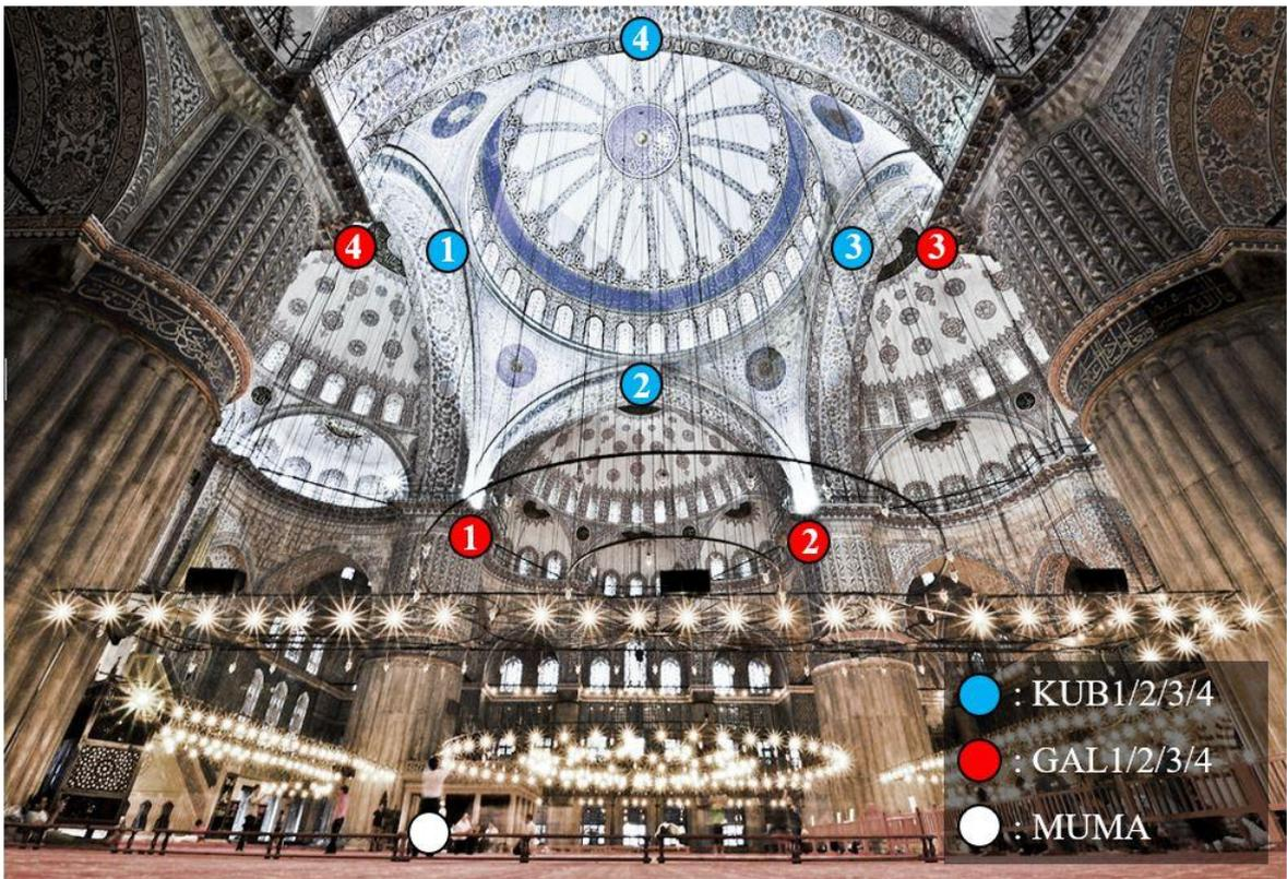
Figure 3.3. The mosque's interior view. The instrumentation layout exhibiting sensors at levels; dome, gallery and ground. (Taken and modified from KayYen's Flickr archive, July 2012)
