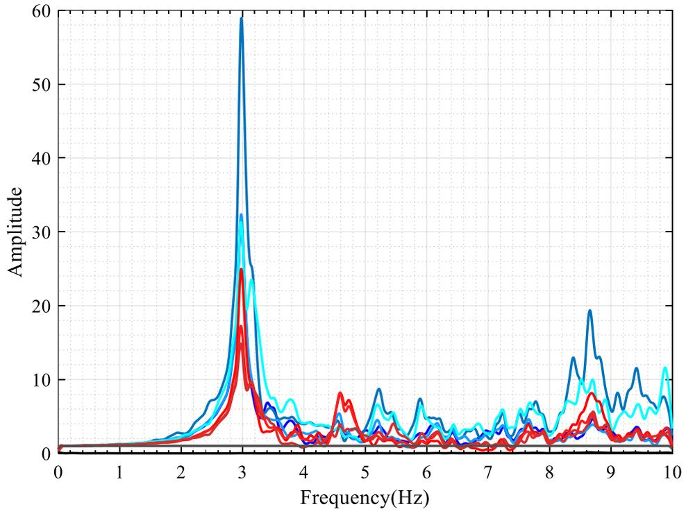
Figure 4.57. Horizontal-Y: FAS of the Mw6.1 Aegean Sea earthquake.
