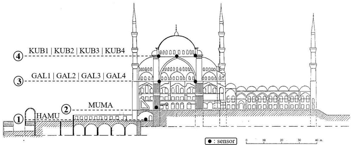
Figure 3.1. The section view from the eastern façade. Sensor groups' layout at four levels of height (Modified from Sayin, 1999).
