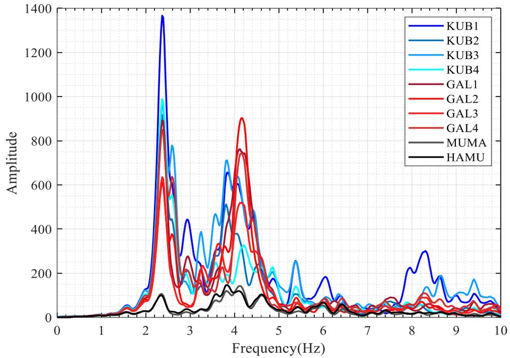
Figure 4.34. Horizontal-X: FAS of the Mw4.0 Cinarcik earthquake.
