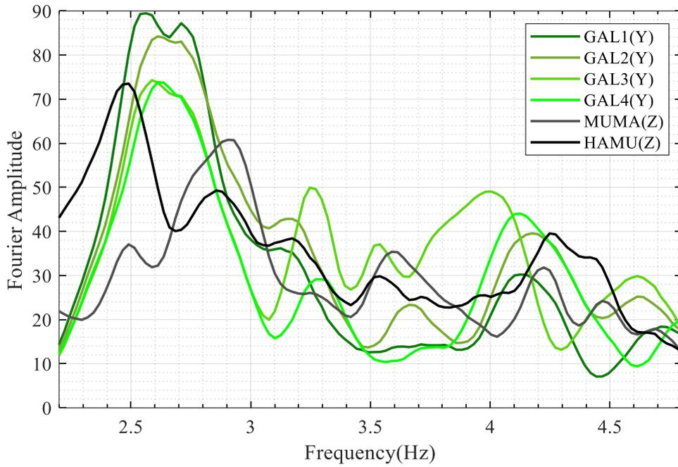
Figure 5.9. The  $M_w$ 4.4 Yalova Earthquake; FAS of vertical components of ground-level sensors and GAL sensors (amplitudes of horizontal Y were divided by 5).
