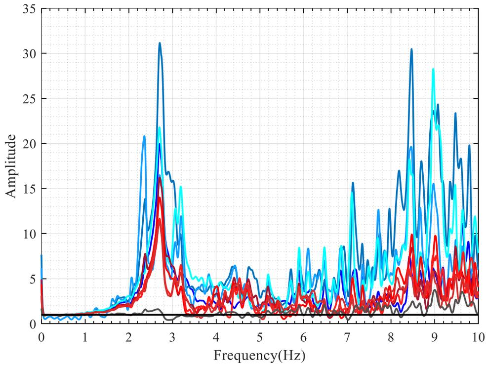
Figure 4.61. Horizontal-Y: TF of the Mw6.8 Aegean Sea earthquake.
