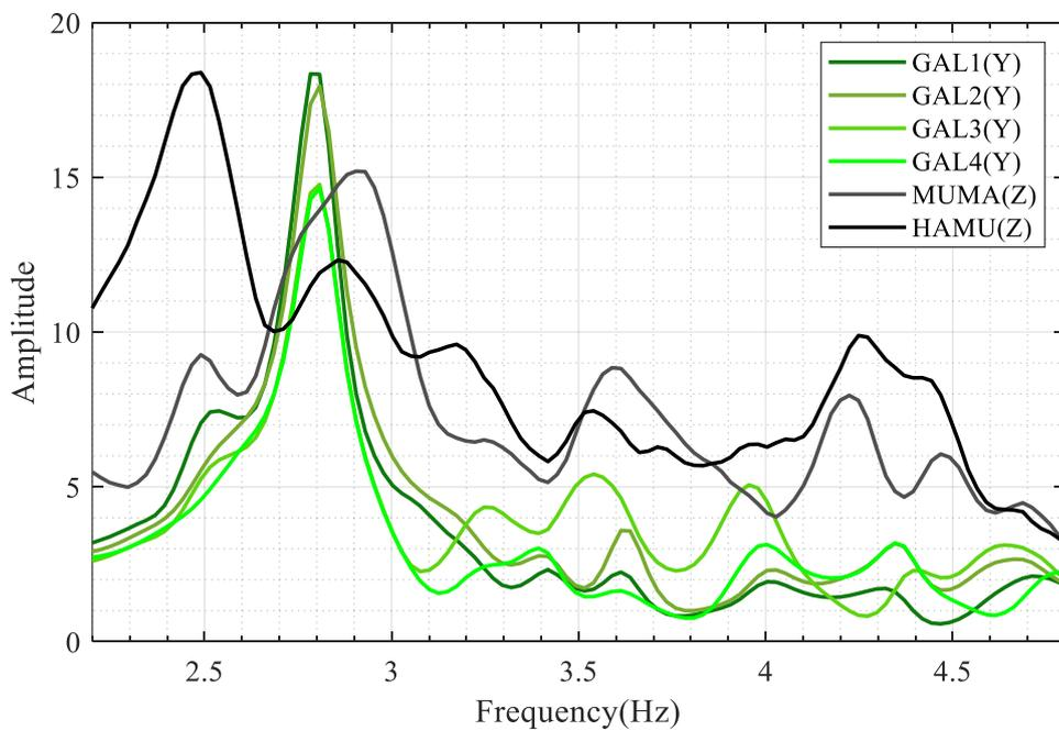
Figure 5.10. The  $M_w$ 4.4 Yalova Earthquake; FAS of HAMU and MUMA, and TF of GAL sensors (amplitudes of HAMU&MUMA were divided by 4).
