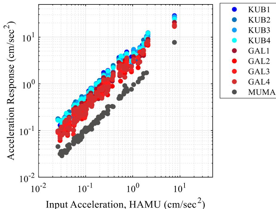
Figure 4.16. Response of the structure to basement-level acceleration amplitudes.
