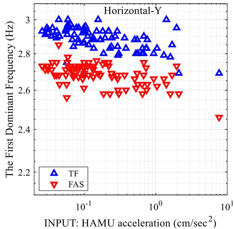
Figure 4.27. The change of the 2<sup>nd</sup> modal frequency with mean accelerations of HAMU.
