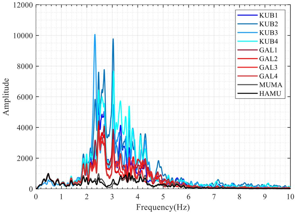
Figure 4.60. Horizontal-Y: FAS of the Mw6.8 Aegean Sea earthquake.
