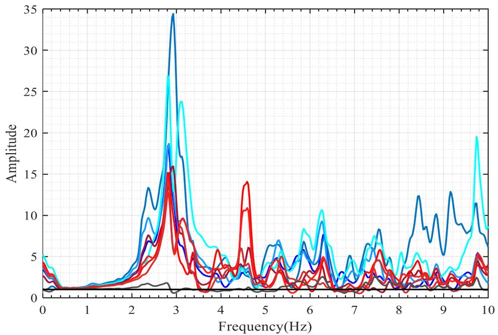
Figure 4.41. Horizontal-Y: TF of the Mw4.3 Kazikli earthquake.
