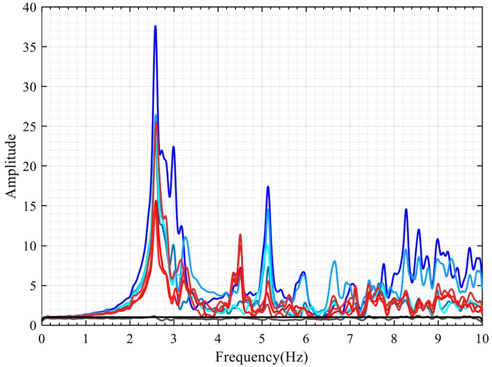
Figure 4.55. Horizontal-X: TF of the Mw6.1 Aegean Sea earthquake.
