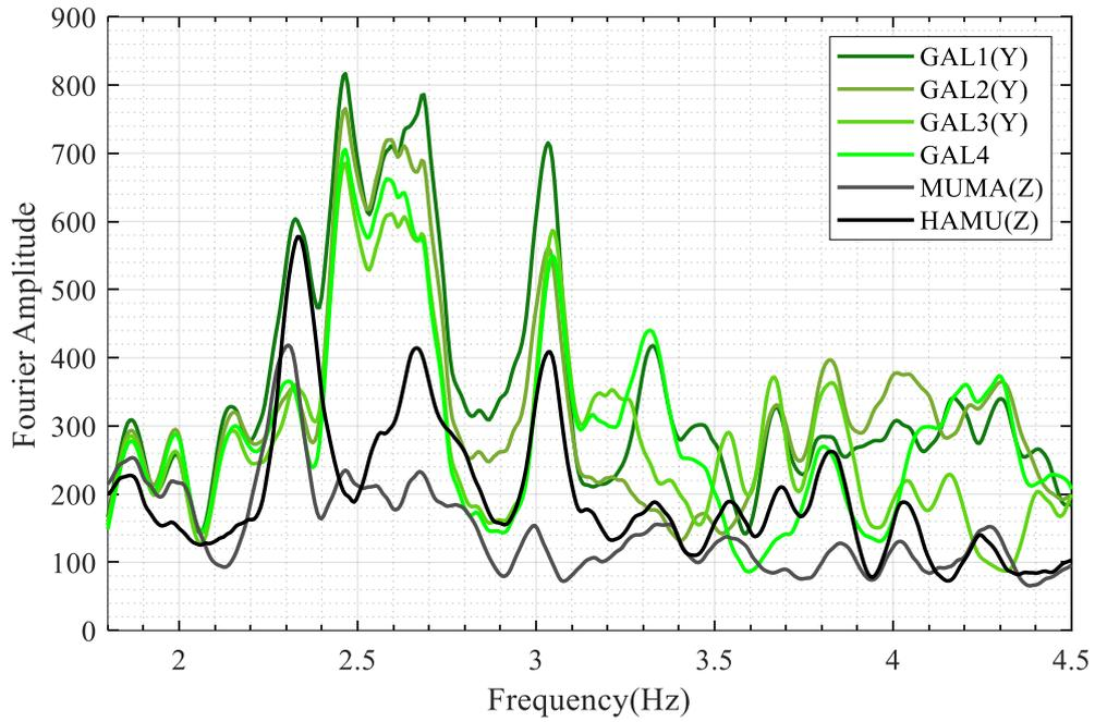
Figure 5.4. The  $M_w6.8$  Aegean Sea Earthquake; FAS of vertical components of ground level sensors and GAL sensors (amplitudes of horizontal Y were divided by 5).
