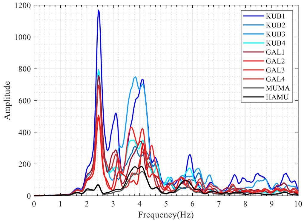
Figure 4.38. Horizontal-X: FAS of the Mw4.3 Kazikli earthquake.
