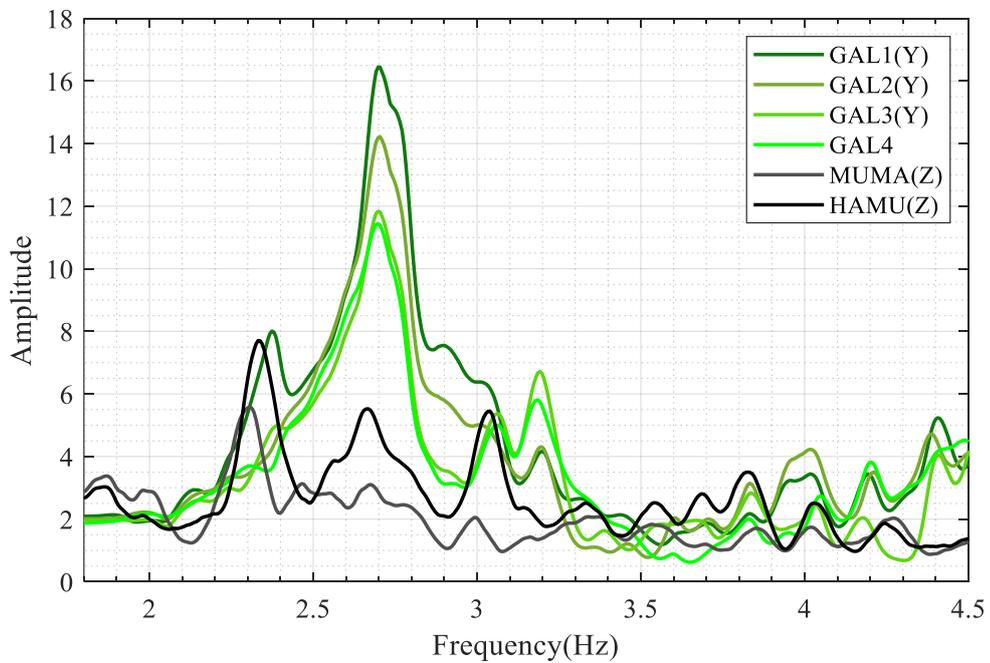
Figure 5.5. The  $M_w6.8$  Aegean Sea Earthquake; FAS of HAMU and MUMA, and TF of GAL sensors (amplitudes of HAMU&MUMA were divided by 75).
