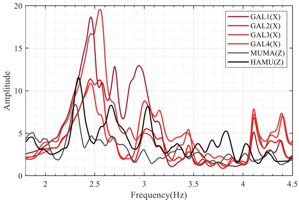
Figure 5.3. The  $M_w6.8$  Aegean Sea Earthquake; FAS of HAMU and MUMA, and TF of GAL sensors (amplitudes of HAMU&MUMA were divided by 50).
