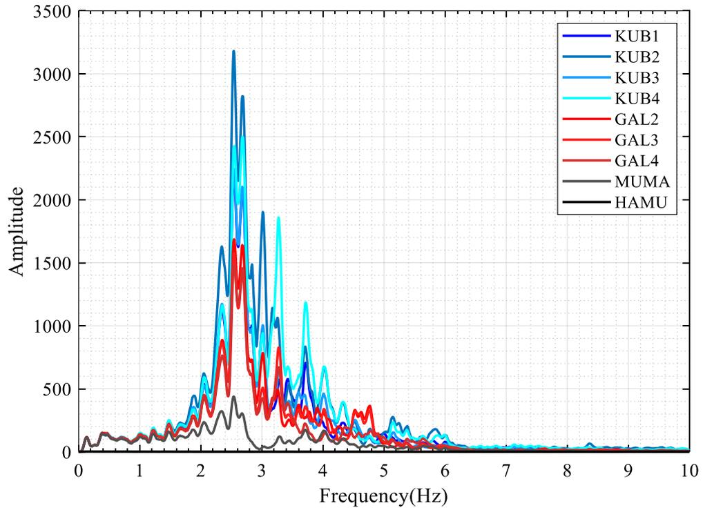
Figure 4.56. Horizontal-Y: FAS of the Mw6.1 Aegean Sea earthquake.
