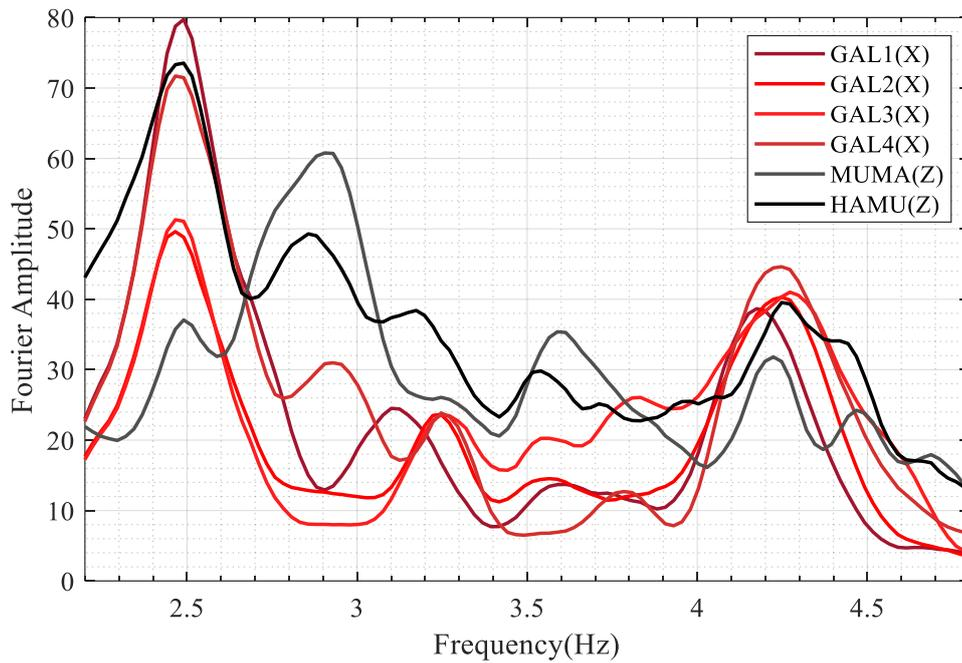
Figure 5.7. The  $M_w$ 4.4 Yalova Earthquake; FAS of vertical components of ground level sensors and GAL sensors (amplitudes of HAMU&MUMA were divided by 20).
