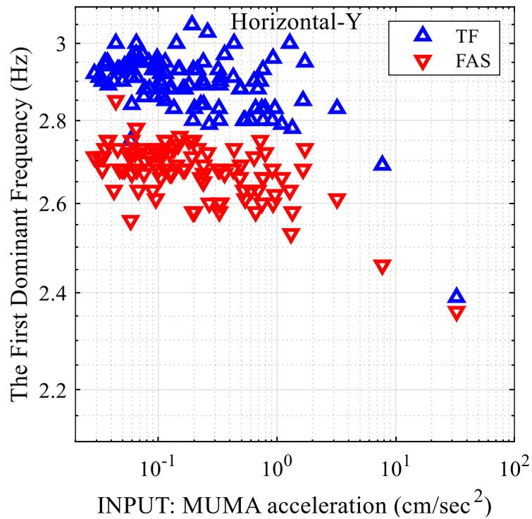
Figure 4.25. The change of the 2<sup>nd</sup> modal frequency with mean accelerations of MUMA.
