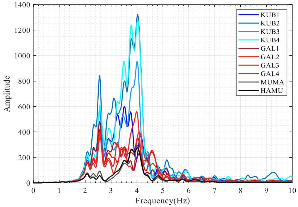
Figure 4.32. Horizontal-Y: FAS of the Mw3.9 Marmara Sea earthquake.
