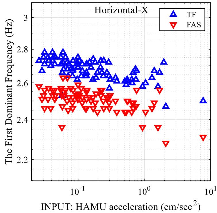
Figure 4.26. The change of the 1<sup>st</sup> modal frequency with mean accelerations of HAMU.
