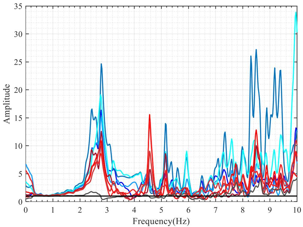
Figure 4.33. Horizontal-Y: TF of the Mw3.9 Marmara Sea earthquake.
