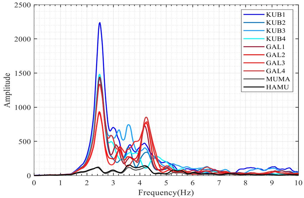
Figure 4.42. Horizontal-X: FAS of the  $M_w$ 4.4 Yalova earthquake.
