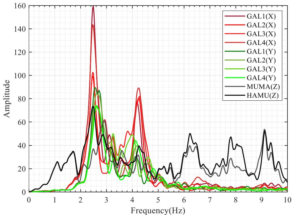
Figure 5.6. The  $M_w$ 4.4 Yalova Earthquake; FAS of vertical components of ground level sensors, HAMU and MUMA, and horizontal components of GAL sensors (amplitudes of horizontal X and Y were divided by 10).
