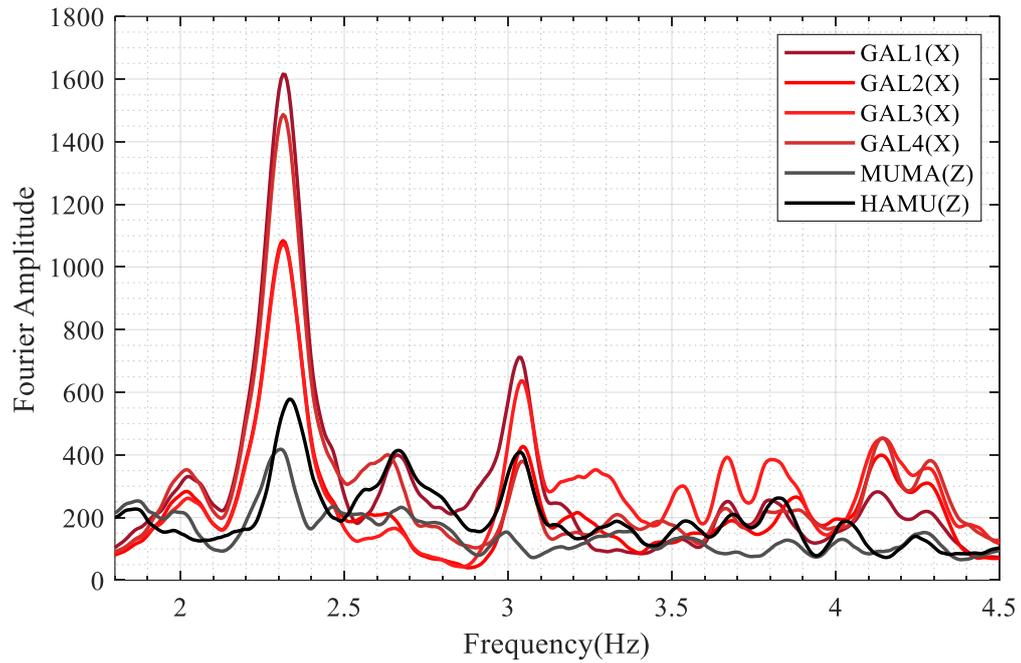
Figure 5.2. The  $M_w6.8$  Aegean Sea Earthquake; FAS of vertical components of ground level sensors and GAL sensors (amplitudes of horizontal X were divided by 8).
