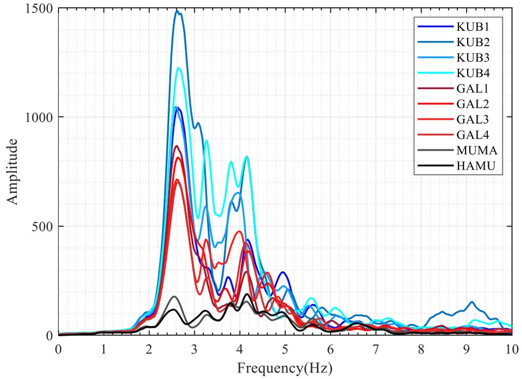
Figure 4.44. Horizontal-Y: FAS of the Mw4.4 Yalova earthquake.
