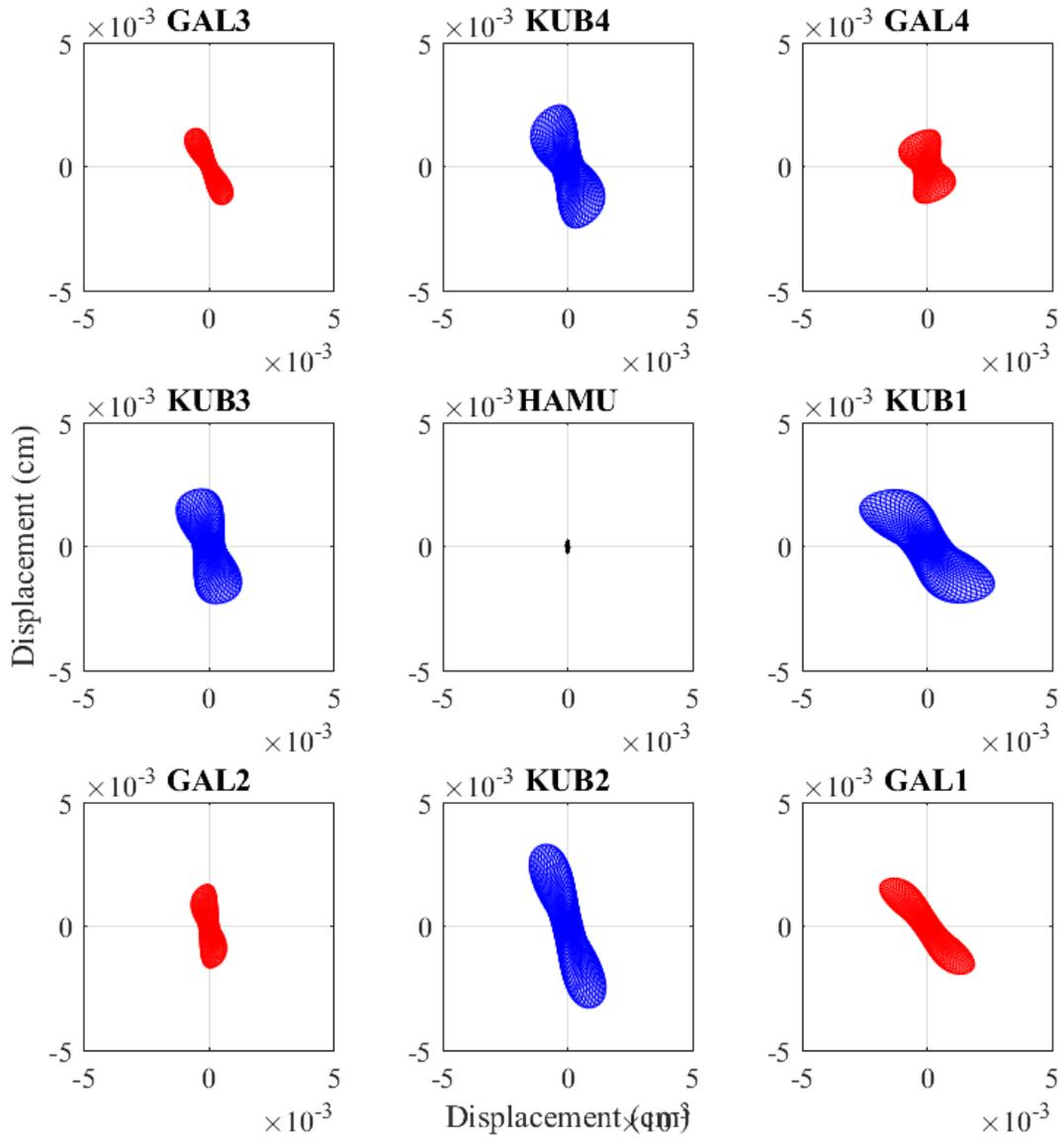
Figure 4.66. The 1<sup>st</sup> mode shape (lateral) observed during the Mw4.3 Kazikli earthquake.
