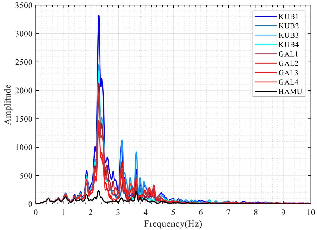
Figure 4.46. Horizontal-X: FAS of the  $M_w$ 5.7 Silivri offshore earthquake.
