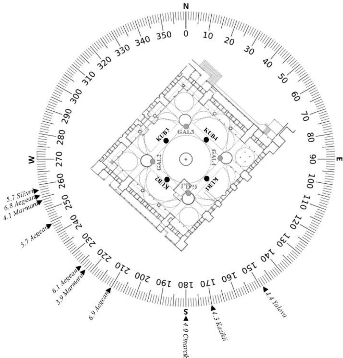
Figure 4.63. Origins of the selected earthquakes with respect to the mosque.
