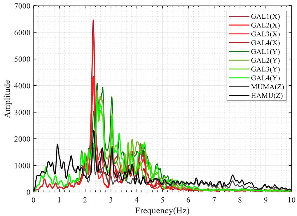
Figure 5.1. The  $M_w6.8$  Aegean Sea Earthquake; FAS of vertical components of ground level sensors, HAMU and MUMA (amplitudes were magnified by 4), and horizontal components of GAL sensors (amplitudes of horizontal X were divided by 2).
