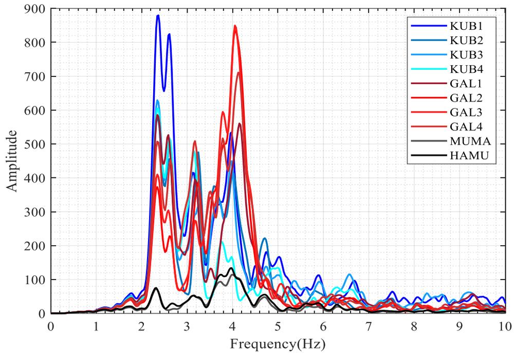
Figure 4.30. Horizontal-X: FAS of the Mw3.9 Marmara Sea earthquake.
