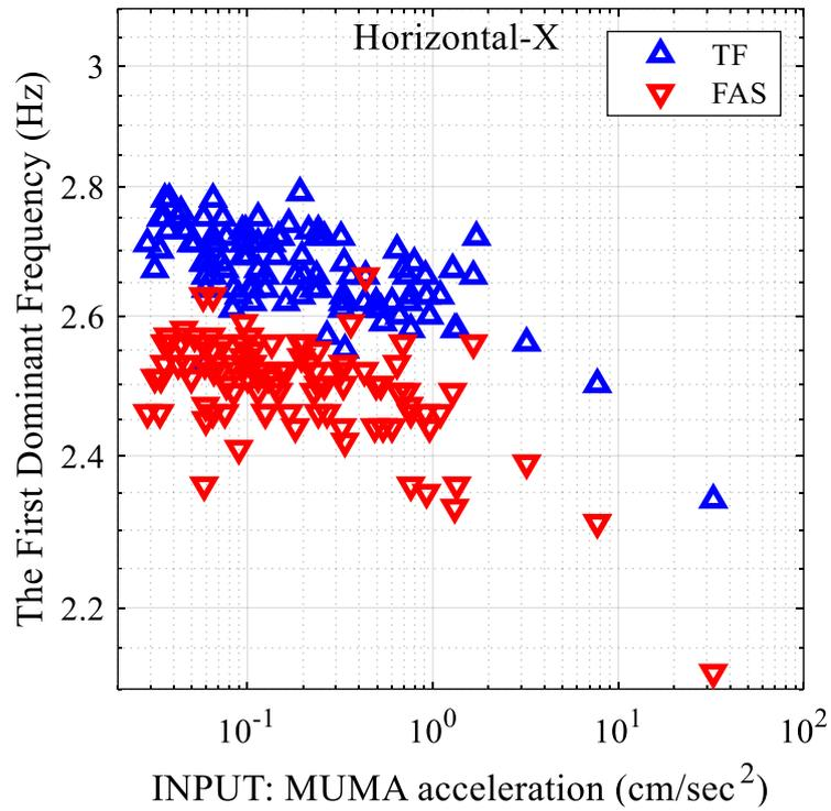
Figure 4.24. The change of the 1<sup>st</sup> modal frequency with mean accelerations of MUMA.
