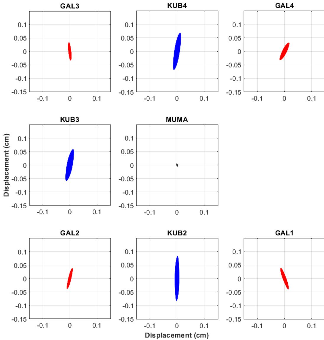
Figure 4.67. The 2<sup>nd</sup> mode shape (lateral) observed during the Mw5.7 Silivri offshore earthquake.
