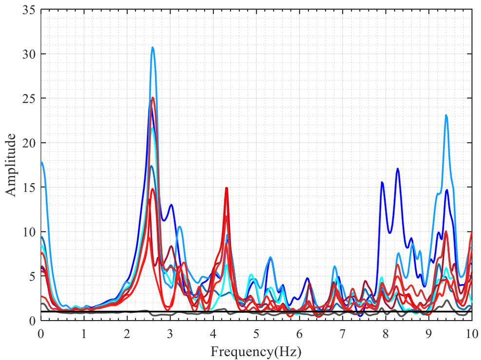
Figure 4.35. Horizontal-X: TF of the Mw4.0 Cinarcik earthquake.
