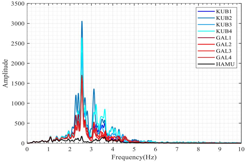
Figure 4.52. Horizontal-Y: FAS of the Mw5.7 Aegean Sea earthquake.
