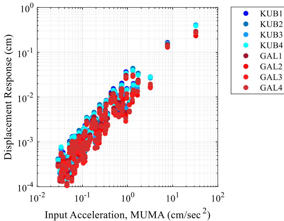
Figure 4.19. Change in displacements with ground-level acceleration amplitudes.
