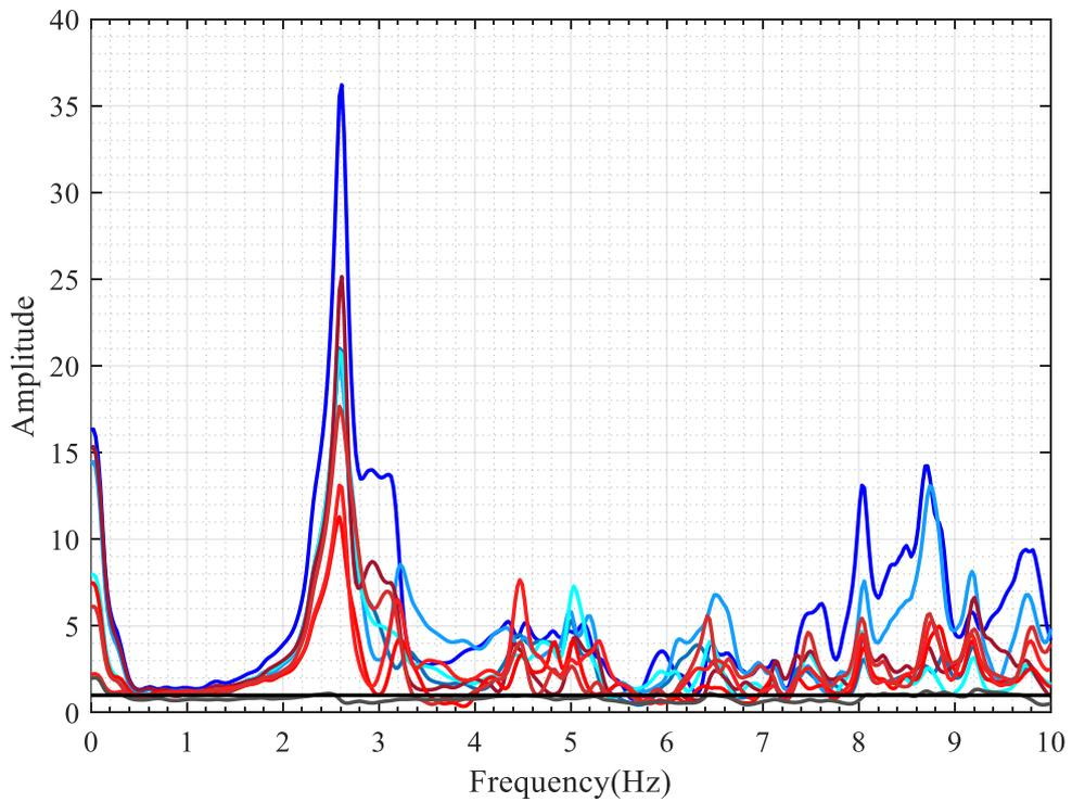
Figure 4.39. Horizontal-X: TF of the Mw4.3 Kazikli earthquake.
