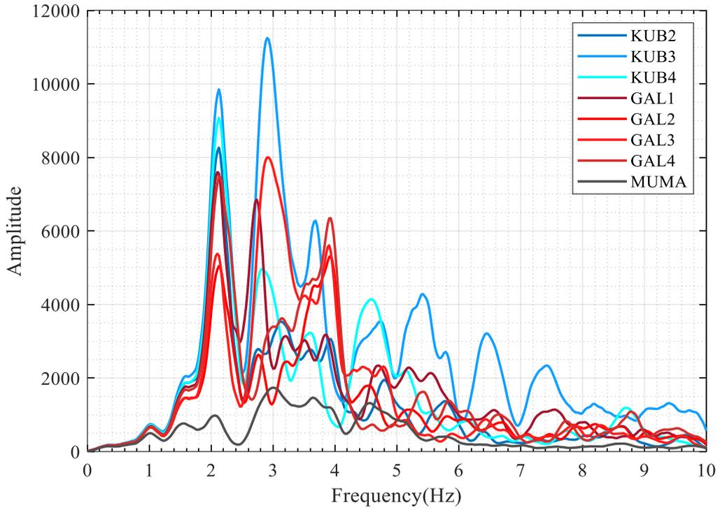
Figure 4.50. Horizontal-X: FAS of the Mw5.7 Aegean Sea earthquake.
