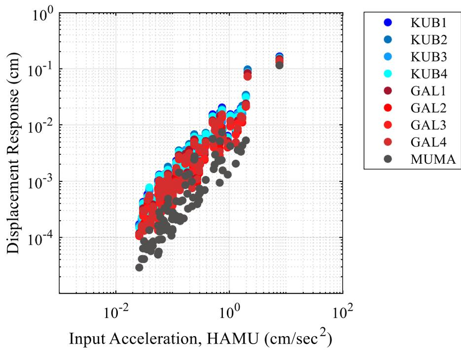
Figure 4.18. Change in displacements with basement-level acceleration amplitudes.
