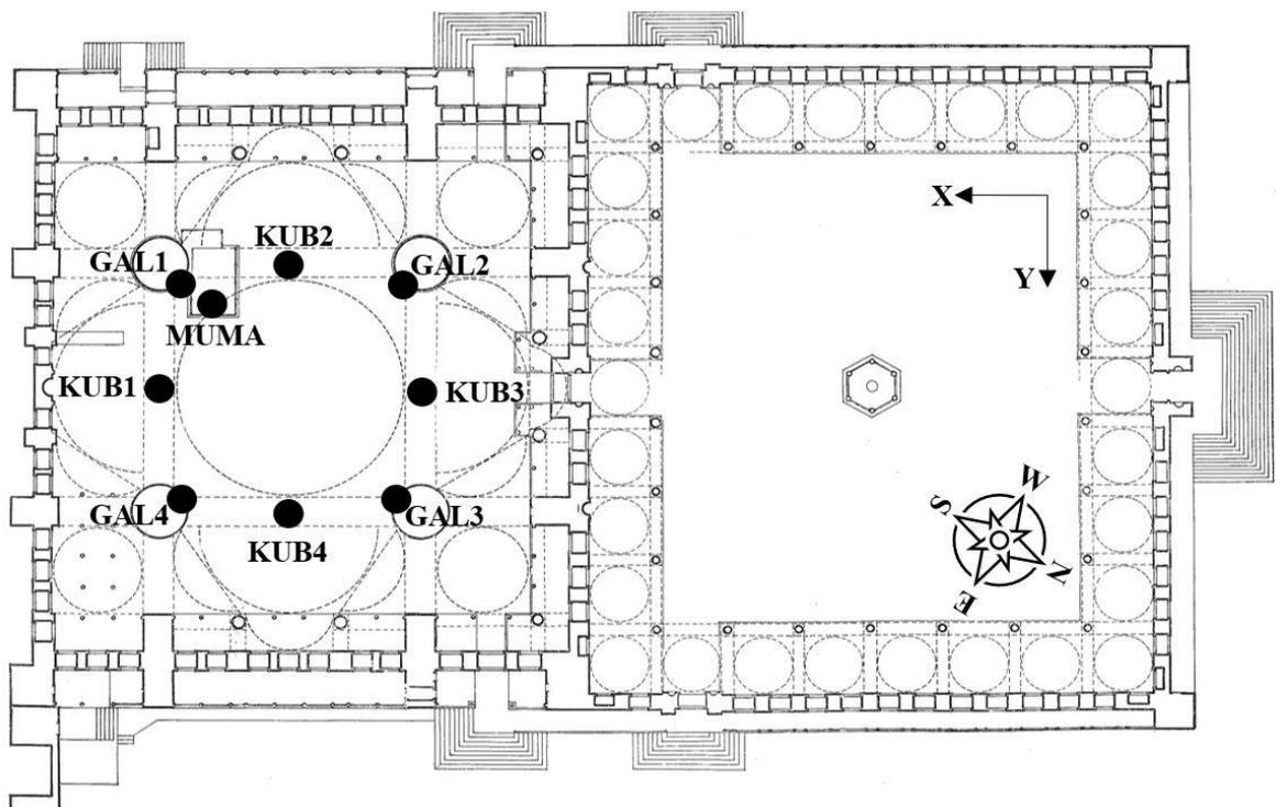
Figure 3.2. Sensors at dome-level, pillar-level and ground-level in the plan view (Modified from Nayır, 1975).
