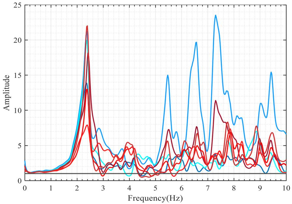
Figure 4.51. Horizontal-X: TF of the Mw5.7 Aegean Sea earthquake.
