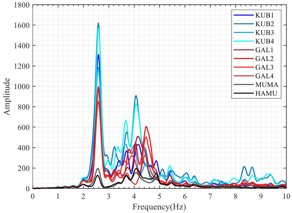
Figure 4.36. Horizontal-Y: FAS of the Mw4.0 Cinarcik earthquake.
