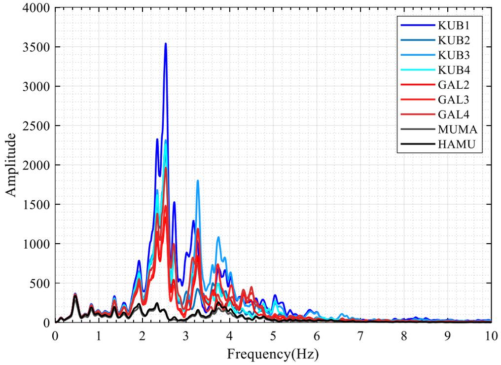
Figure 4.54. Horizontal-X: FAS of the Mw6.1 Aegean Sea earthquake.
