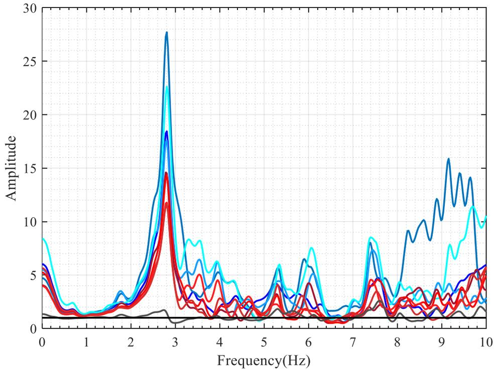
Figure 4.45. Horizontal-Y: TF of the Mw4.4 Yalova earthquake.
