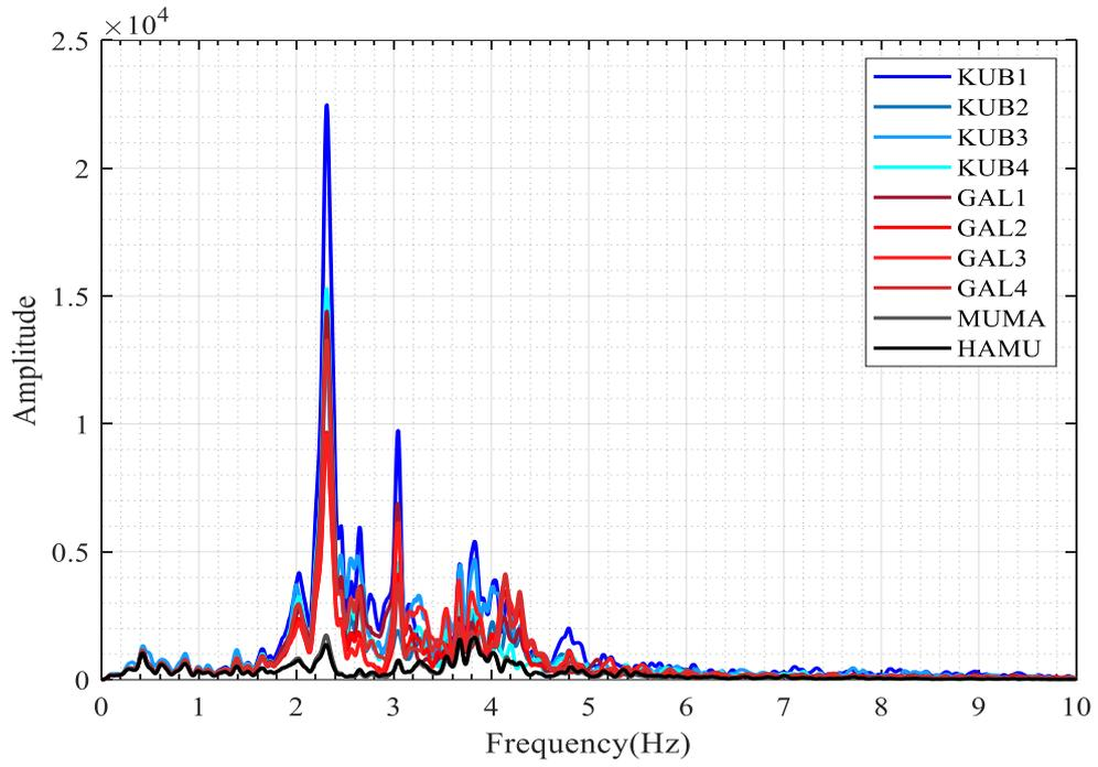
Figure 4.58. Horizontal-X: FAS of the Mw6.8 Aegean Sea earthquake.
