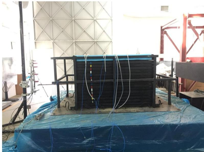
Figure 3.1. A General View of Shaking Table and Laminar Box.
