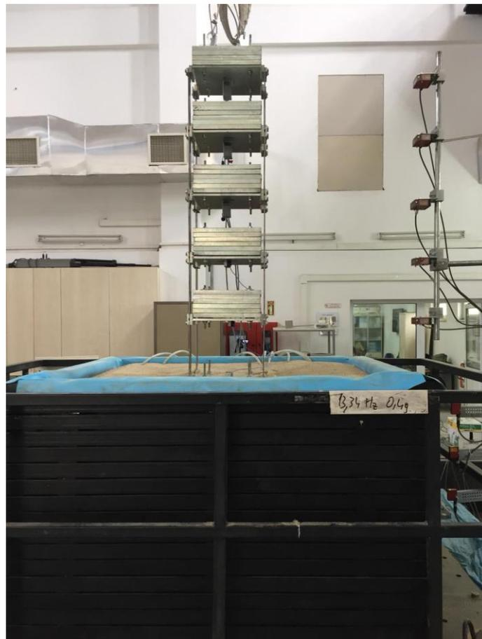
Figure 3.5. The Profile View of 5 Storey Scaled Building Model.
