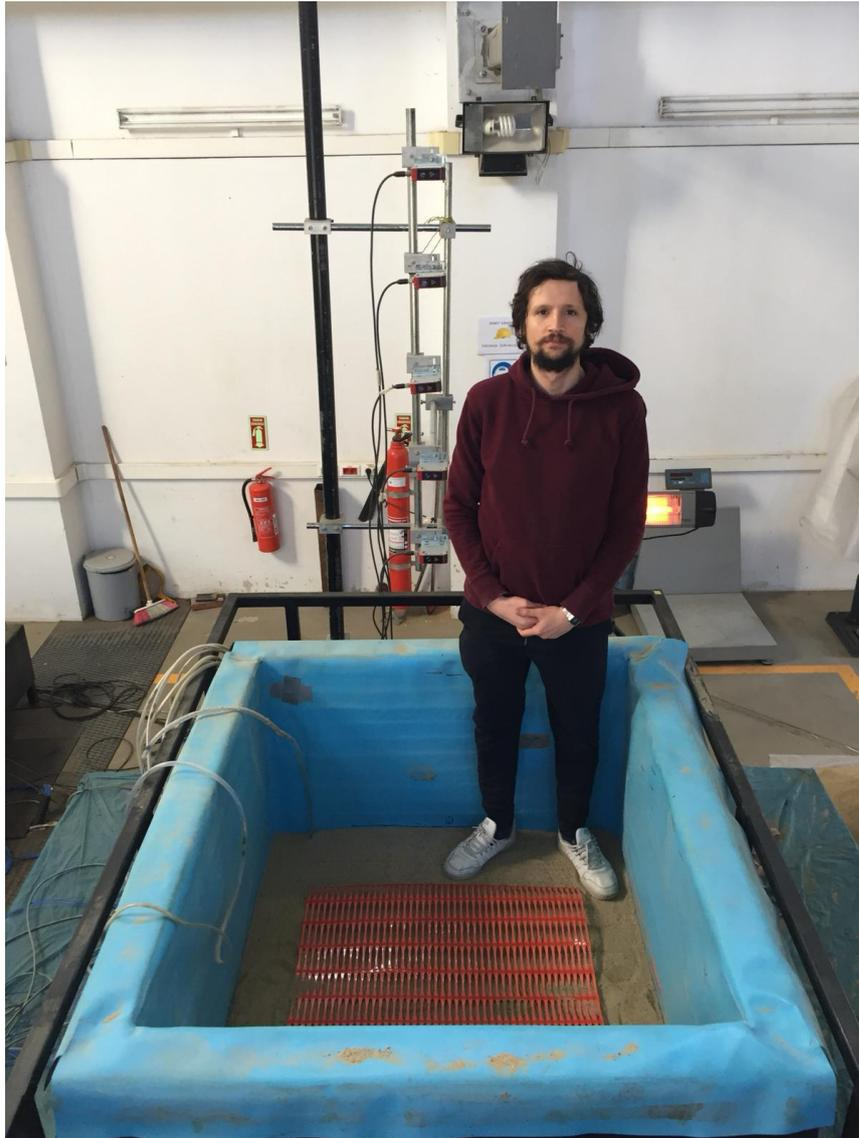
Figure 3.18. Soil Preparation Process of Model.
