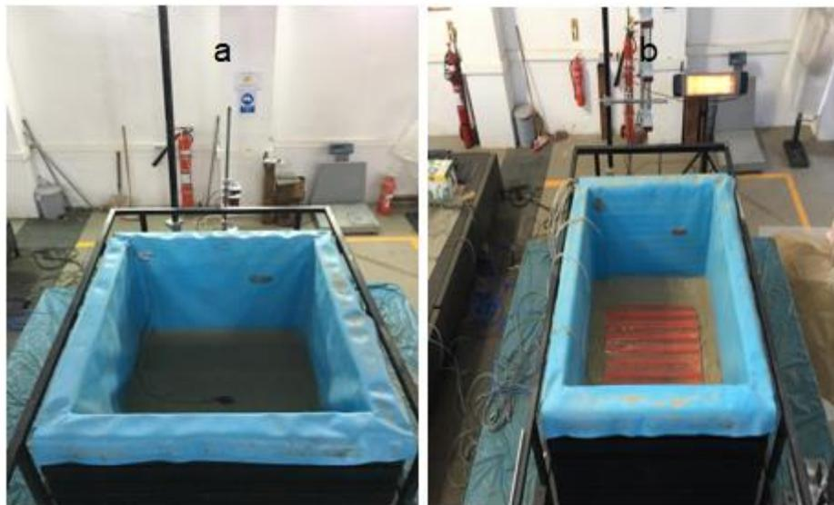
Figure 3.17. Soil Preparation Process of Experimental Model (a) Without Geogrid Reinforcement, (b) With Geogrid Reinforcement.
