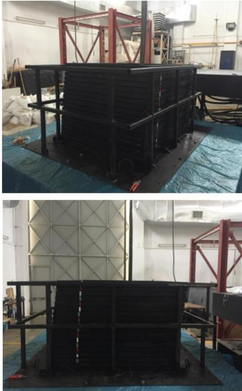
Figure 3.3. A Profile View of Laminar Box.
