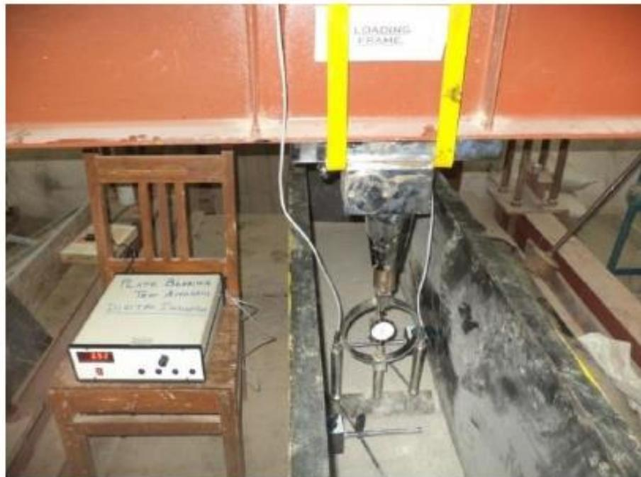
Figure 2.12. A General View of the Model Test Setup. (Yabu & Tripathi, 2013)
