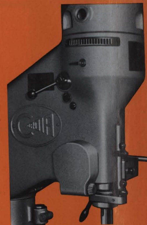
Lever for gear reversal, Control knob for pull back spring, oil sight glass
