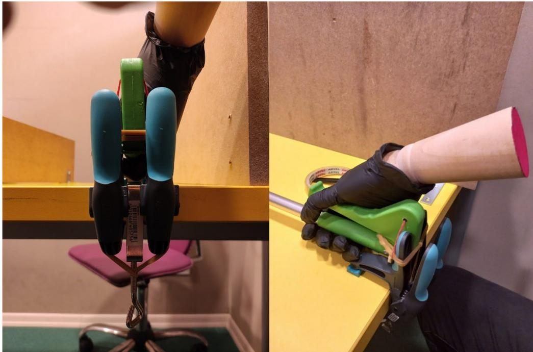
Figure 6. Tool-holding rubber hand mechanism enabling vertical mobility
