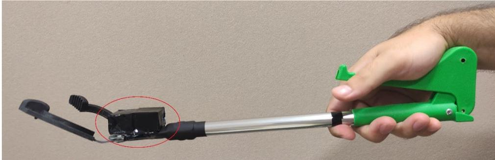
Figure 4. Prescribed grasp of (short) tool with added weight at distal end (in red circle)
