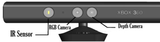
Figure 1.1. Kinect Sensor.
