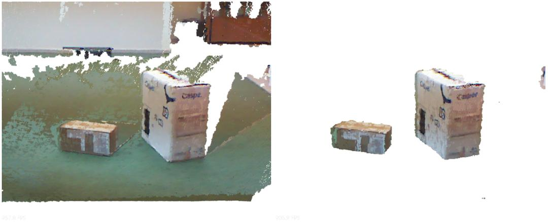
Figure 4.3. Left - Transformed and merged point clouds with manually selected keypoints. Right - Same scene fine tuned with ICP algorithm.
