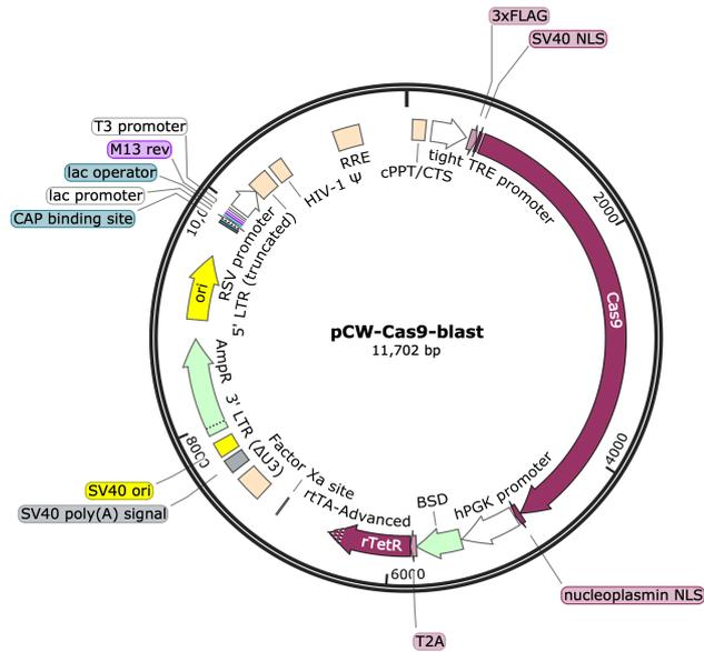
Figure A.3. Vector map of pCW-Cas9-blast (Addgene: 83481) plasmid that is used to generate pCW-dCpf1-blast plasmid (Habashy *et al.*, unpublished).
