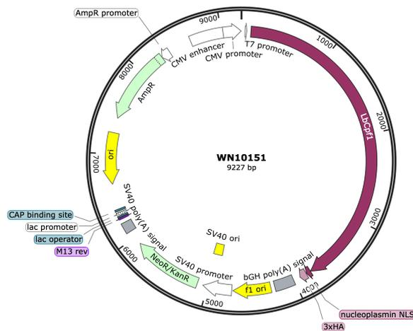
Figure A.6. Vector map of WN10151 plasmid (Addgene: 80441) that is used to generate pCW-dCpf1-blast plasmid (from Toth *et al.*, 2016).
