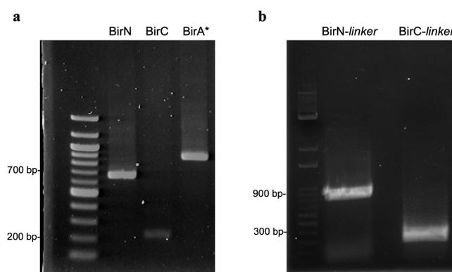
Figure 5.6. BirA\* is split into two halves via PCR reaction. (a) The sizes of BirN, BirC and full length BirA\* is indicated. (b) 3' linkers and homology arms added to BirN and BirC fragments added after the 2<sup>nd</sup> PCR reaction.
