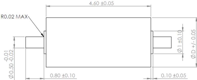
Figure E.1. Small scale end effector roller technical drawing.
