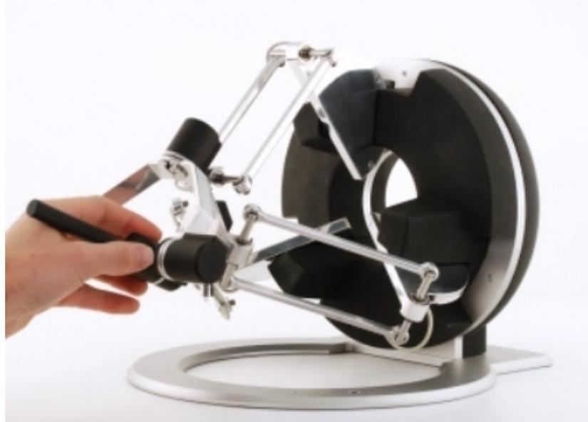
Figure 3.5. Force dimension Omega 6 haptic device.
