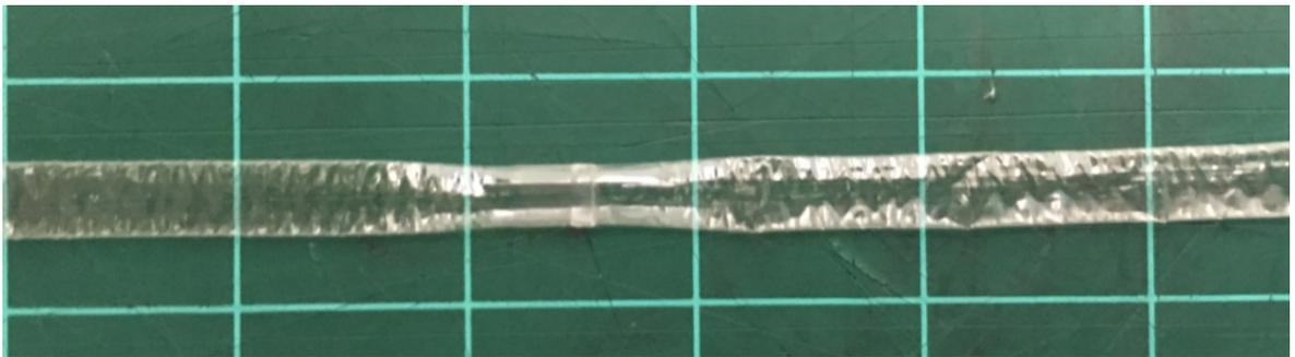
Figure 3.22. Medical PA12 balloon welded using method 3 as explained above. On the connection area conical features can be observed. As also seen in the figure melted material accumulated and generating additional thickness at the weld edge.
