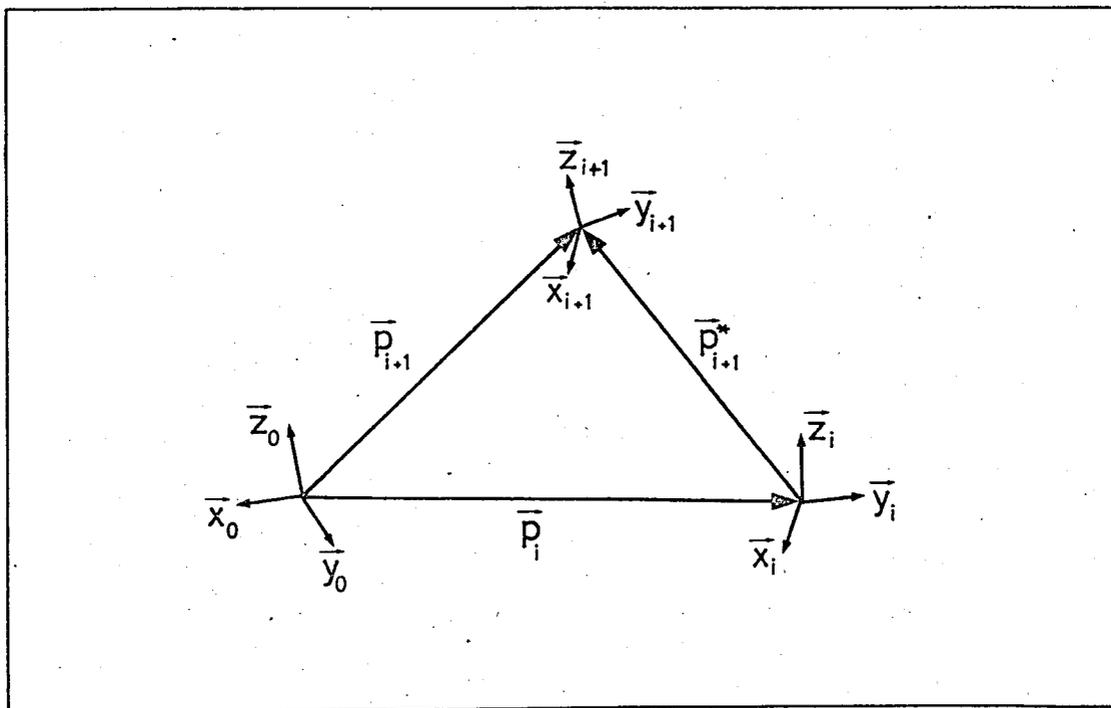
FIGURE 2.3 - Relationship between link coordinate systems.
