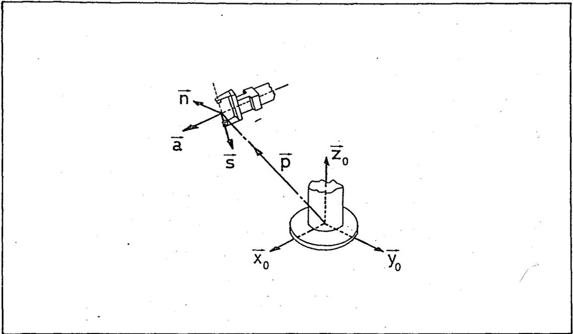
FIGURE 2.2 - Position and orientation vectors of the hand.
