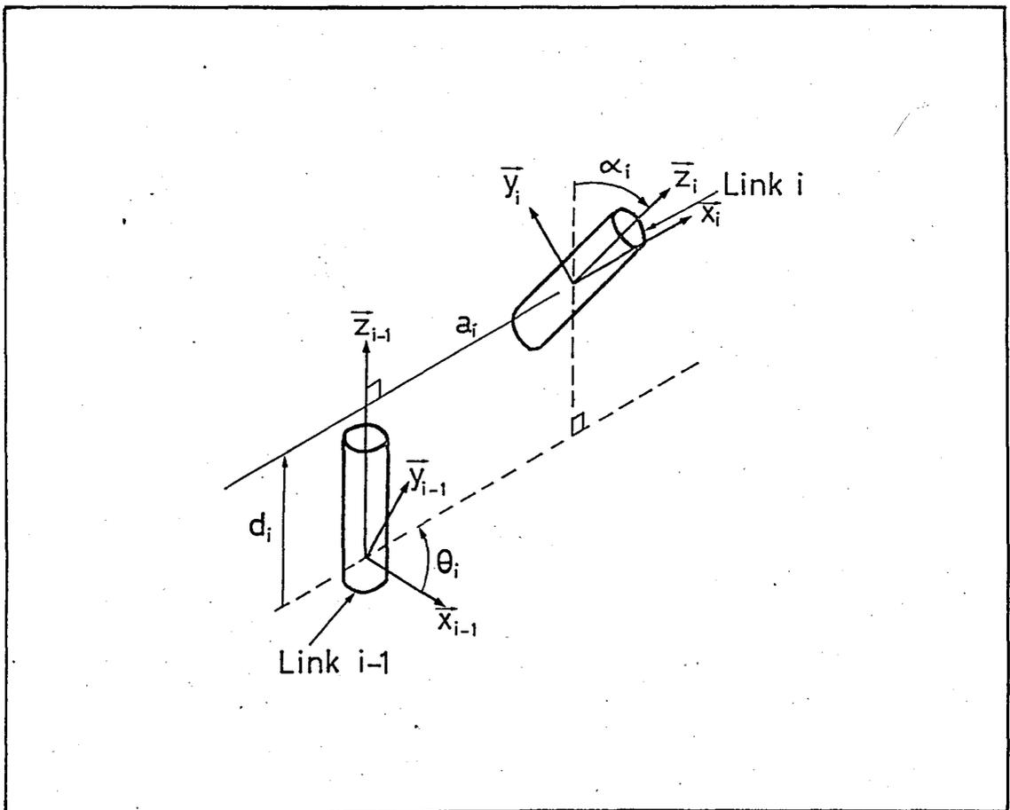
FIGURE 2.1 - Parameters relating adjacent coordinate systems.
