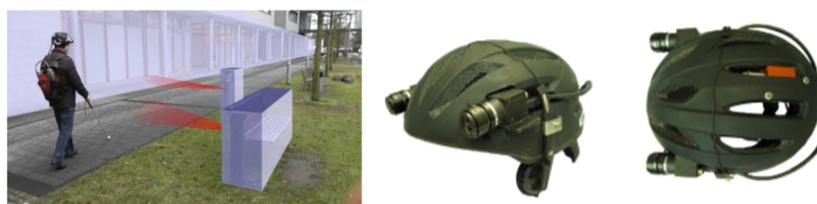
Figure 1.3. Smart helmet system that can detects obstacles and transmits them to user via headphone [36].
