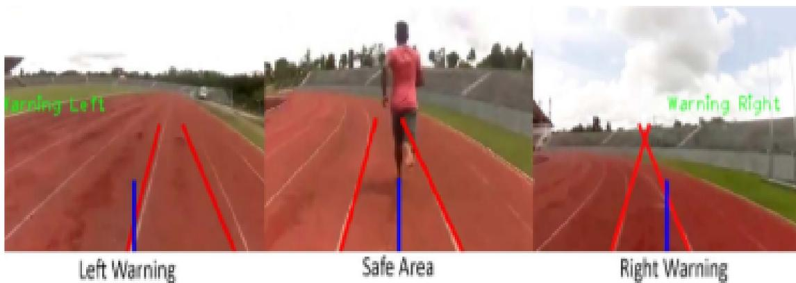
Figure 1.10. EyeVista track detection and warning [2].
