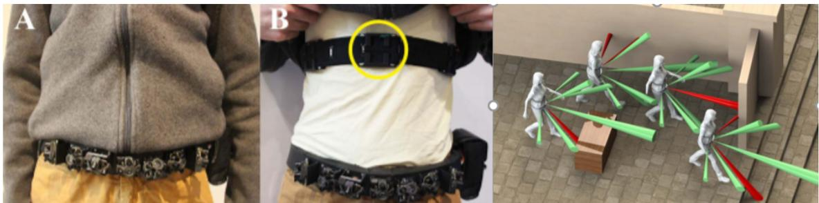
Figure 1.6. Sensor belt is located at bottom and haptic belt is located at top [41].
