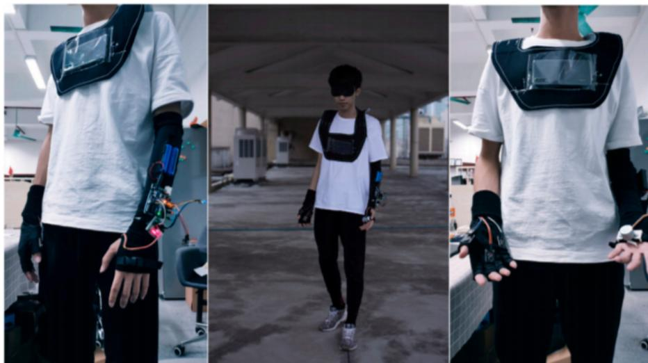
Figure 1.4. Dual channel human machine interaction system prototype [38].
