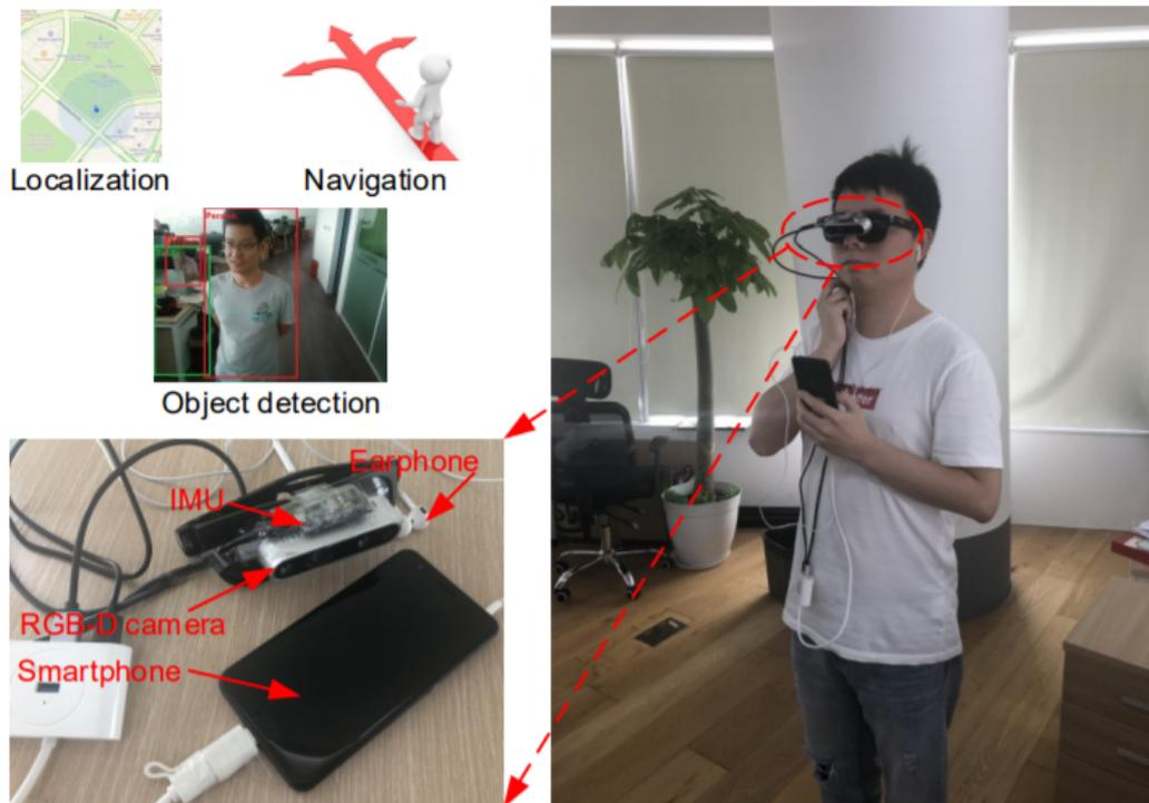
Figure 1.2. Prototype of CNN based wearable assistive device [29].
