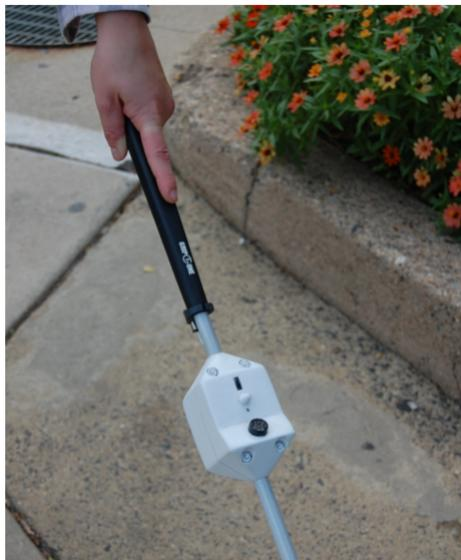
Figure 1.1. A traditional white cane fitted with the smart system [23].
